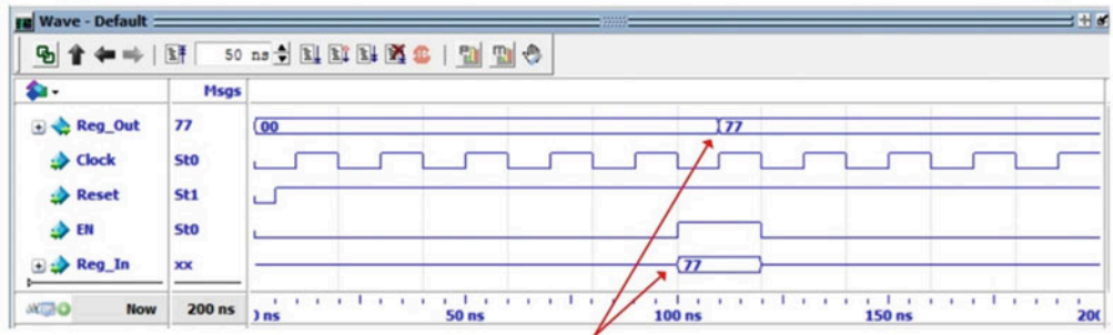
When Enabled ( EN =1), the register will latch in the input value on the rising edge of clock.
