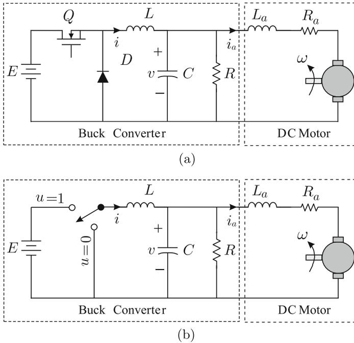
**Fig. 2.41** Electric diagram of the buck power converter-DC Motor system. (a) Construction of the buck power converter DC motor system using a transistor and a diode. (b) Ideal representation of the buck power converter DC motor system
