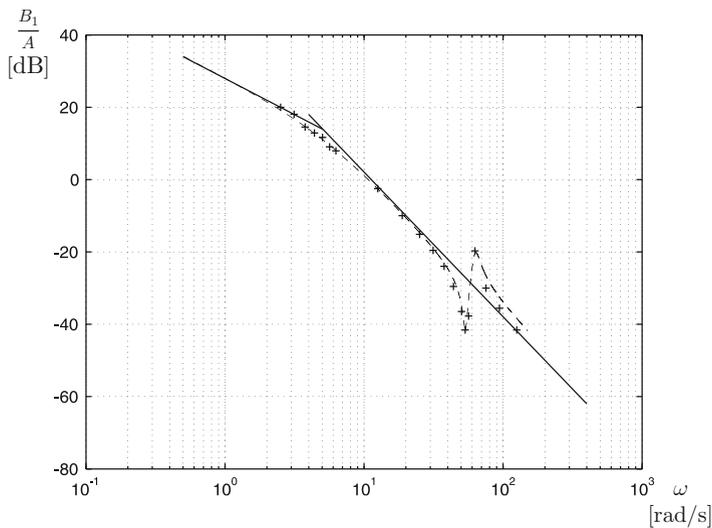
**Fig. 12.2** Experimental identification of  $G_{1u}(s) = \frac{\theta_1(s)}{U(s)}$ . Points marked with “+” represent the experimental data. The dashed line represents data obtained from the identified model. The straight lines represent the estimated asymptotes
