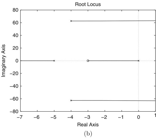
**Fig. 12.7** Root locus diagrams for the closed-loop system in Fig. 12.6
