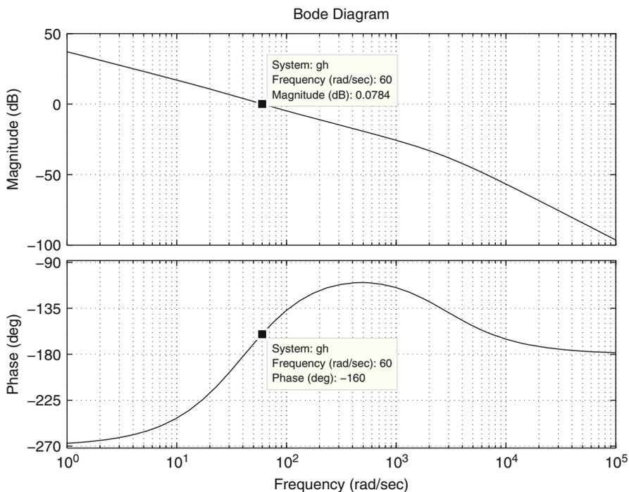
**Fig. 6.105** Bode diagrams of the transfer function in (6.62), i.e.,  $G(s)H(s) = \left(k_p + k_d s + \frac{k_i}{s}\right) \frac{k}{s^3 + 2739s^2 - 1250s - 3.536 \times 10^6}$  with  $k_d = 0.0131$ ,  $k_p = 1.0838$ ,  $k_i = 22.0341$
