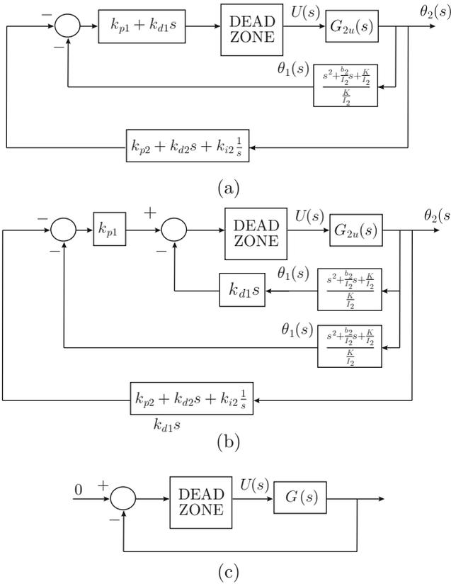
Fig. 12.27 Closed-loop diagrams for limit cycle analysis
