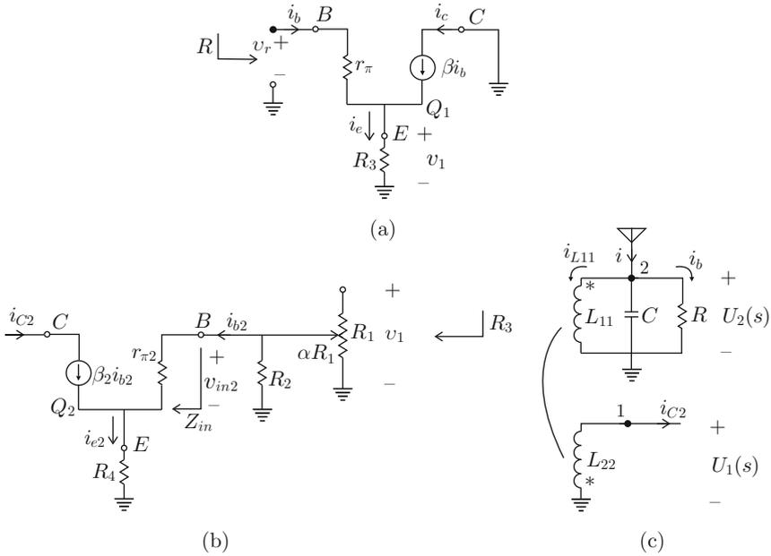
**Fig. 9.51** Different sections of the circuit in Fig. 9.50 . (a) Transistor  $Q_1$ . (b) Transistor  $Q_2$ . (c) Tuning and feedback circuit
