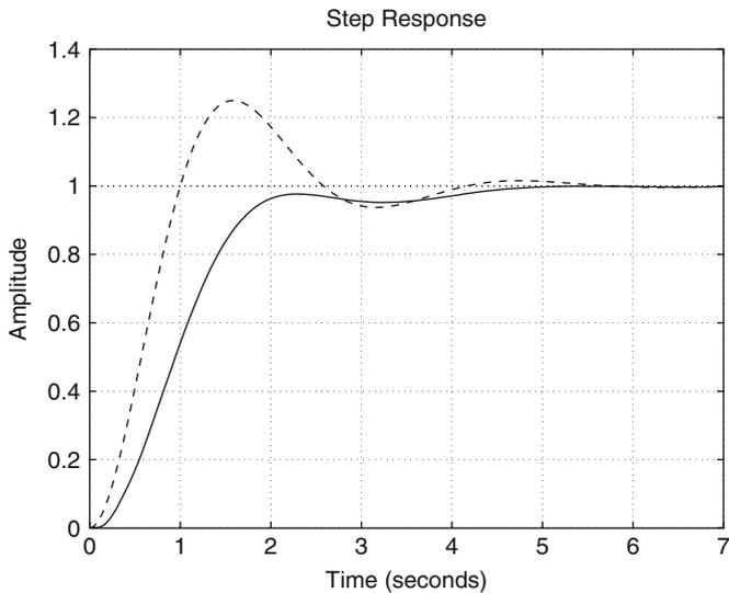
**Fig. 5.54** Closed-loop time response of the ball and beam system when using the block diagram in Fig. 5.53 and the controller gains  $b = 0.7$ ,  $c = 2.8658$ ,  $\gamma = 1.3531$  (continuous). Dashed: desired response
