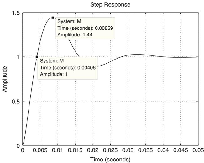
**Fig. 6.109** Time response when the reference is an unit step and a loop is closed around  $G(s)H(s) = \left(k_p + k_d s + \frac{k_i}{s}\right) \frac{k}{s^3 + 2739s^2 - 1250s - 3.536 \times 10^6}$ , with  $k_d = 0.0644$ ,  $k_p = 19.6089$ ,  $k_i = 621.0041$
