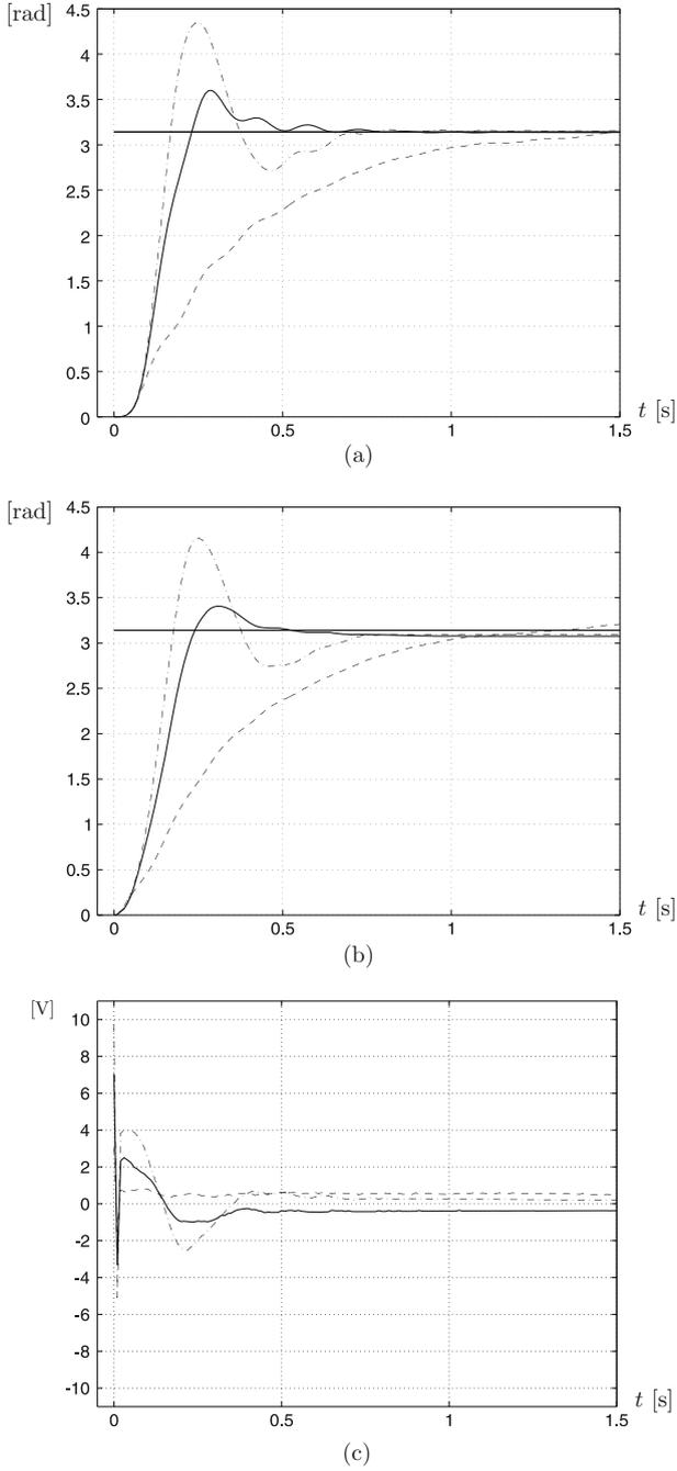
**Fig. 12.16** PID control of  $\theta_2$ . Experimental results. Continuous: PID gains in (12.21). Dashed: PID gains in (12.20). Dash-dot: PID gains in (12.22). Desired load position  $\theta_{2d} = \pi$ . (a)  $\theta_2$ . (b)  $\theta_1$ . (c) Applied voltage,  $u$
