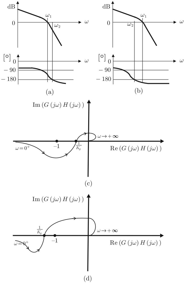
**Fig. 6.42** Frequency response of  $G(j\omega)H(j\omega)$ . The phase and gain margins are determined from the frequency response of the open-loop transfer function . (a) Closed-loop stability. (b) Closed-loop instability. (c) Closed-loop stability. (d) Closed-loop instability
