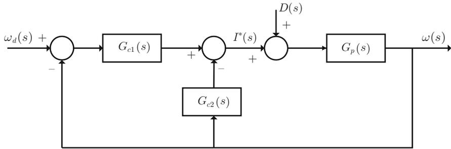
**Fig. 10.5** Closed-loop system with a two-degrees-of-freedom controller
