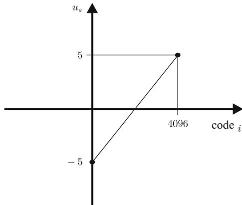
**Fig. 11.23** Conditioning of the signal  $-i^*$ , which is to be sent to the digital/analog converter
