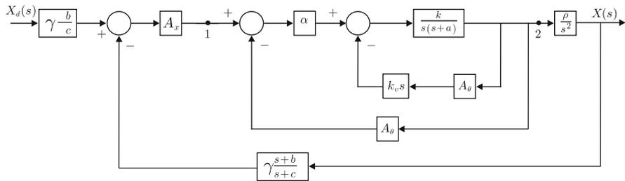
**Fig. 5.53** Use of the lead compensator in the feedback path. The factor  $\gamma \frac{b}{c}$  on the left is included to ensure that  $\lim_{t \rightarrow \infty} x(t) = x_d$
