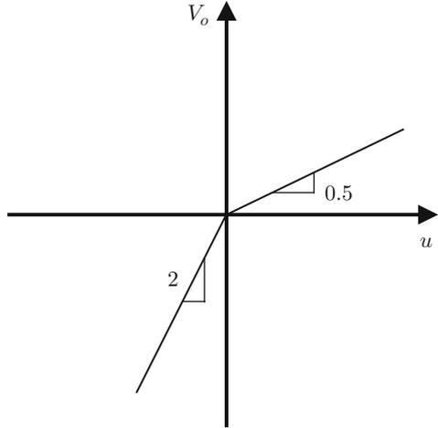
**Fig. 9.4** Voltages at the input  $u$  and the output  $V_o$  of the nonlinear amplifier in Fig. 9.3
