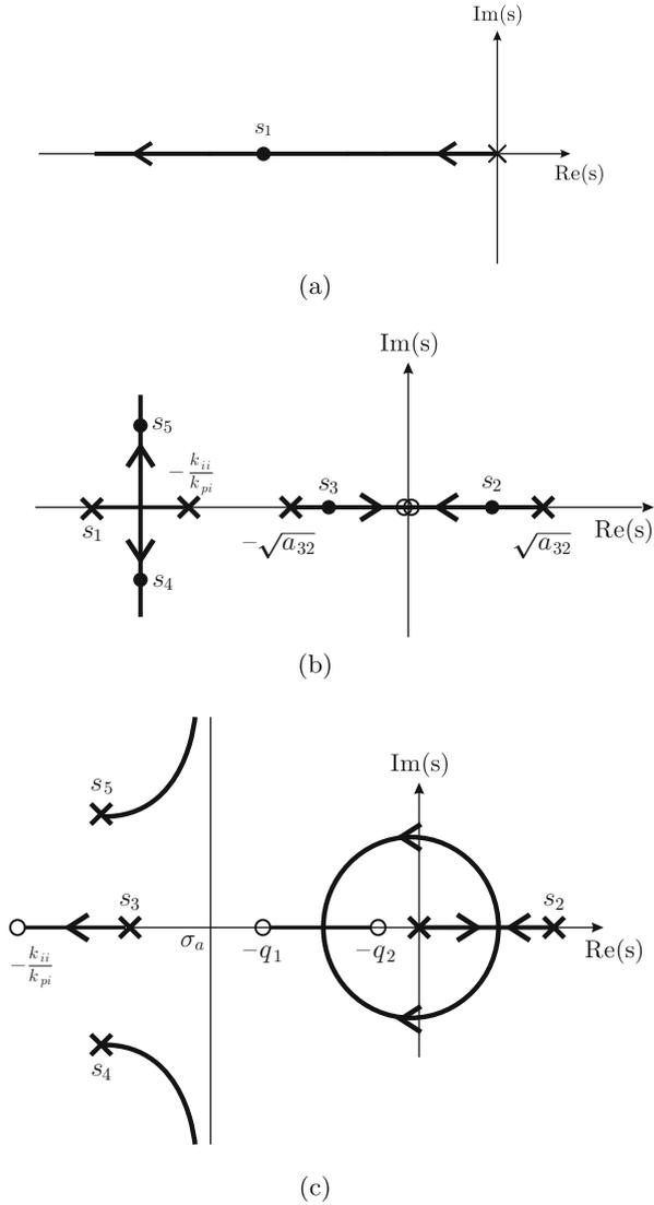
This yields  $k_{ii} = 340.89$  when using  $k_{pi} = 4.7$  as in (13.42). This value for  $k_{pi}$  is chosen to fairly compare with the results in Sects. 13.6.2 and 13.6.3. Hence,  $R = 4.7[\text{K}\Omega]$  and  $C = 3[\mu\text{F}]$  must be used in (13.39). Using the plant parameters corresponding to  $x_2^* = 0.01[\text{m}]$  and the controller gains in (13.45), in addition to  $k_{ii} = 340.89$ ,  $k_{pi} = 4.7$ , it is found that the closed-loop system has poles located at:
