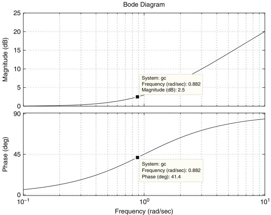
Fig. 6.59 Bode diagrams of the factor  $z + 1$ , where  $z = \frac{1}{b}s$ . The horizontal axis stands for  $\frac{1}{b}\omega$
