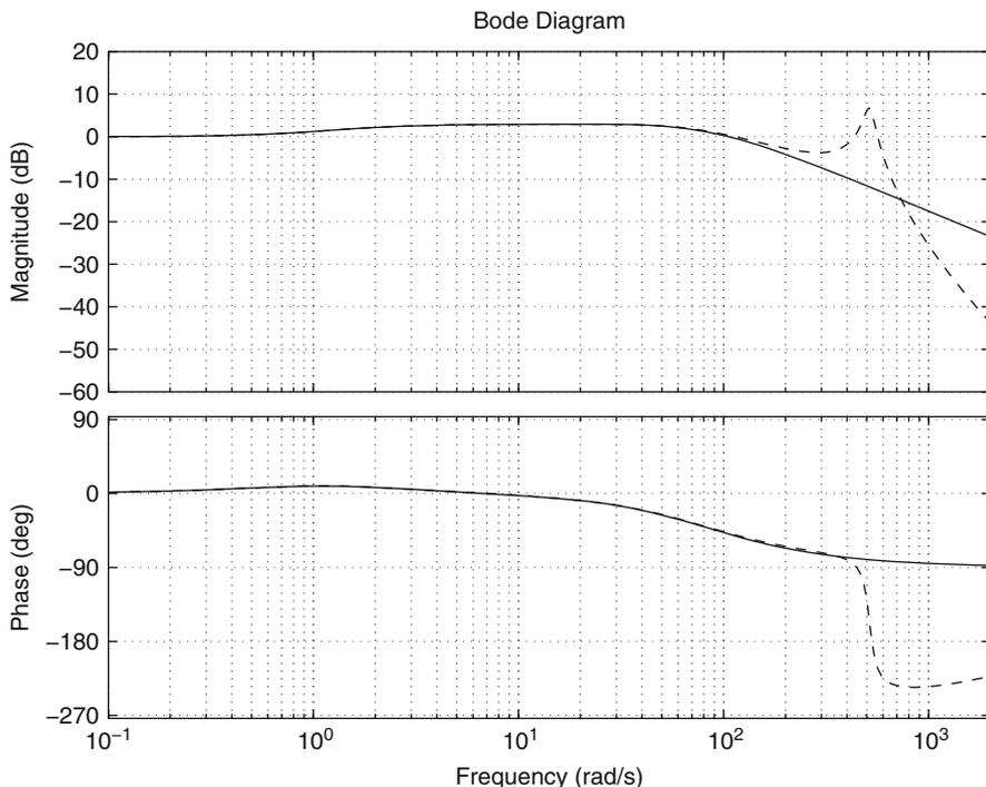
**Fig. 13.43** Closed-loop system Bode diagrams. Continuous: the electrical dynamics is not considered. Dashed: the electrical dynamics is taken into account. Controller gains in Table 13.4c) and  $k_{pi} = 4.7, k_{ii} = 10000$
