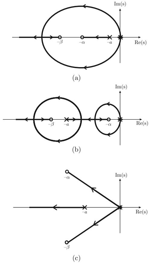
**Fig. 5.29** Proportional-derivative control of the position
