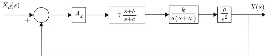
Fig. 6.81 Closed-loop system. Second proposal
