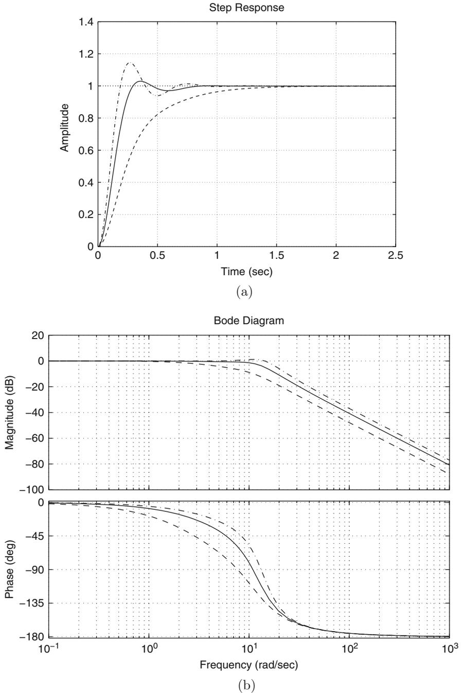
**Fig. 12.17** PID control of  $\theta_2$ . Simulation results. Continuous: PID gains in (12.21). Dashed: PID gains in (12.20). Dash-dot: PID gains in (12.22). (a) Time response of  $\theta_2$  when a unit step change is commanded. (b) Closed-loop Bode diagrams
