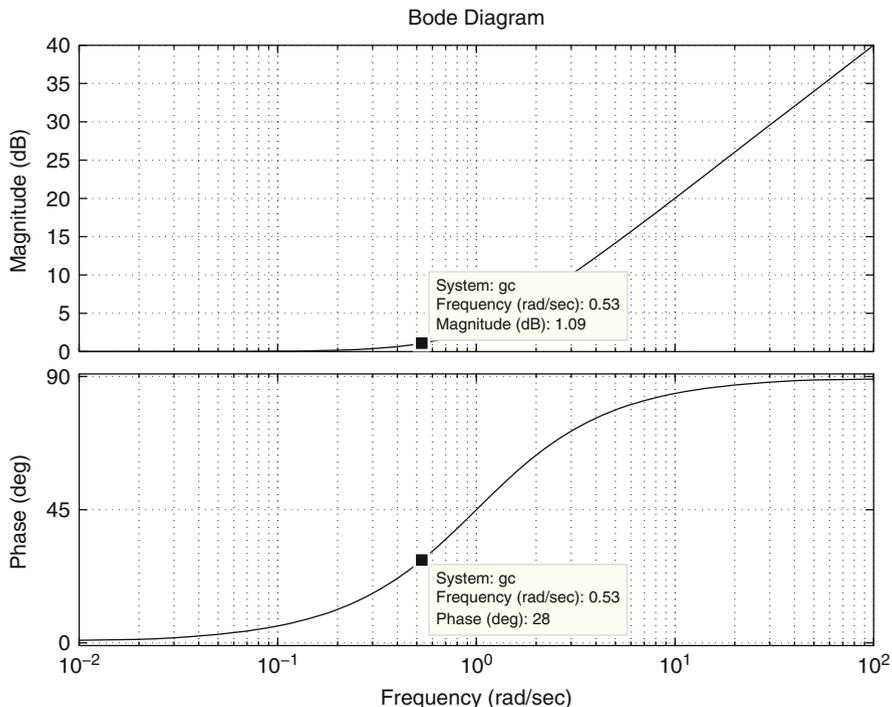
Fig. 10.19 Bode diagrams of the factor  $z + 1$ . The horizontal axis represents  $\frac{\omega}{b}$
