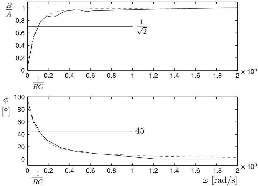
**Fig. 6.4** Experimental (continuous) and theoretical (dashed) data for the circuit in Fig. 6.2b (see Table 6.2)
