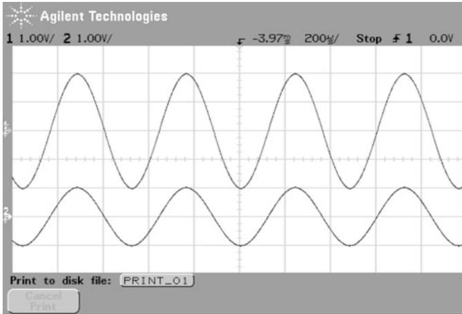
**Fig. 9.12** Experimental results. Voltages at the input and the output of the circuit in Fig. 9.9. Upper line:  $V_o$ , bottom line:  $V_i$
