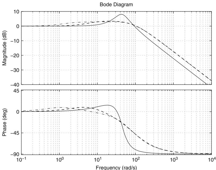
**Fig. 13.30** Bode diagrams of the closed-loop system in Fig. 13.9. Continuous line:  $k_d = 0.01309$ ,  $k_p = 0.8873$ ,  $k_i = 14.2$ . Dashed:  $k_d = 0.02293$ ,  $k_p = 1.063$ ,  $k_i = 4.303$ . Line-dot:  $k_d = 0.02259$ ,  $k_p = 1.09$ ,  $k_i = 1.068$
