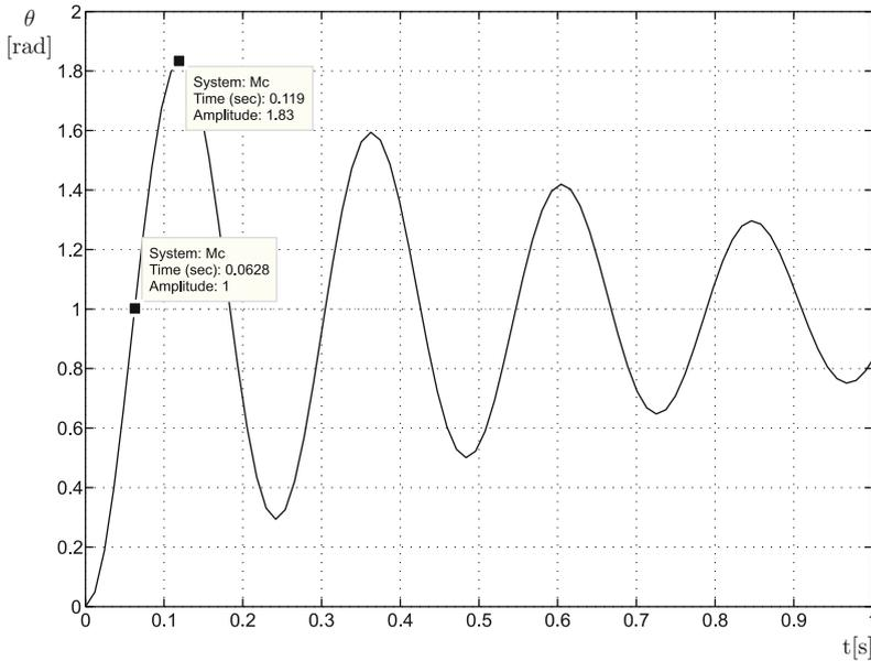
**Fig. 6.61** Time response of the closed-loop system shown in Fig. 6.58, when  $k_p = 1$ ,  $k_d = 0$ ,  $k = 675.4471$  and  $a = 2.8681$
