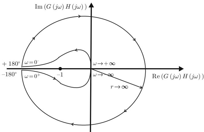
**Fig. 6.71** Polar plot of (6.34) when mapping the modified Nyquist path shown in Fig. 6.57
