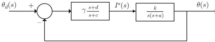
Fig. 11.6 Position control with a lead compensator
