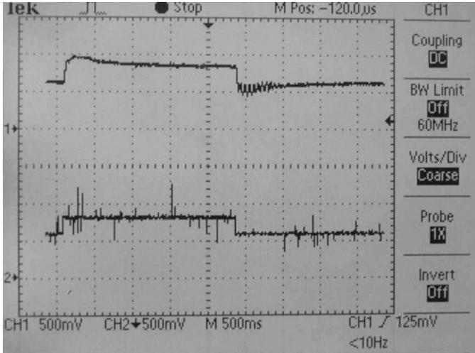
**Fig. 13.14** Experimental results when step changes are applied from  $y_d = z_2^* = 0.006[m]$  to  $y_d = z_2^* = 0.008[m]$  and vice versa. Top line  $x_{2v} = y_v$ , bottom line  $x_{2v}^* = y_v^*$
