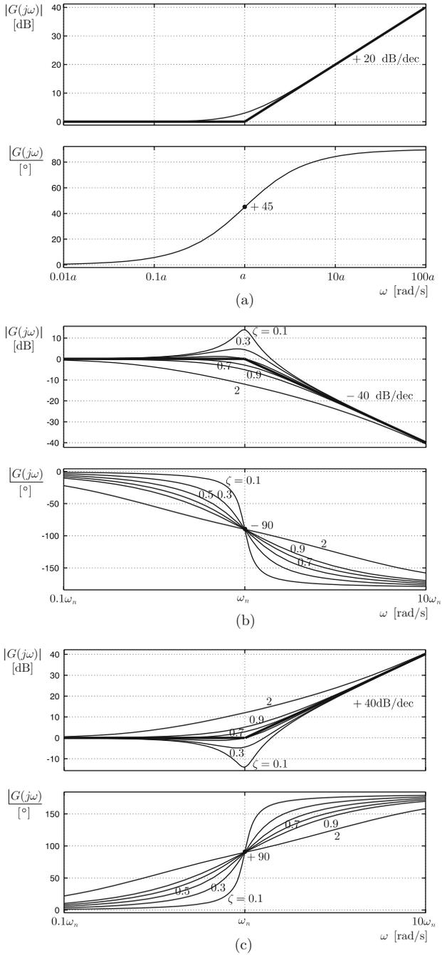
**Fig. 6.17** Bode diagrams of first- and second-order factors in (6.12) (continued). (a)  $G(s) = \frac{s+a}{s}$ . (b)  $G(s) = \frac{\omega_n^2}{s^2 + 2\zeta\omega_n s + \omega_n^2}$ . (c)  $G(s) = \frac{\omega_n^2}{s^2 + 2\zeta\omega_n s + \omega_n^2}$
