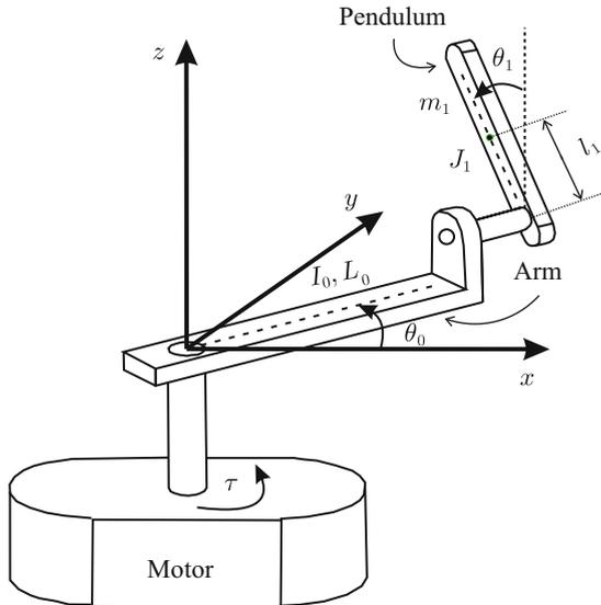
around its center of mass. Note that the pendulum consists of a beam whose mass is not negligible.
