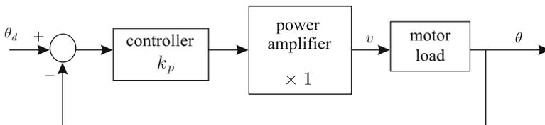
Fig. 1.9 Block diagram of a position control system
