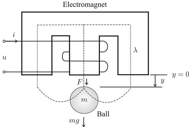
Fig. 13.1 Magnetic levitation system
