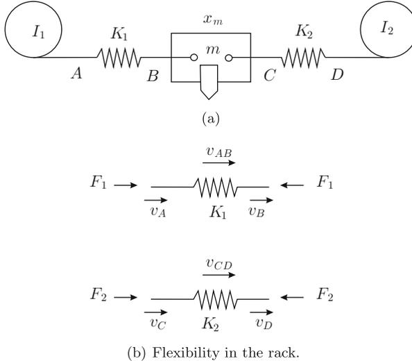
**Fig. 2.30** A transmission system with a flexible rack
