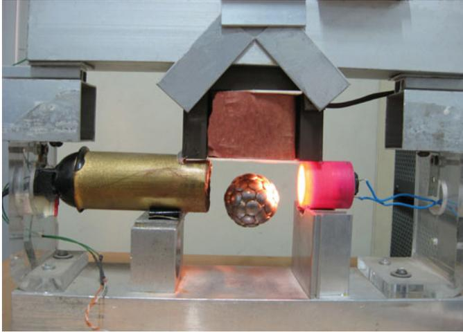
**Fig. 13.18** The magnetic levitation system that has been built
