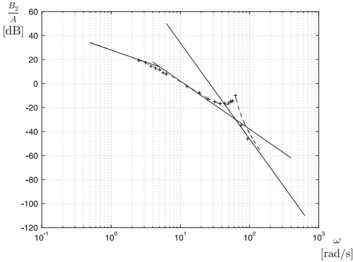
**Fig. 12.3** Experimental identification of  $G_{2u}(s) = \frac{\theta_2(s)}{U(s)}$ . Points marked with “+” represent the experimental data. The dashed line represents data obtained from the identified model. The straight lines represent the estimated asymptotes
