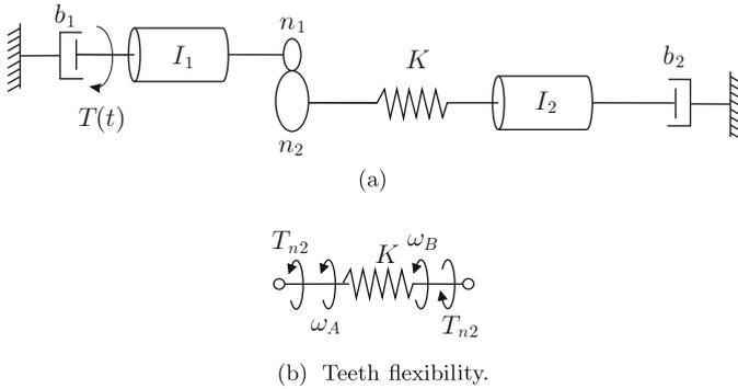
**Fig. 2.31** Transmission system with a flexible gear reducer
