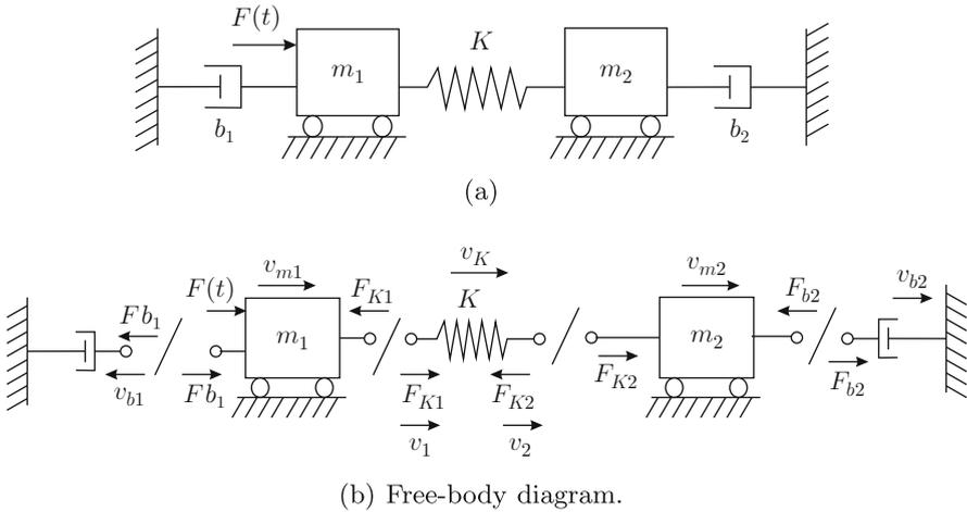
**Fig. 2.7** Two bodies connected by a spring
