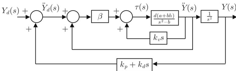
Fig. 15.4 Block diagram of the closed-loop control system
