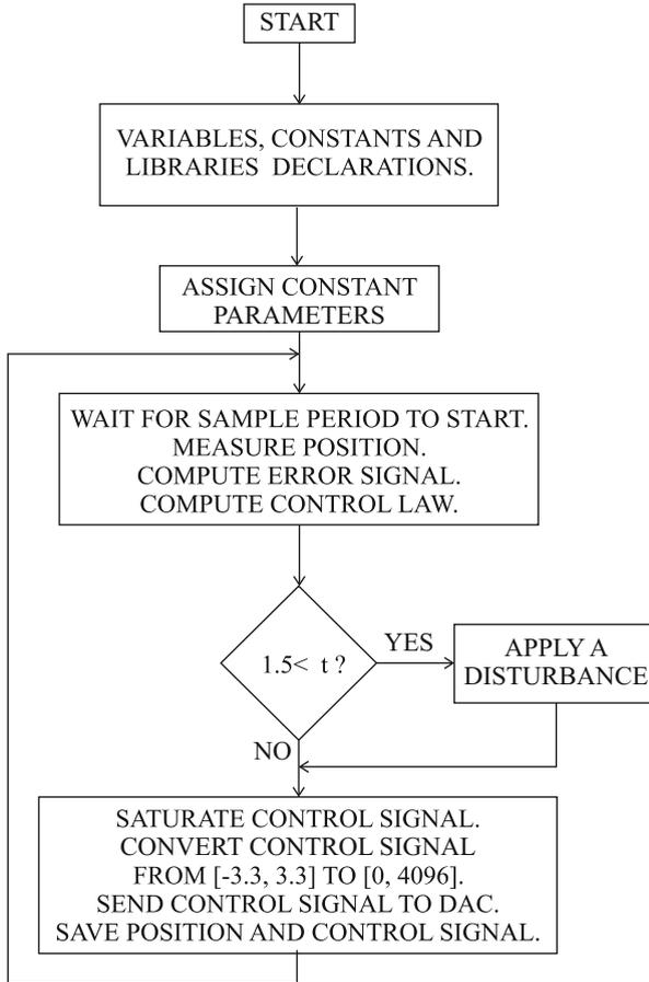
**Fig. 11.25** Flow diagram for the PC programming when controlling the position in a PM brushed DC motor
