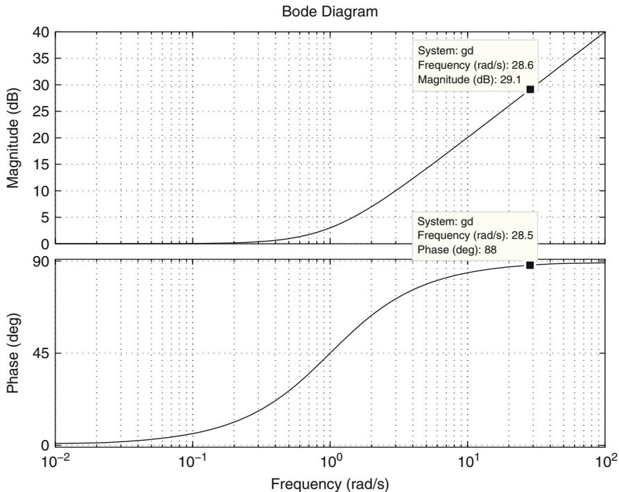
Fig. 13.32 Bode diagrams for  $z + 1$ . The horizontal axis represents  $\frac{\omega}{q_2}$
