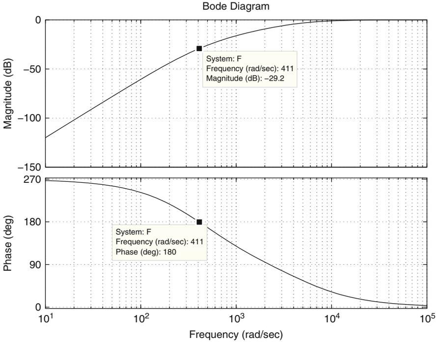
**Fig. 9.31** Bode diagrams of  $F(s)$  in (9.8), when  $RC = 0.001$
