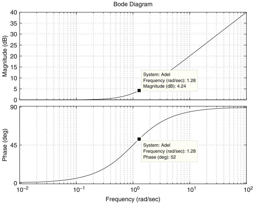
**Fig. 6.104** Bode diagrams of the factor  $z + 1$ . The horizontal axis represents  $\frac{1}{z_2}\omega$
