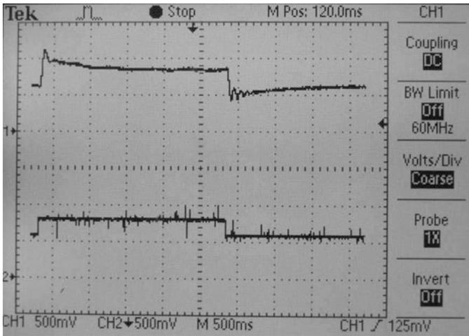
**Fig. 13.41** Experimental results when step changes are applied from  $y_d = z_2^* = 0.006[m]$  to  $y_d = z_2^* = 0.008[m]$  and vice versa. Top line  $x_{2v} = y_v$ , bottom line  $x_{2v}^* = y_v^*$ . Controller gains in Table 13.4c)
