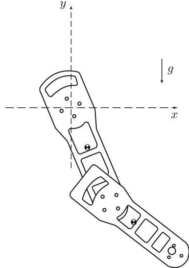
To be capable of efficiently accomplishing these tasks in three-dimensional space, a robotic arm has to be composed of at least seven bodies joined by at least six joints, three for position and three for orientation. Then, it is said that the robotic arm has at least six degrees of freedom. However, to simplify the exposition of ideas, the two-degrees-of-freedom robotic arm depicted in Fig. 1.13 is considered in the following.
