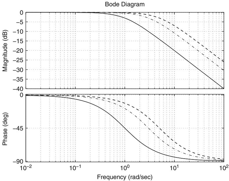
**Fig. 6.46** Bode diagrams of the transfer function  $M(s) = \frac{a}{s+a}$ . Continuous:  $a = 1$ . Dash-dot:  $a = 3$ . Dashed:  $a = 5$
