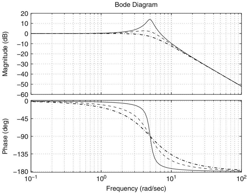
**Fig. 6.48** Bode diagrams of the transfer function  $M(s) = \frac{\omega_n^2}{s^2 + 2\zeta\omega_n s + \omega_n^2}$  when  $\omega_n = 5$ . Continuous:  $\zeta = 0.1$ . Dashed:  $\zeta = 0.4$ . Dash-dot:  $\zeta = 0.7$
