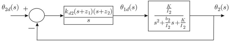
Fig. 12.11 Proportional–integral–derivative (PID) control of the load position (12.11)
