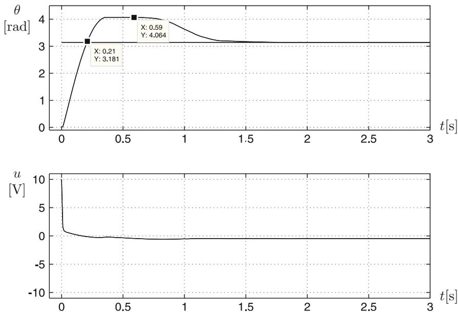
Fig. 11.32 Experimental results for the control scheme in Fig. 11.27.  $k_d = 0.0935$ ,  $k_p = 1.0177$ ,  $k_i = 2.4697$
