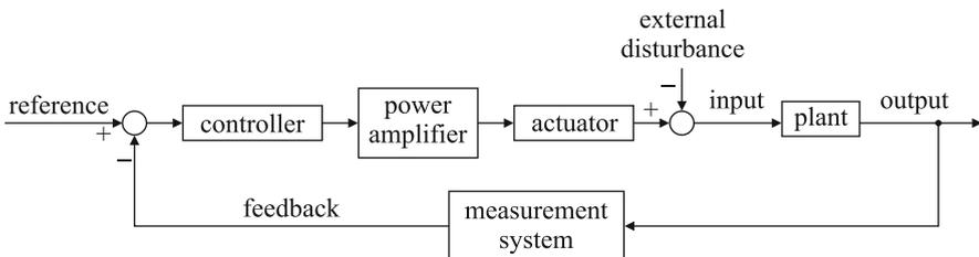
**Fig. 1.17** Nomenclature employed in a closed-loop control system
