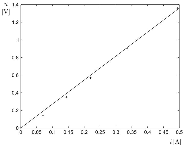
**Fig. 13.4** Experimental measurement of  $R$
