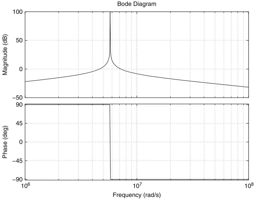
**Fig. 9.55** Bode diagrams of  $G(s)$  in (9.60) for  $\alpha = 0.2619$
