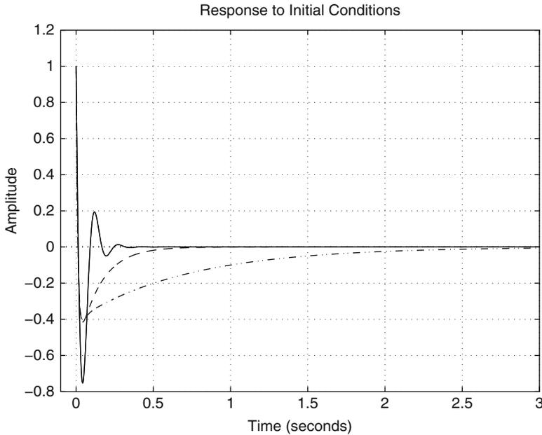
**Fig. 13.29** Closed-loop time response of system in Fig. 13.9 (simulation). Continuous line:  $k_d = 0.01309$ ,  $k_p = 0.8873$ ,  $k_i = 14.2$ . Dashed:  $k_d = 0.02293$ ,  $k_p = 1.063$ ,  $k_i = 4.303$ . Line-dot:  $k_d = 0.02259$ ,  $k_p = 1.09$ ,  $k_i = 1.068$
