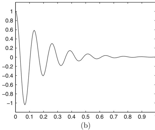
**Fig. 8.21** Simulation response of signal at the input of the saturation nonlinearity in Fig. 8.15. The horizontal axis shows time in seconds. (a)  $k_{pi} = 0.03$ . (b)  $k_{pi} = 0.8$
