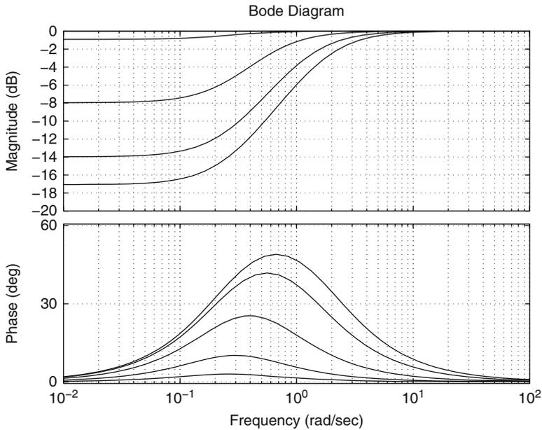
**Fig. 6.24** Bode diagrams for  $G_d(s)$  in (6.14), when  $T = 4$  and  $\xi$  takes the values 0.14, 0.2, 0.4, 0.7, and 0.9. In the magnitude plot,  $\xi$  increases from bottom to top. In the phase plot,  $\xi$  increases from top to bottom
