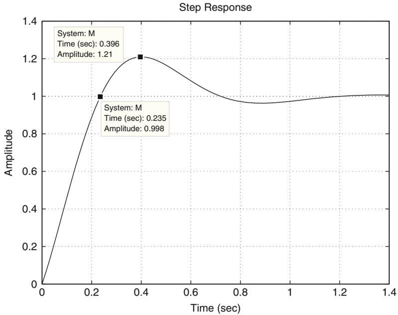
**Fig. 10.21** Simulation response of the control system in Fig. 10.15 when a unit step in the desired velocity is applied.  $k_p = 0.0619$ ,  $k_i = 0.8821$ , (10.46), and (10.47) are used
