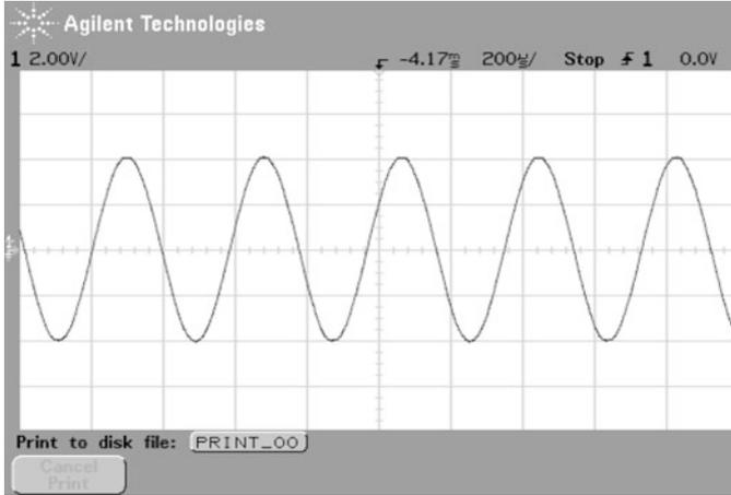
Fig. 9.33 Waveform of the voltage at the output of the operational amplifier in Fig. 9.32
