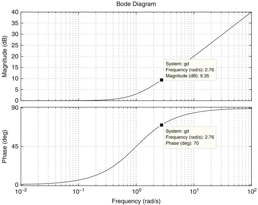
Fig. 13.27 Bode diagrams for  $z + 1$ . The horizontal axis represents  $\frac{\omega}{q_2}$
