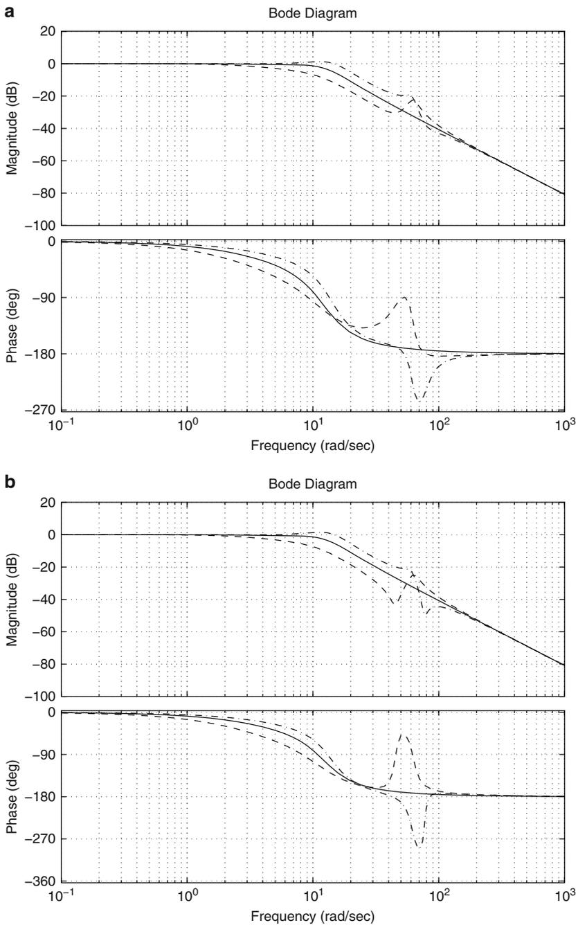
**Fig. 12.23** Closed-loop Bode diagrams when the PID zeros do not cancel out badly damped open-loop poles at  $-6.304 \pm 61.7989j$  exactly. Continuous: PID zeros at  $-6.304 \pm 61.7989j$ . **(a)** Dashed: PID zeros at  $-14 \pm 45j$ , dash-dot: PID zeros at  $-14 \pm 77j$ . **(b)** Dashed: PID zeros at  $-3.2 \pm 45j$ , dash-dot: PID zeros at  $-3.2 \pm 77j$ . In all cases  $k_{d2} = 0.0018$
