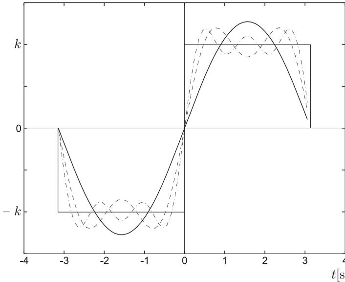
**Fig. 6.9** Different approximations of  $f(t)$  shown in Fig. 6.7. Continuous  $f_1(t) = \frac{4k}{\pi} \sin(t)$ . Dashed  $f_2(t) = \frac{4k}{\pi} \left( \sin(t) + \frac{1}{3} \sin(3t) \right)$ . Dash-dot  $f_3(t) = \frac{4k}{\pi} \left( \sin(t) + \frac{1}{3} \sin(3t) + \frac{1}{5} \sin(5t) \right)$
