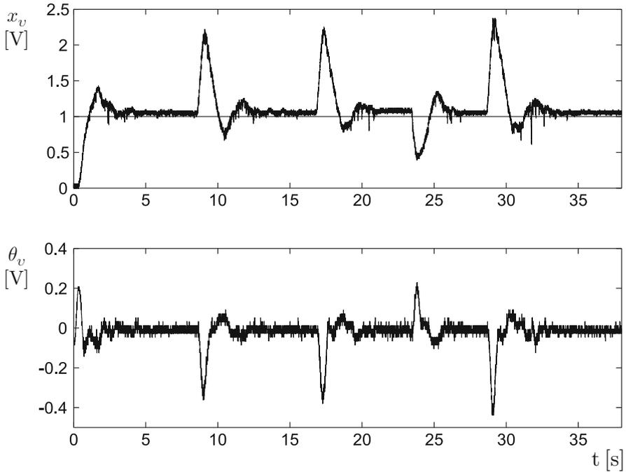
**Fig. 14.27** Experimental results using the microcontroller PIC16F877A. Some ball position deviations are introduced by an external agent
