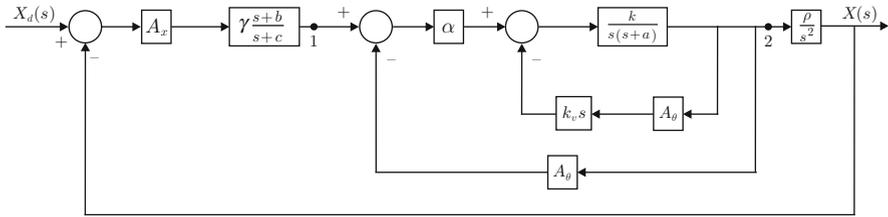
Fig. 4.25 Control of a ball and beam system
