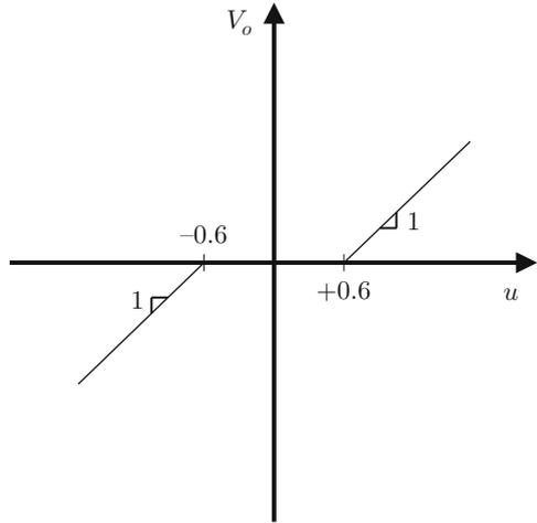
**Fig. 9.8** Voltages at the input  $u$  and the output  $V_o$  of the amplifier in Fig. 9.6
