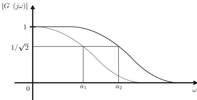
**Fig. 6.15** A larger value of  $a$  in  $\frac{a}{s+a}$  allows a greater effect of the intermediate frequencies and, hence, a faster time response is accomplished
