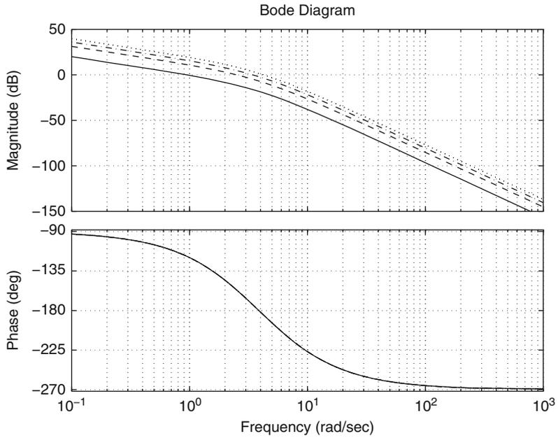
**Fig. 6.53** Bode diagrams of the open-loop transfer function  $G(s)H(s) = \frac{k}{s(s+3)(s+5)}$  in the closed-loop system shown in Fig. 6.52. Continuous:  $k = 15$ . Dashed:  $k = 55$ . Dash-dot:  $k = 95$ . Dotted:  $k = 145$
