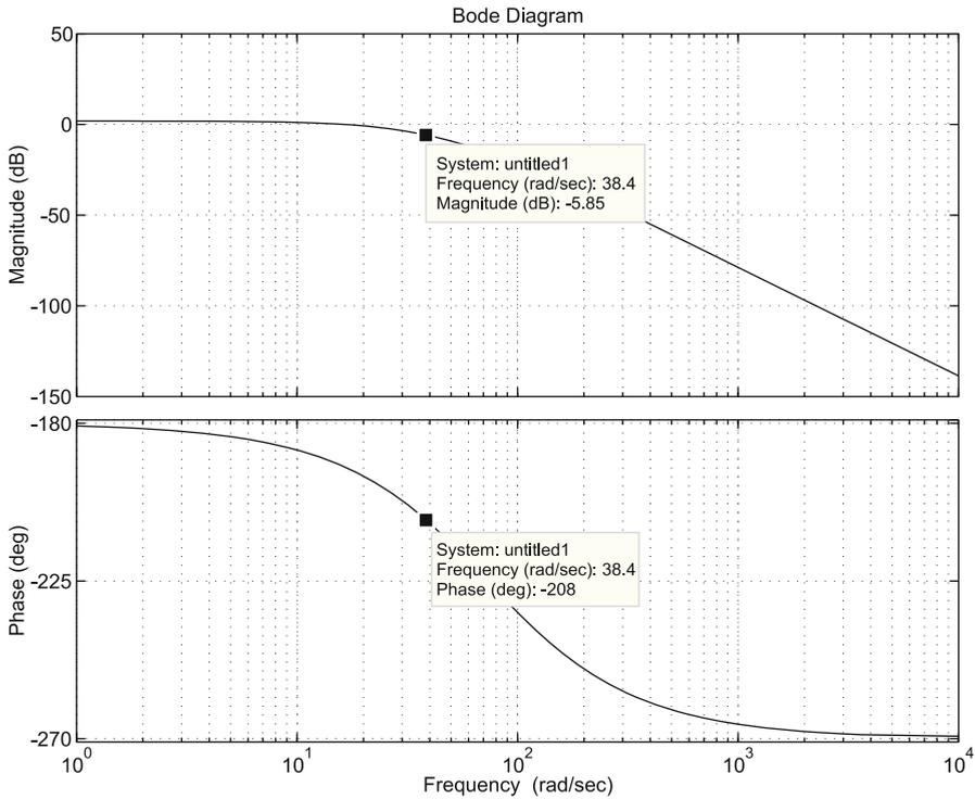
**Fig. 6.91** Bode diagrams of  $\frac{116137}{s^3 + 72.54s^2 - 1250s - 9.363 \times 10^4}$
