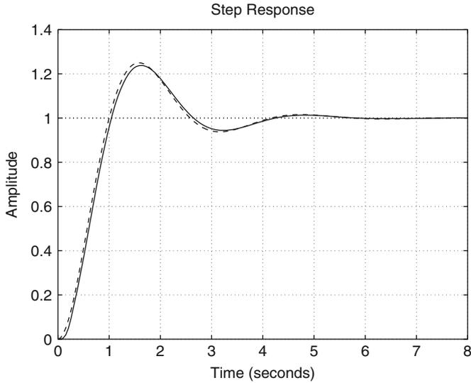
**Fig. 5.58** Closed-loop time response of the ball and beam system when using the block diagram in Fig. 5.53 and the controller gains  $b = 2$ ,  $c = 11.7121$  and  $\gamma = 4.6336$  (continuous). Dashed: desired response
