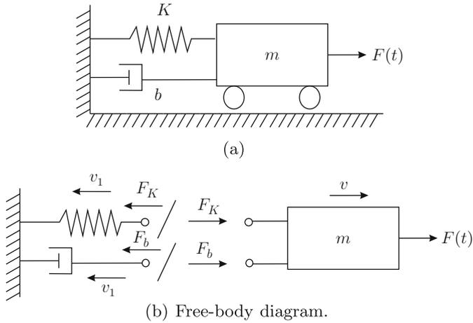
**Fig. 2.6** A mass-spring-damper system
