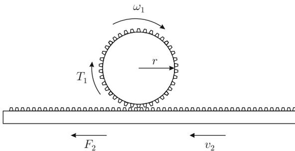
**Fig. 2.25** A rack and pinion system
