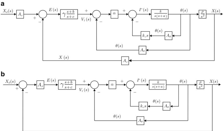
Fig. 14.8 Equivalent block diagrams of the control systems to be designed
