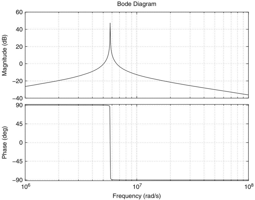
Fig. 9.54 Bode diagrams of  $G(s)$  in (9.60) for  $\alpha = 0.1546$
