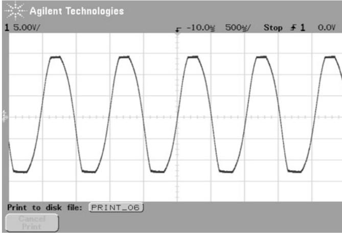
**Fig. 9.23** Waveform of the voltage at the output of the operational amplifier in Fig. 9.21. The potentiometer is at 25.6[KOhm]
