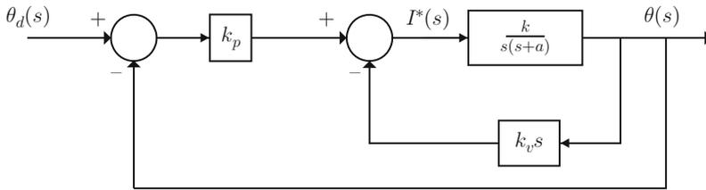
Fig. 11.3 Proportional position control with velocity feedback
