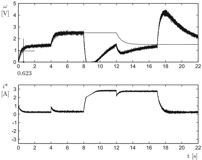
**Fig. 10.11** Classical proportional–integral (PI) velocity control using the tuning rule in (10.43)
