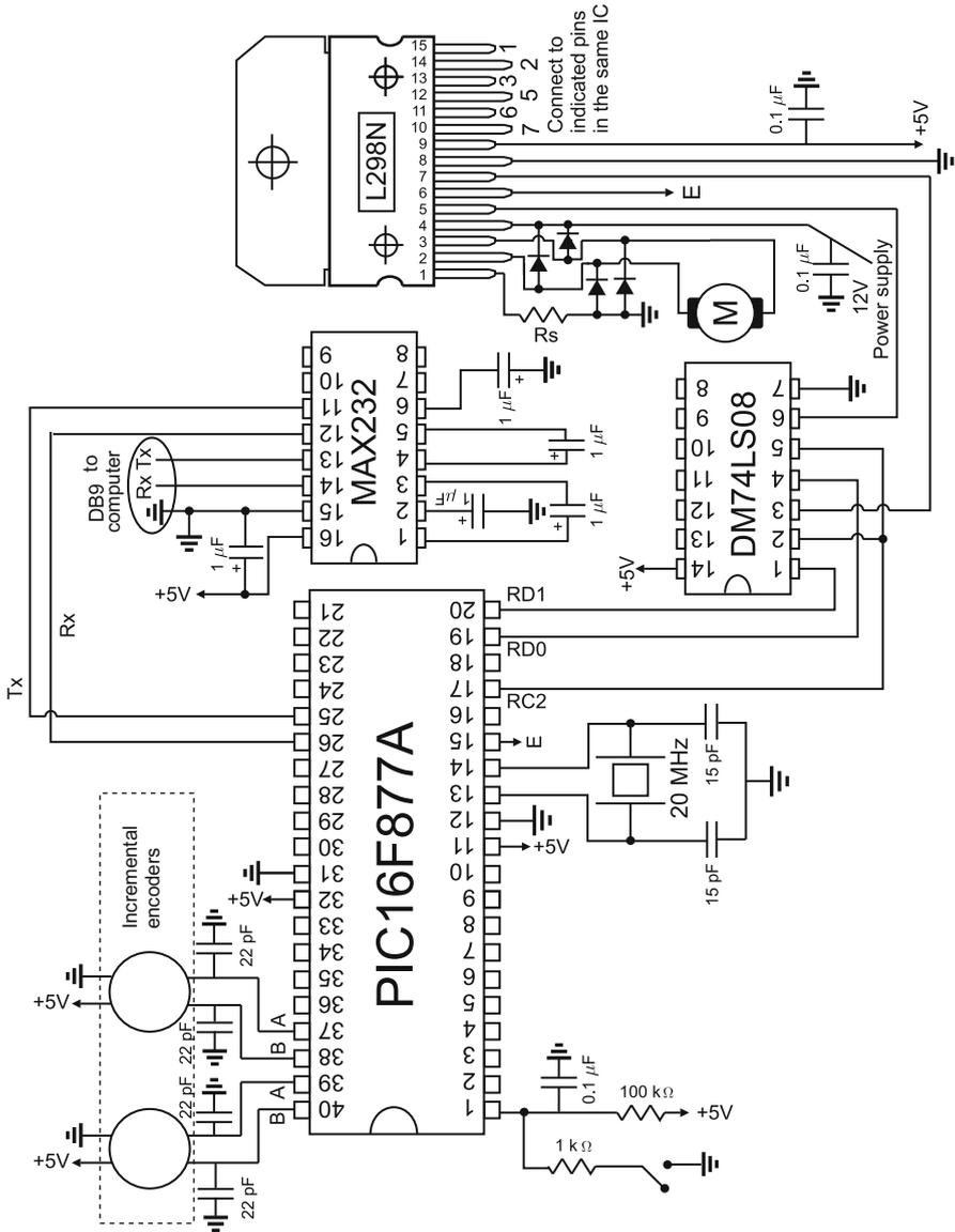
Fig. 12.44 Electric diagram of the complete control system
