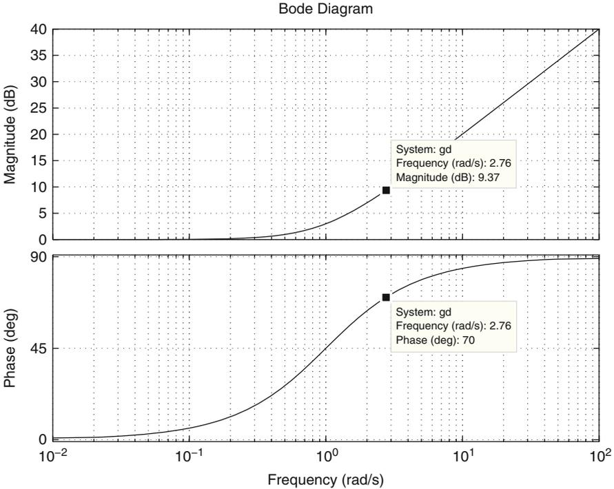
Fig. 13.35 Bode diagrams for  $z + 1$ . The horizontal axis represents  $\frac{\omega}{q_2}$
