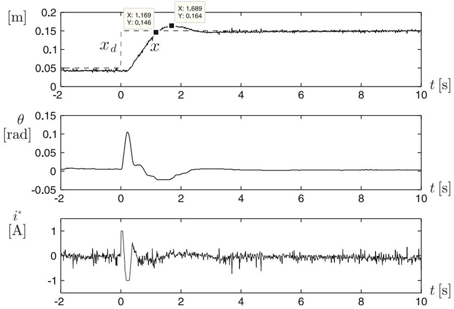
**Fig. 14.17** Experimental response when the control scheme in Fig. 5.53 is used with  $k_v = 0.35$ ,  $\alpha = 30$ ,  $b = 1.4$ ,  $c = 5.1138$ ,  $\gamma = 2.1868$
