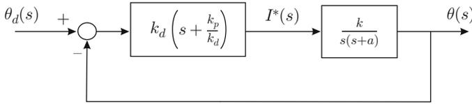
**Fig. 5.15** Proportional–derivative (PD) control of position
