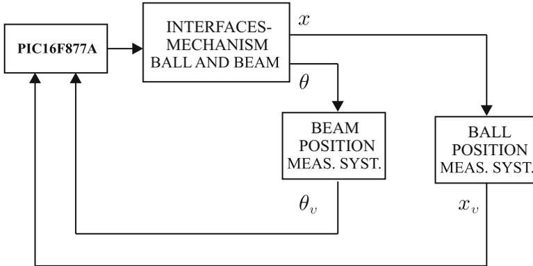
**Fig. 14.22** Block interfaces and ball and beam mechanism are shown in Fig. 14.24. The beam position measurement system is composed of a potentiometer fixed to the beam shaft. The ball position measurement system is shown in Fig. 14.23
