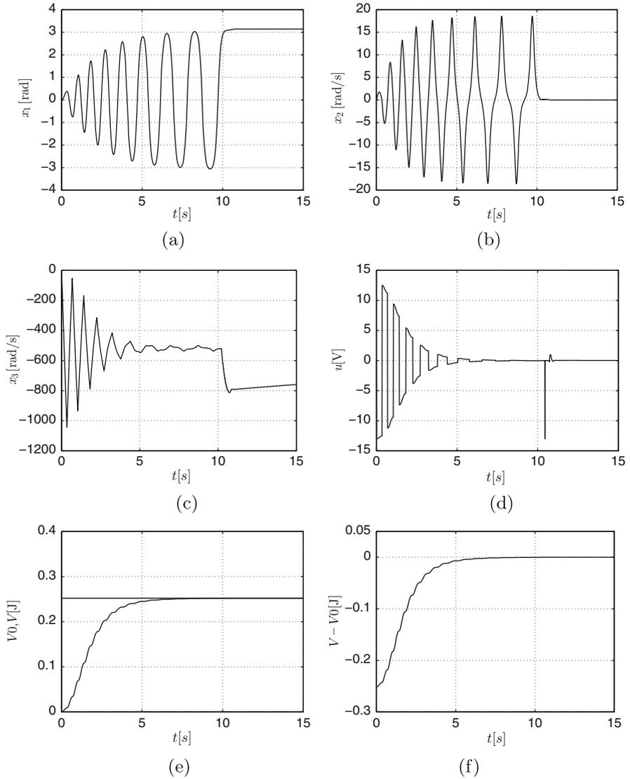
**Fig. 16.7** Simulation results when swinging up and stabilizing the IWP with controllers in (16.10) and (16.30) . (a) Pendulum position. (b) Pendulum velocity. (c) Wheel velocity. (d) Applied voltage. (e) Pendulum energy. (f) Pendulum energy error
