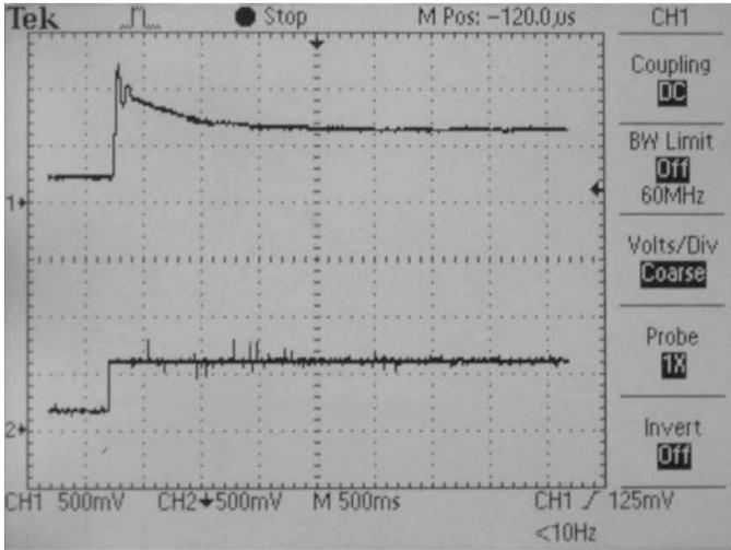
**Fig. 13.16** A step change in the desired position is commanded from  $y_d = x_2^* = 0.002[m]$  ( $y_v^* = 0.2[V]$ ) to  $y_d = x_2^* = 0.006[m]$  ( $y_v^* = 0.6[V]$ ). Top line  $x_{2v} = y_v$ , bottom line  $x_{2v}^* = y_v^*$
