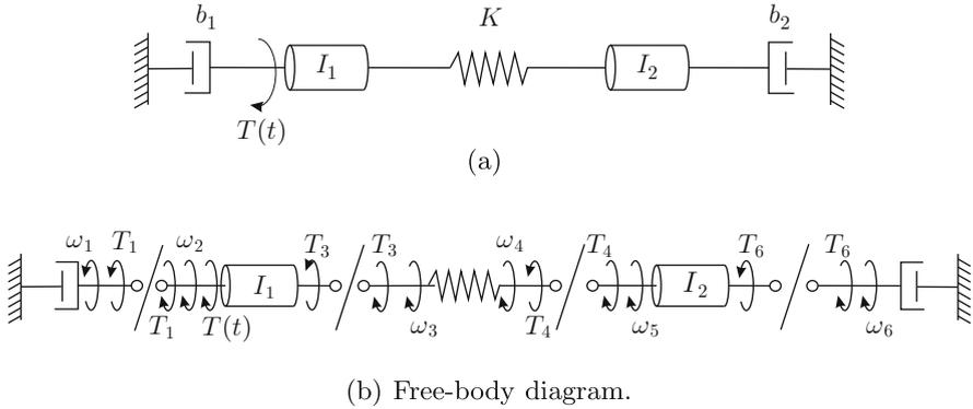
**Fig. 2.14** Two rotative bodies connected by a spring
