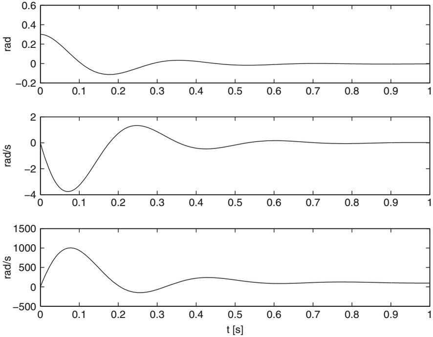
**Fig. 7.11** Simulation results when using the gain vector  $K = [-345.5910 \quad -11.2594 \quad -0.0086]$  to control the inertia wheel pendulum. Top:  $z_1$ . Middle:  $z_2$ . Bottom:  $z_3$
