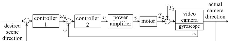
**Fig. 1.15** A gyro-stabilized video camera control system
