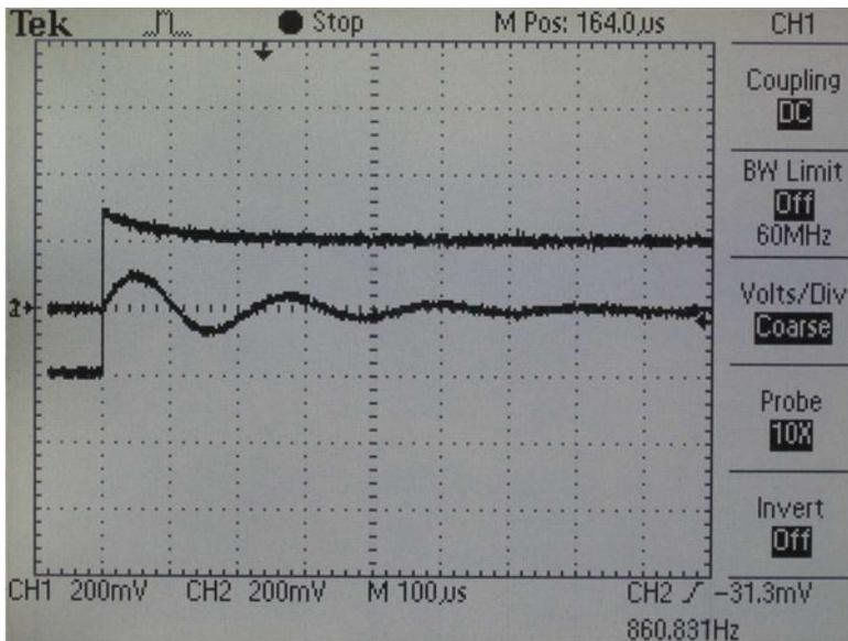
Fig. 6.14 Time response of the circuit in Fig. 6.2d when  $v_i(t)$  is a step signal
