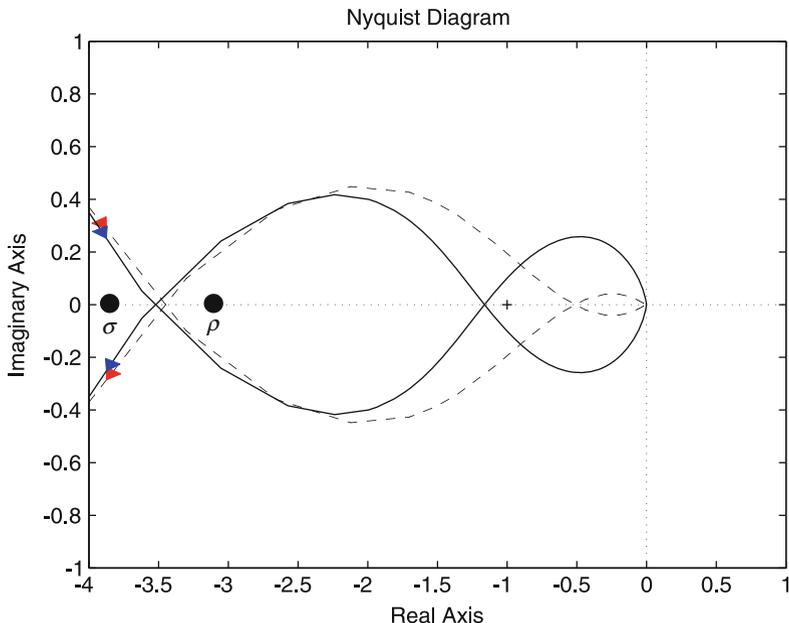
**Fig. 8.18** Polar plot of  $G_C(s)$  in (8.24). Continuous  $k_{pi} = 0.03$ . Dashed  $k_{pi} = 0.8$
