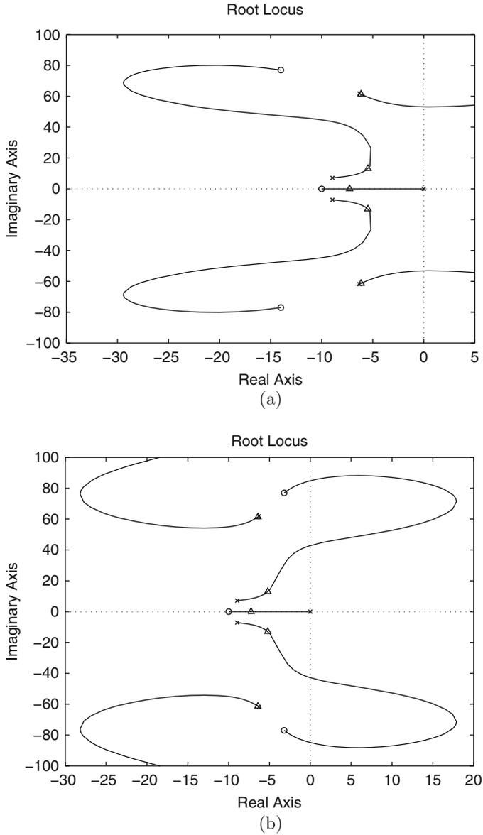
**Fig. 12.21** Root locus diagrams when the PID zeros do not cancel out the undesired open-loop poles at  $-6.304 \pm 61.7989j$  exactly. Triangles represent closed-loop poles in each case. In all cases  $k_{d2} = 0.0018$ . **(a)** PID zeros at  $-14 \pm 77j$ . **(b)** PID zeros at  $-3.2 \pm 77j$
