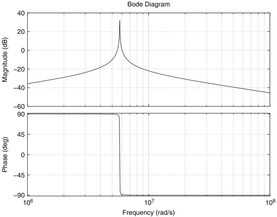
**Fig. 9.53** Bode diagrams of  $G(s)$  in (9.60) for  $\alpha = 0.0515$
