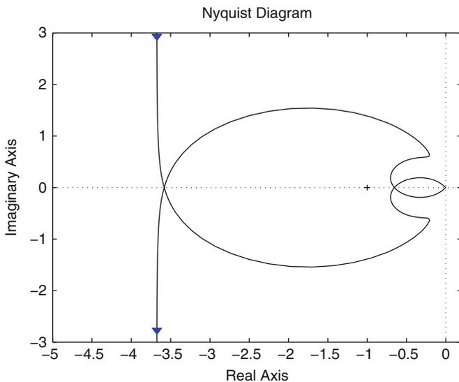
**Fig. 13.44** Open-loop polar diagram taking into account electrical dynamics. Controller gains in Table 13.4c) and  $k_{pi} = 4.7$ ,  $k_{ii} = 10000$
