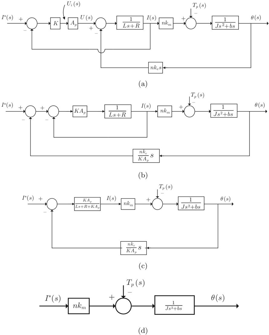
**Fig. 10.2** Equivalent block diagrams for a PM brushed DC motor provided with a proportional current loop and a power amplifier
