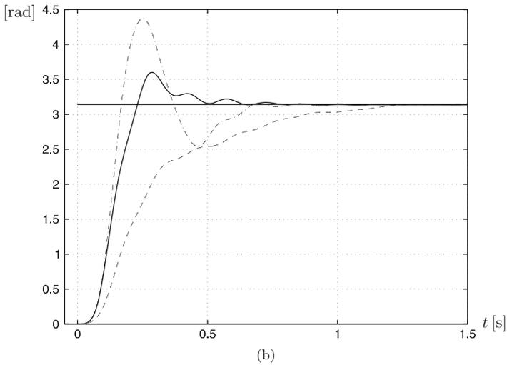
**Fig. 12.18** PID control of  $\theta_2$  when the zeros of the PID controller do not cancel out the open-loop poles of the plant located at  $-6.304 \pm 61.7989j$  exactly. Experimental results. Continuous: PID controller gains in (12.21). **(a)** Dashed: PID zeros at  $-14 \pm 45j$ . Dash-dot: PID zeros at  $-14 \pm 77j$ . **(b)** Dashed: PID zeros at  $-3.2 \pm 45j$ . Dash-dot: PID zeros at  $-3.2 \pm 77j$ . In all cases  $k_{d2} = 0.0018$ . **(a)**  $\theta_2$ . **(b)**  $\theta_2$
