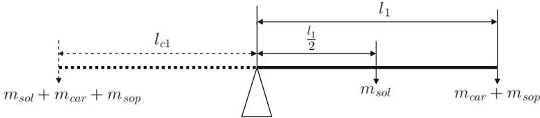
**Fig. 16.5** The balance principle to compute  $l_{c1}$
