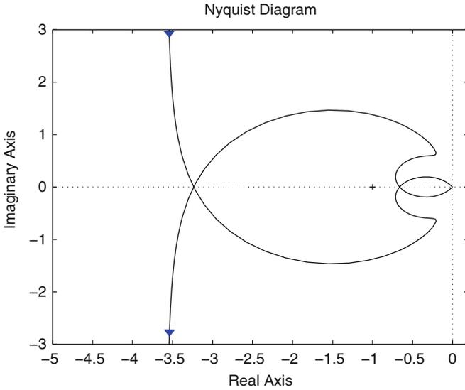
**Fig. 13.40** Open-loop polar plot taking into account electrical dynamics. Controller gains in Table 13.4b) and  $k_{pi} = 4.7, k_{ii} = 10000$
