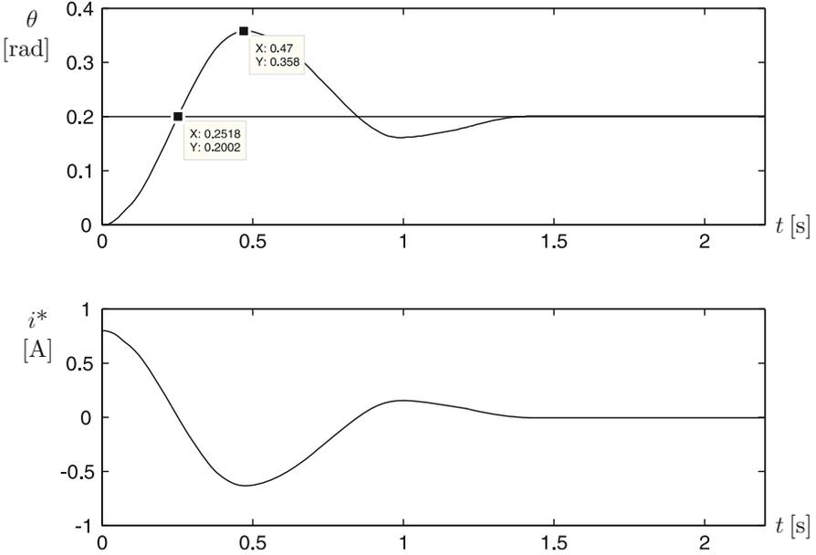
**Fig. 14.6** Experimental results using  $k_p = 4$  and the block diagram in Fig. 14.5
