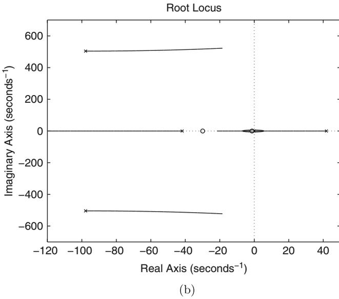
**Fig. 13.13** Root locus diagram corresponding to the block diagram in Fig. 13.8e . (a) Zoom-in. (b) Zoom-out
