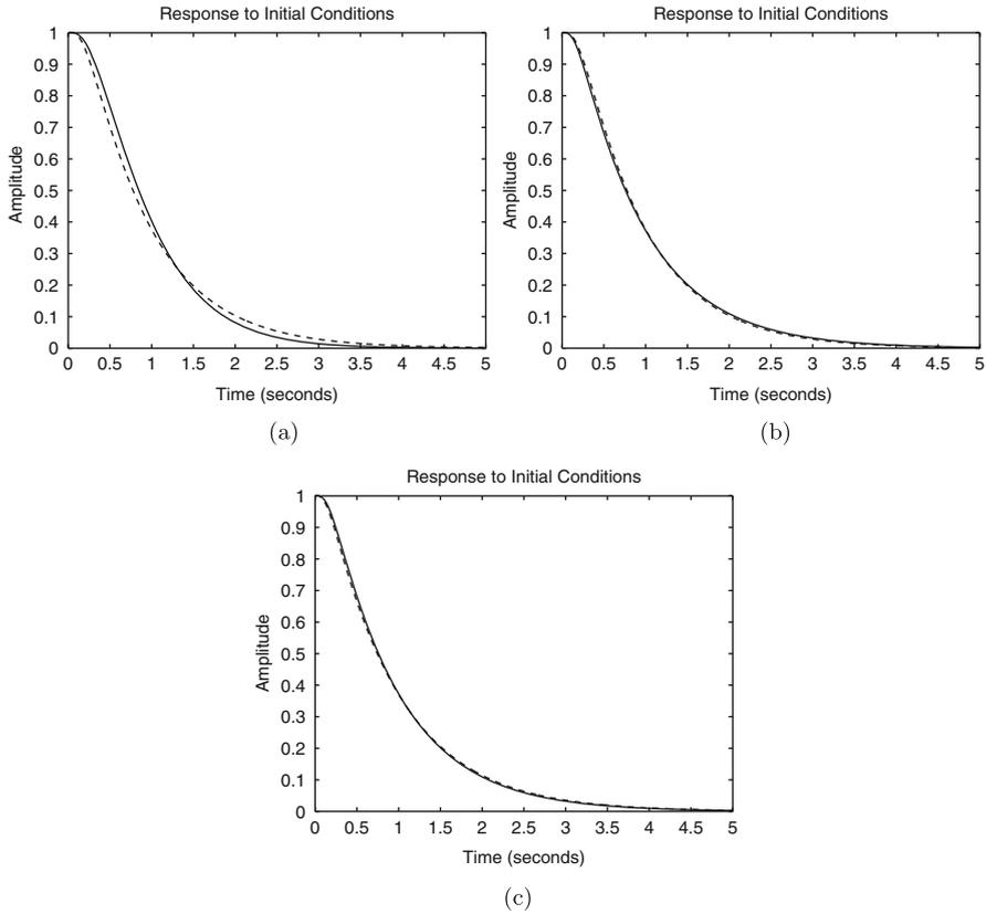
**Fig. 15.7** Flat output  $y$  response obtained in simulation when using the controller (15.21) with gains in Table 15.3 . (a) Continuous, Table 15.3a. Dashed, Table 15.3b. (b) Dashed, Table 15.3b. Continuous, Table 15.3c. (c) Continuous, Table 15.3c. Dashed, Table 15.3d
