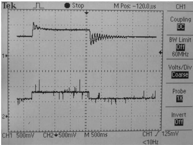
**Fig. 13.37** Experimental results when step changes are commanded from  $y_d = z_2^* = 0.006[m]$  to  $y_d = z_2^* = 0.008[m]$  and vice versa. Top line  $x_{2v} = y_v$ , bottom line  $x_{2v}^* = y_v^*$ . Controller gains in Table 13.4b)
