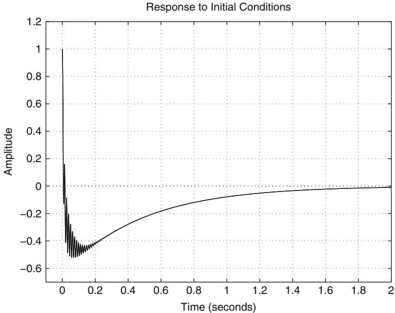
**Fig. 13.12** Plot of  $z_2(t)$  when  $z_1(0) = 0$ ,  $z_2(0) = 1$ ,  $z_3(0) = 0$ , and zero initial conditions for both integral parts of the controllers
