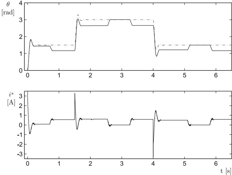
**Fig. 11.15** Classical proportional–integral–derivative (PID) position control ( $\alpha = 0.01$ ). Experimental results
