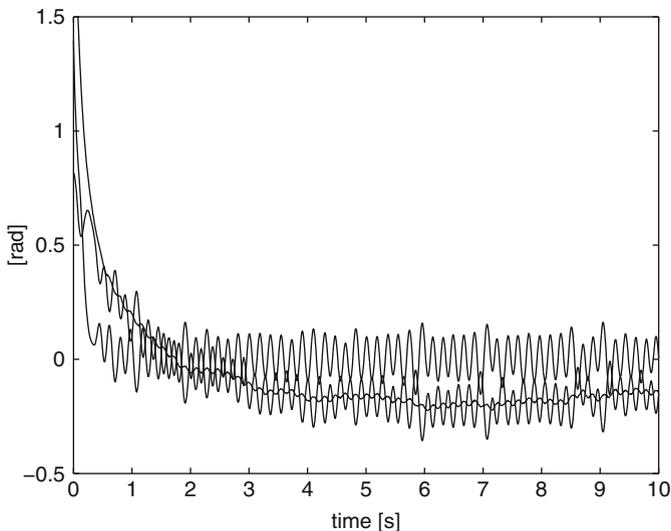
**Fig. 15.25** Experimental results when using the controller gains in Table 15.3d). Smallest amplitude oscillatory line:  $y$ [rad]. Lower oscillatory line:  $z_1$ [rad]. Upper oscillatory line:  $h_{z3}$ [rad]
