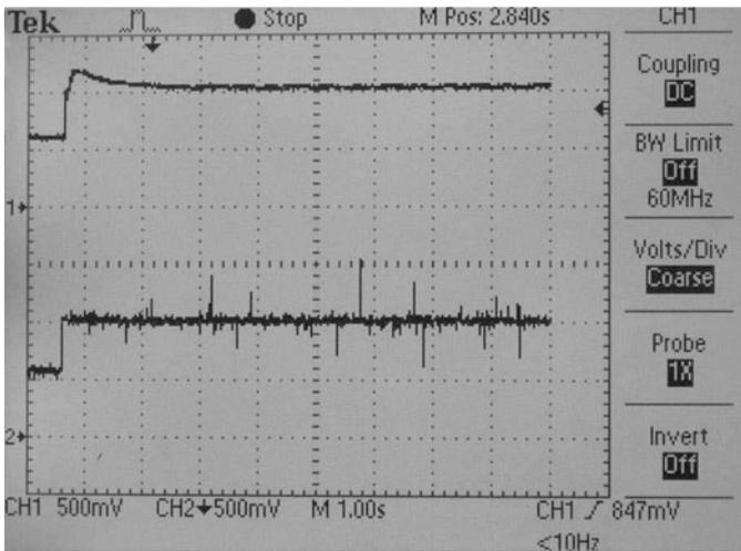
**Fig. 13.17** A step change in the desired position is commanded from  $y_d = x_2^* = 0.006[m]$  ( $y_v^* = 0.6[V]$ ) to  $y_d = x_2^* = 0.01[m]$  ( $y_v^* = 1.0[V]$ ) Top line  $x_{2v} = y_v$ , bottom line  $x_{2v}^* = y_v^*$
