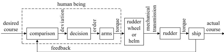
**Fig. 1.2** Actions performed when steering a ship
