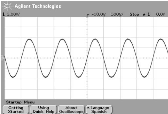
Fig. 9.22 Waveform of voltage at the output of the operational amplifier in Fig. 9.21. The potentiometer is at 20[KOhm]
