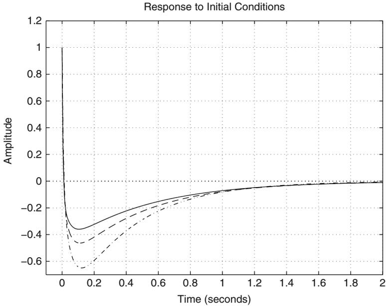
**Fig. 13.11** Plot of  $z_2(t)$  when  $z_1(0) = 0$ ,  $z_2(0) = 1$ ,  $z_3(0) = 0$ . Continuous: controller gains in (13.38). Dashed: controller gains in (13.34). Dotted line: controller gains in (13.36)
