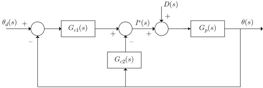
**Fig. 11.9** Closed-loop system with a two-degrees-of-freedom controller
