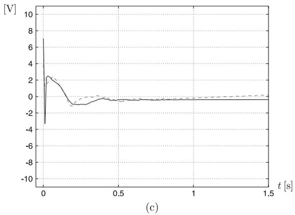
**Fig. 12.25** PID control of  $\theta_2$ . Experimental results. Continuous: PID gains in (12.21). Dashed: the design of the internal controller for  $\theta_1$  and the external PID controller for  $\theta_2$  is carried out using the root locus. The controller gains are given in (12.26) and (12.27) respectively. (a)  $\theta_2$ . (b)  $\theta_1$ . (c) Applied voltage,  $u$
