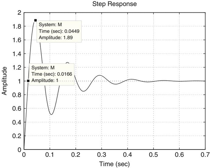
**Fig. 6.106** Time response when the reference is a unit step and a loop is closed around  $G(s)H(s) = (k_p + k_d s + \frac{k_i}{s}) \frac{k}{s^3 + 2739s^2 - 1250s - 3.536 \times 10^6}$  with  $k_d = 0.0131$ ,  $k_p = 1.0838$ ,  $k_i = 22.0341$
