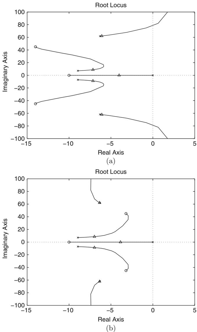
**Fig. 12.20** Root locus diagrams when the PID zeros do not cancel out the undesired open-loop poles at  $-6.304 \pm 61.7989j$  exactly. Triangles represent closed-loop poles in each case. In all cases  $k_{d2} = 0.0018$ . **(a)** PID zeros at  $-14 \pm 45j$ . **(b)** PID zeros at  $-3.2 \pm 45j$
