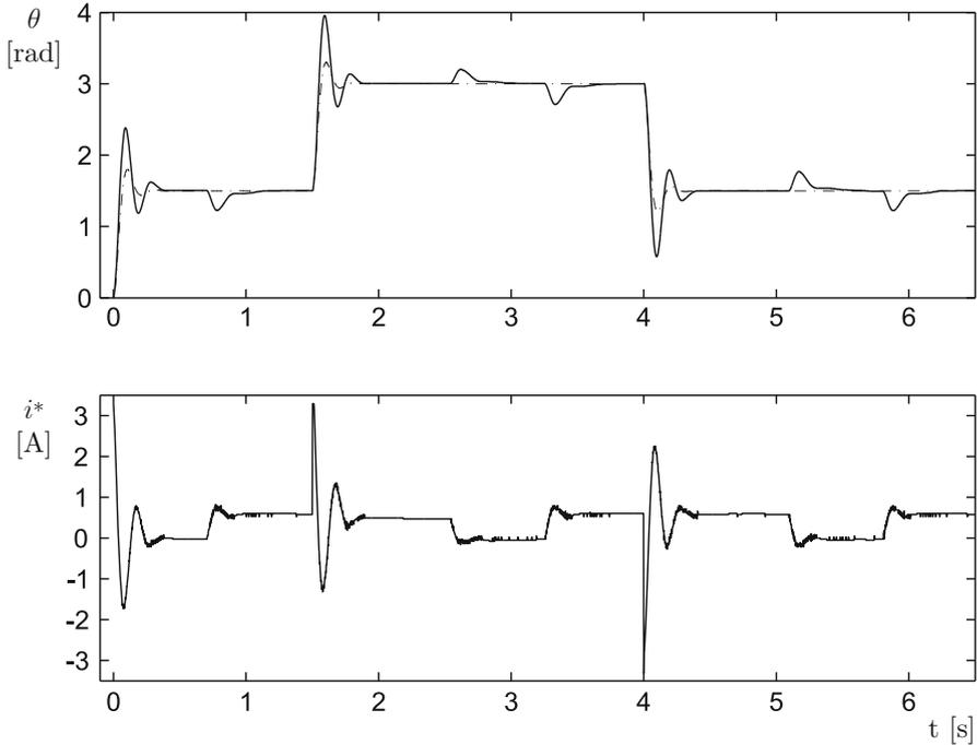
**Fig. 11.16** Classical PID position control ( $\alpha = 10$ ). Experimental results
