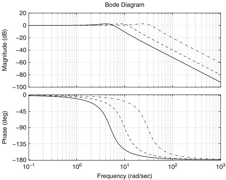
**Fig. 6.50** Bode diagrams of the transfer function  $M(s) = \frac{\omega_n^2}{s^2 + 2\zeta\omega_n s + \omega_n^2}$  when  $\zeta = 0.4$ . Continuous:  $\omega_n = 5$ . Dashed:  $\omega_n = 10$ . Dash-dot:  $\omega_n = 30$
