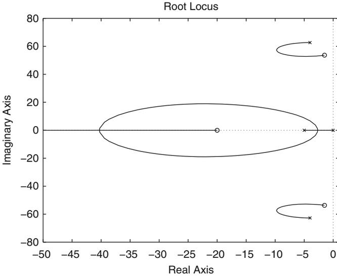
**Fig. 12.10** Root locus diagram for  $G(s)H(s) = k_{d1}(s + b_1)G_{1u}(s)$
