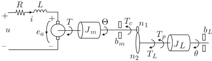
**Fig. 10.1** A loaded permanent magnet (PM) brushed direct current (DC) motor
