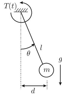
which is valid only when the pendulum remains close to the downward vertical configuration, i.e.,  $\theta$  is “small,”  $\theta \approx 0$  (see Example 7.5, Chap. 7). Find the required pendulum length  $l$  to produce oscillations with a period of 1 s.
