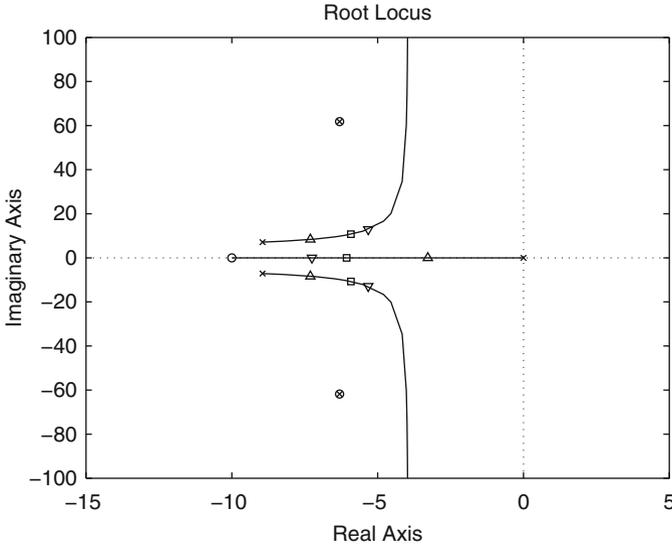
**Fig. 12.15** Root locus diagram for the open-loop transfer function in (12.18), (12.19). Some closed-loop poles are shown corresponding to three particular values of  $k_{d2}$ : triangle up  $k_{d2} = 0.0008$ , square  $k_{d2} = 0.0018$ , triangle down  $k_{d2} = 0.0028$
