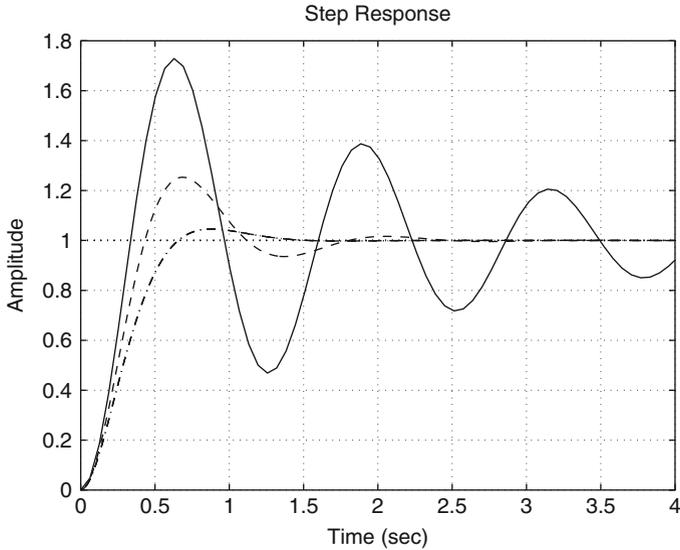
**Fig. 6.49** Response to a unit step input of the transfer function  $M(s) = \frac{\omega_n^2}{s^2 + 2\zeta\omega_n s + \omega_n^2}$  when  $\omega_n = 5$ . Continuous:  $\zeta = 0.1$ . Dashed:  $\zeta = 0.4$ . Dash-dot:  $\zeta = 0.7$
