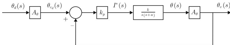
Fig. 14.5 Proportional control of the beam position
