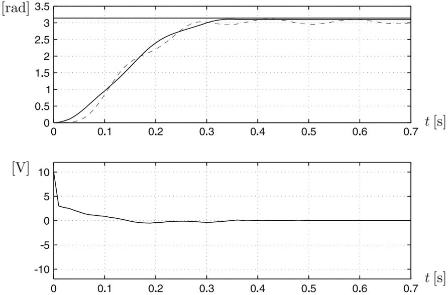
**Fig. 12.14** PD control of  $\theta_1$ . Experimental results. Top figure: continuous line  $\theta_1$ , dashed line  $\theta_2$ . Bottom figure: applied voltage  $u$ . The desired position is set to  $\theta_{1d} = \pi$  [rad]
