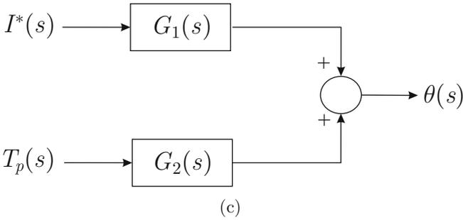
**Fig. 4.5** Simplifying the block diagram in Fig. 4.4c . (a) Block diagram when  $T_p(s) = 0$ . (b) Block diagram when  $I^*(s) = 0$ . (c) Block diagram equivalent to any of the block diagrams in Fig. 4.4
