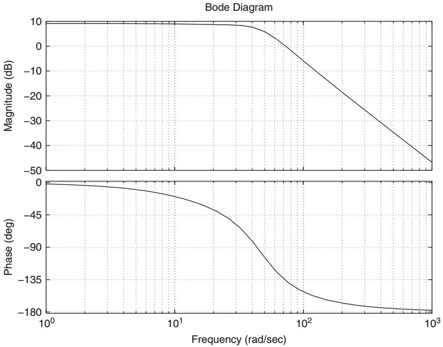
Fig. 6.99 Bode diagram of the closed-loop transfer function
