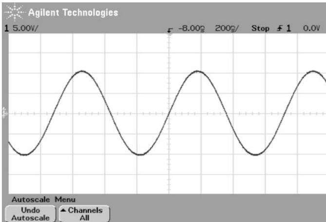
Fig. 9.46 Voltage waveform at the inductance terminals when  $R_t = 11000[\text{Ohm}]$
