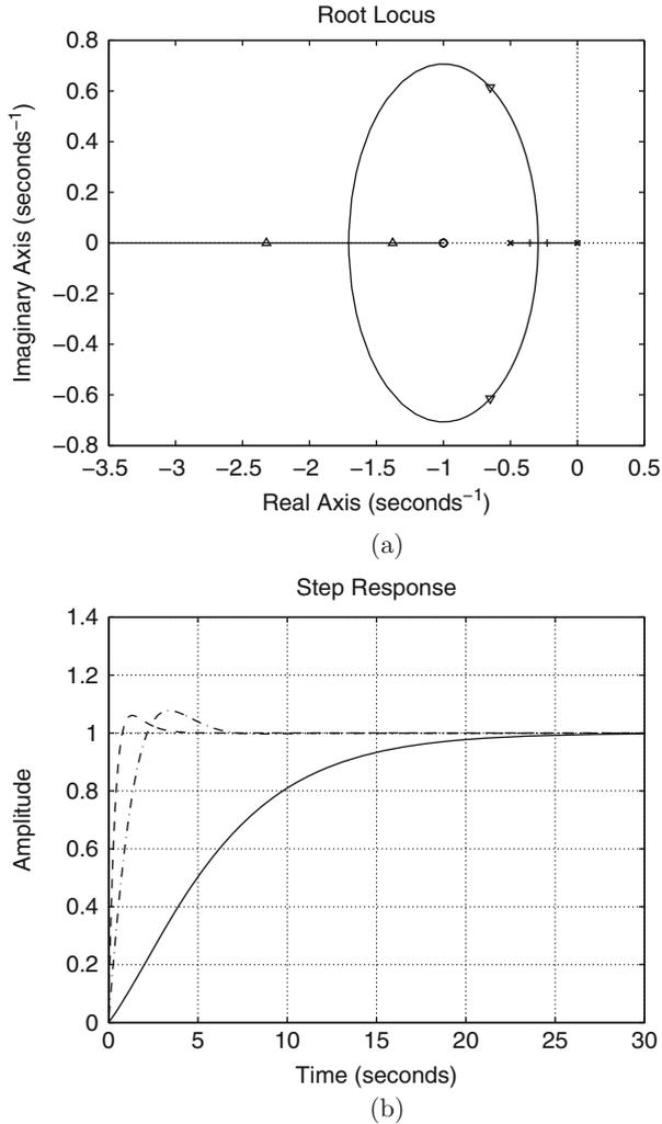
**Fig. 8.2** Root locus and closed-loop time response for system (1), when  $\frac{k_p}{k_d} = 1$  and  $k_d$  takes different values. **(a)** Closed-loop poles +:  $k_d = 0.01$ ; triangle down:  $k_d = 0.1$ ; triangle up:  $k_d = 0.4$ . **(b)** Continuous:  $k_d = 0.01$ ; Dash-dot:  $k_d = 0.1$ ; Dashed:  $k_d = 0.4$
