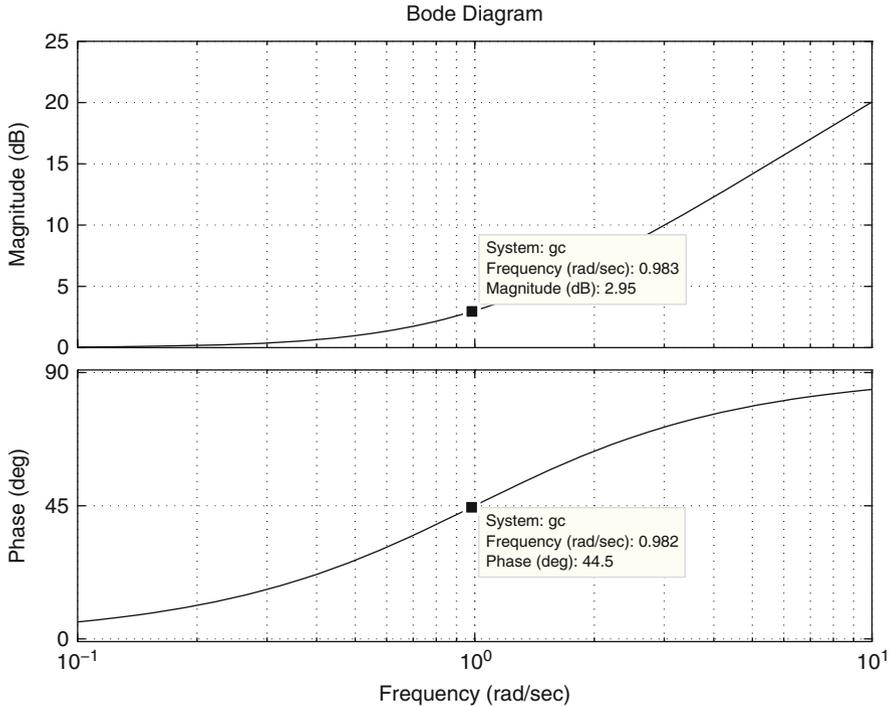
**Fig. 6.67** Bode diagrams of the factor  $z + 1$ . The horizontal axis represents  $\frac{1}{b}\omega$
