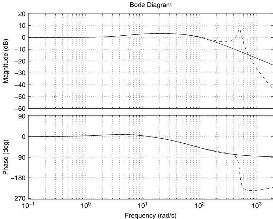
**Fig. 13.39** Closed-loop system Bode diagrams. Continuous: the electrical dynamics is not considered. Dashed: the electrical dynamics is taken into account. Controller gains in Table 13.4b) and  $k_{pi} = 4.7$ ,  $k_{ii} = 10000$
