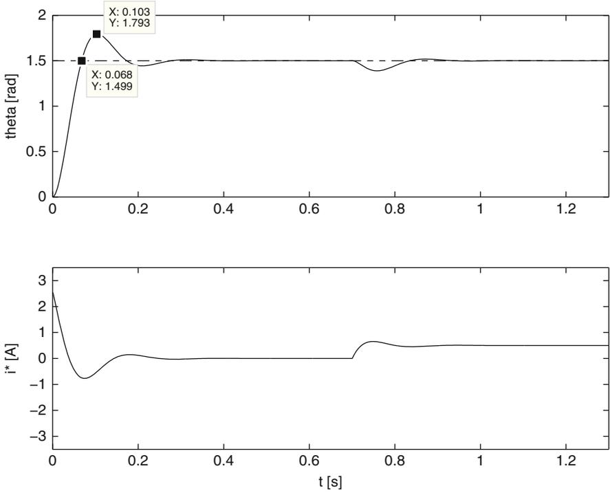
**Fig. 11.10** Position control using a two-degrees-of-freedom controller. Simulation results ( $\theta_d = 1.5$ [rad])
