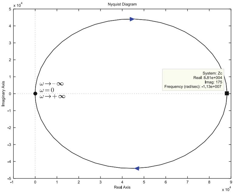
**Fig. 9.47** Polar plots using the numerical values for the circuit experimentally tested . (a)  $M(s)$ . (b)  $Z_c(s)$
