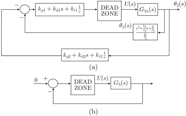
Fig. 12.34 Closed-loop diagrams for limit cycle analysis
