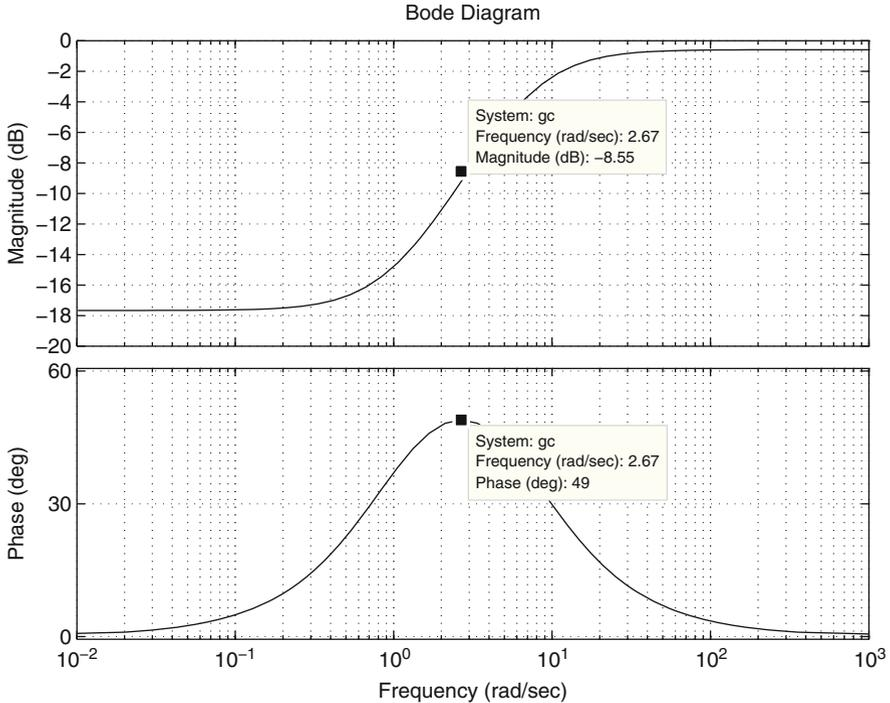
Fig. 6.86 Bode diagrams of  $G_d(Ts)$  in (6.55). Horizontal axis stands for  $T\omega$
