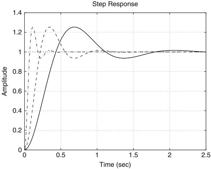
**Fig. 6.51** Response to a unit step input of the transfer function  $M(s) = \frac{\omega_n^2}{s^2 + 2\zeta\omega_n s + \omega_n^2}$  when  $\zeta = 0.4$ . Continuous:  $\omega_n = 5$ . Dashed:  $\omega_n = 10$ . Dash-dot:  $\omega_n = 30$
