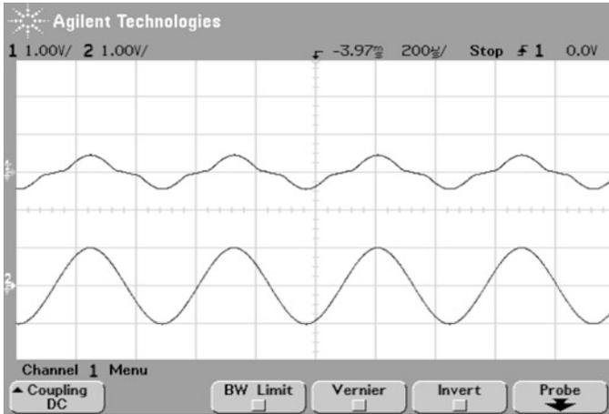
**Fig. 9.11** Experimental results. Voltages at the input and the output of the circuit in Fig. 9.6. Upper line:  $V_o$ , bottom line:  $u$
