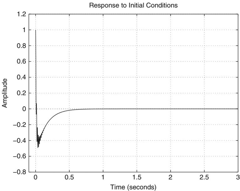
**Fig. 13.38** Simulated time response when taking into account the electrical dynamics and the PI electric current controller. Controller gains in Table 13.4b) and  $k_{pi} = 4.7$ ,  $k_{ii} = 10000$
