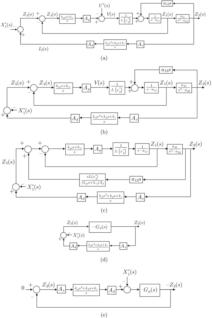
**Fig. 13.8** Equivalent block diagrams of the control system. The disturbance  $-X_1^*(s)$  is only taken into account when the switch SW2 is open in Fig. 13.3 or, equivalently, when the switch SW2 selects the signal “0” in Fig. 13.7
