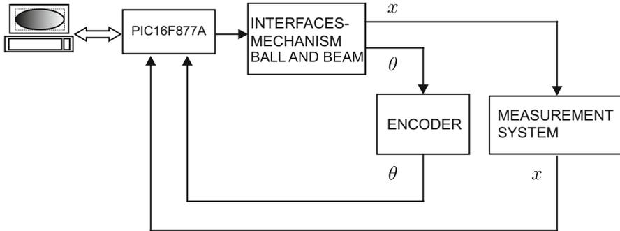
**Fig. 14.2** Block diagram of the complete control system. Block interfaces–mechanism ball and beam is shown in Fig. 14.19. Block measurement system is shown in Fig. 14.3
