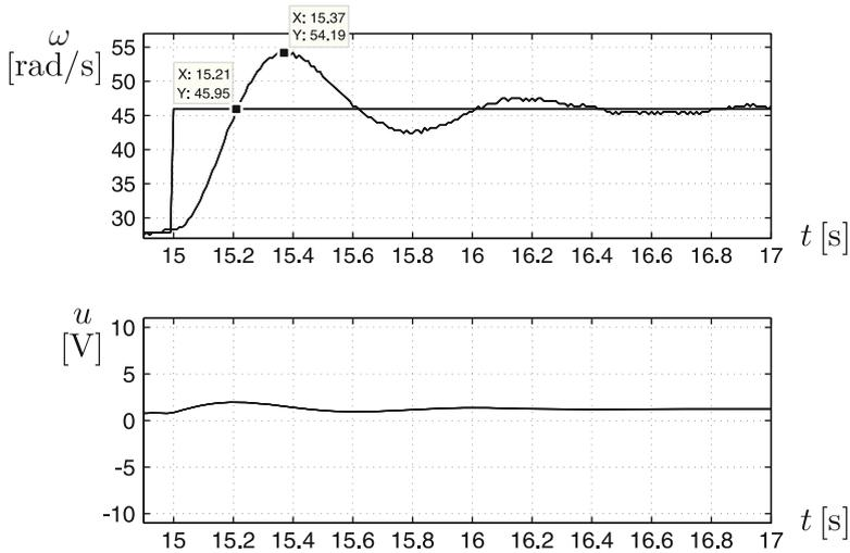
**Fig. 10.17** Experimental response of the control system in Fig. 10.16, i.e., an integral controller of velocity with  $k_i = 1, k_p = 0$
