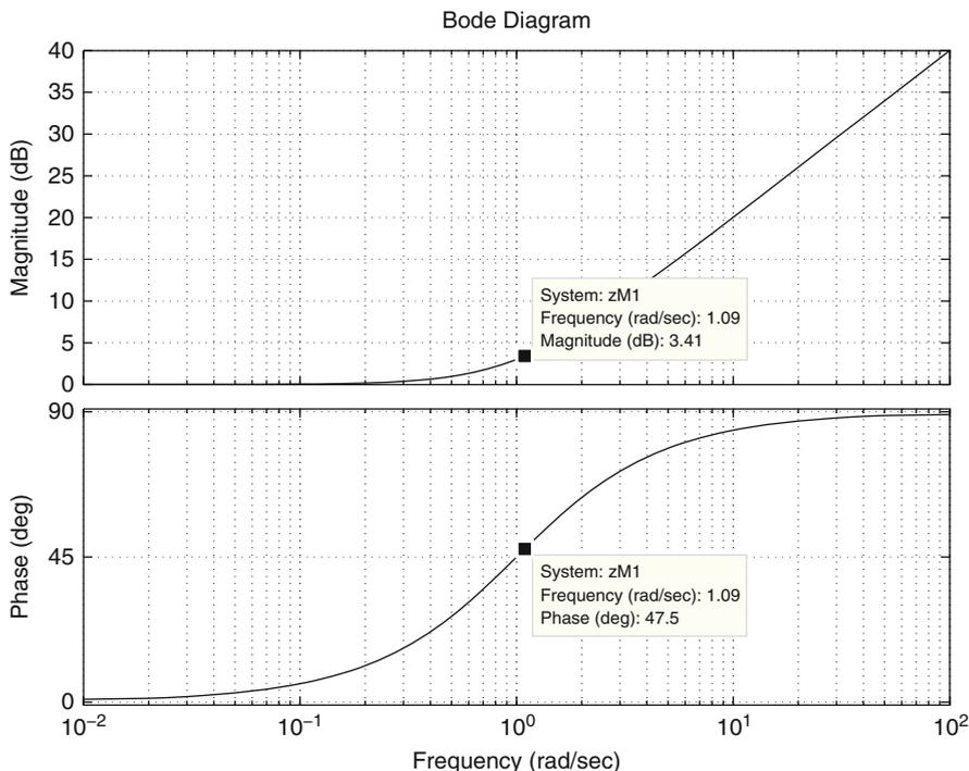
Fig. 11.29 Bode diagrams of the factor  $z + 1$ . The horizontal axis represents  $\frac{\omega}{z_2}$
