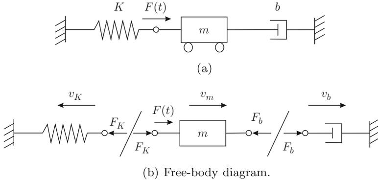
**Fig. 2.5** A mass-spring-damper system
