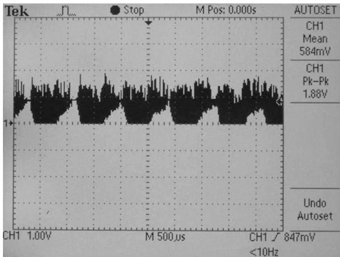
**Fig. 13.20** Waveform of the electric current flowing through the power transistor TIP 141 when  $k_i = 10^5$
