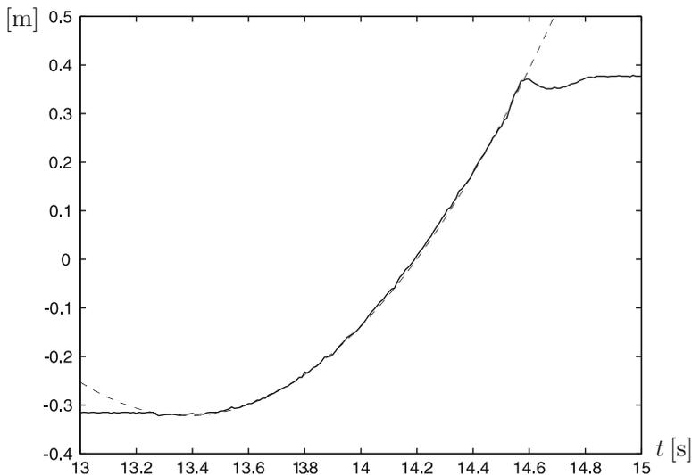
**Fig. 14.7** Experimental identification of the parameter  $\rho$ . Continuous:  $x(t)$  measured in the experiment. Dashed:  $x(t) = \frac{1}{2}\rho\theta_0(t - 13.38)^2 - 0.322$ ,  $\theta_0 = 0.2[\text{rad}]$ ,  $\rho = 4.8$
