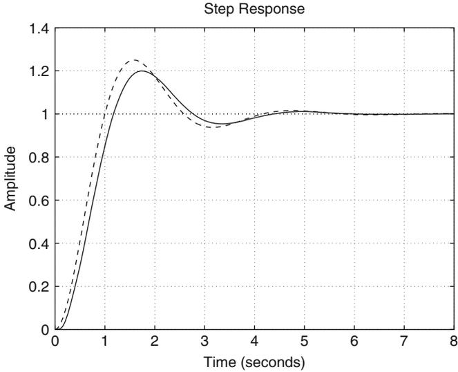
**Fig. 5.56** Closed-loop time response of the ball and beam system according to the block diagram in Fig. 5.53 and controller gains  $b = 1.4$ ,  $c = 5.1138$ ,  $\gamma = 2.1868$  (continuous). Dashed: desired response
