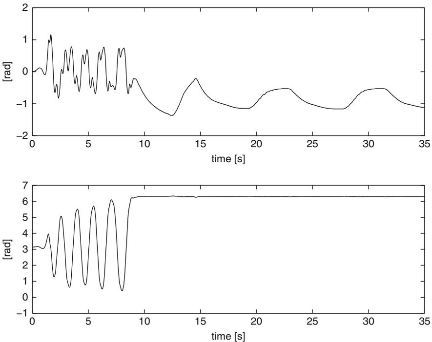
**Fig. 15.10** Experimental results when using the controller gains in Table 15.3a). Top line:  $\theta_0$ [rad]. Bottom line:  $\theta_1$ [rad]
