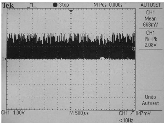
**Fig. 13.21** Waveform of the electric current flowing through the power transistor TIP 141 when  $k_i = 10^6$
