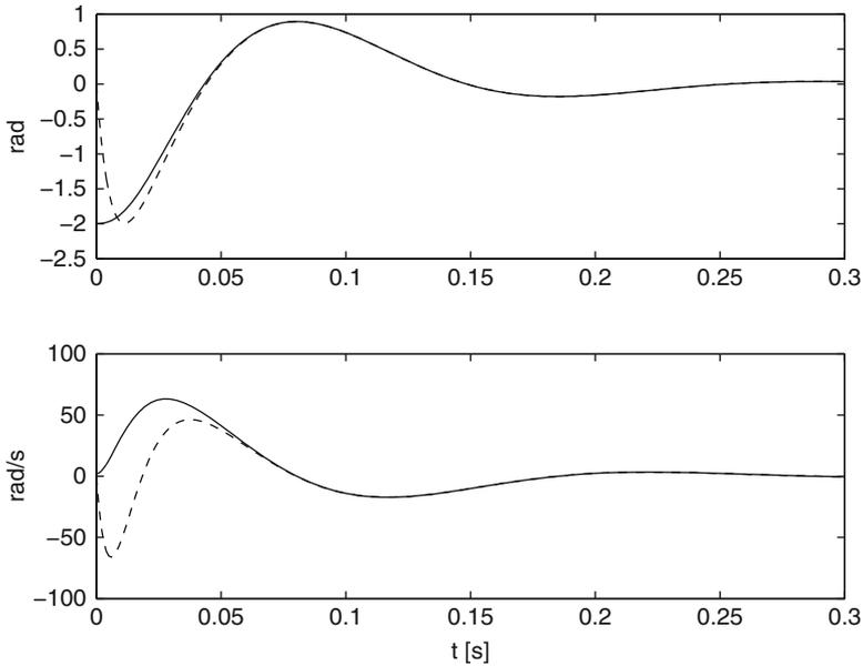
**Fig. 7.9** Simulation results. Use of the observer in (7.94) to control a DC motor Top figure: continuous  $\tilde{x}_1$ , dashed  $z_1$  Bottom figure: continuous  $\tilde{x}_2 = x_2$ , dashed  $z_2$
