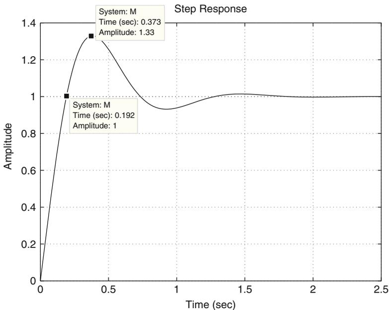
Fig. 11.31 Simulation response of the closed loop system in Fig. 11.27.  $k_d = 0.0935$ ,  $k_p = 1.0177$ ,  $k_i = 2.4697$
