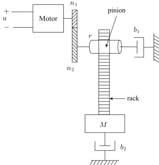
**Fig. 2.33** Free-body diagrams corresponding to the servomechanism in Fig. 2.32
