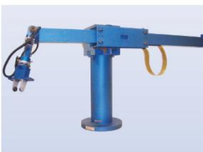
**Prismatic joints.** Robot joints are commonly revolute (rotational) but can also be prismatic (linear, sliding, telescopic, etc.). The SCARA robot of Fig. III.1b has a prismatic third joint while the gantry robot of Fig. III.1c has three prismatic joints for motion in the  $x$ -,  $y$ - and  $z$ -directions.
