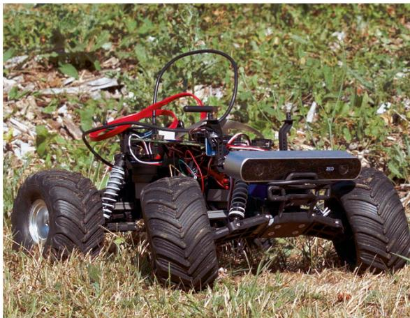
**Fig. 14.19.** A small stereo camera sensor mounted on a mobile robot and capable of real-time depth map generation (image courtesy of Stereolabs Inc.)
