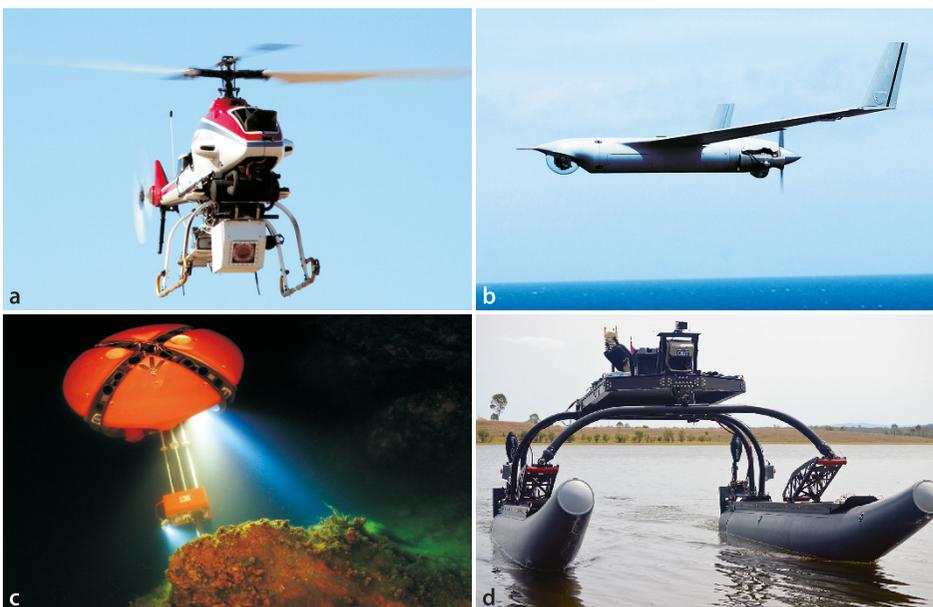
**Fig. II.3.** Some mobile air and water robots: **a** Yamaha RMAX helicopter with 3 m blade diameter (photo by Sanjiv Singh). **b** Fixed-wing robotic aircraft (photo of ScanEagle courtesy of Insitu). **c** DEPTHX: Deep Phreatic Thermal Explorer, a 6-thruster under-water robot. Stone Aerospace/CMU (2007) (photo by David Wettergreen, © Carnegie-Mellon University). **d** Autonomous Surface Vehicle (photo by Matthew Dunbabin)
