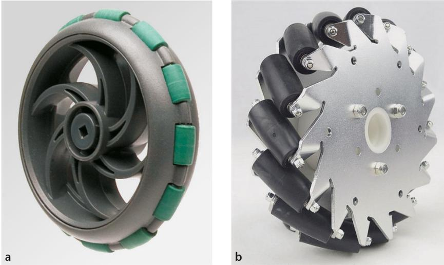
**Fig. 4.15.** Two types of omnidirectional wheel, note the different roller orientation. **a** Allows the wheel to roll sideways (courtesy Vex Robotics); **b** allows the wheel to drive sideways (courtesy of Nexus Robotics)
