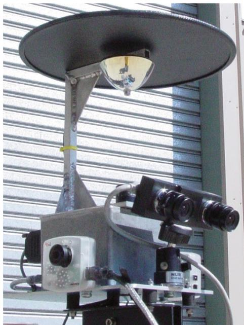
Fig. IV.2. A cluster of cameras on an outdoor mobile robot: forward looking stereo pair, side looking wide angle camera, overhead panoramic camera mirror (CSIRO mobile robot)
