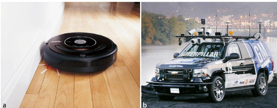
**Fig. II.2.** Some mobile ground robots: **a** The Roomba robotic vacuum cleaner, 2008 (photo courtesy iRobot Corporation). **b** *Boss*, Tartan racing team's autonomous car that won the Darpa Urban Grand Challenge, 2007 (Carnegie-Mellon University)
