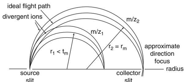
**Fig. 4.20** Direction focusing properties of a  $180^\circ$  magnetic sector on a diverging beam of ions of the same  $m/z$  and the same kinetic energy and effect on ions of different  $m/z$ . In this illustration,  $B$  has to come out of the plane towards the reader for positive ions
