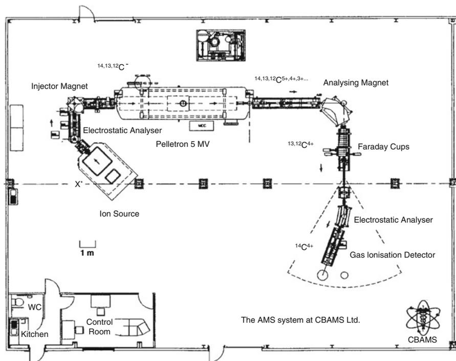
**Fig. 15.20** AMS facility of CBAMS. The instrument is typical for its kind. Note the scale bar for 1 m. CBAMS, founded in 1997, is the first private company in the world to offer a fully commercial analytical service using an accelerator mass spectrometer (Reproduced from Ref. [14] with permission. © John Wiley & Sons, Ltd., 1999)
