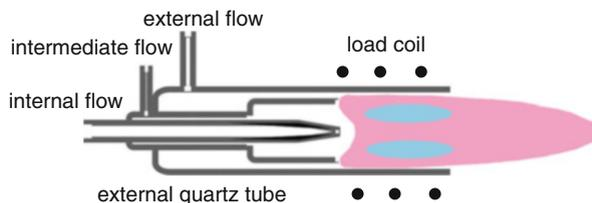
**Fig. 15.10** ICP torch. Three concentric quartz tubes deliver the internal flow containing the sample, the intermediate argon flow to support the plasma, and an external flow to provide cooling to the outer wall. The temperature reaches about 10,000 K inside the coil and drops to about 6000 K at the tip of the plasma from where ions are collected at the sampling cone (Adapted from Ref. [71] with permission. © Royal Chemical Society, 2015)
