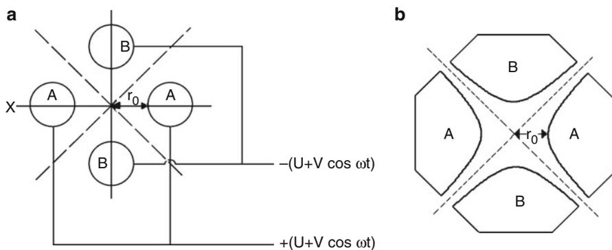
**Fig. 4.30** Cross section of a quadrupole (a) for the cylindrical approximation and (b) for the hyperbolic profile of the rods. The electric field is zero along the *dotted lines*, i.e., along the asymptotes in (b) (a) Courtesy of Waters Corp., MS Technologies, Manchester, UK
