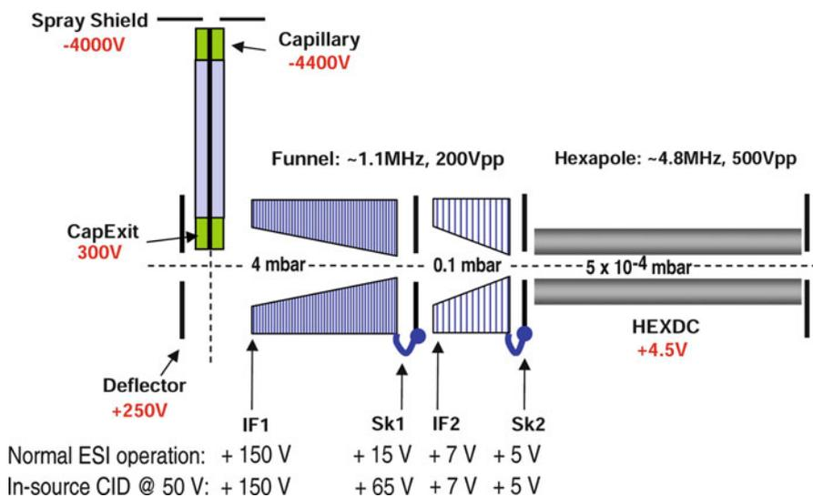
**Fig. 12.12** ESI interface with differential pumping in a dual ion funnel arrangement (Bruker Apollo II™). In normal ESI operation the main DC gradient is located in the first ion funnel while ions drop only by about 8 V into the second. Lifting the exit potential of the first funnel causes the ions to enter the second ion funnel at much higher velocity, which is sufficient for NSD (Courtesy of Bruker Daltonik GmbH, Bremen)
