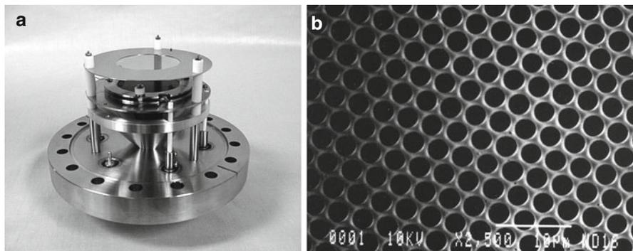
**Fig. 4.96** MCP detector (top inner, glossy disk) mounted on top of a flange (a) and SEM micrograph of a high-resolving MCP showing channels of 2  $\mu\text{m}$  diameter (b) (By courtesy of (a) R.M. Jordan Company, Grass Valley, CA and of (b) Burle Industries, Baesweiler)
