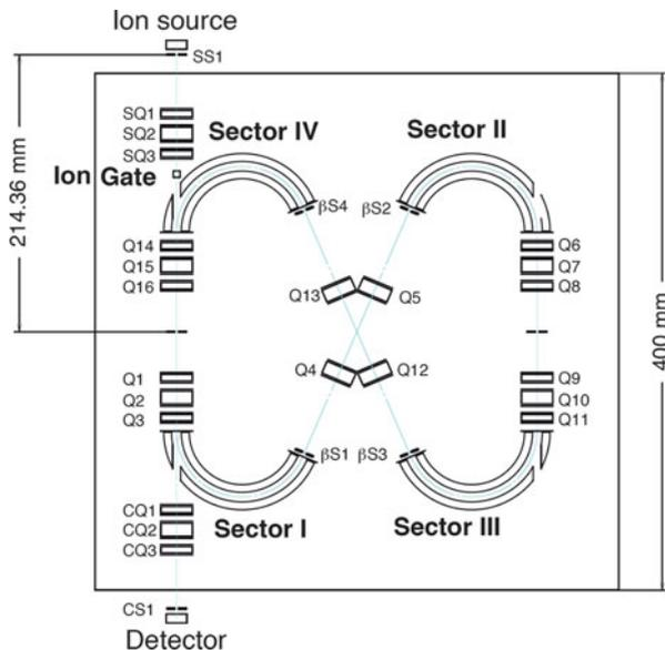
**Fig. 4.14** Simulated ion trajectories in the MULTUM Linear plus (cf. Fig. 4.13). The *arrows* indicate the direction of ion motion (Adapted from Ref. [44] by permission. © John Wiley & Sons, 2003)
