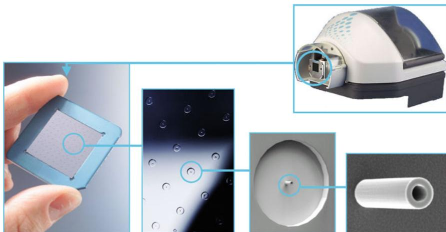
**Fig. 12.16** Chip-based Advion nanoESI system. The pictures stepwise zoom in from the pipetting unit to the spray capillary on the silicon chip (By courtesy of G. Schultz, Advion BioSciences, Ithaca, NY)
