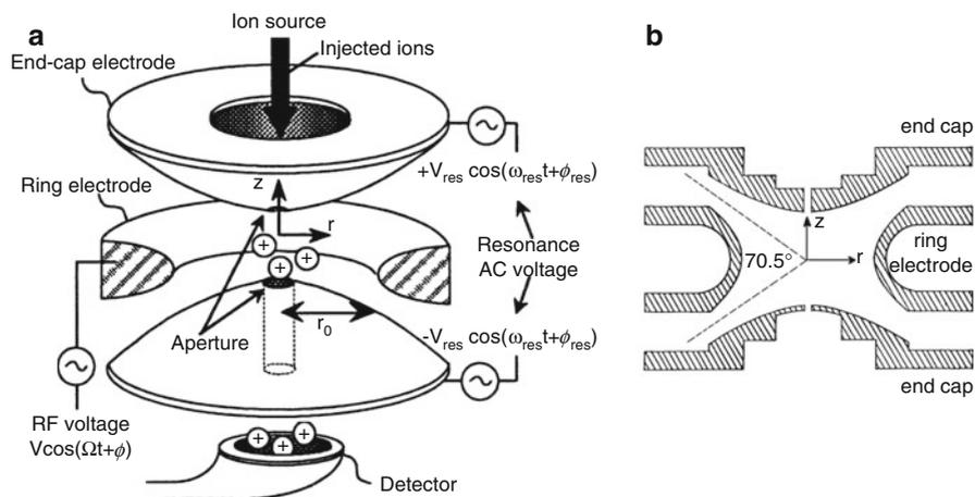
**Fig. 4.52** A quadrupole ion trap. (a) QIT with external ion source (illustration stretched in  $z$ -direction) and (b) section in the  $rz$ -plane (in scale). (a) (Reproduced from Ref. [153] by permission. © John Wiley & Sons, 2000)
