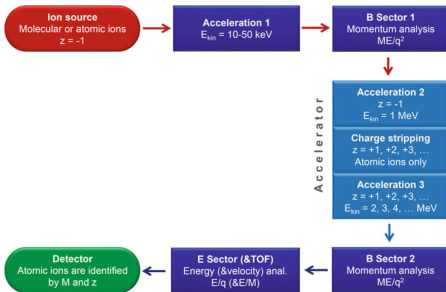
**Fig. 15.19** Sequence of events and general experimental setup of AMS [4]. The instrument consists of a medium ion kinetic energy section, an ion accelerator, and a high-energy section to detect multiply charged atomic ions at highest sensitivity and specificity
