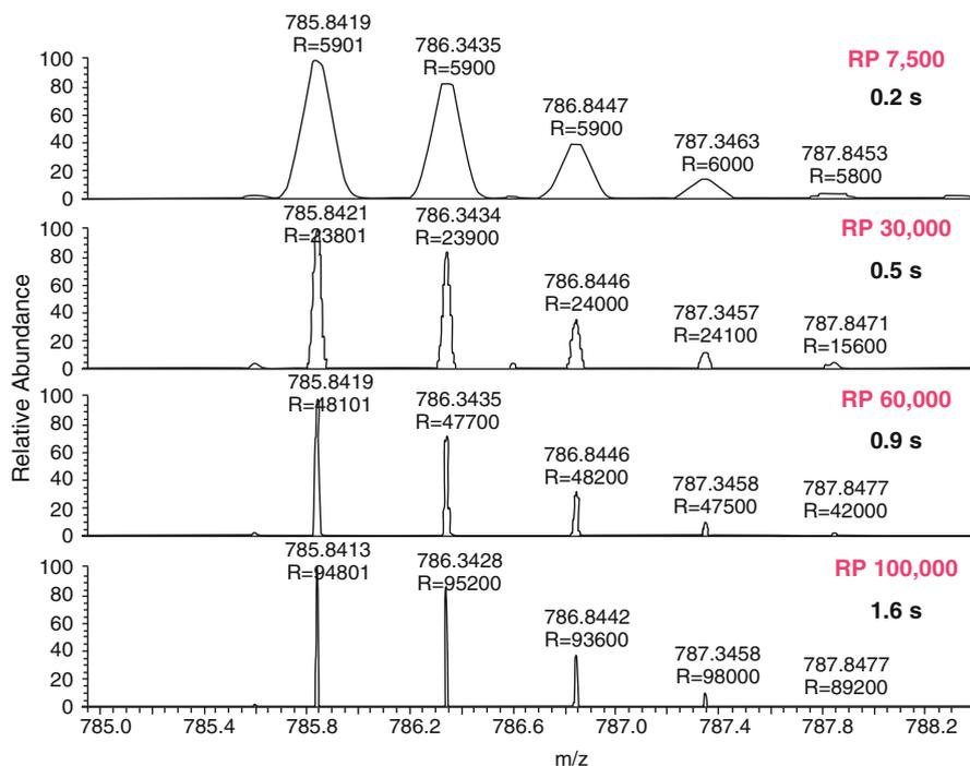
**Fig. 4.80** Resolving power of a commercial Orbitrap instrument as achieved for doubly charged peptide ions at detection intervals ranging from 95 to 1267 ms resulting in cycle times from 0.2 to 1.6 s. The cycle times are longer than pure detection intervals due to preparation of ion packets, data processing etc. The values specified are calculated with reference to the manufacturer's standard value of  $m/z$  400 (Reproduced from Ref. [241] with permission. © Wiley-VCH, Weinheim, 2006)
