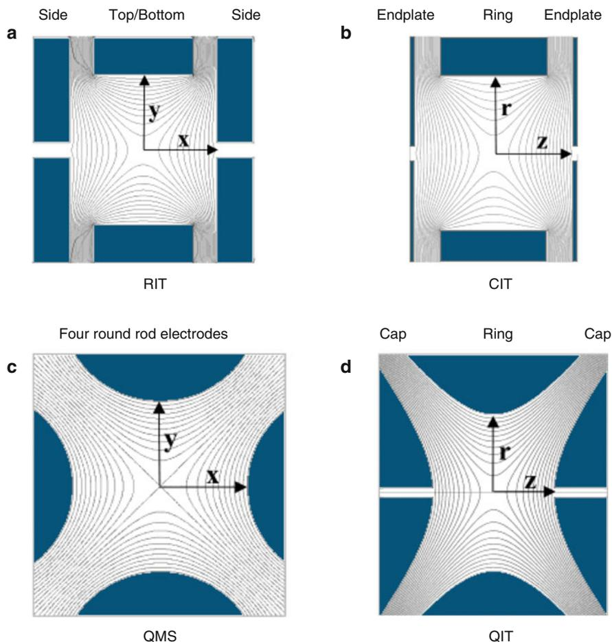
**Fig. 4.59** Calculated trapping fields for (a) a rectilinear ion trap, (b) a cylindrical ion trap with planar endplates, (c) a quadrupole mass filter with round rods, and (d) a quadrupole ion trap with hyperbolic electrodes (Paul trap). Analyzer views (a) and (c) are end-on, (b) and (d) side-on (Adapted from Ref. [185] with permission. © American Chemical Society, 2004)
