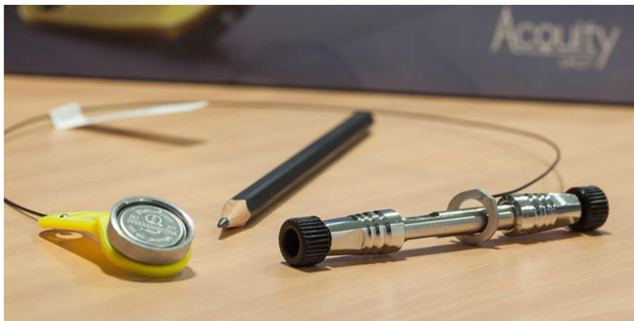
**Fig. 14.8** UPLC column. The actual column (*right*), here shown with the two end caps still in place, is quite small as by comparison to the pencil. This particular column is a Waters BEH C18 reversed phase type of 50 mm length and 2.1 mm inner diameter filled with 1.7- $\mu\text{m}$ -sized particles. The column is locked to a transponder (*left*) that is used to identify the column by the data system
