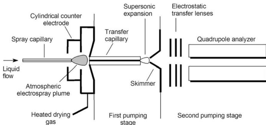
**Fig. 12.3** Schematic of an early electrospray interface design [16]
