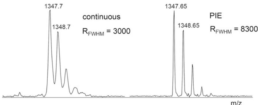
**Fig. 4.11** MALDI-TOF spectra of substance P, a low-mass peptide, as obtained from a Bruker Biflex ReTOF in continuous extraction reflector mode (in 1995, *left*) and after PIE upgrade of this instrument (in 2001, *right*)
