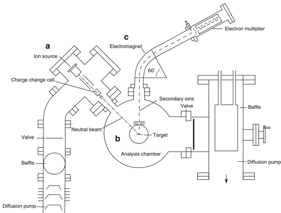
**Fig. 10.1** MBSA instrument. The noble gas is ionized in the primary ion source (a) and ions of the gas are accelerated and guided through a charge transfer cell. The neutral beam hits a target in the analytical ion source (b) where sample material gets sputtered and ionized. Ions are extracted for mass analysis into a magnetic sector analyzer (c) (Reproduced from Ref. [7] by permission. © Wiley, 1982)
