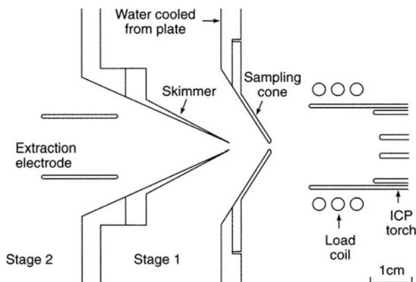
**Fig. 15.12** Ion extraction interface for ICP-MS. Ions arrive from the right, a small portion is transmitted through the water-cooled sampling cone into the first pumping stage (rotary pump), the center of the free-jet expansion is then transmitted through the second skimmer cone, behind which it is guided by electric potentials through the second pumping stage (turbo pump) into the mass analyzer (Reprinted with permission from Ref. [3]. © John Wiley & Sons Ltd., 1997)
