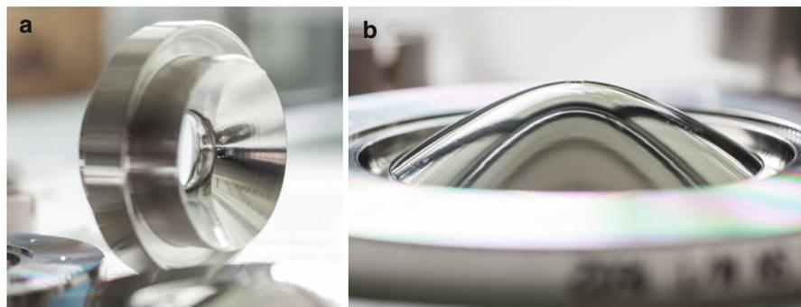
**Fig. 4.53** Electrodes of the Finnigan LCQ quadrupole ion trap analyzer. (a) Ring electrode with symmetrical hyperbolic cross section of the inner walls of the ring. (b) One of the pair of hyperbolic end cap electrodes
