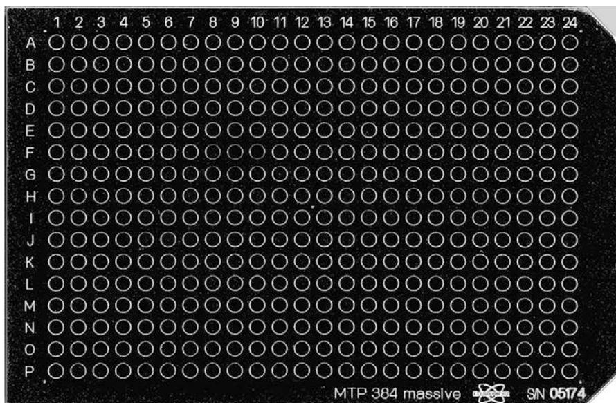
**Fig. 11.12** Typical MALDI target: Bruker Scout384™ target offers a 16 × 24 spot array with up to 384 positions for sample preparation. Here, a standard nickel-coated massive aluminum version is shown; its dimensions are 84 × 128 mm with engraved marks of 3 mm in diameter
