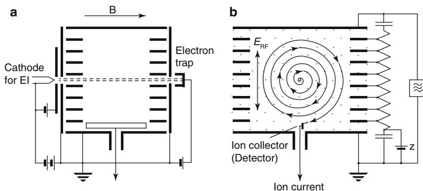
**Fig. 4.66** Omegatron. (a) View parallel to  $B$  (*horizontal*) and parallel to the electron beam (*horizontal*) used to generate ions by EI inside the cell. The accelerating electric RF field acts vertical to  $B$ . (b) View on-axis to  $B$  shows the spiral motion of accelerating ions until the radius of their orbit approaches that of the cell where the ions hit an ion collector for detection (Adapted from Ref. [91] with kind permission of Curt Brunnée)
