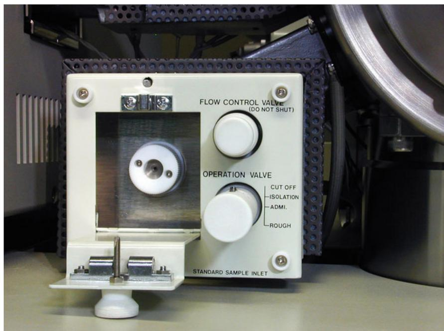
**Fig. 5.6** Reservoir inlet of a JEOL JMS-700 sector instrument with the septum injection port opened. The “operation valve” switches between evacuation, isolation, and admission of the sample; a needle valve allows regulation of the sample flow. The GC transfer line crosses in the upper background from the GC (*left*) to the ion source housing (*upper right*)
