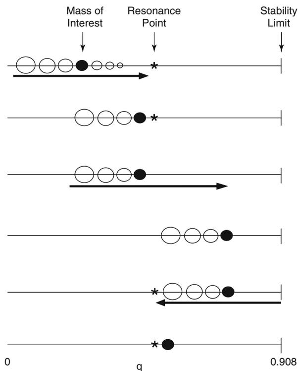
**Fig. 9.22** The principle of isolation of a precursor ion by using forward and reverse scanning of a QIT. Ions smaller than the precursor are ejected by exciting them above the stability limit at  $q = 0.908$ , then settings are changed so that reduction of the RF amplitude causes ejection of the heavier ions (Reproduced from Ref. [109] with permission. © John Wiley & Sons, 1992)
