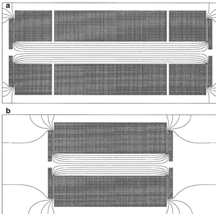
**Fig. 4.49** SIMION simulation of the resonance excitation field comparing (a) a three-section ion trap and (b) a single-section device with end plates for trapping. In (a) the field inside the trapping compartment remains unperturbed from fringing fields (Adapted with permission from Ref. [130]. © Elsevier Science Publishers, 2002)
