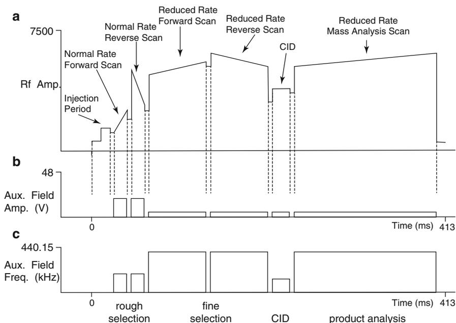
**Fig. 9.23** Sequence of changes of (a) RF amplitude, (b) auxiliary voltage amplitude, and (c) auxiliary voltage frequency to first achieve a rough precursor ion selection, then a fine selection by repetition at slow rates, followed by CID, and product ion scan (Adapted from Ref. [109] with permission. © John Wiley & Sons, 1992)
