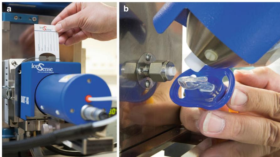
**Fig. 13.30** DART configurations in use. (a) Open Source for transmission mode DART with disposable sample cards (corresponds to setup **b** in Fig. 13.29), (b) alignment at an angle of  $45^\circ$  for the analysis of objects placed in the gap (corresponds to setup **c** in Fig. 13.29). Both photos show the DART source attached to a Bruker instrument by means of the Vapur Interface
