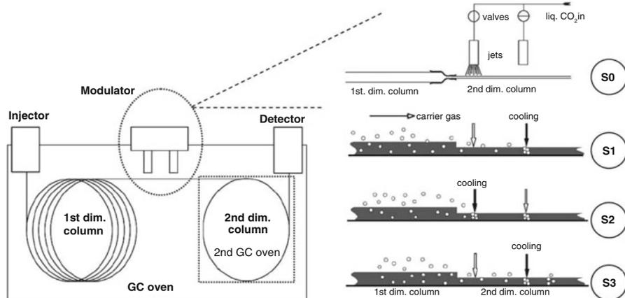
**Fig. 14.6** Schematic of GC  $\times$  GC instrumentation (*left*) and operation (*right*). The eluate from the first column is collected, e.g., by a dual-jet cryogenic modulator. The modulator switches from trapping to evaporation mode on two short adjacent segments at the junction of the columns (Reproduced from Ref. [24] with permission. © Elsevier, 2006)
