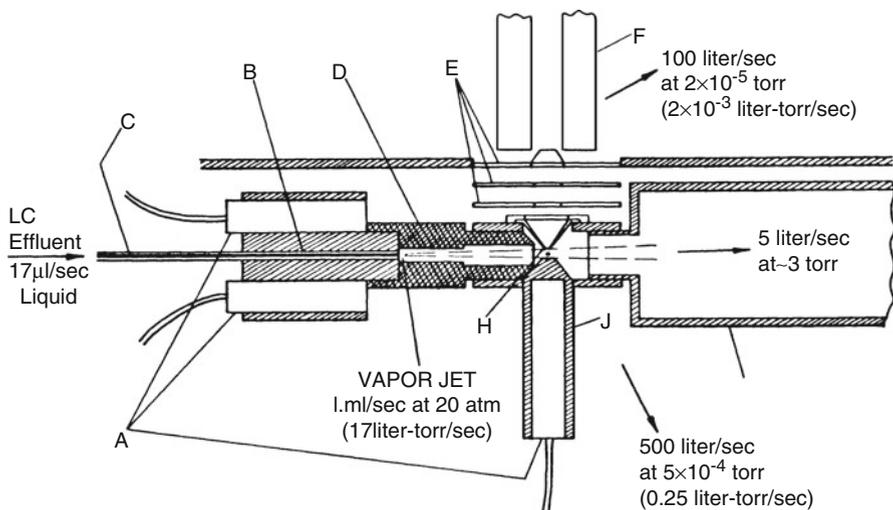
**Fig. 12.2** Thermospray interface. *A* cartridge heater; *B* copper block brazed to stainless steel capillary; *C* capillary; *D* copper tube; *E* ion lenses; *F* quadrupole mass analyzer; *G* line to rotary vane pump; *H* ion exit aperture; *J* source heater (Reproduced from Ref. [35] by permission. © American Chemical Society, 1983)
