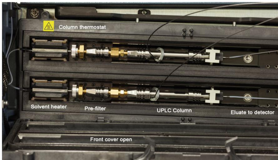
**Fig. 14.10** A column thermostat of a Waters Acquity system with two UPLC columns mounted inside. The sample solution first passes a heater cartridge to ensure constant temperature equal to that of the column, then a pre-filter to prevent the column from clogging, and finally enters the UPLC column. The column compartments of the thermostat are inclined to direct solvent towards a drain in case of a leakage
