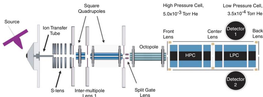
**Fig. 9.28** The Thermo Fisher LTQ Velos instruments have a dual linear ion trap, the first section of which is operated at higher pressure (HPC), the second is run at lower pressure to achieve better resolving power (LPC). The dual LIT design also increases the speed of operation, because the first LIT can already prepare ions for the second while this is still mass-analyzing fragments from the previous cycle (Reprinted from Ref. [119] with permission. © American Chemical Society, 2009)
