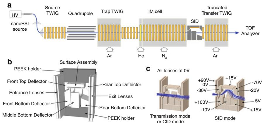
**Fig. 9.10** Waters Synapt G2 modified to incorporate a SID device in front of the transfer TWIG. (a) Setup of the instrument (dimensions of the ion optics are not to scale). (b) 3D perspective view of the SID device assembly. (c) Cutaway views of a SIMION simulation showing the ion paths in transmission mode versus SID mode. The voltages on the SID lenses are given relative to the potential on the transfer TWIG (Reproduced from Ref. [40] with permission. © American Chemical Society, 2012)
