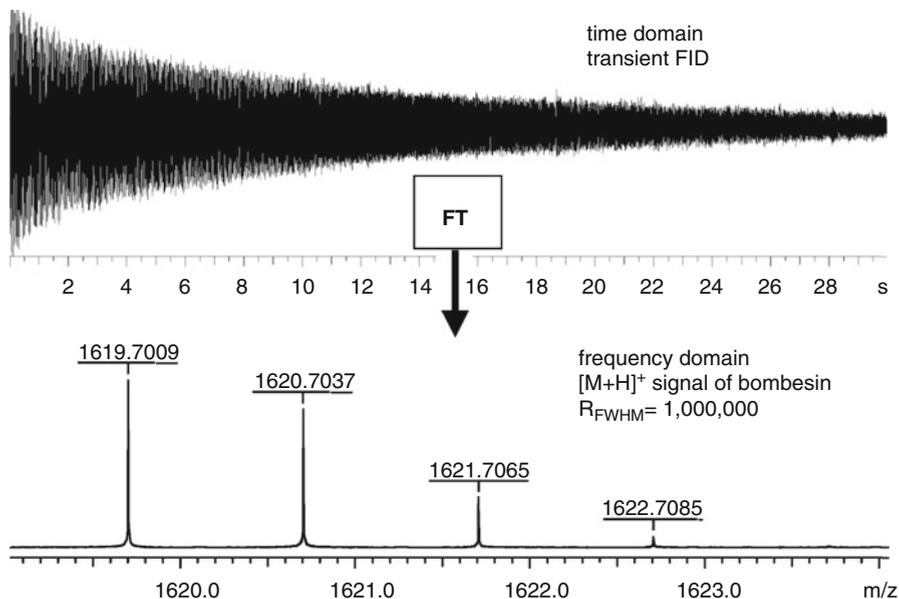
**Fig. 4.73** The principle of FT-ICR-MS. In detail, the procedure includes recording the transient, apodization of the transient, zero-filling, FT, and finally the calculation of  $m/z$  values from the cyclotron frequencies. The longer the detection interval the higher the attainable resolving power. This example shows the  $[M + H]^+$  ion of the peptide bombesin,  $m/z$  1619.7009, where a 30 s transient resulted in a spectrum at  $R = 10^6$  (By courtesy of Bruker Daltonik, Bremen)
