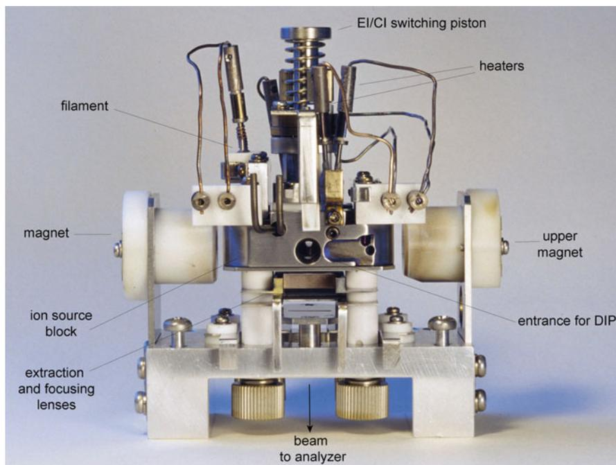
**Fig. 5.2** EI/CI/FAB combination ion source of a JEOL JMS-700 sector instrument
