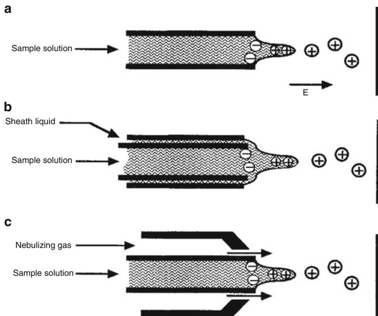
**Fig. 12.5** Different sprayers for ESI. (a) Pure electrospray, (b) ESI with sheath liquid, (c) pneumatically-assisted ESI (Adapted from Ref. [6] (p. 109) by permission. © John Wiley & Sons, Inc., 1997)
