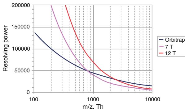
**Fig. 4.81** For an Orbitrap analyzer the drop in resolving power with increasing  $m/z$  is less pronounced than for FT-ICR instruments. While FT-ICR clearly outperforms Orbitraps up to  $m/z$  8000 (7 T, pink line) or even  $m/z$  2500 (12 T, red line) the Orbitrap can deliver somewhat better resolving power in the high mass range (blue line) (Reproduced from Ref. [241] with permission. © Wiley-VCH, Weinheim, 2006)
