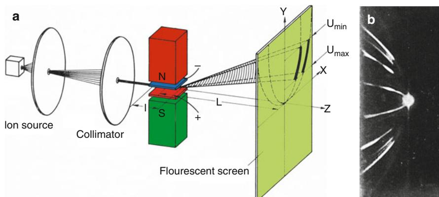
**Fig. 1.2** Parabola spectrograph as constructed by J. J. Thomson. (a) Schematic, (b) photograph of the light emission from the fluorescent screen as obtained with this instrument (shown rotated by  $90^\circ$  with respect to the schematic) (Adapted from Ref. [31] with kind permission of Curt Brunnée)
