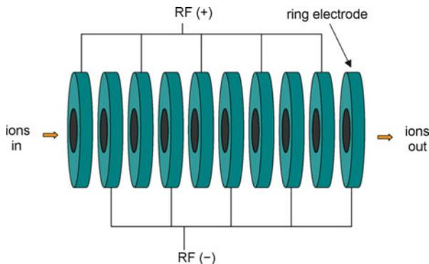
**Fig. 4.88** A stacked ring ion guide. Rings are connected to an RF drive voltage in alteration of the phase. Normally tens of pairs are used to build one ion guide. Ions entering from the left experience a deep radial potential well with comparatively steep walls toward the inner ring surfaces when traveling through the apertures (Reproduced from Ref. [281] with permission. © Elsevier Science Publishers, 2007)
