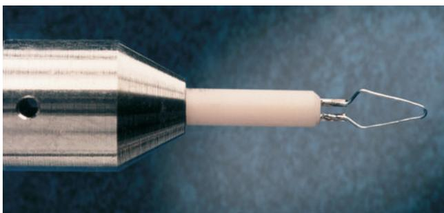
**Fig. 5.16** Tip of a direct exposure probe of a GC-*oa*TOF mass spectrometer for EI and CI (By courtesy of Waters Corporation, MS Technologies, Manchester, UK)
