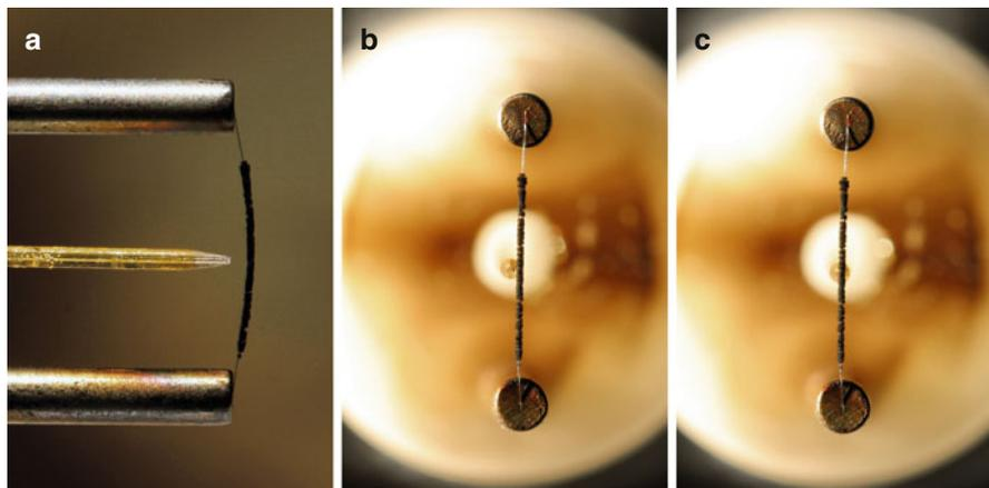
**Fig. 8.24** Alignment of the fused silica capillary on the emitter axis; the photographs are similar to what would be observed using a  $8\times$  magnifying glass. (a) Side view to show the distance between the tip of the capillary and the activated emitter, (b, c) on axis views. In (b) the capillary is left side off-axis while in (c) it is well aligned
