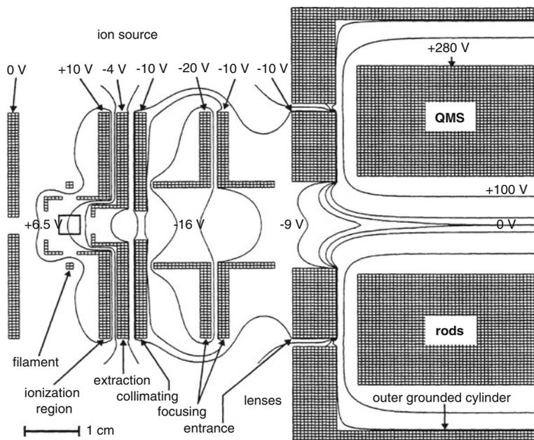
**Fig. 5.4** The EI ion source of a quadrupole mass spectrometer with equipotentials as calculated by the computer simulation program SIMION three-dimensional version 6.0 (Reproduced from Ref. [15] with permission. © Elsevier Science, 1998)
