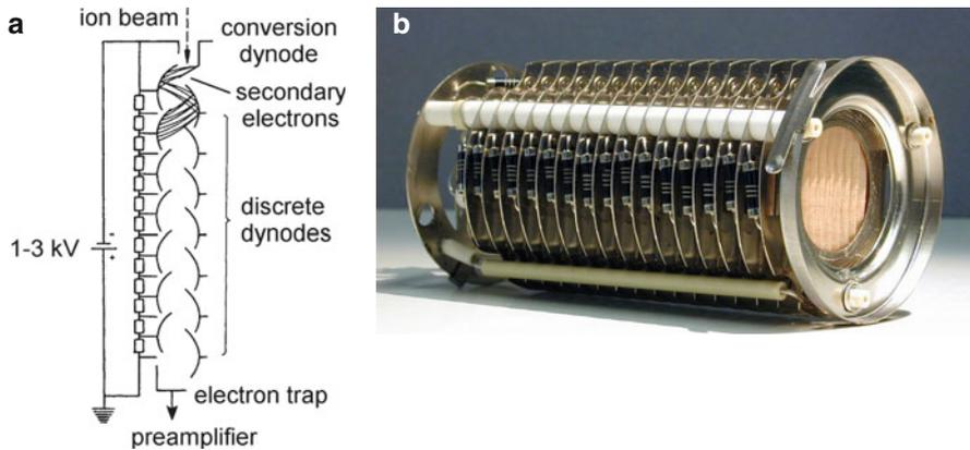
**Fig. 4.93** Discrete dynode electron multipliers. (a) Schematic of a 14-stage SEM. (b) An old-fashioned 16-stage Venetian blind-type SEM clearly showing the resistors and ceramics insulators between the stacking dynodes at its side ((a) Adapted from Ref. [292] by permission. © Springer-Verlag Heidelberg, 1991)
