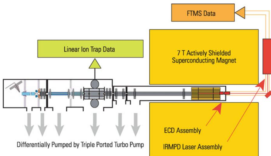
**Fig. 4.86** Schematic of a LIT-FT-ICR hybrid instrument, the Thermo Scientific LTQ FT Ultra, incorporating a fully functional LTQ front end (as in LTQ Orbitrap) for highest versatility (Courtesy Thermo Fisher Scientific, Bremen)
