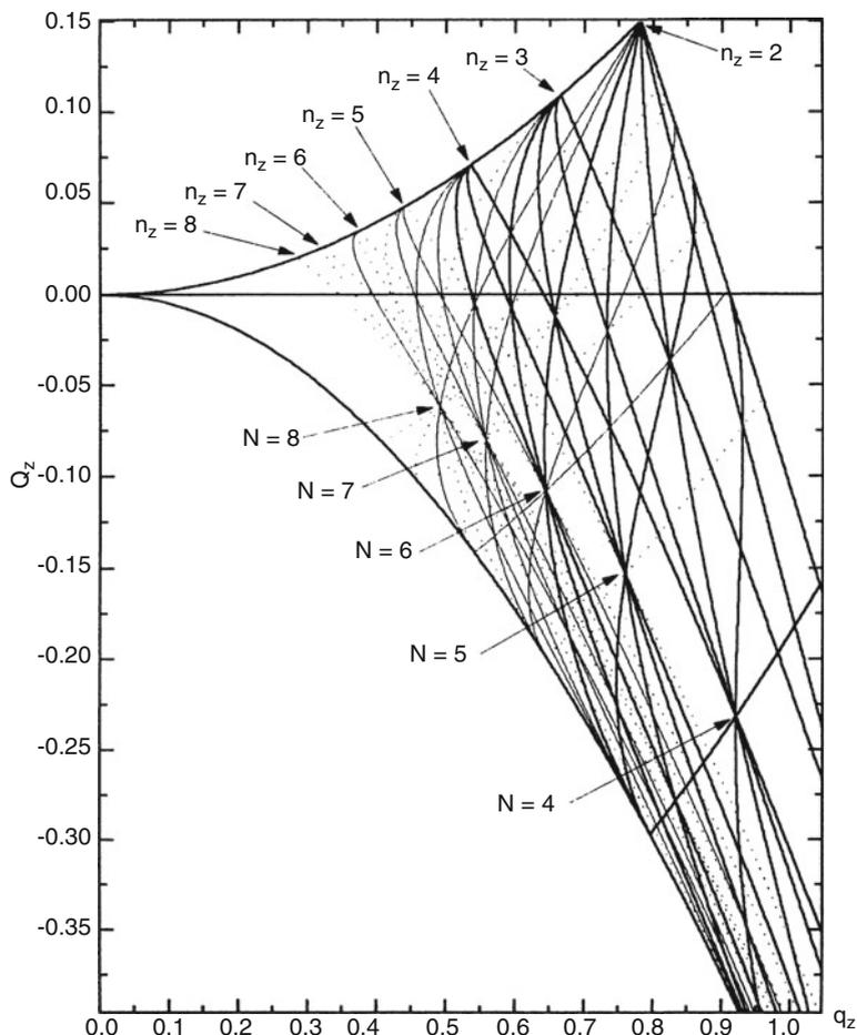
**Fig. 4.58** Plot of theoretical lines of instability corresponding to the relation  $n_r/2\beta_r + n_z/2\beta_z = 1$  for different orders  $N = n_r + n_z$  (strong resonances represented by *solid lines*, weak ones by *dotted lines*) (Reproduced from Ref. [154] by permission. © Elsevier Science, 1996)
