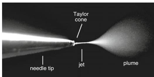
**Fig. 12.18** Electro spray from a nanoESI capillary. The jet emitted from the Taylor cone is clearly visible and separate from the region of rapid expansion into a plume of microdroplets (By courtesy of New Objective, Woburn, MA)
