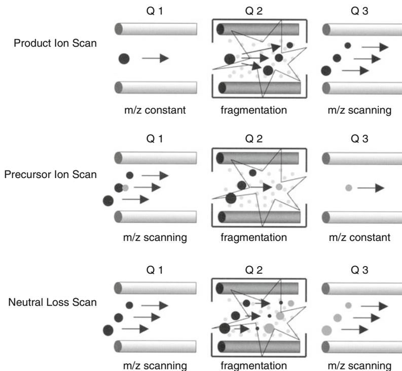
**Fig. 9.21** Scan modes of triple quadrupole mass spectrometers (Adapted from Ref. [101] with permission. © Springer-Verlag, 2004)
