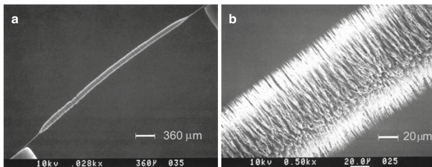
**Fig. 8.6** SEM pictures of activated tungsten wire emitters; (a) overview showing the thin tungsten wire close to the holders and the whisker-bearing middle section, (b) detail of the central part revealing whiskers (By courtesy of Carbotec, Bergisch Gladbach, Germany)
