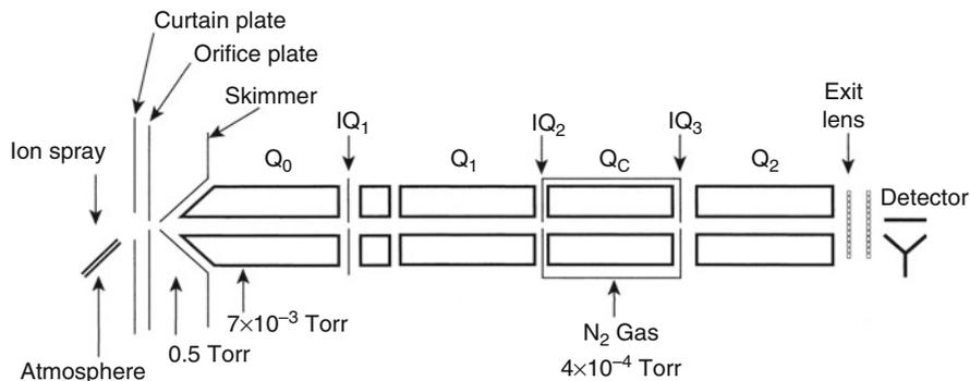
**Fig. 4.46** A quadrupole-LIT hybrid instrument. In this scheme, the RF-only collision quadrupole has been replaced by the LIT. The other option, replacement of Q2 by a LIT, is finally in commercial use (Adapted from Ref. [129] with permission. © John Wiley & Sons, Ltd., 2002)
