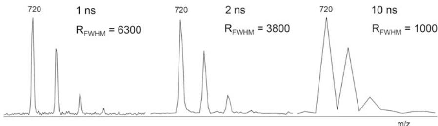
**Fig. 4.92** The [60]fullerene molecular ion peak depicted at different settings of the dwell time per data point of the analog-to-digital converter obtained on the aforementioned instrument after PIE upgrade. At 1 ns per data point (1 GHz) the peaks are well resolved and resolution is limited by the analyzer. At 2 ns (500 MHz) some broadening occurs. At 10 ns (100 MHz) peak shapes are reduced to triangles because detection provides just about two points per  $m/z$
