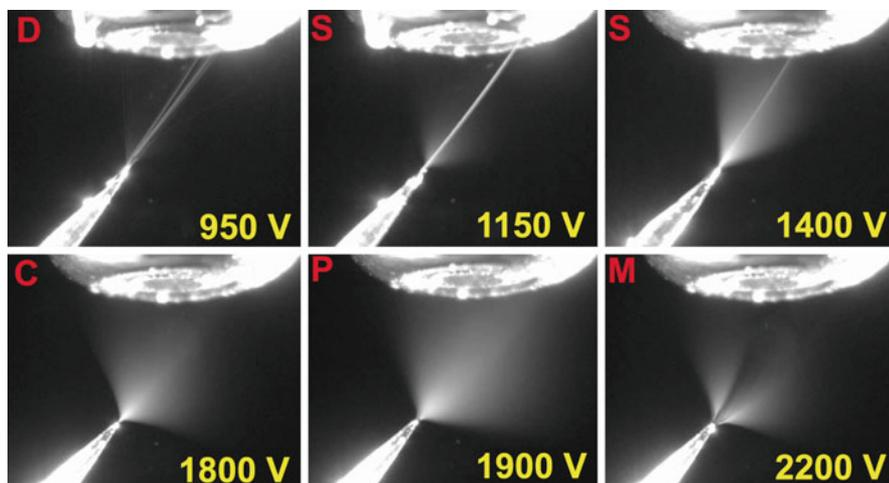
**Fig. 12.15** Photographs of nanoelectrospray plumes as effected by different spray voltages. The modes observed starting from the *upper left* are dripping (*D*), spindle (*S*), cone-jet (*C*), pulsed cone-jet (*P*), and multi-jet (*M*). Only pure cone-jet mode will deliver stable electrospray for analytical work (Reproduced from Ref. [88] with permission. © Elsevier, 2004)
