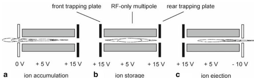
**Fig. 4.42** Operation of a linear RF multipole ion trap illustrated using typical DC voltage offsets for positive ions. (a) Ion accumulation with backside potential wall up, (b) storage of ions with both trapping potentials up, and (c) axial ejection of ions from trap using an attractive exit plate potential. The trapping RF multipole section is held at constant DC offset of +5 V in this example
