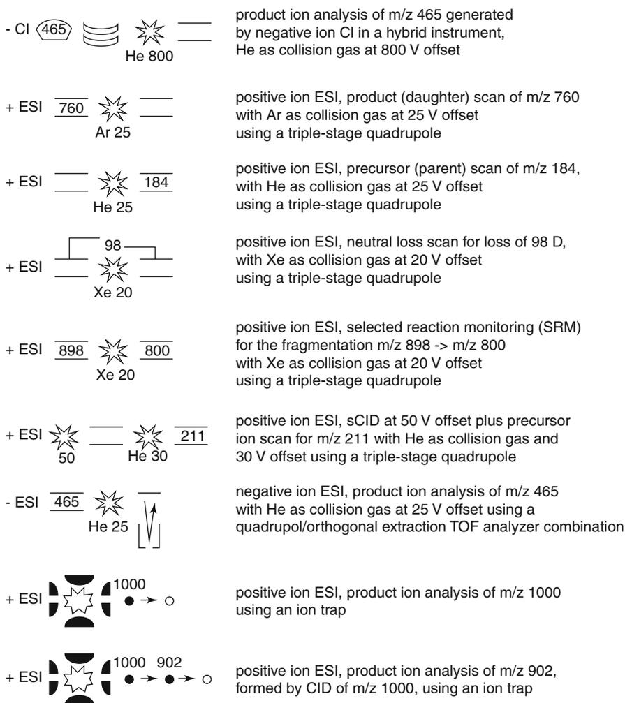
**Fig. 9.3** Pictograms for tandem MS (Reproduced from Ref. [12] with permission. © Elsevier Science Inc., 1997)
