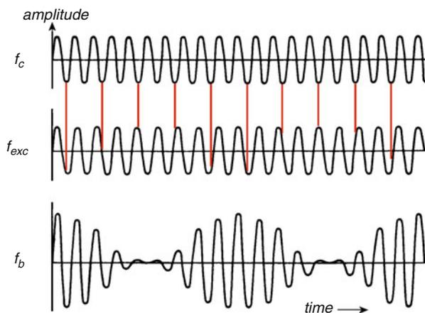
**Fig. 9.32** Generation of an oscillation of ion kinetic energy as defined by a beat frequency due to off-resonance excitation; vertical connections are to locate points of positive and negative interferences, respectively. The larger the amplitude of  $f_b$  the more kinetic energy is contained in the circulating ions. One SORI-CID experiment consists of hundreds of beats
