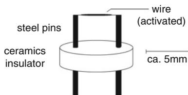
**Fig. 8.5** A wire emitter: high voltage is supplied via the emitter-holding pins. These also serve to pass a current for resistive heating through the (activated) wire
