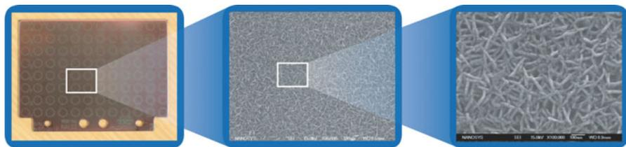
**Fig. 11.33** NALDI target plate. The figure shows the NALDI target plate (*left*) and increasing magnification SEM images (*center* and *right*) of the nanostructured coating that provides the active surface for desorption/ionization of deposited analytes (Courtesy of Bruker Daltonik GmbH, Bremen)
