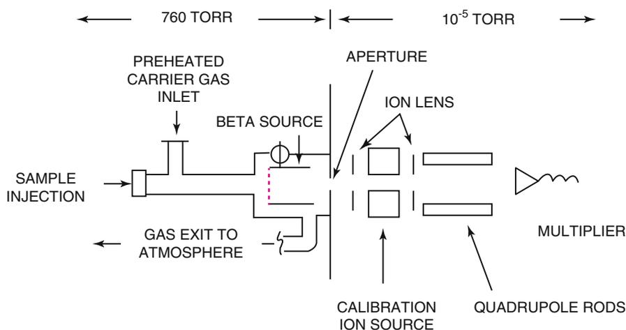
**Fig. 7.20** The original implementation of API. Here, primary electrons are delivered by a  $^{63}\text{Ni}$  foil. For API, the filament of the EI calibration source was switched off and only the electrostatic lenses were used to pass the ions into the quadrupole mass analyzer chosen for its tolerance to moderate vacuum conditions (Reproduced from Ref. [118] with permission. © The American Chemical Society, 1973)
