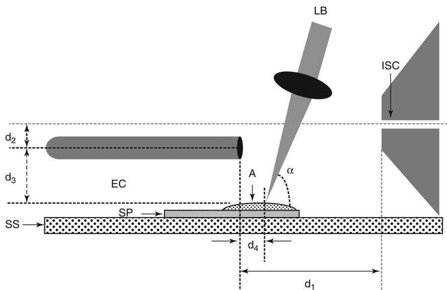
**Fig. 13.16** ELDI setup. *A* analyte, *SP*: stainless steel sample support plate, *SS* mobile sample stage, *EC* electro spray capillary, *LB* UV laser beam, *ISC* ion sampling capillary of the API interface. The distances  $d_1$  through  $d_4$  are all in the order of millimeters (Reproduced from Ref. [55] with permission. © John Wiley & Sons, Ltd., 2005)
