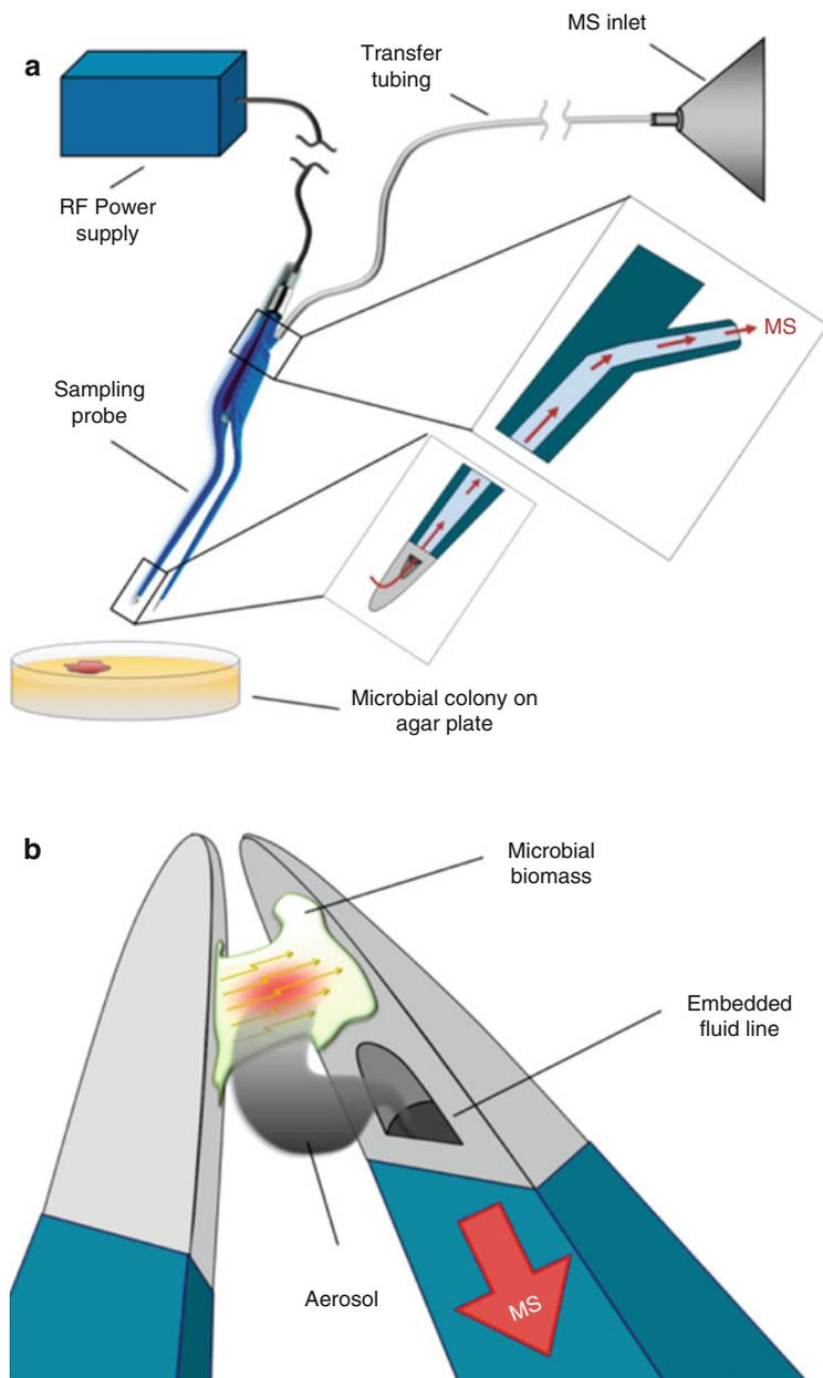
**Fig. 13.19** (a) Setup used for analysis of bacteria by REIMS. (b) Scheme of analysis. Microbial biomass is held between the two electrodes of the irrigated bipolar forceps, electrical current is applied, sample is evaporated thermally, and the produced aerosol is aspirated into the opening of the embedded fluid line (Reproduced from Ref. [67] with permission. © American Chemical Society, 2014)
