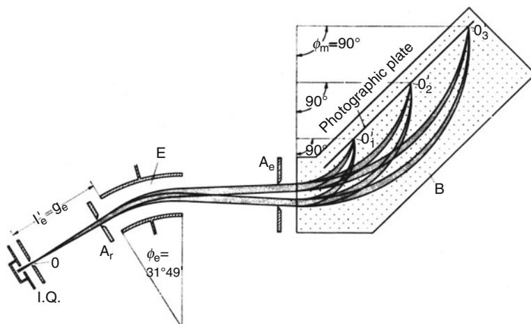
**Fig. 4.23** Mattauch-Herzog double-focusing mass spectrograph providing direction and momentum focusing of ions on a plane [89]. The ESA precedes the magnet. Placing a photographic plate in the image plane allows simultaneous recording of a  $m/z$  range (Reproduced from Ref. [91] with kind permission of Curt Brunnée)
