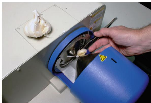
**Fig. 13.31** Commercial DART source of the first generation on a JEOL AccuTOF instrument. Here it is used for the analysis of volatiles from a garlic clove [125, 126]. The sample is simply held into the open gap between the metastable atom source (*lower right part*) and the orifice of the API interface (*upper left*). Photograph by courtesy of JEOL USA
