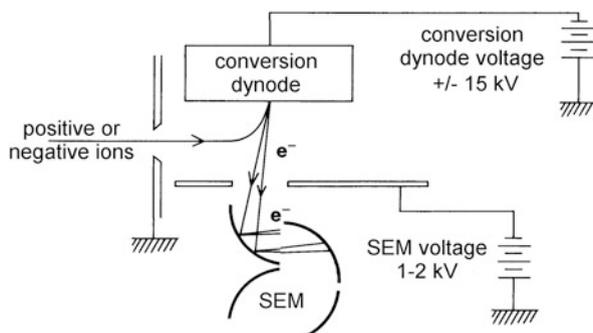
**Fig. 4.98** Detector configuration with conversion dynode (By courtesy of JEOL, Tokyo)
