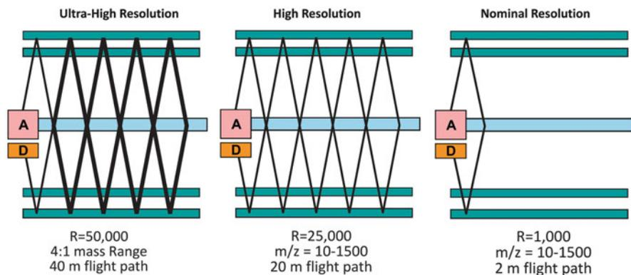
**Fig. 4.17** Scheme of multi-reflecting TOF operational modes (A ion source, D detector). By using a switchable deflector ions can either be passed through one double reflection to deliver  $R = 1000$ , to five double reflection to achieve  $R = 25,000$ , or even to have a second full passage enabling  $R = 50,000$  (Courtesy of LECO, Germany)
