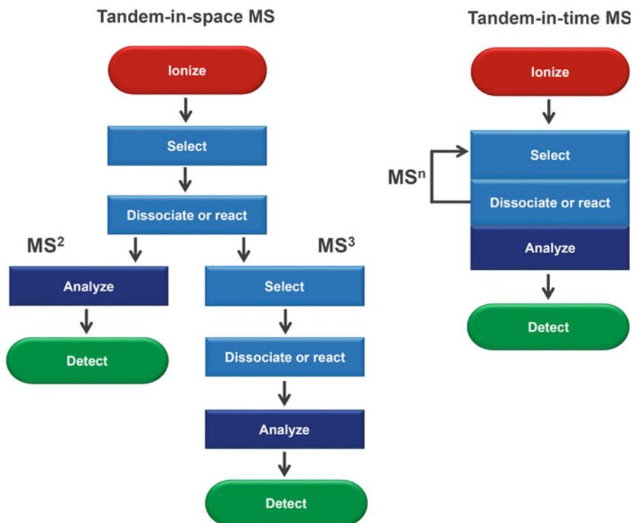
**Fig. 9.1** Comparison of tandem-in-space and tandem-in-time MS. Obviously, higher order MS<sup>n</sup> can be better realized by tandem-in-time setups, whereas tandem-in-space instrumentation is usually designed for MS<sup>2</sup> with MS<sup>3</sup> representing already the rare exception
