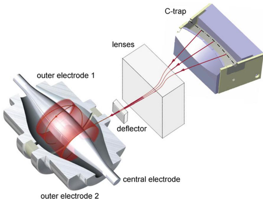
**Fig. 4.82** The Orbitrap mass analyzer with ions being injected from the C-trap through lenses and a deflector. During injection, the C-trap acts as a convex lens with the outer rods pushing and the inner short rods pulling the ions by a DC pulse. Trapping voltage is applied to the central electrode (Courtesy of A. Makarov, Thermo Fisher Scientific)
