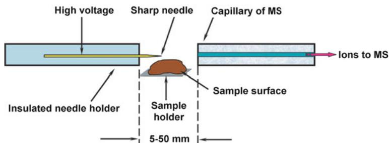
**Fig. 13.10** Schematic of a DAPCI source for operation with moist ambient air as reagent gas. The sharp needle discharge electrode is coaxially centered in a capillary of 3 mm i.d. delivering humidified nitrogen gas if the ambient air is below 20% relative humidity (Adapted from Ref. [33] with permission. © John Wiley & Sons, Ltd., 2007)
