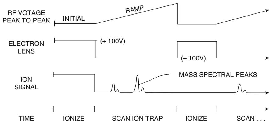
**Fig. 4.56** Timing sequence used for mass-selective instability mode (about 1.5 cycles shown). With an external ion source the ionization time is replaced by the ion injection pulse (Reproduced from Ref. [155] by permission. © Elsevier Science, 1984)
