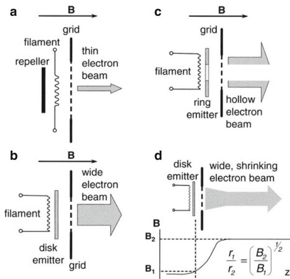
**Fig. 9.41** Electron injection systems for ECD-FT-ICR instruments: (a) directly heated filament in homogeneous magnetic field, (b) disk-shaped indirectly heated cathode in homogeneous magnetic field, (c) ring-shaped indirectly heated cathode, and (d) cathode in fringing magnetic field region with beam collimation (Reproduced from Ref. [158] with permission. © John Wiley & Sons, Ltd., 2004)
