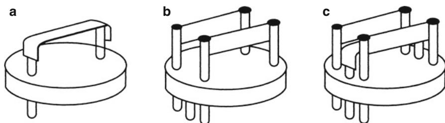
**Fig. 15.4** From left (a) single filament, (b) double filament, and (c) triple filament assemblies for thermal ionization of metal salts and oxides (Reproduced from Ref. [3] with permission. © John Wiley & Sons Ltd., 1997)
