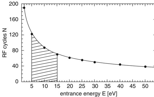
**Fig. 4.36** Relation of RF cycles experienced by the ions as a function of entrance energy. The shaded area marks the region of optimized performance (Reproduced from Ref. [109] with permission. © Elsevier Science, 1998)
