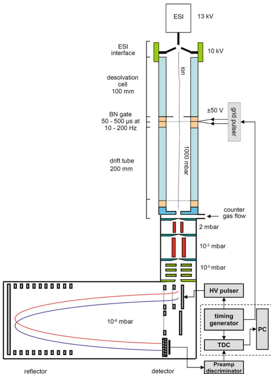
**Fig. 4.87** Basic design of an ambient-pressure IMS-TOF mass spectrometer. Ions from an electrospray source are entering a desolvation chamber from where packets are pulsed into the ion mobility tube by means of a Bradbury-Nielsen (BN) ion gate. The ion path is shown uneven to indicate diffusion of ions. After ion mobility separation the ions are transferred into the reflector via a differentially pumped interface (Courtesy of ToFwerk AG, Thun, Switzerland)
