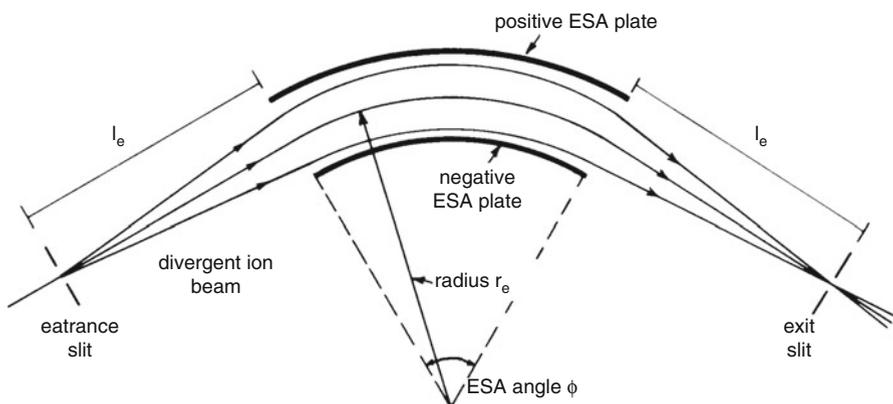
**Fig. 4.22** Direction focusing of a radial electric field. Ions of appropriate kinetic energy are focused at the exit slit. Divergent ions pass the ESA close to either plate. Here, the electric potentials are set to transmit positive ions. The image distance  $l_e$  depends on the ESA angle
