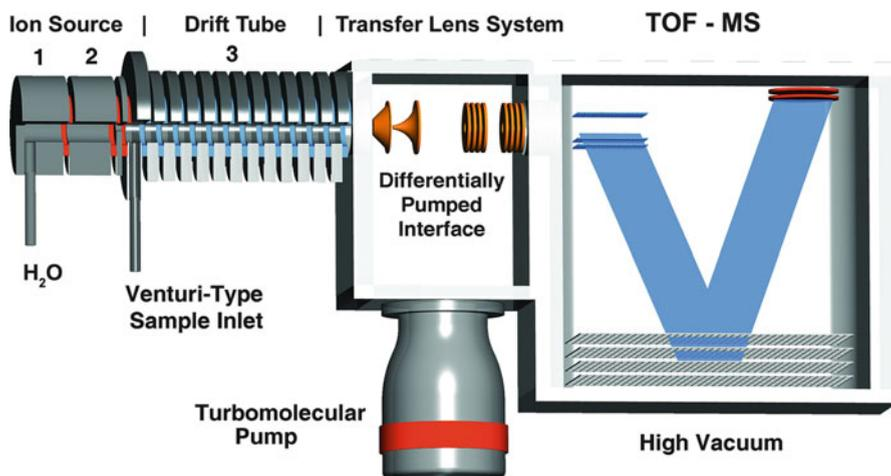
**Fig. 7.9** PTR mass spectrometer. The ion source of the Ionicon PTR-TOF 2000™ is divided into a compartment for reagent ion generation from H<sub>2</sub>O by (1) a hollow cathode and (2) a source drift region in front of the sample inlet, and (3) the drift tube for analyte ion formation. The TOF analyzer has its own turbomolecular pump to maintain high vacuum (*not shown*) (By courtesy of Ionicon Analytik GmbH, Innsbruck, Austria)
