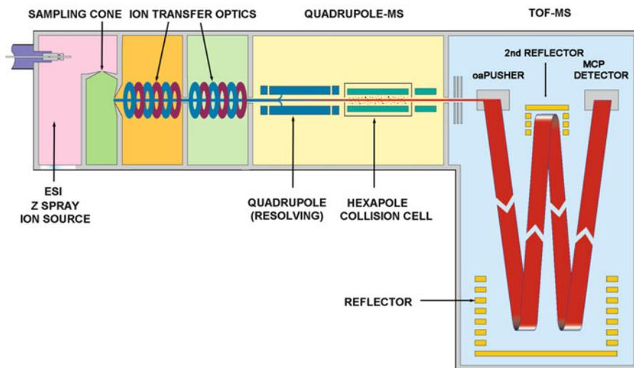
**Fig. 4.84** The Q-TOF Ultima, Qh-oaTOF design, with ESI ion source in MS/MS mode. The TOF analyzer has a reflector that can either be operated using the large reflector alone (V-mode) or adding a second stage of ion reflection (W-mode) for higher resolving power (Courtesy of Waters Corporation, MS Technologies, Manchester, UK)
