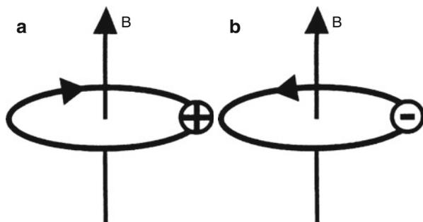
**Fig. 4.63** Circular motion of ions in a magnetic field. Viewing along the direction of the magnetic field one observes (a) a counterclockwise motion for positive ions and (b) a clockwise motion for negative ions (Adapted from Ref. [219] with permission. © Elsevier Science Publishers, 2002)
