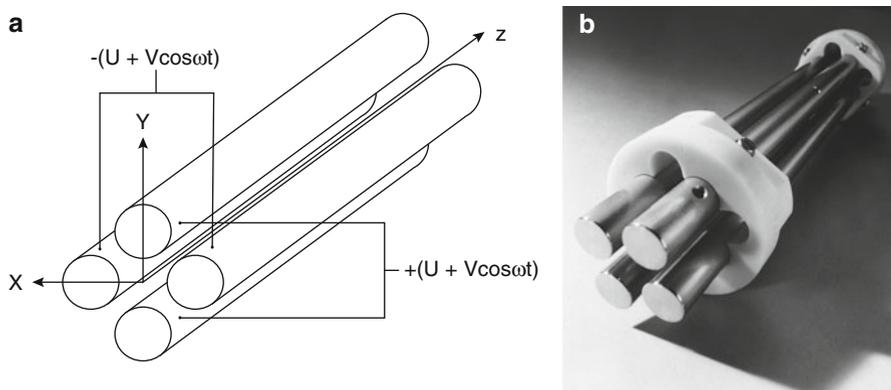
**Fig. 4.31** Linear quadrupole mass analyzer: schematic (a) and photograph (b) (By courtesy of (a) JEOL, Tokyo and (b) Waters Corp., MS Technologies, Manchester, UK)
