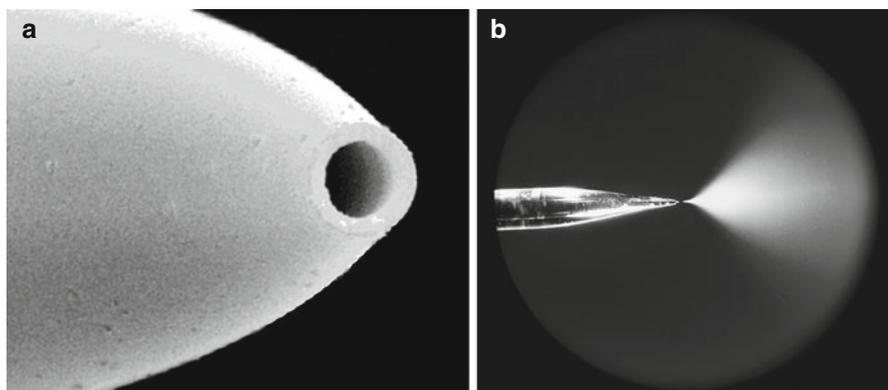
**Fig. 12.14** Nanoelectrospray; (a) SEM micrograph of the open end of a glass nanoESI capillary having a 2- $\mu\text{m}$  aperture, (b) microscopic view of the spray from a nanoESI capillary as provided by observations optics (By courtesy of New Objective, Woburn, MA)
