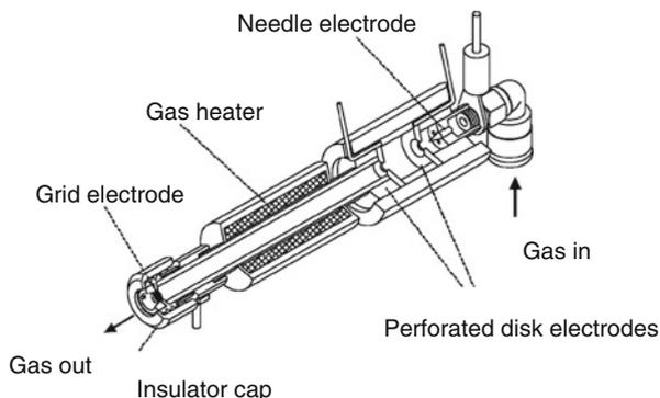
**Fig. 13.25** Cutaway view of the DART source. The emanating gas effects ionization of sample independent of its state of aggregation (Reproduced from Ref. [3] with permission. © The American Chemical Society, 2005)
