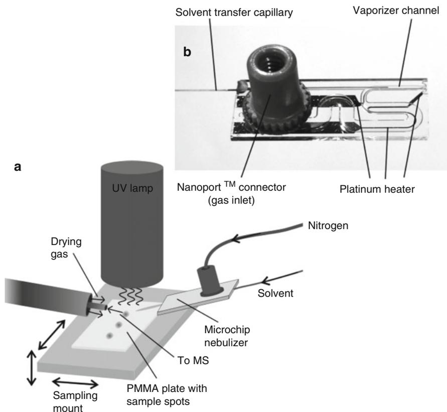
**Fig. 13.12** Schematic of (a) the DAPPI setup and (b) photograph of the microchip nebulizer. The small solvent flow is mixed with nitrogen gas and vaporized in the microchip nebulizer by resistive heating of the platinum wire. The krypton UV lamp irradiates the sample surface that is in contact with the hot reagent gas (Reproduced from Ref. [16] with permission. © The American Chemical Society, 2007)
