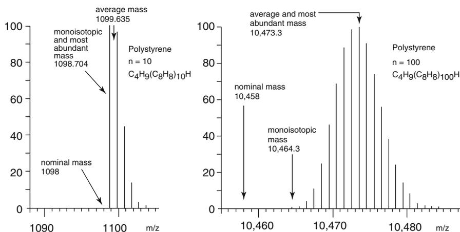
**Fig. 3.41** Polystyrene. Calculated isotopic patterns of large ions (Adapted from Ref. [67] with permission. © American Chemical Society, 1983)
