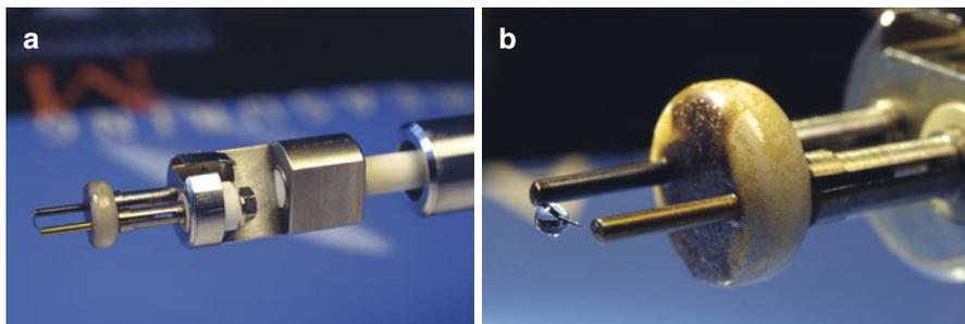
**Fig. 8.8** FD probe. (a) Emitter holder of a JEOL FD probe tip, (b) a drop formed of 1–2  $\mu\text{l}$  of analyte solution placed onto the activated emitter by means of a microliter syringe
