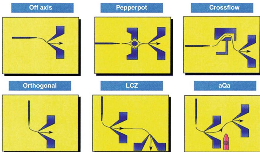
**Fig. 12.6** Some strategies used in commercial API ion sources to increase solvent compatibility and system robustness. Some of these designs are (were) commercial brands: Peppercot, Crossflow, and LCZ (“z-spray”, Micromass); AQA (Thermo Finnigan) (Reproduced from Ref. [66] by permission. © John Wiley & Sons, 1999)
