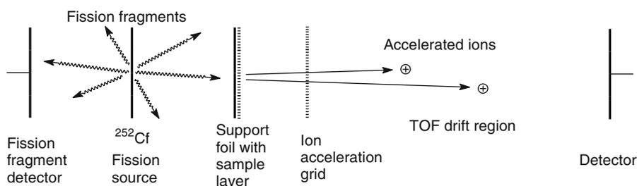
**Fig. 10.21** Schematic of a <sup>252</sup>Cf-plasma desorption TOF instrument [143]
