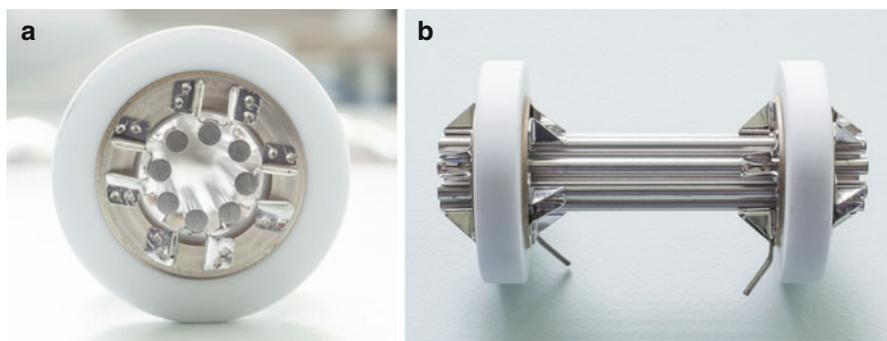
**Fig. 4.40** RF octopole ion guide used to bridge a differential pumping stage of an ESI interface in a Finnigan LCQ instrument. (a) Head-on view to show the octopole alignment and (b) side view. Each of the two pins pointing down is connected to supply the RF voltage to four of the rods in alternation. The round rods are ca. 3 mm in diameter and the length of this device is about 7 cm
