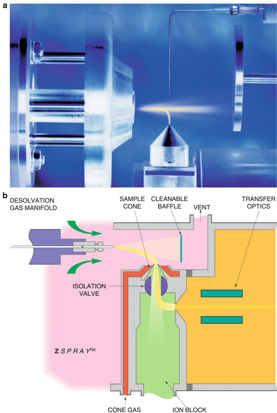
**Fig. 12.7** Micromass z-spray interface. (a) Photograph of the actual spray from which charged constituents are extracted downwards into the entrance orifice. While large droplets and neutrals are traveling on a straight path toward the counter electrode, small highly charged droplets are attracted by the entrance at the cone-shaped electrode. (b) Schematic including the inner parts of the interface (By courtesy of Waters Corporation, MS Technologies, Manchester, UK)
