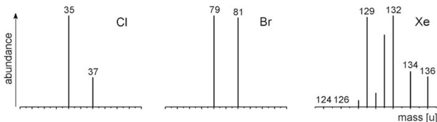
**Fig. 3.2** Isotopic patterns of chlorine, bromine, and xenon. The bar graph representations of the isotopic distributions have the same optical appearance as mass spectra. You should compare these graphical representations to the compositions listed in Table 3.1. Afterwards, you may decide for yourself which type you would consider to be easier to perceive and to compare
