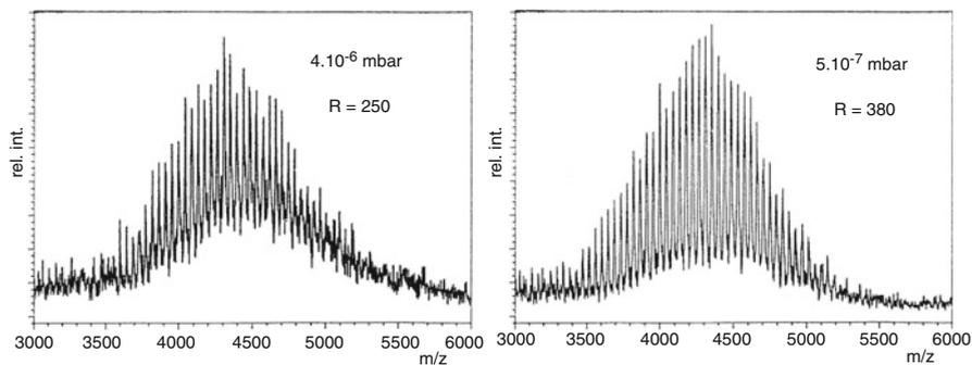
**Fig. 4.6** Dependence of resolution on analyzer pressure: linear MALDI-TOF spectra of polyethylene glycol 4000 recorded at a pressure of  $4 \times 10^{-4}$  Pa (*left*) and  $5 \times 10^{-5}$  Pa (*right*) (Adapted from Ref. [45] with permission. © John Wiley & Sons, 1994)
