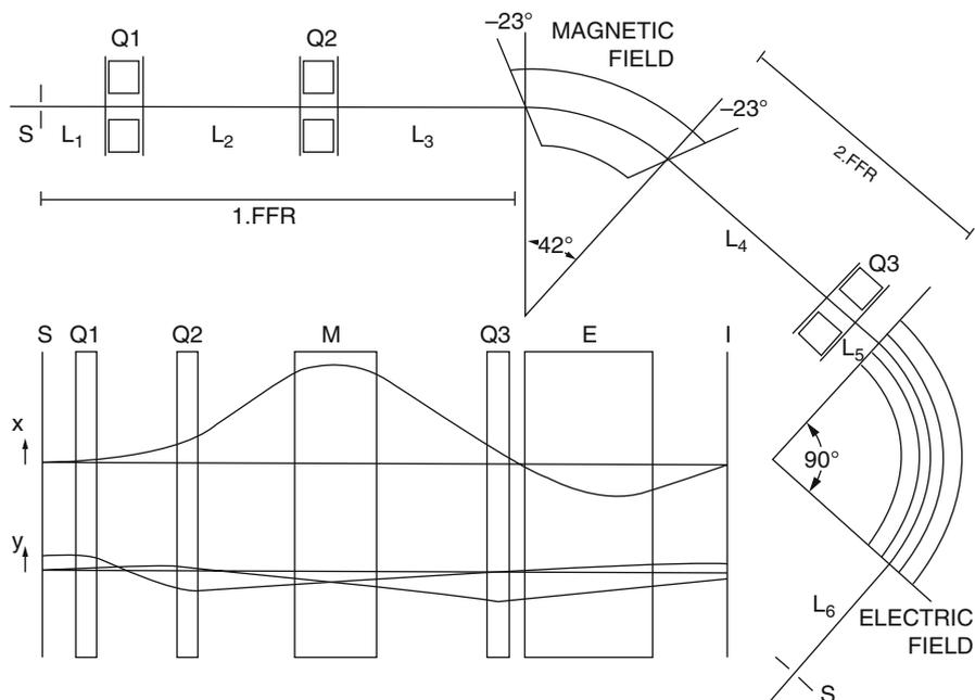
**Fig. 4.29** Layout of the JEOL JMS-700. Three DC quadrupole lenses are used to improve the transmission of the magnetic sector. The inset shows horizontal ( $x$ ) and vertical ( $y$ ) trajectories where the height of the beam ( $y$ ) is clearly reduced to pass through a narrow gap between the pole shoes of the magnet (Adapted from Ref. [99] with permission. © Elsevier Science, 1985)
