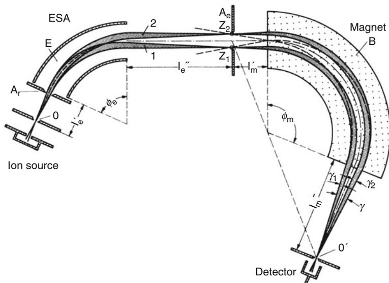
**Fig. 4.24** Double-focusing mass spectrometer of EB geometry, basically a Nier-Johnson type instrument. Direction and velocity focusing are shown exaggerated. After exiting the ESA, the energy-resolved beam passes through a wide intermediate slit into the magnetic sector. The large aperture ensures good overall transmission (Reproduced from Ref. [91] with kind permission of Curt Brunnée)
