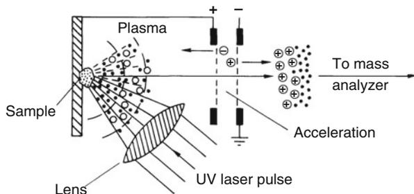
**Fig. 11.2** Simplistic laser desorption ion source for nonresonant light absorption by a solid; in practice, the solid is supplied as a thin microcrystalline layer. Here, positive ions are continuously being extracted as long as the supply is sustained by the laser desorption plasma (Reproduced from Ref. [28] by permission. © Elsevier Science, 1994)
