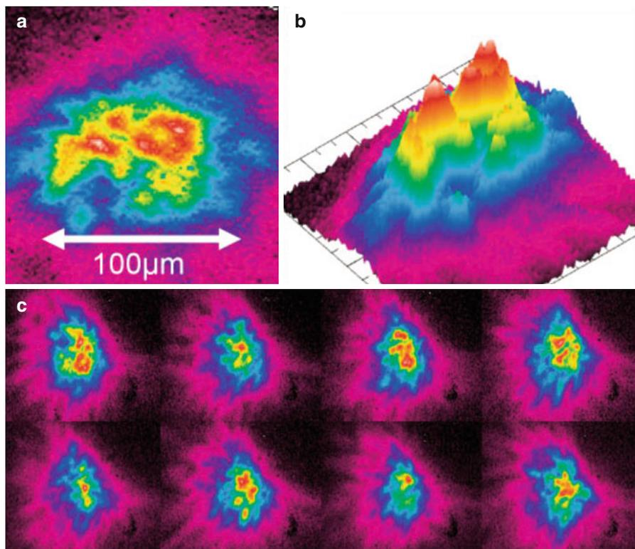
**Fig. 11.5** Typical profile of a nitrogen laser. (a) View from top, (b) 3D view from the side, (c) beam profile of eight consecutive laser shots, demonstrating the shot-to-shot variation in the profile of the nitrogen laser. Different colors represent different intensities (Reproduced from Ref. [55] with permission. © Wiley, 2006)
