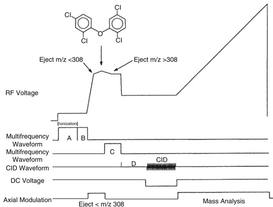
**Fig. 4.57** Complex scan function used for a tandem mass spectrometric study of 2,4,3',6'-tetrachlorodiphenylether (Reproduced from Ref. [168] by permission. © John Wiley and Sons, 1997)
