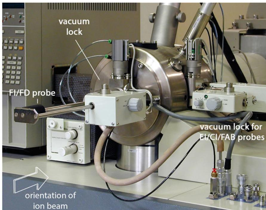
**Fig. 8.4** FD probe inserted into the vacuum lock. FD probes are generally inserted in axial position to free the vacuum lock of the DIP for FI use. The emitter wire is now oriented vertically to comply with the beam geometry of the magnetic sector analyzer
