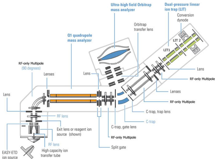
**Fig. 4.85** The Orbitrap Fusion Lumos tribrid mass spectrometer. The first RF-only multipole is bent by  $90^\circ$  to get rid of neutrals before ions are entering the analyzer section comprising quadrupole (orange), Orbitrap (blue), and LIT/LIT (green) (Adapted from Thermo Fisher technical documentation with kind permission. © Thermo Fisher Scientific, Bremen, 2015)
