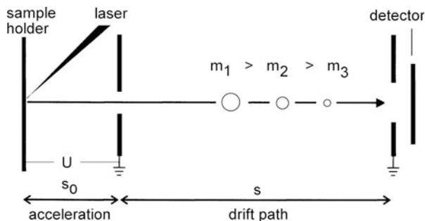
**Fig. 4.5** Scheme of a linear TOF instrument designed for use in combination with a laser desorption ion source. Once created during a laser pulse onto the sample layer, ions are continuously accelerated by a voltage  $U$ . While drifting along the field-free drift path  $s$ , they are dispersed in time. Lighter ions reach the detector first
