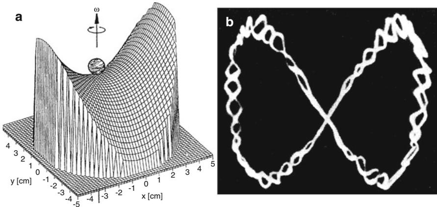
**Fig. 4.55** Visualization of ion motion in the ion trap. (a) Mechanical analog of the QIT. (b) Photograph of ion trajectories of charged aluminum particles in a quadrupole ion trap ((a) Reproduced from Ref. [102] with permission. © World Scientific Publishing, 1993. (b) Reproduced from Ref. [158] with permission. © American Institute of Physics, 1959)
