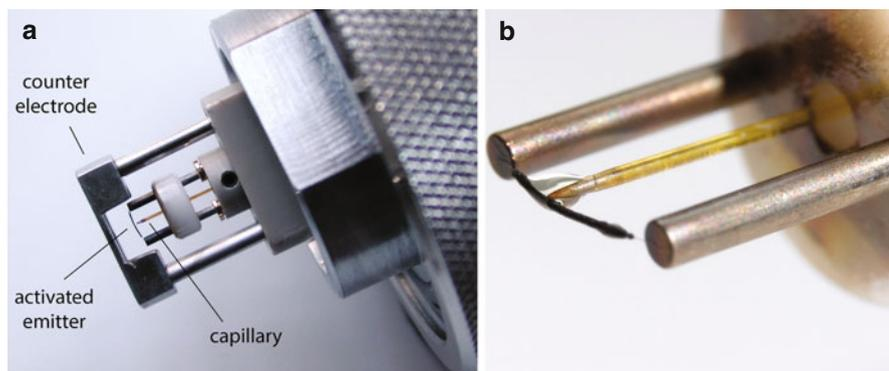
**Fig. 8.23** (a) LIFDI probe tip with the fused silica capillary that delivers the sample to the “backside” of the activated emitter; here, the counter electrode is part of the probe, and (b) wetting of the emitter with solvent spreading out over the activated zone. The 13- $\mu\text{m}$  tungsten wire connecting this section to the posts is barely visible (By courtesy of Linden CMS, Leeste, Germany)
