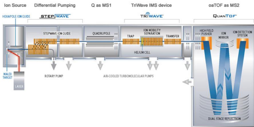
**Fig. 4.91** The Waters Synapt G2-Si, a Q-IMS-*oaTOF* hybrid, here shown with MALDI source. The combination of three ring ion guide sections is used to build a complete IMS device comprising a trap at the entrance to supply ion packages, the IMS itself, and an ion guide for transfer to the mass analyzer (cf. *TriWave* in Fig. 4.89) (Adapted with permission. Courtesy of Waters MS Technologies)
