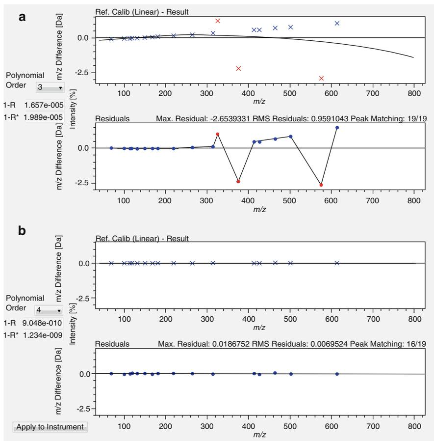
**Fig. 3.31** Calibrations based on PFTBA. (a) 3rd-order polynomial calibration yields a gently bent curve. Three outliers (*red*) were identified and deleted. (b) Repetition of calibration using the corrected set of peaks and a 4th-order polynomial. Upon these measures, the correlation coefficients improve from the order of  $10^{-5}$  to  $10^{-9}$ . Figure composed of screenshots of JEOL AccuTOF GCx calibration software
