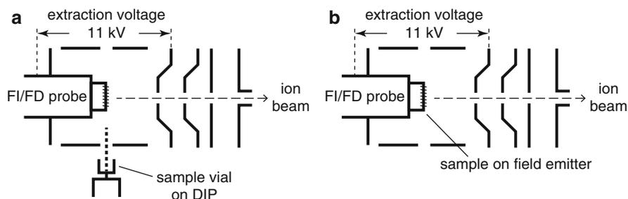
**Fig. 8.3** Schematic of an FI/FD ion source (a) in FI mode, (b) in FD mode. The distance between emitter and counter electrode is exaggerated for clarity (Adapted from Ref. [41] by permission. © Springer-Verlag, Heidelberg, 1991)
