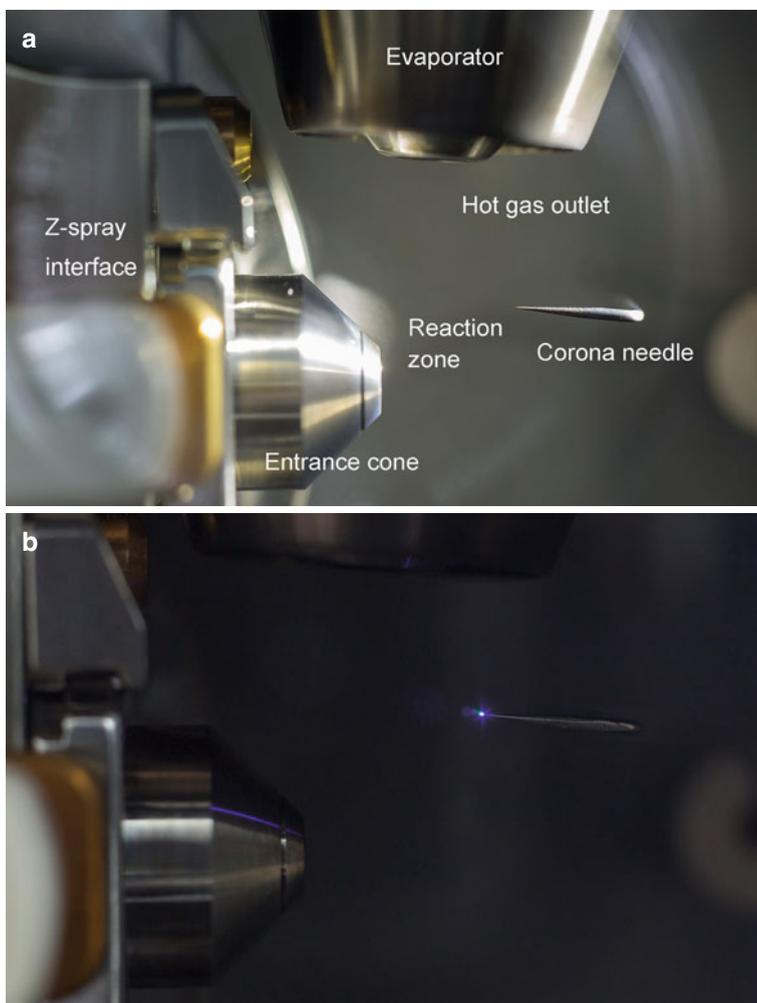
**Fig. 7.22** APCI source of a Waters SQD2 instrument attached to a Z-spray interface. (a) APCI source as seen in daylight, (b) shaded source in operation. The blueish corona discharge corresponding to about  $10\ \mu\text{A}$  discharge current at the tip of the needle is only visible in virtual darkness
