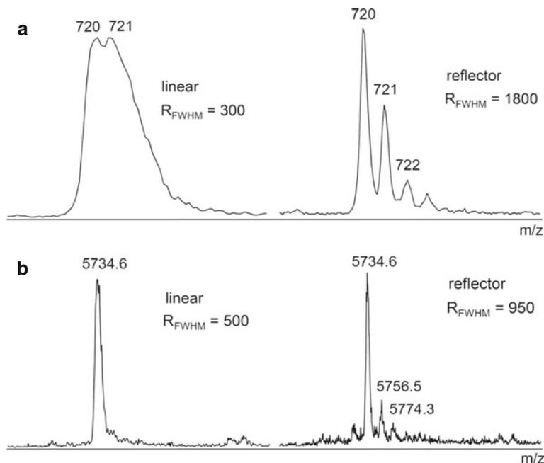
**Fig. 4.9**  $C_{60}$  molecular ion signal of at  $m/z$  720 (a) and the  $[M + H]^+$  ion signal of bovine insulin,  $m/z$  5734.6 (b), as obtained on a TOF instrument in linear mode (left) and reflector mode (right). All other experimental parameters remained unchanged
