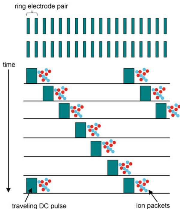
**Fig. 4.89** Effect of a traveling wave DC pulse along a stacked ring ion guide. Ions in front of the DC pulse are moving along from stack to stack and are thus propelled through the device (T-wave ion guide). A buffer gas is required to narrow down the thermal energy distribution (Reproduced from Ref. [281] with permission. © Elsevier Science Publishers, 2007)
