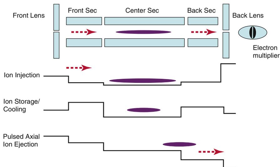
**Fig. 4.45** Sequence of DC voltages applied of the lenses and sections of a segmented linear ion trap to achieve mass-selective isolation and axial pulse-out of trapped ions from the mass analyzer. The reasons for segmenting of the LIT are explained in Sect. 4.5.3 and Fig. 4.49 (Reproduced from Ref. [140] with permission. © American Chemical Society, 2004)
