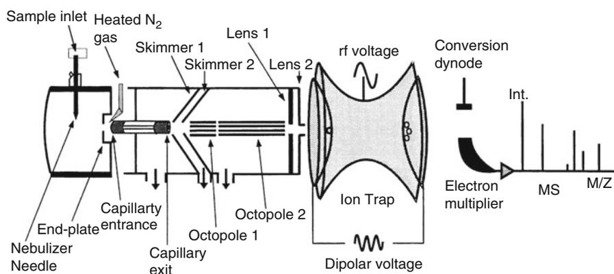
**Fig. 4.61** Layout of a quadrupole ion trap instrument equipped with an external ESI ion source. The analogy to the ESI-LIT configuration shown in Fig. 4.50 is striking (Reproduced from Ref. [193] by permission. © John Wiley & Sons, 2000)
