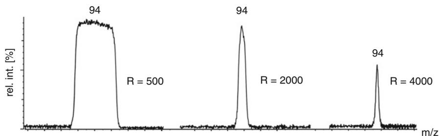
**Fig. 4.26** The influence of relative slit width settings on peak shape and resolution on a magnetic sector instrument. The peak shape first changes from flat-topped (*left*) to Gaussian (*center*) and finally resolution improves at cost of peak height (*right*)
