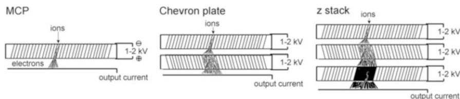
**Fig. 4.97** Stacking of MCPs to increase gain. *From left:* single MCP, Chevron plate, and z-stack configuration. Note the loss of spatial resolution upon stacking
