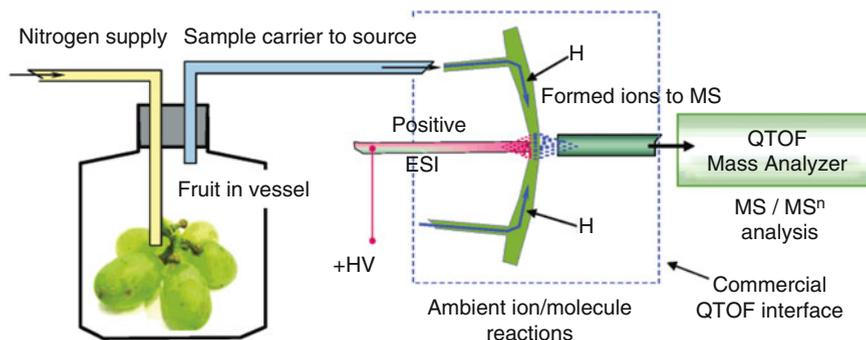
**Fig. 13.15** Schematic of an EESI source where the sample carrier gas is fed into the curtain gas of the API interface. Here, the experiment is designed to determine the ripening of fruit from its headspace, i.e., odor (Adapted from Ref. [50] with permission. © The American Chemical Society, 2007)
