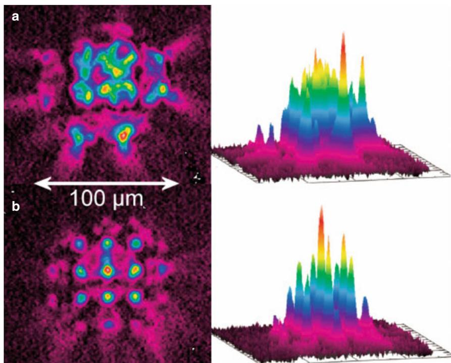
**Fig. 11.6** Beam profiles of two differently structured beams of an Nd:YAG laser as employed in Bruker's Smartbeam lasers, (a) structured with FWHM of a Gaussian fit of the envelope of 60  $\mu\text{m}$  and (b) with fit of 45  $\mu\text{m}$ . The overlapping local maxima and the pattern are clearly visible (Reproduced from Ref. [55] with permission. © Wiley, 2006)
