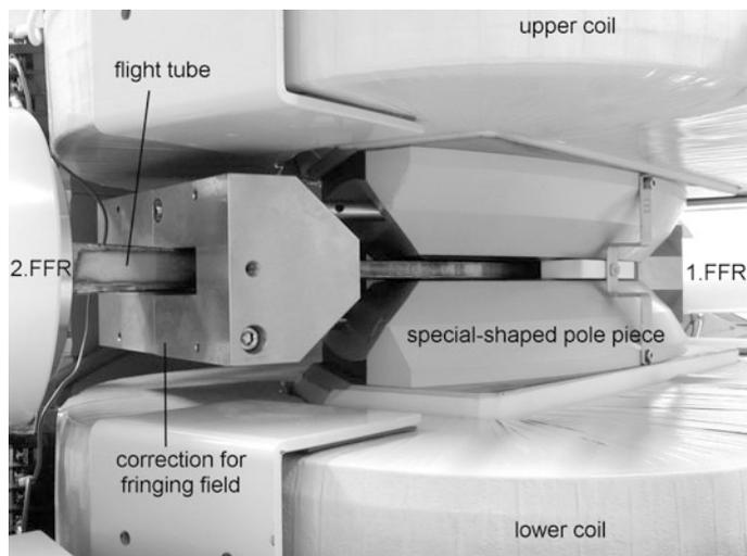
**Fig. 4.28** Flight tube passing through the gap of the magnetic sector of a JEOL JMS-700 instrument seen from the ESA side. The shapes of the pole pieces of the yoke and the additional blocks around the tube are designed to minimize fringing fields. In addition the pole faces are rotated to increase the mass range
