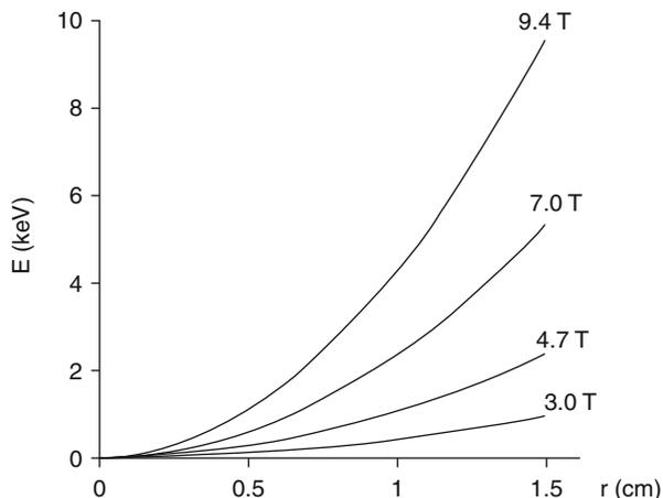
**Fig. 4.65** Kinetic energy of  $m/z$  100 ions in an ICR cell vs. orbital radius at magnetic field strengths from 3.0 to 9.4 T (Adapted from Ref. [220] with permission. © John Wiley and Sons, Inc., 1998)
