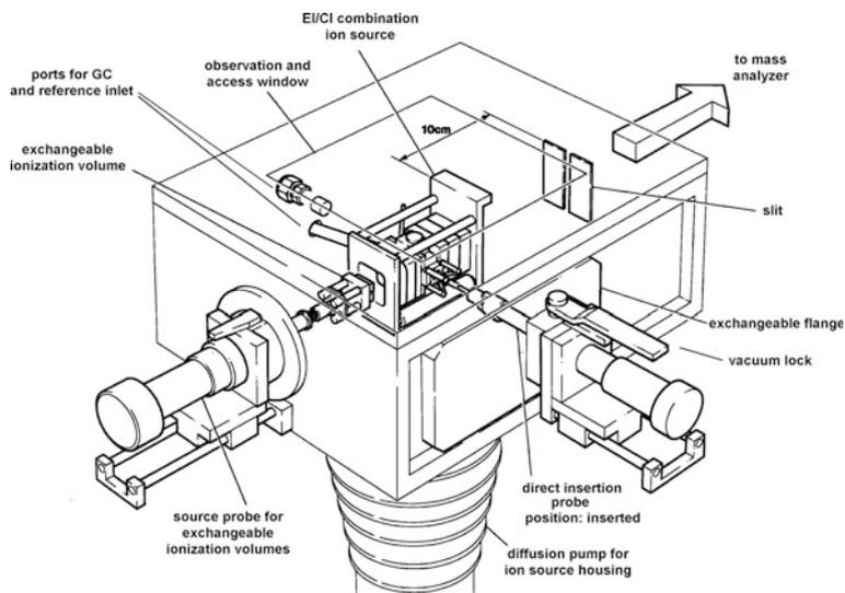
**Fig. 5.8** Ion source housing of a Waters Micromass Autospec™ magnetic sector instrument. The ion source can be accessed from several directions to allow for simultaneous connection to DIP/DEP, GC and reference inlet system (By courtesy of Waters Corporation, MS Technologies, Manchester, UK)
