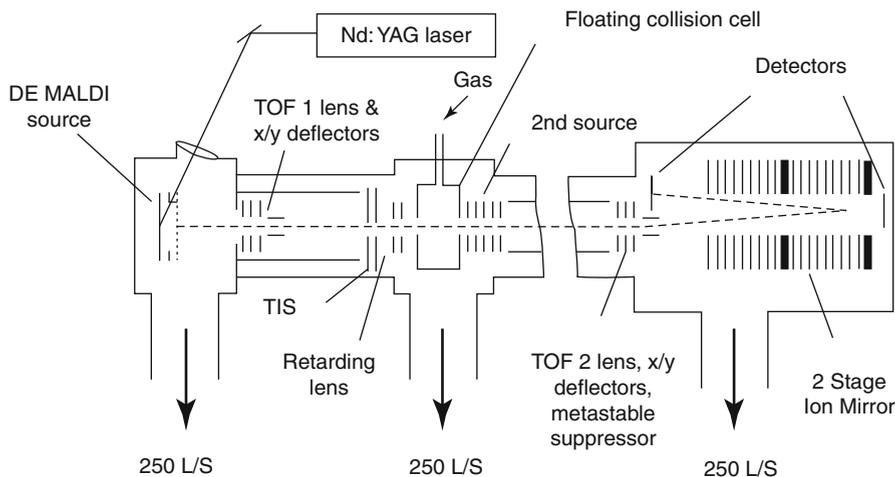
**Fig. 9.15** Tandem TOF analyzer with linear TOF1 and ReTOF2. The ions from TOF1 are  $m/z$ -selected by a timed ion selector, decelerated, fragmented by CID, accelerated, and then passed into ReTOF2 (Reproduced from Ref. [54] with permission. © Elsevier Science, 2002)
