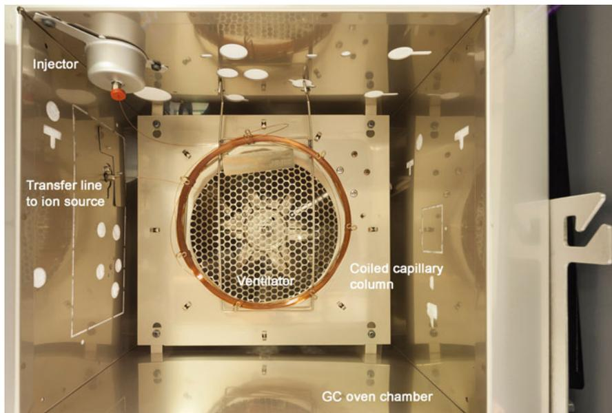
**Fig. 14.4** GC oven for capillary gas chromatography with open front door. The GC column wound onto a coil is suspended to hang freely in the heated air. In this Agilent 7890B GC, the injector is on the *top left side* and the exit of the capillary to the transfer line is in the *middle of the left side lining*
