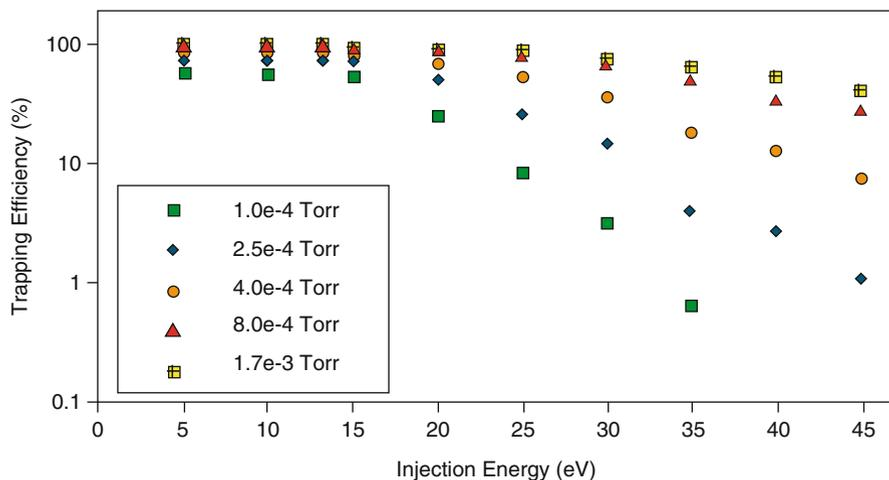
**Fig. 4.44** Dependence of the trapping efficiency of an LIT on ion injection energy (reserpine  $[M + H]^+$  ions,  $m/z$  609) for varying LIT pressures (from the top  $1.3 \times 10^{-4}$  mbar,  $3.3 \times 10^{-4}$  mbar,  $5.3 \times 10^{-4}$  mbar,  $1.1 \times 10^{-3}$  mbar,  $2.3 \times 10^{-3}$  mbar) (Adapted from Ref. [129] with permission. © John Wiley & Sons, Ltd., 2002)
