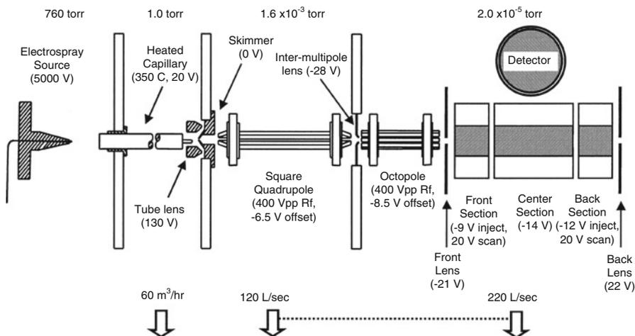
**Fig. 4.50** Radial ejection LIT mass spectrometer with ESI source, more precisely the Thermo Fisher LTQ as of 2002. A square RF quadrupole is used to bridge the second pumping stage while an RF octopole like the one shown in Fig. 4.40 is used in the third pumping state. Typical operating voltages and pressures are given (Reprinted with permission from Ref. [130]. © Elsevier Science Publishers, 2002)
