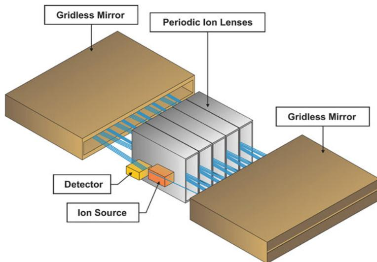
**Fig. 4.18** Schematic of the multi-reflecting TOF analyzer. During the most part of their journey, ions are traveling either within reflectors or are passing electrostatic lenses (Courtesy of LECO, Germany)
