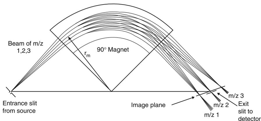
**Fig. 4.21** Ion separation and direction focusing in a plane by a  $90^\circ$  magnetic sector. A divergent beam of ions of  $m/z$  1, 2, 3 is separated into three beams and focused to a point on the image plane (divergence shown exaggerated). Only ions of  $m/z$  2 are passing the exit slit and eventually hit the detector (Adapted from Ref. [88] with permission. © Wiley-VCH, 1999–2014)
