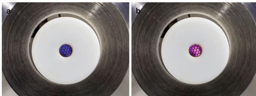
**Fig. 13.26** DART discharges as seen when looking into the source. (a) Blue shining discharge in nitrogen, (b) pale pink discharge in helium. The hexagonal pattern is caused by the exit grid electrode
