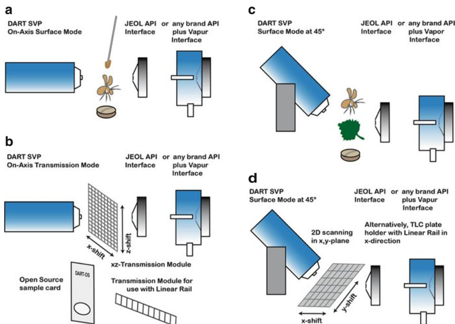
**Fig. 13.29** DART configurations. (a) First design with axial orientation of source and orifice of the API interface, (b) axial orientation for transmission mode when presenting samples on a mesh, (c) surface mode with source at an angle for analyzing small objects, and (d) surface mode at an angle for automated analysis of an array of samples (Adapted from Ref. [8] with permission. © Springer, 2013)
