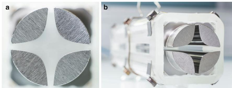
**Fig. 4.37** Linear quadrupole with hyperbolic rods. (a) Head on view showing the cross section of the rods and (b) whole device partially revealing the polished inner surfaces. The rods are mounted in a precision-machined quartz frame. This particular quadrupole once belonged to a Finnigan TSQ 700 instrument
