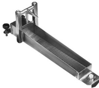
29.12 figure Photo of Bostwick consistometer (Courtesy of Cole-Parmer, Vernon Hills, IL)
