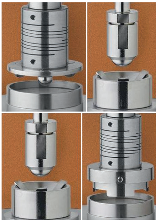
29.17 Tribological testing geometries (Courtesy of TA Instruments, New Castle, DE) figure
