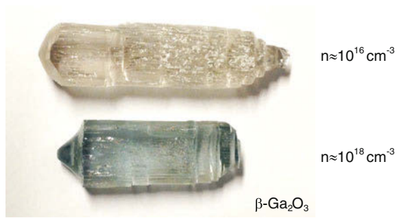
Fig. 9.39 Czochralski-grown \text{Ga}_2\text{O}_3 crystals with different electron concentration, courtesy of Z. Galazka, IKZ Berlin
