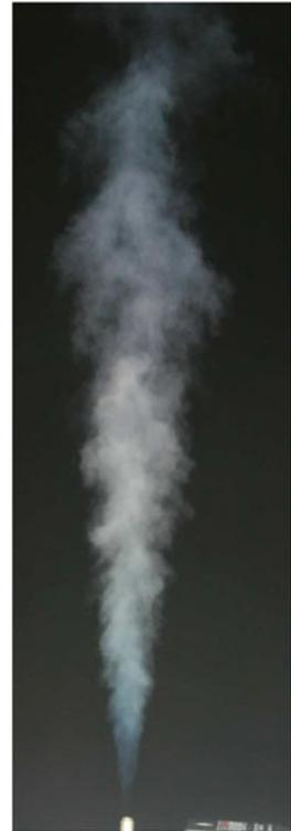
**Fig. 9.9** Steam jet at the outlet of a pressure cooker. Note the conical shape of the jet steam
