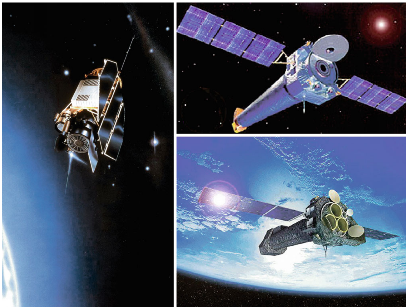
Fig. 1.47 Left: ROSAT, a German-US-British cooperation, observed from 1990 to 1999 in the energy range between 0.1 and 2.5 keV (soft X-ray). Upper right: Chandra was launched in July 1999. The energy range of its instruments lies between 0.1 and 10 keV. Its highly elliptical orbit permits long uninterrupted exposures. Lower right: XMM-Newton was launched in December 1999 and has since been in operation; it
