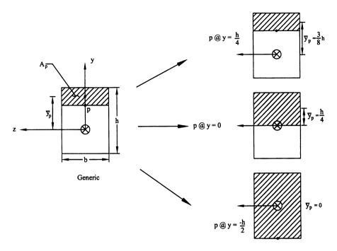
FIGURE 5.10 Illustration of the method for determining the value of  $Q = \overline{y}_p A_p$  in a rectangular cross section. The subscript p reminds us that these quantities are defined for the cross-sectional areas above a point p rather than over the entire cross section. Forgetting this is a common error. Q is seen to be zero at the top and bottom surfaces for different reasons.
