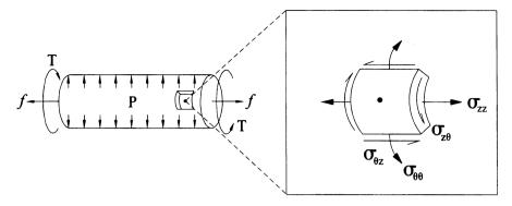
FIGURE 4.23 Complex state of stress in a cylindrical tube. Relative to z and  $\theta$ , the axial stress  $\sigma_{zz}$  is induced by the axial load f, the shear stress  $\sigma_{z\theta}$  is induced by the torque T, and the circumferential stress  $\sigma_{\theta\theta}$  is induced by the pressure P. Superposition applies because the problem is linear.
