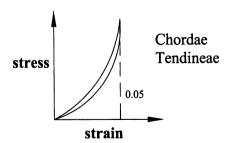
FIGURE 2.26 Schema of stress—strain data from a uniaxial test on an excised chordae tendineae, the thin stringlike tissue that connects the heart valve to the papillary muscle. Note the small, but not infinitesimal, strain. Many ligaments and tendons exhibit similar behavior.
