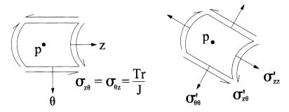
FIGURE 4.14 For pure torsion of a circular LEHI cylinder, the only nonzero component of stress at a point p is  $\sigma_{z\theta}$  relative to z and  $\theta$ . Relative to z' and  $\theta'$  however, we may have additional components of stress, including normal and shear. We are reminded, therefore, that components of stress at a point depend on the coordinate system that is employed; they are not unique physical measurables or quantities that are "felt" directly by a cell or tissue.
