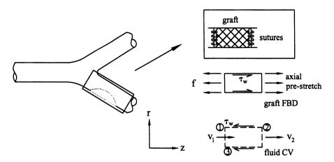
FIGURE 10.6 Free-body diagram and associated control volume for a combined solid mechanics/fluid mechanics analysis of stresses in an in-line arterial graft.
