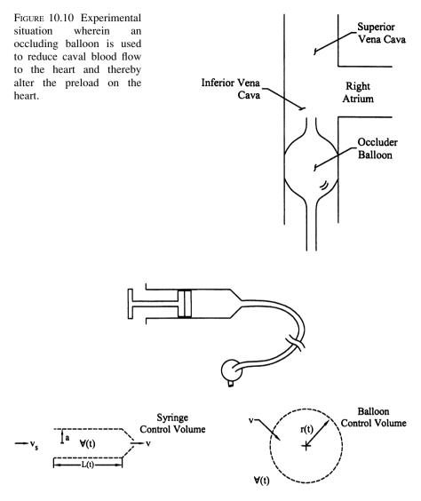
FIGURE 10.11 Inflation of a balloon via a syringe. Shown are separate control volumes for the syringe and the balloon.
