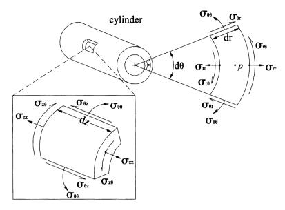
Figure 2.8 Components of stress relative to a cylindrical coordinate system, again using the standard notation  $\sigma_{(face)(direction)}$ .
