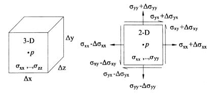
FIGURE 3.1 Representative stresses at a point p, with particular attention to those components in the x-y plane at distances  $\pm \Delta x/2$  and  $\pm \Delta y/2$  from point p. Note, therefore, that the components of stress may vary from point to point in general (because of the differential areas, the value of stress on an given surface area is represented by its mean over that area).
