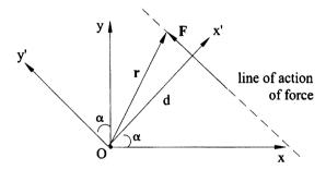
FIGURE 1.10 Schema of a force F acting in the x-y plane relative to an origin O. Although forces are vectors, and thus defined independent of a coordinate system (i.e., an origin and basis), they must be resolved into components relative to convenient coordinate systems to permit computations.
