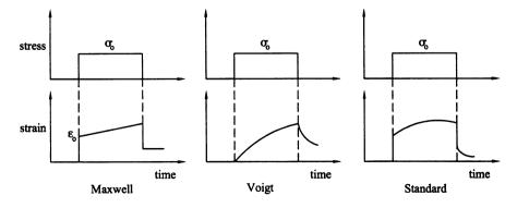
FIGURE 11.20 Similar to Fig. 11.19 except for creep.
