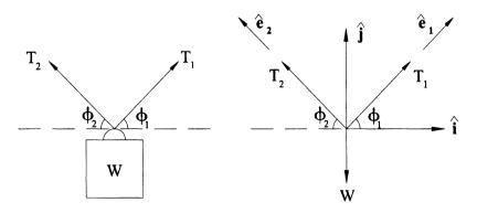
FIGURE 1.14 A weight W is supported by two cables, each having individual tensions  $T_1 = |F_1|$  and  $T_2 = |F_2|$ . The free-body diagram is shown to the right.
