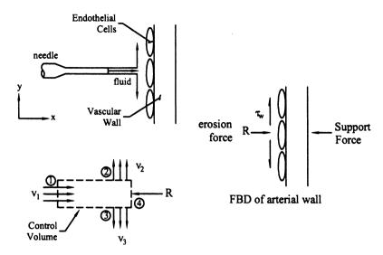
FIGURE 10.8 Experimental setup to determine the erosion stress for endothelial cells. Shown are a possible control volume for the fluid and a free-body diagram for the arterial segment. Although the fluid will exert shear stresses on the cells, we are interested primarily in the normal force R in this experiment.
