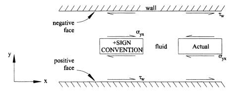
Figure 9.5 Positive sign convention for fluid stresses  $\sigma_{(face\ direction)}$  relative to a Cartesian coordinate system and the associated actual shear stresses in a fluid element  $\sigma_{xy}$  and on the wall  $\tau_w$  in a parallel-plate experiment.
