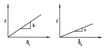
FIGURE 11.16 Mechanical behavior of a linear spring, with modulus k, and a linear dashpot, with viscosity c.
