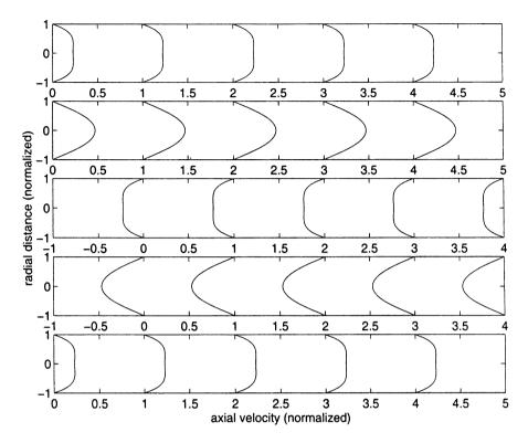
FIGURE 9.20 Pulsatile velocity profiles computed for low frequencies (1 Hz). Results are shown for different phase angles  $\omega t$ , values being 0° at the top and increasing by 90° for subsequent panels. Note that the flow "develops" over time at a single location similar to its development with distance in an entrance length. [From Zamir (2000), with permission from Springer].
