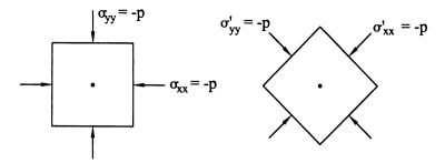
FIGURE 7.10 So-called hydrostatic state of stress (shown in two dimensions simply for convenience) wherein the normal components each equal -p, the fluid pressure, and the shear components are all zero—both relative to all coordinate systems.
