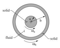
FIGURE 9.14 Steady flow of an incompressible Newtonian fluid between two concentric, rigid, circular cylinders which may rotate at different angular velocities  $\omega_a$  and  $\omega_b$ . In practice, the gap distance h = b - a would be small in comparison to a; thus, the gap is exaggerated for illustrative purposes only.
