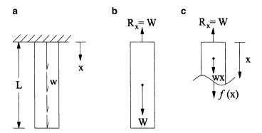
FIGURE 4.5 A vertically loaded member subject to its own weight, given as w (force per unit length) and thus a total weight W = wL, which acts at the center of gravity. Shown is the physical problem, a free-body diagram of the whole to isolate reaction  $R_x$  at the fixed support, and a free-body diagram of a part to isolate the internal force f(x).
