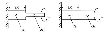
FIGURE 4.16 Two idealized circular cylinders of length L are acted upon by a single, constant end torque T. The cylinder on the *left* has a nonconstant cross section, whereas the one on the *right* is nonhomogeneous in composition.
