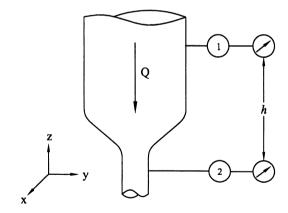
8.7 Derive the streamline direction Euler equation for the case where the streamlines are horizontal and all parallel; assume an arbitrary body force vector *g*, which may include gravity and electromagnetic effects (see Fig. 8.22).
