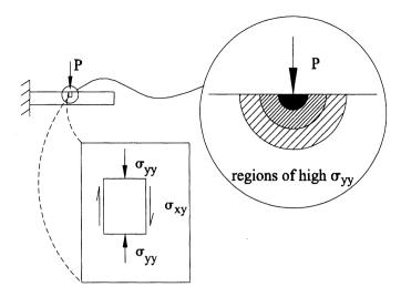
FIGURE 5.13 Schema of y-face, y-direction stresses  $\sigma_{yy}$  in the neighborhood of a concentrated load P. The *contour lines* show that the value of  $\sigma_{yy}$  decreases (shown by cross-hatching that becomes less dense) as one gets farther from the source of the concentrated load. No real load is truly concentrated, of course, for it must act over a finite, albeit possibly small, area.
