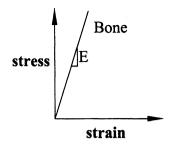
FIGURE 2.27 Schema of stress–strain data from bone prior to yield, which reveals an initially linear, nearly elastic response. Note that bone (type I collagen impregnated with hydroxyapatite) is much stiffer and less extensible than the chordae (Fig. 2.26; primarily type I collagen).
