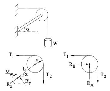
FIGURE 1.15 An ideal (frictionless) pulley of radius a is mounted from a wall at angle  $\alpha$  and length L. Free-body diagrams of the whole pulley and its rotating part alone isolate reaction and internal forces and moments of interest.
