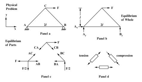
FIGURE 1.17 Shown is a simple 2-D truss (panel a) and associated free-body diagrams of the whole structure (panel b) and individual parts (panel c). Panel (d) shows results of the final analysis with regard to which members support tension versus compression.
