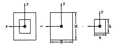
FIGURE 5.27 Another example of the method of composite sections to determine a second moment of area—this time for a cross section with a hole.
