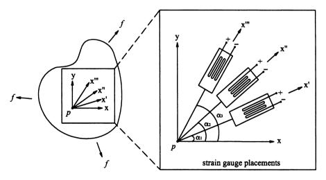
FIGURE 2.22 Placement of three strain gauges to form a so-called strain rosette. It is assumed that each gauge is affixed to the surface at a known angle. Although small, strain gauges are obviously of finite, not infinitesimal, size, thus information from rosettes necessarily represent mean values of strain within the region of measurement.
