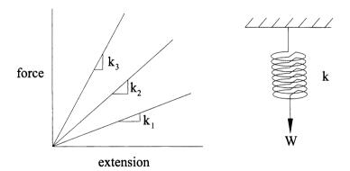
FIGURE 2.2 Force—extension behavior of three different metallic springs, which exhibit linear behaviors and thereby can be quantified by individual spring constants k (or stiffnesses). Although many springs exhibit a linear behavior, nonlinear springs exist as well.
