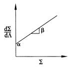
FIGURE 6.5 Fung's idea to plot stiffness (i.e., a change in stress with respect to stretch,  $d\Sigma/d\Lambda$  in one dimension) versus the first Piola–Kirchhoff stress ( $\Sigma$ ), which, for many tissues, results in a nearly linear relationship.
