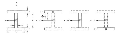
FIGURE 5.26 Illustration that, like first moments of area (cf. Appendix 3 of Chap. 3), second moments of area can be determined using a method of "composite" sections shown by *solid lines*. The parallel axis theorem is fundamental to such determinations.
