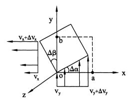
FIGURE 7.6 Rigid-body rotation of a fluid element in two dimensions. Note that such a rotation implies that the velocity must vary from point to point, such as the y-direction velocity at point a (e.g.,  $v_y + \Delta v_y$ ) must be greater than that at point o (e.g.,  $v_y$ ) for the line  $\overline{oa}$  to rotate counterclockwise. A similar difference must exist in  $v_x$  at points b and o.
