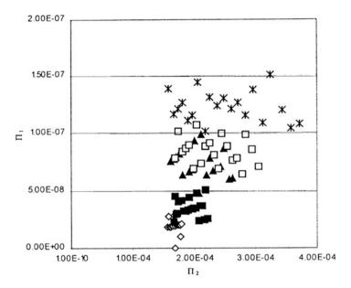
FIGURE 11.3 Data for two of the nondimensional parameters from Eq. (11.20):  $\pi_1$  versus  $\pi_2$  for various values of  $\pi_7$  (denoted by *open diamonds*, *closed squares*, *closed triangles*, *open squares*, and *asterisks* for increasing levels of stretch from 1.0 to 1.6, clearly finite deformations). With permission from Elsevier Science.
