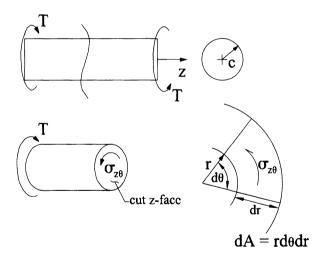
FIGURE 4.12 Alternate free-body diagram for the circular cylinder shown in Fig. 4.11, this time isolating a  $\sigma_{z\theta}$  stress, on a cut z face, which serves to balance the applied torque. This balance is achieved, of course, via the net effect of all such stresses acting on their respective cross-sectional differential areas dA and at a distance from the axis called the moment arm.
