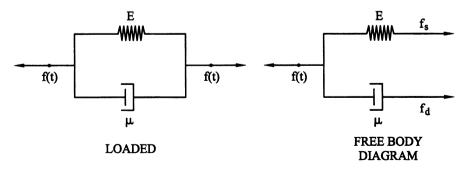
FIGURE 11.17 The Kelvin-Voigt element consisting of a linear spring and dashpot in parallel.
