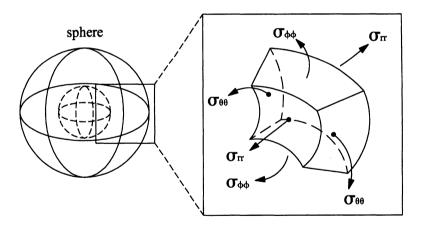
Figure 2.9 Normal components of stress relative to a spherical coordinate system, again denoting the components as  $\sigma_{(face)(direction)}$ . As an exercise, add the shearing components.
