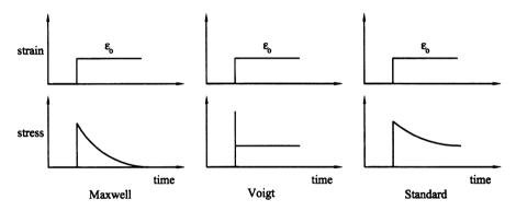
FIGURE 11.19 Characteristic stress relaxation responses of the Maxwell, Kelvin-Voigt, and Standard element consistent with the derivations in the text.
