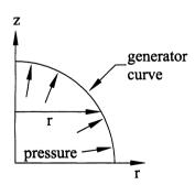
FIGURE 6.13 Pressure–volume geometry for an axisymmetrically inflated membrane. By axisymmetric, we mean that a generator curve can be revolved about an axis to yield the surface of the membrane. Axisymmetry imposes certain restrictions on the material properties and applied loads.
