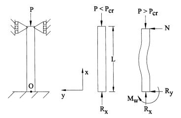
FIGURE 5.24 Solutions of beam-column problems are very sensitive to the boundary conditions. Shown here is a fixed-pinned column.
