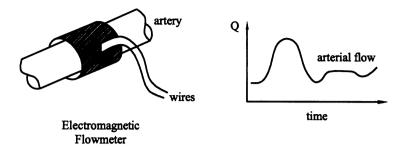
FIGURE 8.14 Schema of the time-varying volumetric flow rate Q measured in vivo using an electromagnetic flowmeter.
