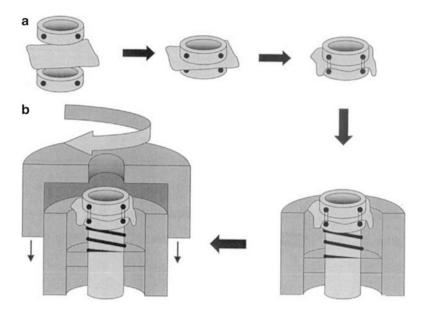
FIGURE 11.2 Expanded view of the specimen fixture from Fig. 11.1. Note that the specimen is placed within the fixture in a stress-free configuration (Panel *a*). This is facilitated by having a waxed platform inside the restraining rings on which a fluid film can support the specimen prior to mounting. Turning the outer lid pushes down on the membrane holder, which, in turn, imposes a uniform radial stretch of the specimen (Panel *b*). With permission from Elsevier Science.
