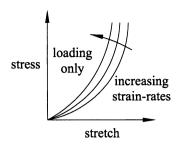
FIGURE 6.3 Possible sensitivity of the stress-stretch response to changes in strain rate (loading curves only). In many cases, however, there is little change in the response with three orders of magnitude changes in strain rate.
