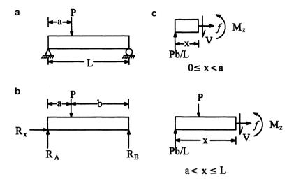
FIGURE 5.2 Shown here is a transversely loaded, simply supported beam (panel  $\mathbf{a}$ ), the free body of the whole structure (panel  $\mathbf{b}$ ), and free-body diagrams of two parts of the structure (panel  $\mathbf{c}$ ) that isolate the internal loads and moments in two regions of interest. Note: Remember that judicious cuts are often best taken between abrupt changes in loads, as done here.
