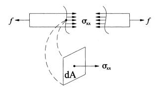
FIGURE 3.4 A free-body diagram constructed by making a fictitious cut in the central region of a test sample for isolating the *x*-face stresses of interest. We assume that only the normal stress  $\sigma_{xx}$  acts on the cut face for shear stresses are not needed to balance the applied axial load *f*. Moreover, although  $\sigma_{xx}$  is assumed to be uniform in the central region, far enough away from the ends, we must remember that stresses act over differential, not total, areas.
