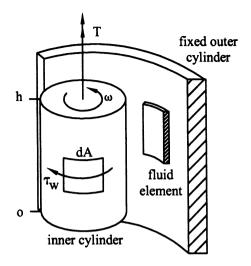
concentric cylinder viscometer
