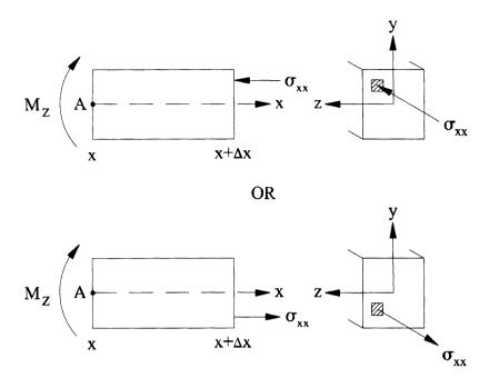
FIGURE 5.7 Side view and oblique view of a fictitiously cut beam that exposes the normal stress  $\sigma_{xx}$ , which acts over a differential area dA = dydz. Given the applied moment shown, the stress is expected to be compressive in the upper portion of the beam (y > 0) and tensile in the lower portion (y < 0). Either free-body diagram (top or bottom) is sufficient for purposes of a force balance.
