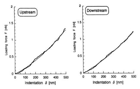
FIGURE 5.17 Measurement of the mechanical response of an isolated endothelial cell to an AFM indentation force. Shown are the force–indentation data, which reveal a nonlinear character and that the upstream portion of the cell tends to be slightly stiffer than the downstream portion when subjected to a flow-induced shear stress. [From Sato et al. (2000) J Biomech 33:127–135, with permission from Elsevier].
