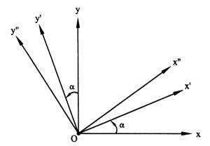
FIGURE 2.6 Interrelations, via single angles, between different Cartesian coordinate systems that share a common origin and a z-axis. The angle  $\alpha$  is taken to increase in the direction given by the right-hand rule: counterclockwise, with the z-axis coming out of the paper.
