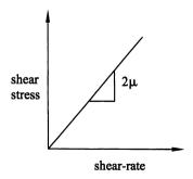
FIGURE 7.9 Shear stress plotted versus shear rate for a Newtonian fluid. Note the linear relationship, the slope of which is denoted by  $2\mu$ , where  $\mu$  is the (absolute) viscosity. The factor 2 is included simply to cancel the 1/2 that appears in the expression for shear rates [e.g.,  $D_{xy}$ , as in Eq. (7.56)].
