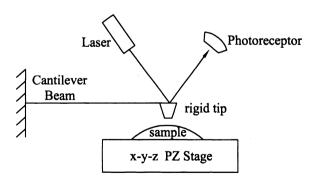
FIGURE 5.16 Schema of the basic components of an atomic force microscope (AFM). The deflection of the cantilevered beam (i.e., probe) is measured with an optical lever consisting of a laser source and photoreceptor (cf. Fig. 4.21). The sample is placed on a piezoelectric (PZ) stage that can move in *x-y-z*. In some systems, the PZ stage moves the probe rather than the sample, but the net effect is the same.
