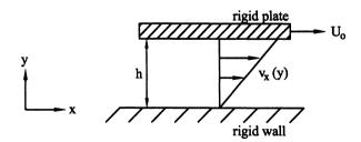
FIGURE 9.7 Couette flow induced by the relative motion of an *upper plate*, at constant velocity  $U_0$ , relative to a fixed rigid plate at the *bottom*. The associated velocity profile in the fluid is linear and, consequently, the fluid shear stress is uniform.
