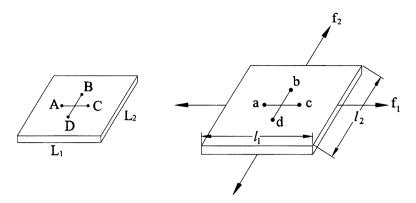
FIGURE 6.10 Dimensions of a biaxial specimen in the central region, before and after loading and assuming a homogeneous deformation; a, b, c, and d denote tracking markers for computing strain in the central region of the soft tissue sample. Strain gauges cannot be used, of course, because of their extreme stiffness.
