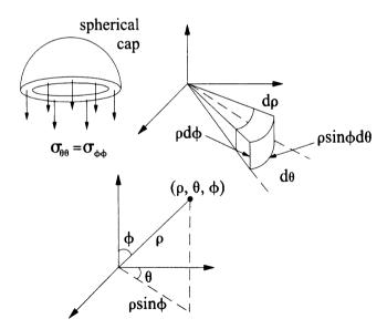
FIGURE 3.19 Free-body diagram of half of a pressurized spherical membrane, the associated coordinate system  $(\rho, \theta, \phi)$ , and a convenient differential area for force balance.  $\sigma_{\theta\theta} = \sigma_{\phi\phi}$  simply because of spherical symmetry—in other words, because a force balance and free-body diagram that separates the sphere into left and right halves yields the same result as one that separates it into top and bottom halves.
