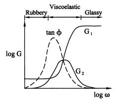
FIGURE 11.21 Characteristic complex moduli for viscoelastic behaviors in rubbery and glassy regimes.
