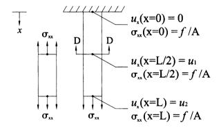
FIGURE 2.18 Displacements at various locations in a uniformly loaded, vertically suspended structural member. Note, in particular, that the value of the displacement varies from point to point (i.e., it is nonuniform), whereas the value of the xx component of stress does not vary.
