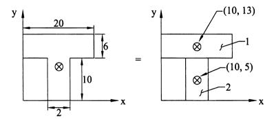
Figure 3.25 Compute the first moment of area of this composite section.
