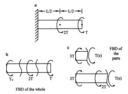
FIGURE 4.17 A LEHI circular cylinder subjected to multiple applied torques. A free-body diagram of the whole allows the reaction support  $T_w$  to be determined; free-body diagrams of judiciously selected parts allows internal torques to be determined as a function of z. Remember that judicious cuts are typically those taken between abrupt changes in applied loads.
