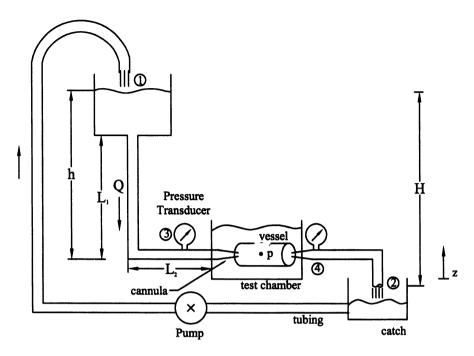
Figure 10.17 Possible laboratory setup to examine flow through a stenotic vessel.
