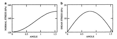
FIGURE 2.14 Plot of the normal and shear stresses  $\sigma'_{xx}$  and  $\sigma'_{xy}$  as a function of  $\alpha \in [0, \pi/2]$  radians (i.e.,  $90^{\circ}$ ). Note that the local extrema for the normal stress occur at  $\alpha = 0$  and  $90^{\circ}$ , whereas the local maximum for the shear stress is at  $\alpha = 45^{\circ}$ .
