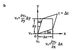
FIGURE 7.7 Panel (a): Schema of an experimental system that gives rise to a simple shear of a fluid element; panel (b): similar to Fig. 7.6 except for a pure shear rather than a rigid-body rotation. In this case, the internal angle decreases a small amount,  $(\Delta \alpha + \Delta \beta)$ , over an interval of time  $\Delta t$ .
