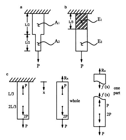
Figure 4.6 Axially loaded rods having a nonconstant cross section (panel  $\mathbf{a}$ ), a nonconstant material composition (panel  $\mathbf{b}$ ), and multiple applied loads (panel  $\mathbf{c}$ ). Although we need to draw free-body diagrams of the whole and multiple parts for each case, we show only the free-body diagram of the whole structure and one free-body diagram for a part of the rod of panel  $\mathbf{c}$ .
