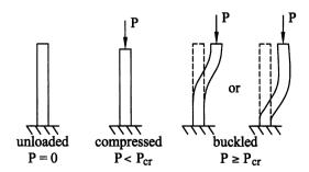
FIGURE 5.20 A cantilevered beam is subjected to a compressive end load P. Initially the beam-column will simply compress and the stress  $\sigma_{xx} = -P/A$ , as in Chap. 3. After a critical value  $P_{\rm cr}$  is reached, the beam column will buckle (i.e., bend abruptly) and the analysis of stress and strain becomes much more complex. Hence, rather than computing these complex states of stress or strain, let us focus simply on that value of  $P_{\rm cr}$  that induces buckling.
