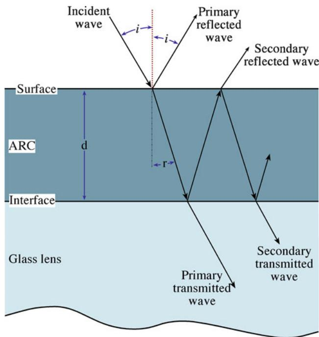
FIGURE 32.8. How antireflection coating works.
