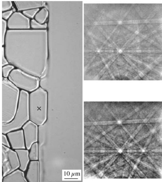
FIGURE 24.20. Scanning electron microscopy shows two electron-beam backscattering diffraction (EBSD) patterns from a series of engineered GBs in  $\text{Al}_2\text{O}_3$ . The upper DP is from point X, and the lower DP is from the large grain on the left, showing the basal-twin relationship.
