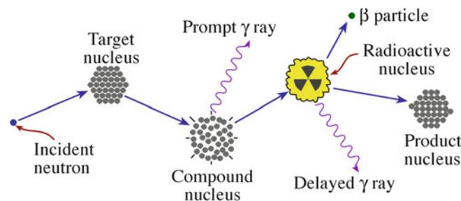
FIGURE 10.36. Neutron activation analysis (NAA) process.
