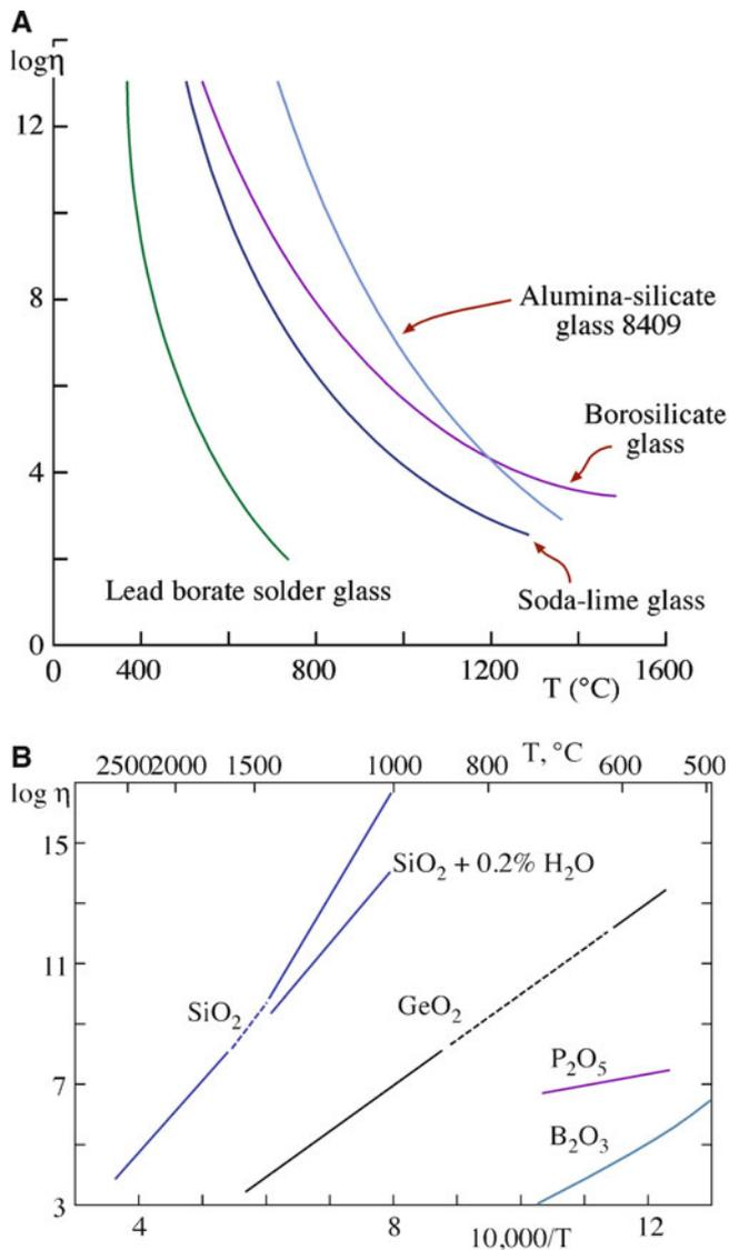
**FIGURE 21.4.** (A) Viscosity as a function of temperature ( $T$ ) for several silicate glasses: units of  $\eta$  are dPa·s. (B) Viscosity as a function of temperature ( $1/T$ ) for the main glass-forming oxides. Notice the effect that a small amount of water has on the viscosity of silica glass.
