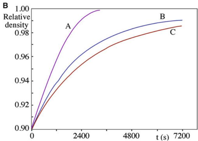
**FIGURE 24.10.** Calculated densification curves at the final stage of sintering at 1,727°C for alumina powder compacts for grain sizes of 0.8 and 4.0  $\mu\text{m}$  (B) at 90% density. The curves are calculated using different equations but show the same trends.
