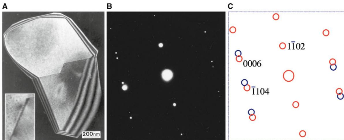
**FIGURE 14.20.** Rhombohedral twin boundary in Al<sub>2</sub>O<sub>3</sub> and its diffraction pattern.
