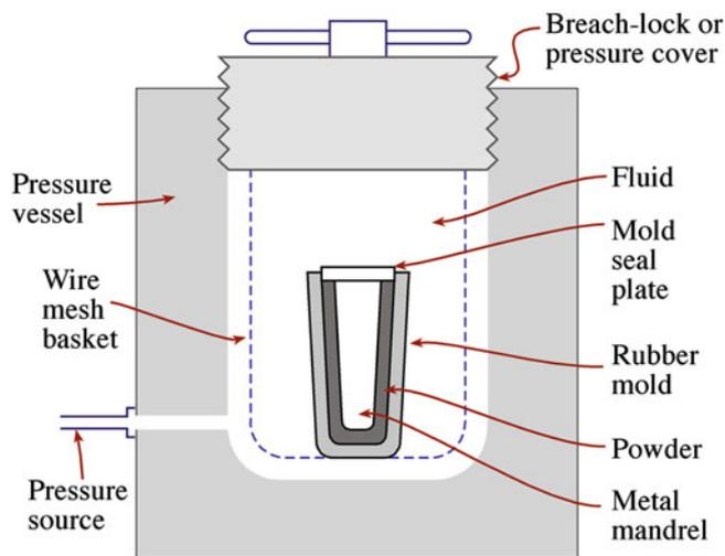
FIGURE 23.3. Wet-bag isostatic pressing system.
