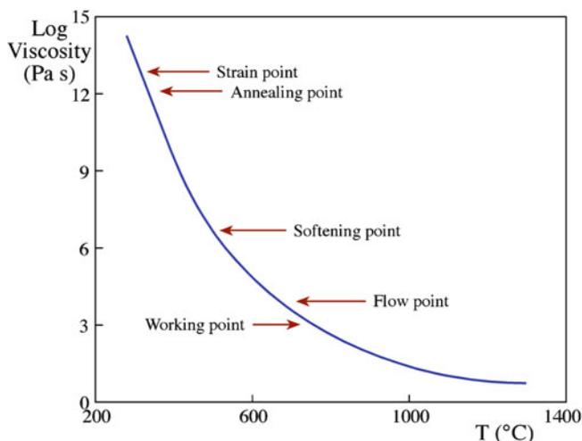
FIGURE 17.21. Temperature dependence of viscosity for a soda-lime-silica glass.
