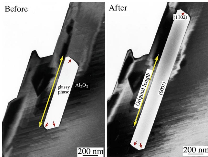
FIGURE 15.7. Glass “particles” in a thin film of  $\alpha$ - $\text{Al}_2\text{O}_3$ , before and after additional heat treatment.
