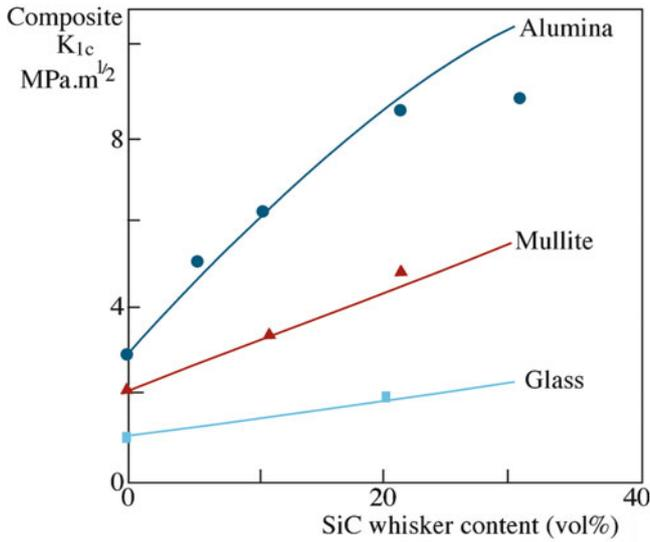
FIGURE 18.20. Effect of SiC whisker content on toughness enhancement in different matrices.
