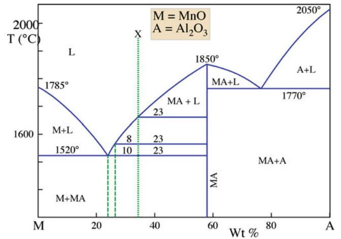
FIGURE 8.22. MnO-Al<sub>2</sub>O<sub>3</sub> phase diagram.
