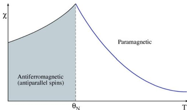
**FIGURE 33.8.** How  $\chi$  varies with  $T$  for an antiferromagnetic material. At  $\theta_N$ , it becomes paramagnetic.
