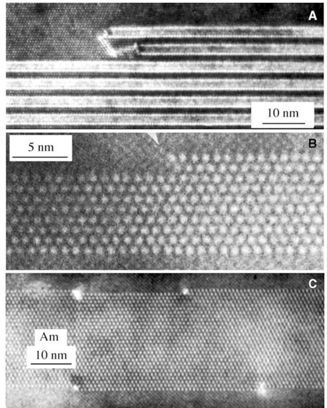
**FIGURE 25.17.** Chemical reactions by movement of steps on an interface. (A)  $\beta\text{-Al}_2\text{O}_3$  growing in spinel. (B, C) Amphibole growing in orthopyroxene.
