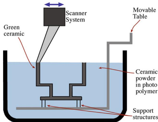
FIGURE 23.13. Stereolithography (SLA) solid free-form fabrication (SFF) process.
