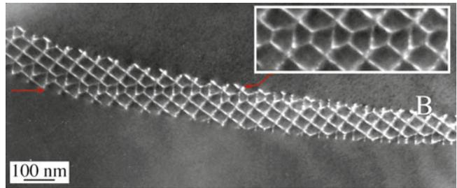
**FIGURE 14.13.** Extrinsic dislocation interacting with a low-angle {001} twist GB in spinel. Inset: note how all the dislocations are changed by the interaction.
