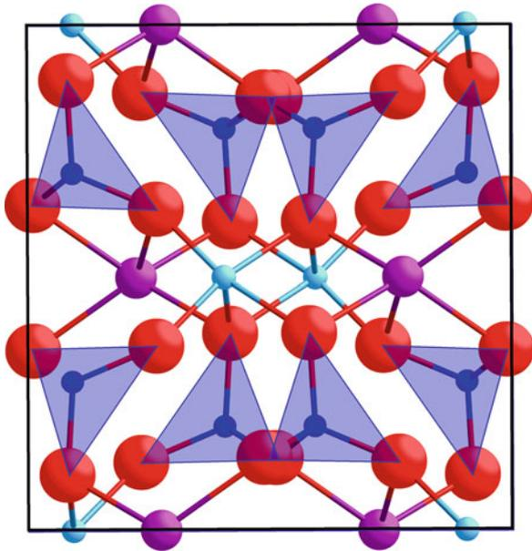
**FIGURE 7.11.** Crystal structure of a pyroxene (spodumene) shows layers of  $\text{Li}^+$  (larger) and  $\text{Al}^{3+}$  (smaller) ions in octahedra alternating with layers of  $\text{Si}^{4+}$  in tetrahedra, giving a nominal formula of  $\text{LiAlSi}_2\text{O}_6$ .
