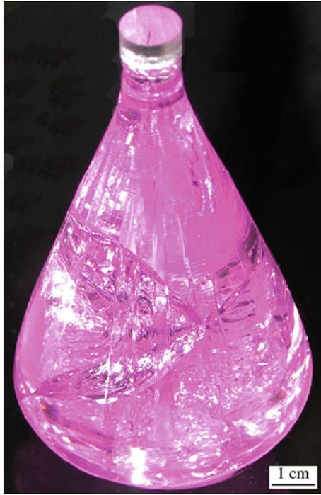
FIGURE 16.1. Cracking in an Nd-doped YAG boule.
