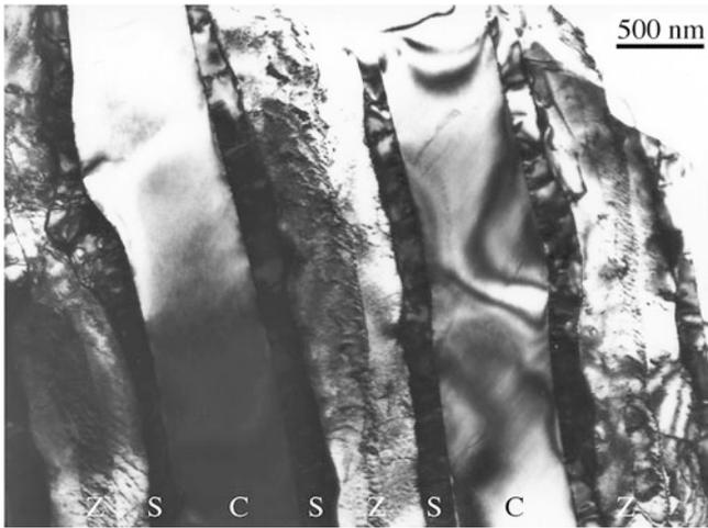
**FIGURE 15.18.** CoO/ZrO<sub>2</sub> eutectic after solidification and subsequent oxidation. Z: ZrO<sub>2</sub>; C: CoO; S: Co<sub>3</sub>O<sub>4</sub> (spinel).
