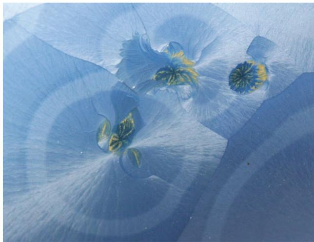
FIGURE 21.15. Spherulitic crystallization in a glass.
