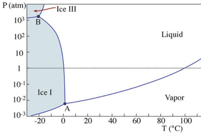
FIGURE 8.6. H<sub>2</sub>O phase diagram (1,000 atm. is ~100 MPa).
