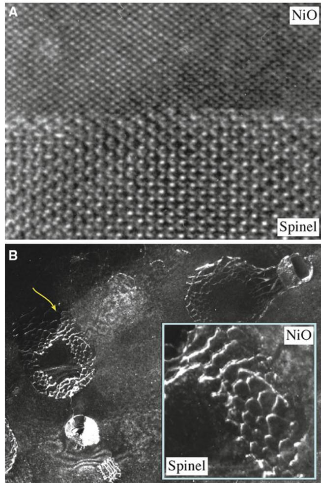
**FIGURE 15.3.** Spinel/ $\text{NiO}$  PB. (A) HRTEM image of lattice-matched PB. (B) Dislocations present at the interface after relaxation to accommodate lattice misfit. The inset is from the arrowed region.
