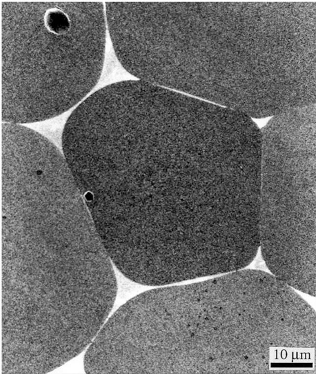
**FIGURE 14.29.** Scanning electron microscopy (SEM) image of glass-infiltrated MgO shows glass located at the GB and at triple junctions (TJs), but even in a GB it need not be a uniform layer.
