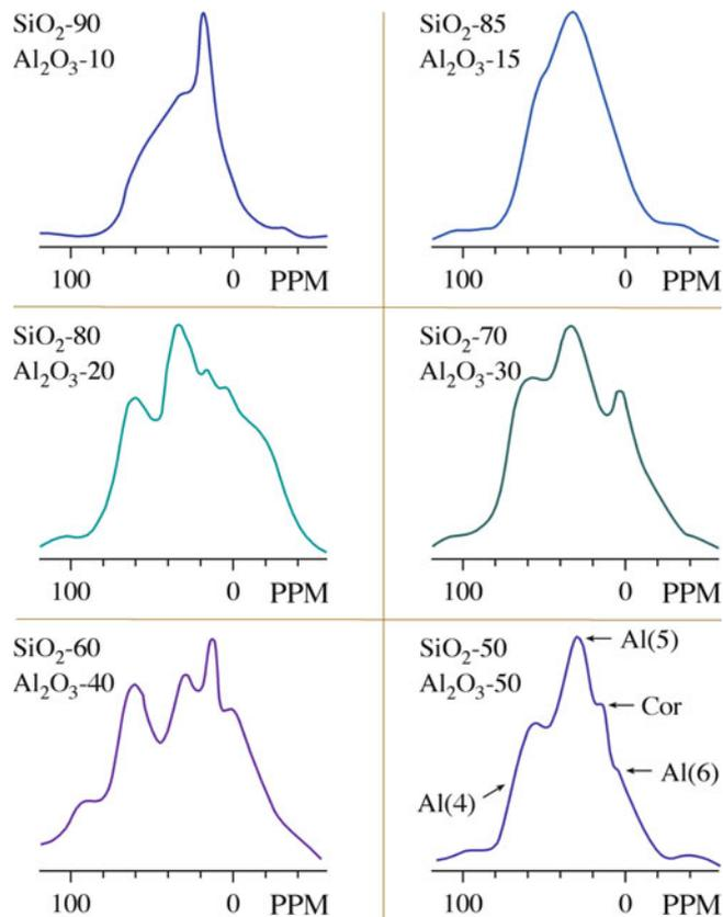
FIGURE 10.22. NMR signals from an Al-Si glass.
