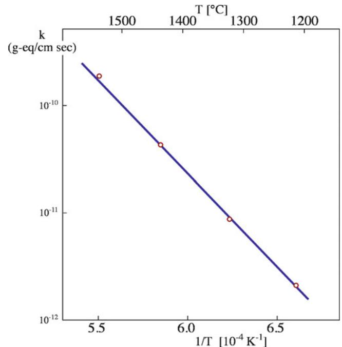
FIGURE 3.8. Arrhenius plot. The slope of the line indicates the activation energy for the process.
