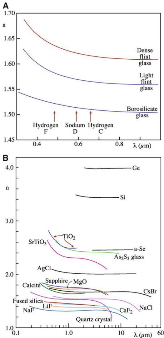
**FIGURE 32.5.** (A) Change in  $n$  with  $\lambda$  for several commercial glasses. (Hydrogen F, Sodium D, and Hydrogen C refer to specific light sources that have  $\lambda = 589$ , 486, and 656 nm, respectively). (B) Change in  $n$  with  $\lambda$  for several ceramics and glasses.
