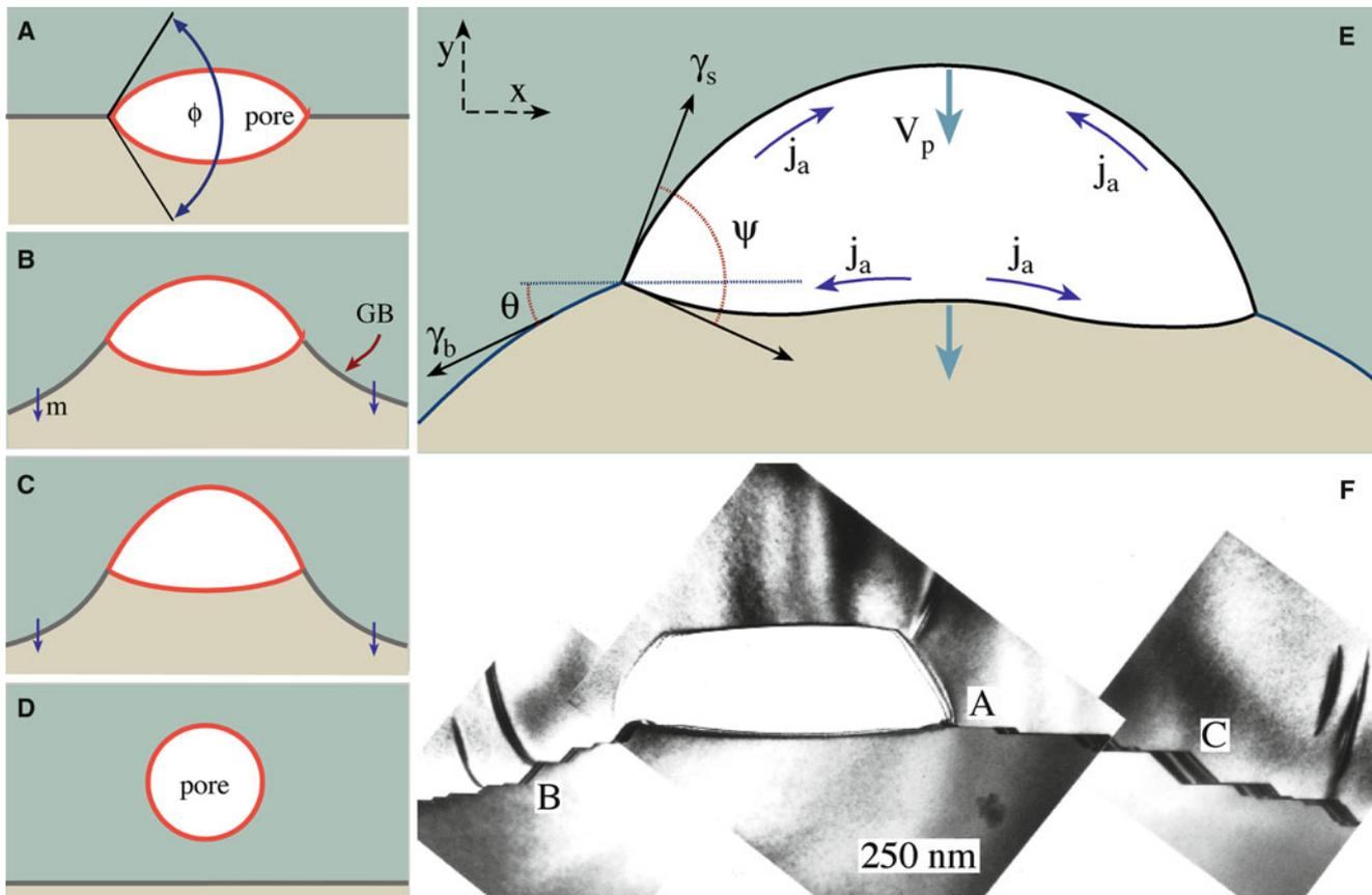
FIGURE 24.14. GB–pore interaction: the break-away process.
