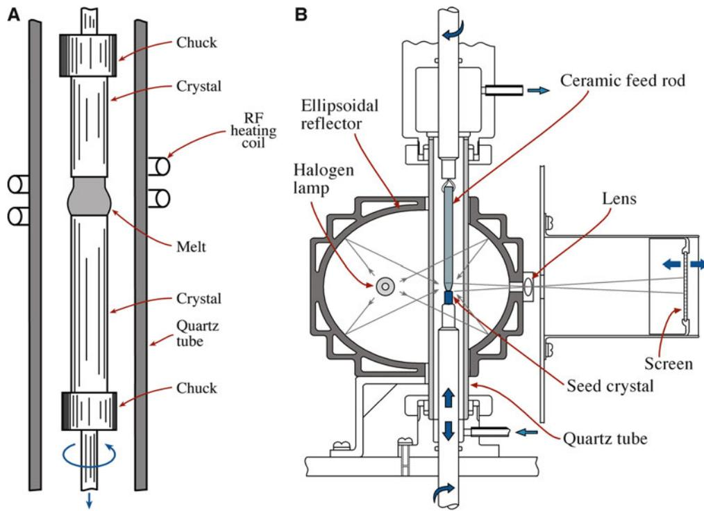
FIGURE 29.2. (A) Vertical float zone. (B) Arc-image furnace.
