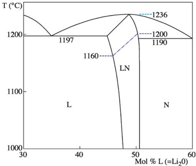
FIGURE 29.10. Part of the  $\text{Nb}_2\text{O}_5\text{-Li}_2\text{O}$  phase diagram.
