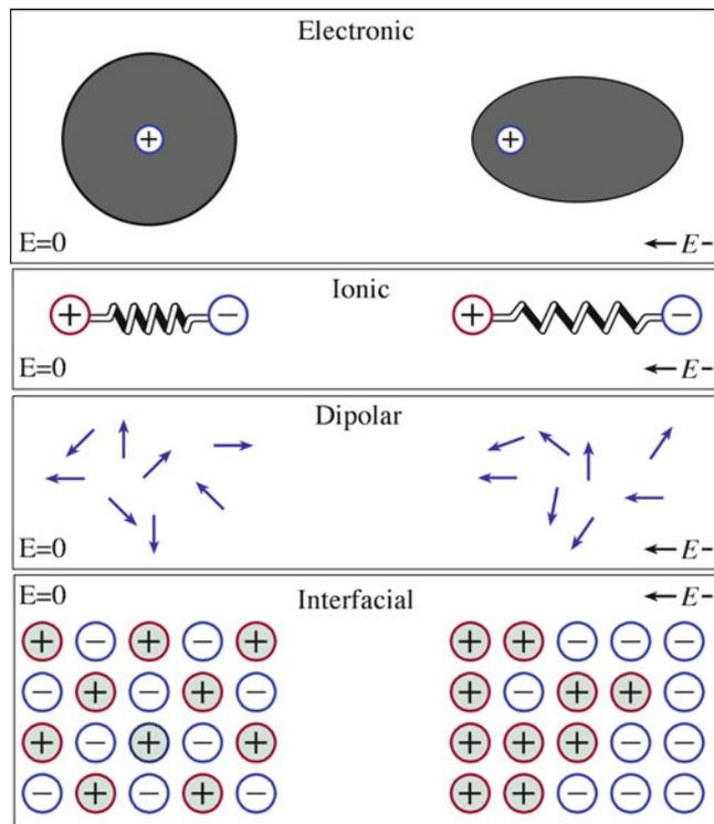
**FIGURE 31.1.** Different polarization mechanisms in a solid.
