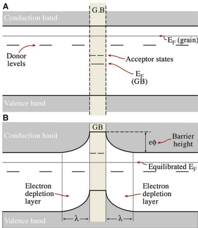
**FIGURE 30.18.** Proposed band diagram for two semiconducting ZnO grains separated by an IGF. (A) Location of acceptor sites in the IGF. (B) At equilibrium. Application of a potential decreases the barrier height.
