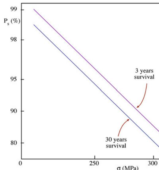
**FIGURE 16.27.** Stress–probability–time (SPT) diagram for medical-grade  $\text{Al}_2\text{O}_3$ . Survival probability decreases with increasing stress and longer times.
