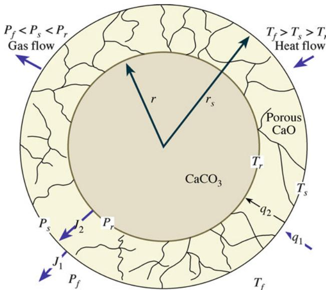
FIGURE 25.25. Processes involved in decomposing a carbonate.
