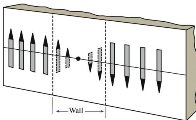
**FIGURE 31.5.** A 180° domain wall. The width is ~0.2–0.3 nm.
