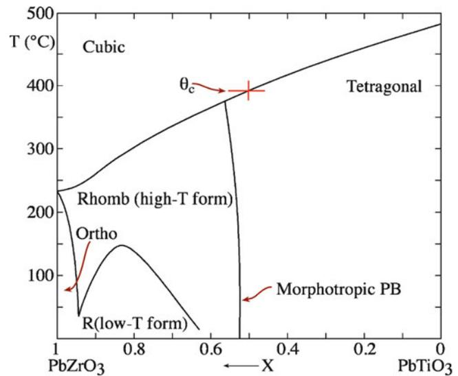
FIGURE 31.20. Lead zirconate titanate (PZT) phase diagram.
