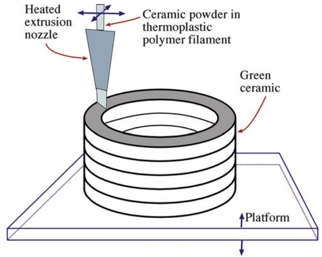
FIGURE 23.14. Fused deposition (FD) SFF process.
