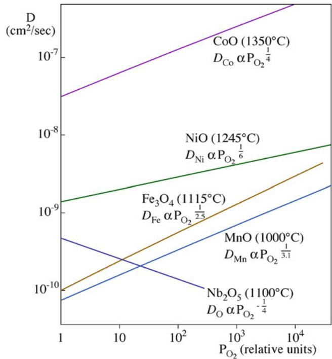
FIGURE 11.14. Diffusion coefficients varying with  $p_{O_2}$ .
