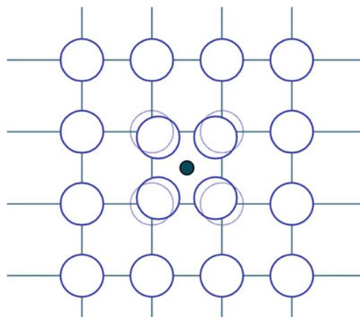
FIGURE 30.29. Lattice distortion around a free electron, which leads to the formation of Cooper pairs.
