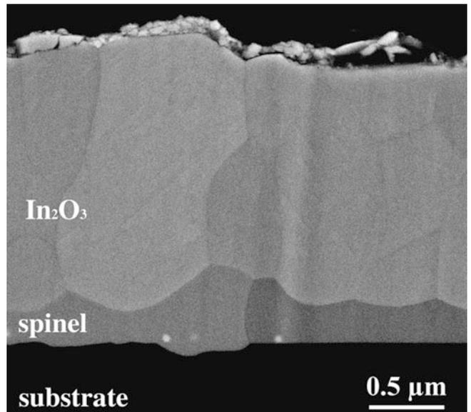
**FIGURE 10.7.** Backscattered electron (BSE) microscopy shows different contrast from different materials in an MgO/In<sub>2</sub>O<sub>3</sub> reaction couple.
