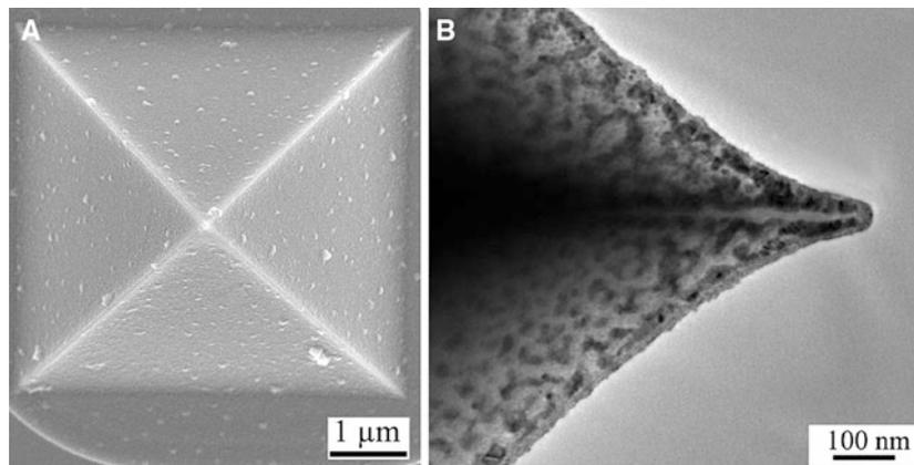
**FIGURE 13.17.** Electron microscopy images of atomic force microscopy (AFM) probe tips: end-on (SEM) and side view (TEM). The latter has been coated to test the interaction with the sample.
