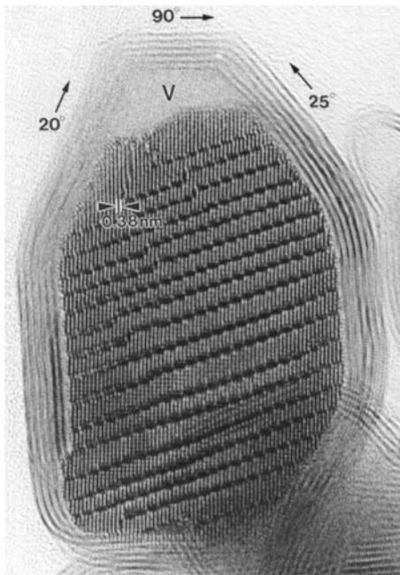
**FIGURE 14.25.** Defect W oxide encapsulated in a fullerene.
