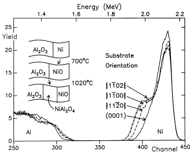
**FIGURE 10.29.** RBS data sets obtained using a 2.8-MeV beam of He<sup>2+</sup> ions with the samples tilted 45°. Each sample has been annealed at 700°C for 2 h followed by 1,020°C for 5 h. The Ni peak shows that the extent of the reaction varies with the surface orientation.
