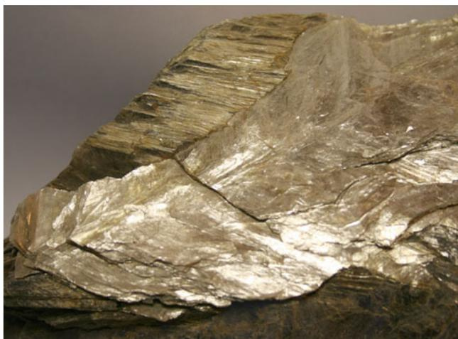
FIGURE 2.6. Large “grains” of mica clearly show the lamellar nature of the mineral. Two orientations are present in this one piece, which is about 10 cm wide.
