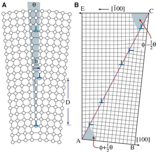
FIGURE 14.6. Low-angle tilt GBs. (A) Symmetric. (B) Asymmetric.
