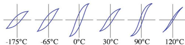
**FIGURE 31.13.** Hysteresis loops for BaTiO<sub>3</sub> as a function of temperature.
