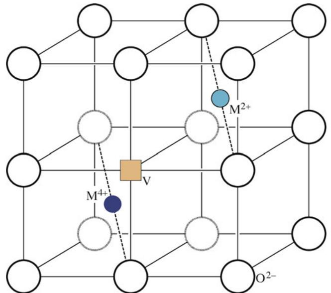
FIGURE 11.5. Accommodation of Ca<sup>2+</sup> in ZrO<sub>2</sub>. Note: this is just half of the unit cell.
