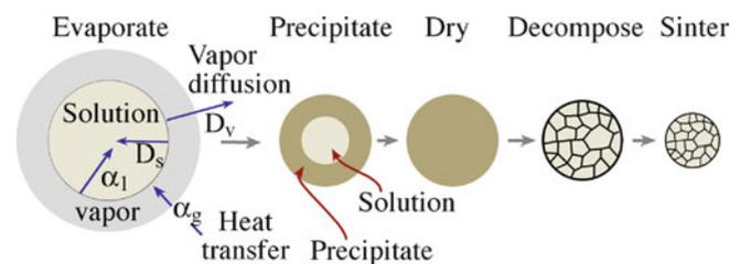
**FIGURE 20.4.** Stages in the spray pyrolysis process.
