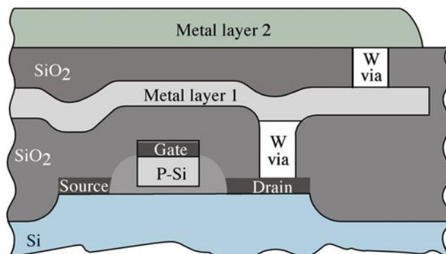
**FIGURE 28.3.** Cross section of multilayer metallization to a polysilicon gate field effect transistor. The contacts to the source and drain are silicides. Tungsten is used to provide vertical interconnects through vias in the oxide layer.
