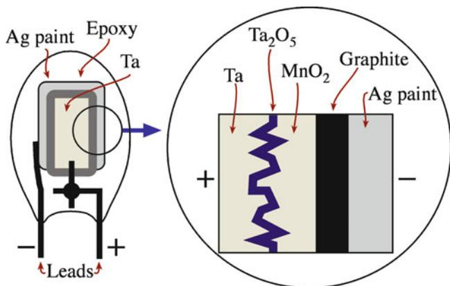
FIGURE 38.8. Structure of a solid electrolyte Ta capacitor.
