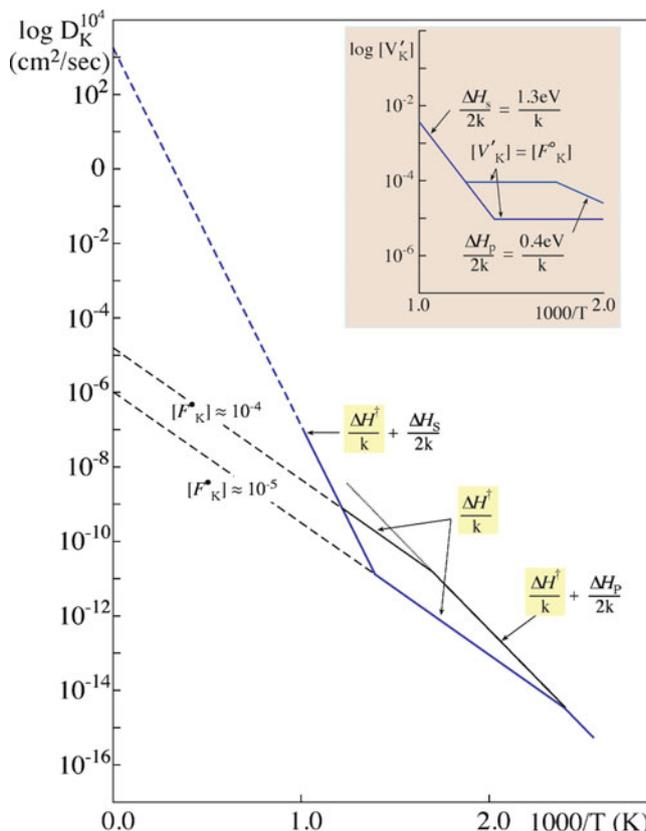
**FIGURE 11.11.** Diffusion coefficients in the intrinsic and extrinsic ranges. KCl with 10<sup>-4</sup> and 10<sup>-5</sup> atomic fraction divalent cation impurities.
