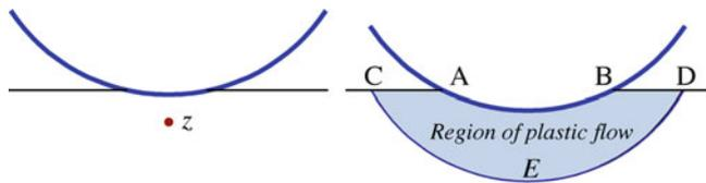
FIGURE 16.15. Plasticity under the indenter (shaded area) causes the deviation from Hertzian behavior.
