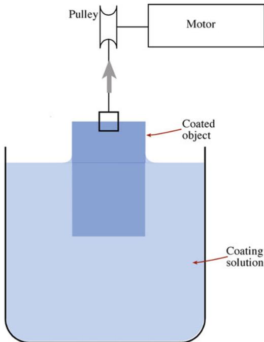
FIGURE 27.6. Simple dip-coating process.
