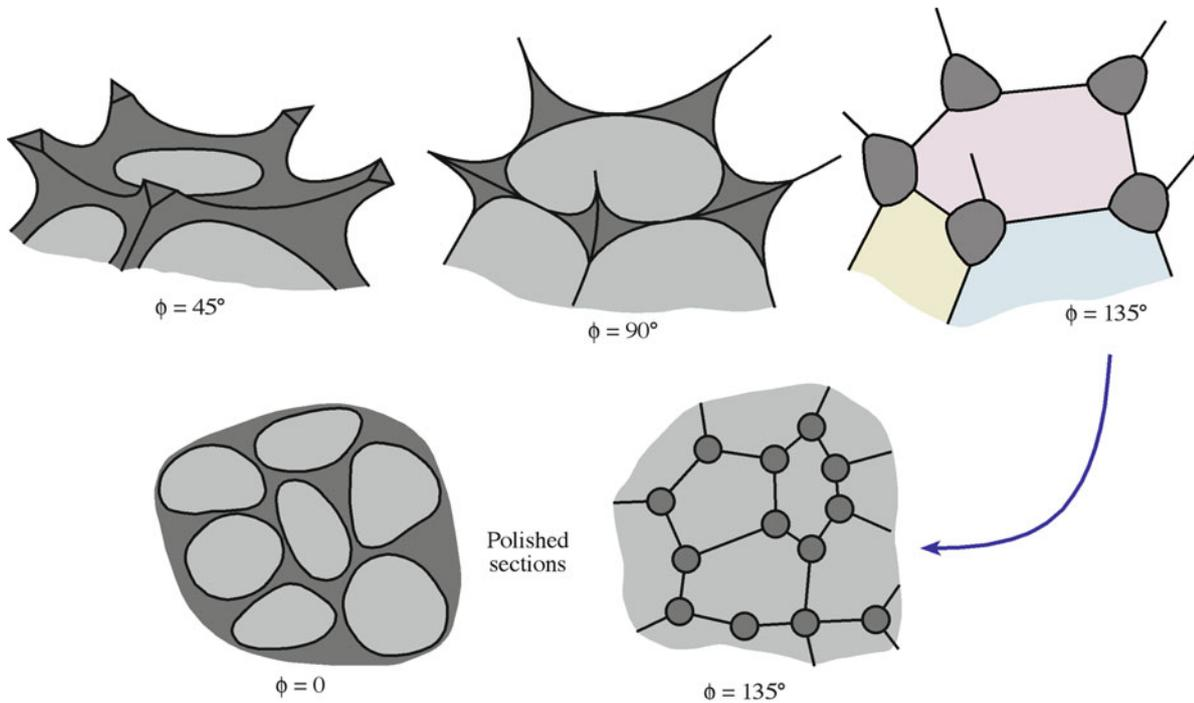
**FIGURE 14.33.** Three-dimensional relationships between IGFs, TJs, and QJs as the wetting angle is changed. Lower: a reminder that we usually see sections of these structures.
