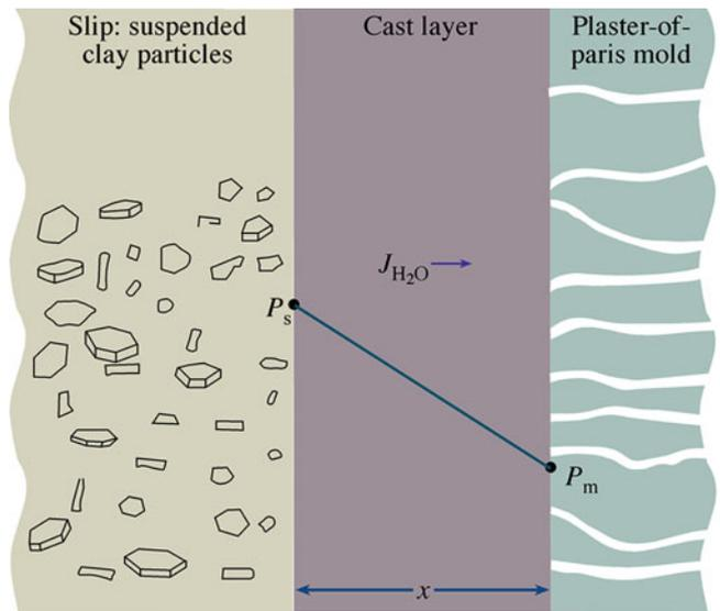
**FIGURE 25.11.** Slip drying to form a slip-cast layer.
