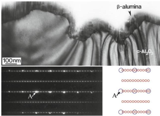
**FIGURE 25.22.** Corrosion of  $\text{Al}_2\text{O}_3$  by reaction with  $\text{K}_2\text{O}$  vapor showing a transmission electron microscopy image, the DP, and a schematic of the DP.
