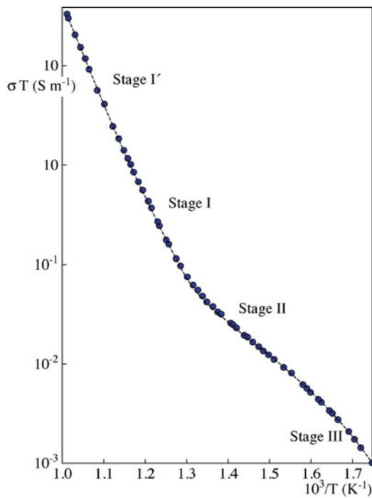
FIGURE 11.16. Ionic conductivity of NaCl varying with  $T^{-1}$ .
