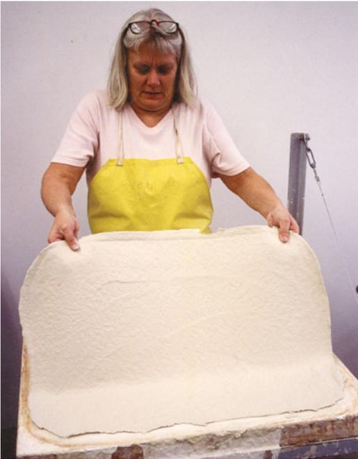
FIGURE 23.17. Removing paper clay from the substrate.
