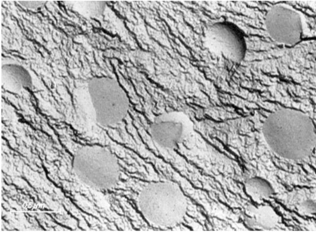
**FIGURE 21.12.** Scanning electron microscopy (SEM) of crystallized glass. The glass is a binary Li-Be fluoride opal glass 40 mol% LiF, 60 mol% BeF<sub>2</sub> containing small amounts of Ag and Ce (0.001 and 0.01 mol%, respectively). The glassy droplets (BeF<sub>2</sub>-rich) are surrounded by crystallized matrix.
