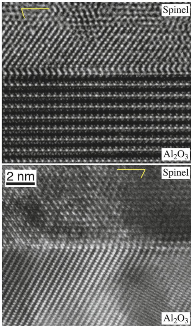
**FIGURE 15.2.** High-resolution transmission electron microscopy (HRTEM) images of two crystallographically different spinel/ $\text{Al}_2\text{O}_3$  PBs. White lines show the {111} planes in the spinel.
