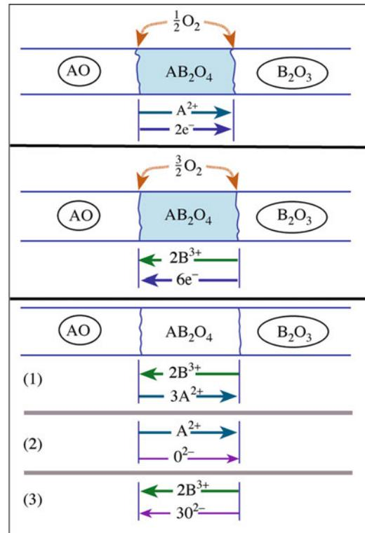
FIGURE 25.12. Mechanisms for the reaction between AO and B<sub>2</sub>O<sub>3</sub>.
