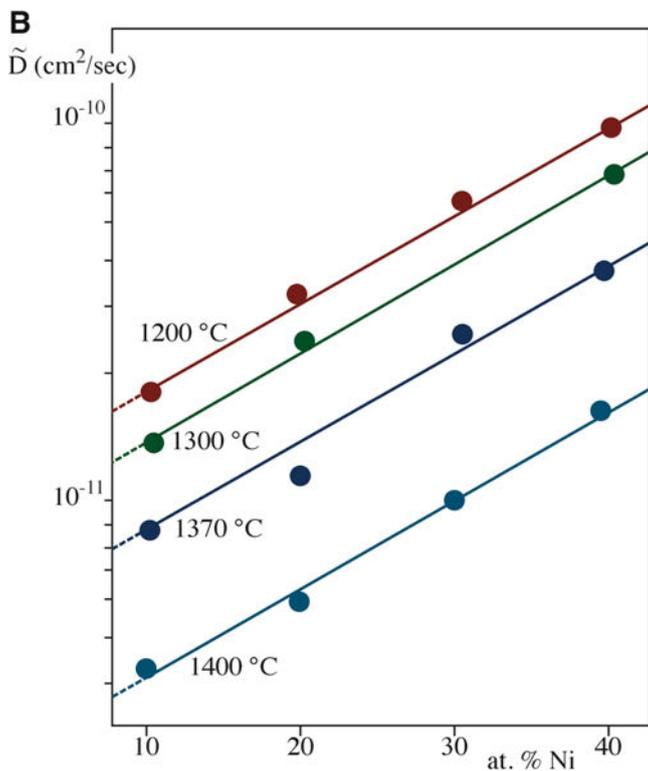
**FIGURE 25.15.**  $D$  as the composition varies. (A) Using tracer diffusion at two values of  $T$  in  $\text{CoO-NiO}$  mixed oxide. (B) Diffusivities for  $\text{MgO-NiO}$  mixed oxides.
