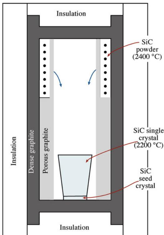
FIGURE 29.18. Modified sublimation process for SiC single crystals.
