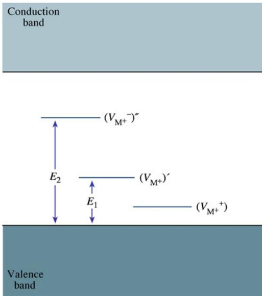
FIGURE 30.15. Energy levels in a deficit semiconductor such as  $\text{Cu}_{2-x}\text{O}$ .
