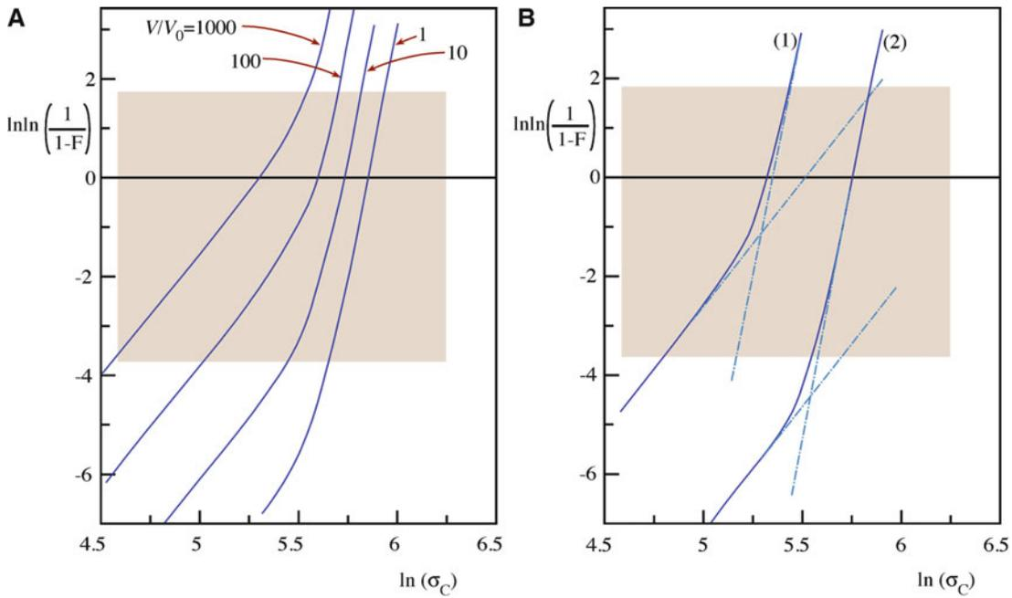
FIGURE 16.24. (A) Different flaws lead to different values of  $m$ . (B) Weibull plot for a sample having both surface and volume flaws.
