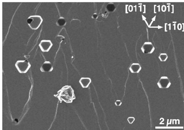
FIGURE 13.2. Faceting of small voids in  $\text{UO}_2$ .
