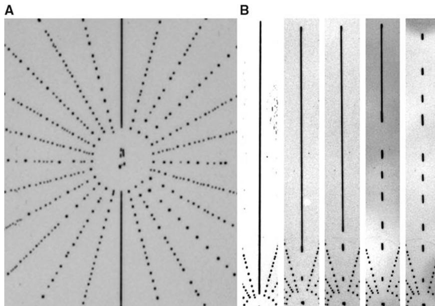
**FIGURE 15.12.** Method for systematically studying voids. (A) Grooves lying along different crystallographic directions break up to form pores at different rates. (B) Breakup of one channel pore can be followed over time.
