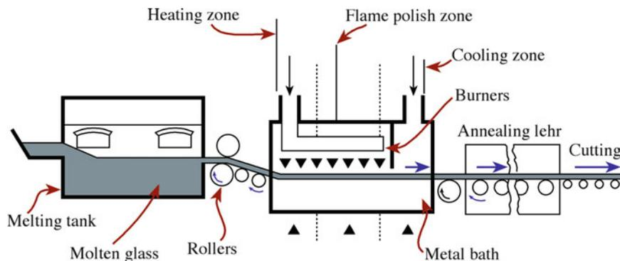
**FIGURE 26.9.** Float glass process.
