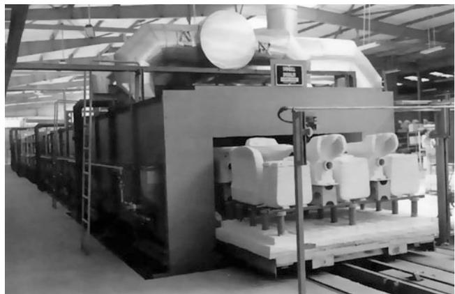
**FIGURE 9.5.** Large continuous furnace used in industry to produce traditional ceramic products and advanced ceramics, such as multilayer chip capacitors.
