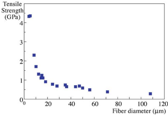
**FIGURE 18.3.** Tensile strength of glass fiber as a function of fiber diameter.
