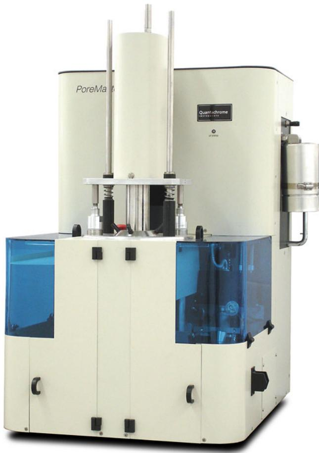
FIGURE 15.13. Commercial porosimeter.
