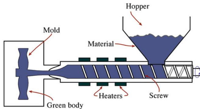
FIGURE 23.12. Cross-sectional side view of a screw-type machine.
