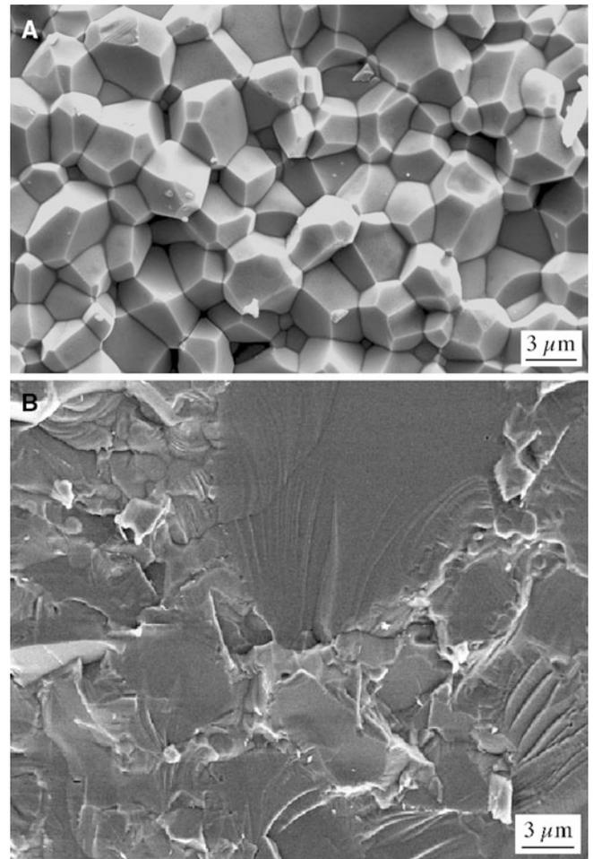
**FIGURE 18.13.** (A) Fracture surface of polycrystalline AlN. (B) Fracture surface of polycrystalline SiC.
