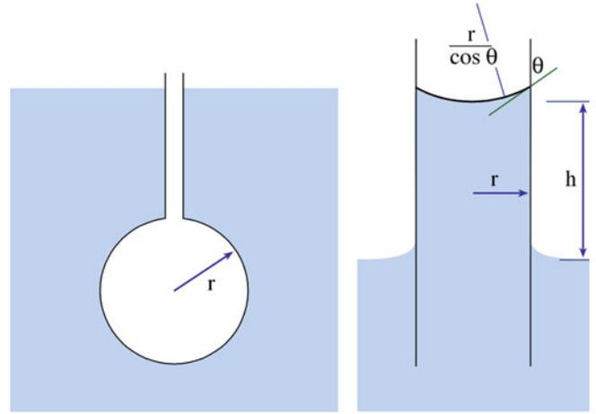
FIGURE 13.8. Geometry used to calculate the capillarity equation.
