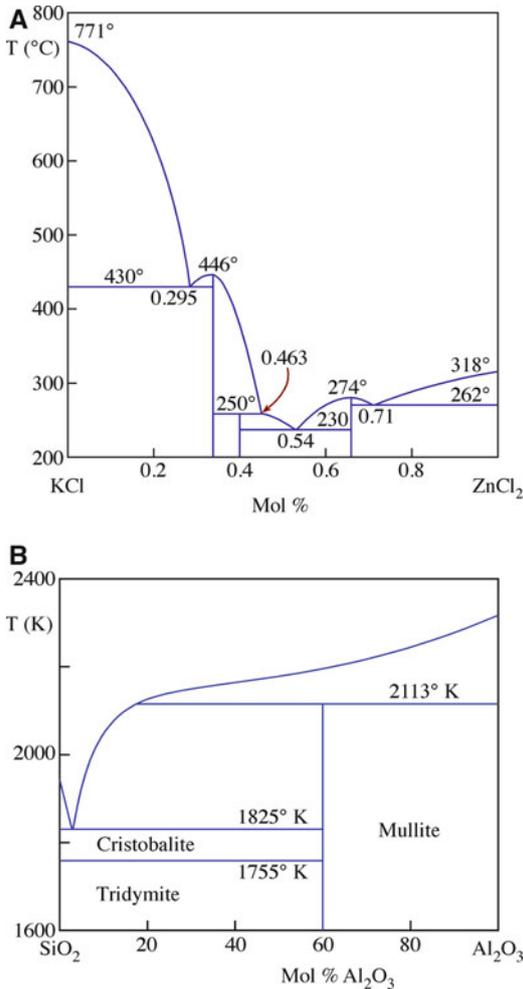
FIGURE 8.5. (a) CALPHAD phase diagram for KCl–ZnCl<sub>2</sub>. (b) CALPHAD phase diagram for SiO<sub>2</sub>–Al<sub>2</sub>O<sub>3</sub>.
