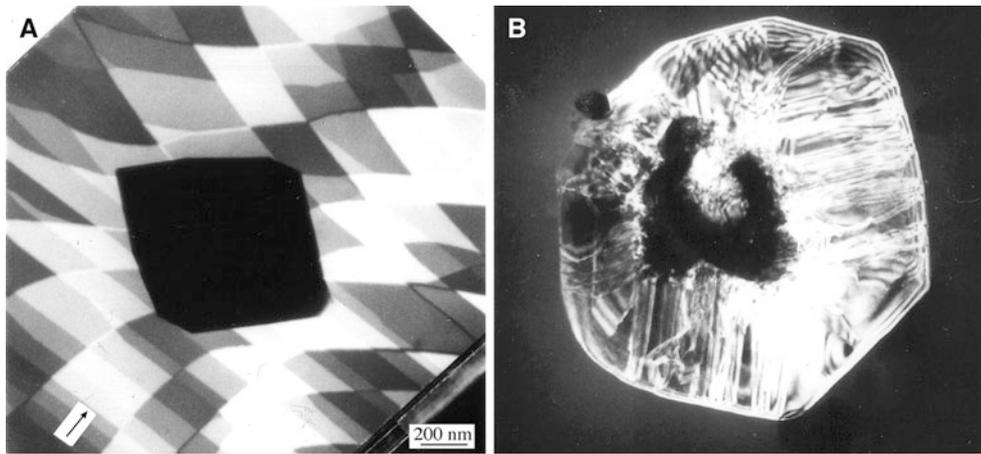
**FIGURE 10.10.** Bright-field (A) and dark-field (B) microscopy (using a spinel reflection) of a particle of NiO on a film of Al<sub>2</sub>O<sub>3</sub> before and after reaction.
