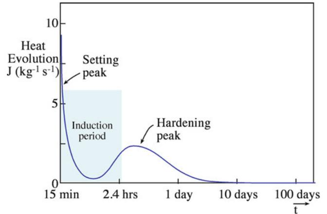
**FIGURE 2.10.** Heat evolution during the setting and hardening of Portland cement.
