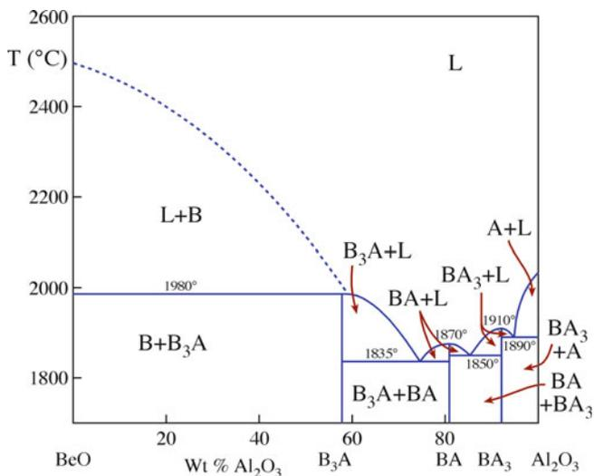
FIGURE 8.13. BeO–Al<sub>2</sub>O<sub>3</sub> phase diagram.
