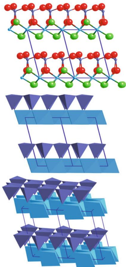
**FIGURE 7.10.** In the crystal structure of kaolinite, the  $\text{SiO}_4$  tetrahedra form one side of the sheet, and the octahedra contain  $\text{OH}^-$  on the outer layer attached to the  $\text{Al}^{3+}$  ions. The sheets are held together only by van der Waals bonds.
