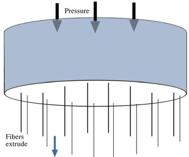
**FIGURE 22.9** Spinnerette used to produce fibers and yarn.
