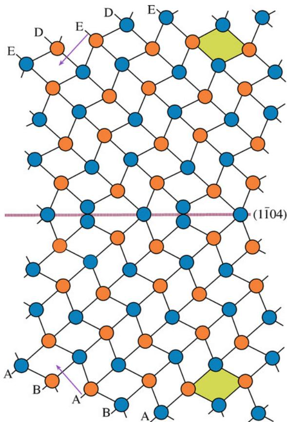
**FIGURE 14.19.** A  $(\bar{1}\bar{1}04)$  twin boundary in Al<sub>2</sub>O<sub>3</sub>. The arrows show the  $\langle 0001 \rangle$  directions; the letters show the hexagonal close-packed (hcp) stacking of the anions. The cations are omitted but sit in the octahedral, shown by the shaded rhombi.
