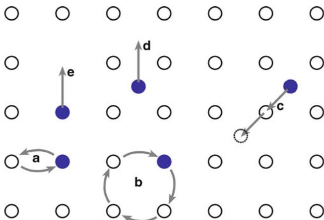
FIGURE 11.10. Possible mechanisms occurring during diffusion. (a) Exchange, (b) ring, (c) knock-on, (d) interstitial, (e) vacancy.
