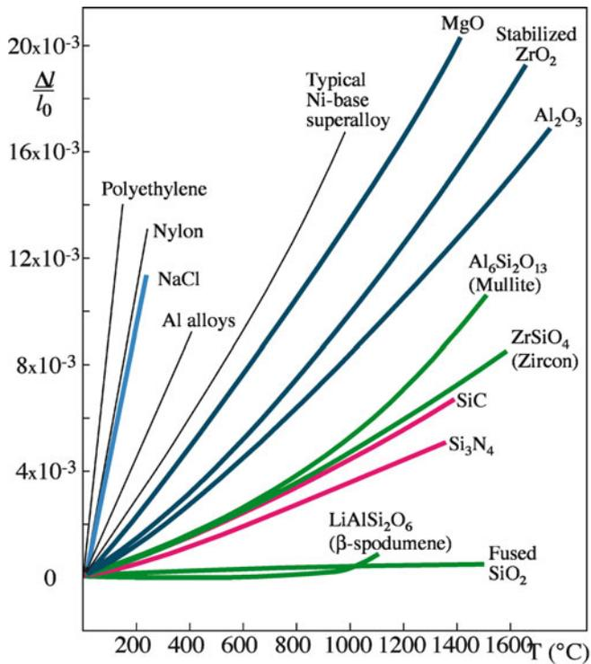
**FIGURE 34.15.** Thermal expansion characteristics of several polycrystalline ceramics.
