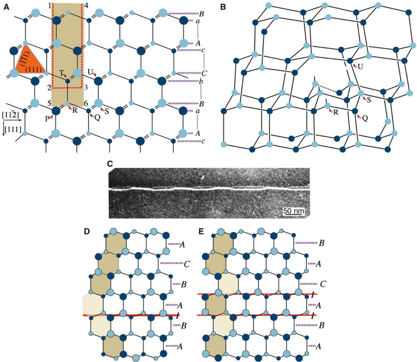
**FIGURE 12.11.** Models for forming dislocations and stacking faults in sphalerite. (A) Two cuts in which to make an edge dislocation. (B) Dislocation made by removing 1234. (C) Dislocation in Si alternating between a compact core and a dissociated structure. (D, E) Intrinsic and extrinsic SFs in Si.
