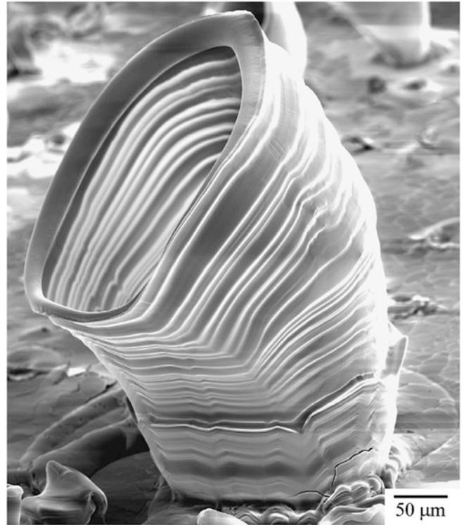
FIGURE 17.22. Microblown silica shape formed on oxidized SiC.
