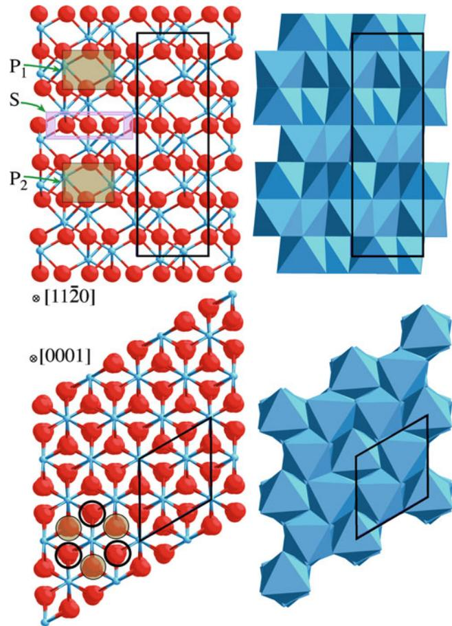
**FIGURE 6.12.** Sapphire crystal structure. (Top)  $[11\bar{2}0]$  view. (Bottom)  $[0001]$  view. (Left) Atomic models. (Right) Stacking octahedra.  $P_1$  and  $P_2$  are two unoccupied octahedra. S is a triangle of more closely spaced  $O^{2-}$  ions. Open circles (lower left) show AB stacking of the anions. The unit cell is outlined for both projections.
