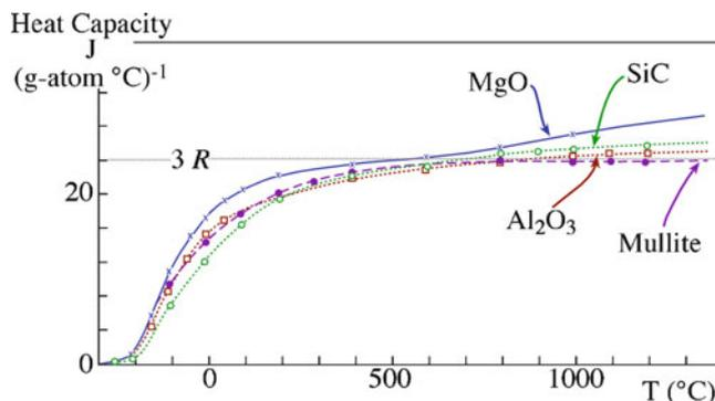
**FIGURE 34.1.** Heat capacity of some ceramics as a function of temperature.
