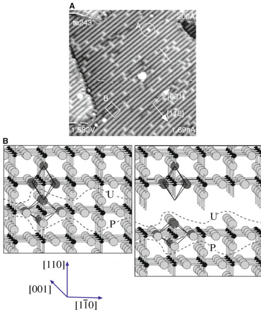
**FIGURE 10.14.** STM image of the (110) surface of  $\text{TiO}_2$ . The features labeled “A” have been assigned as oxygen vacancies; the features labeled “B” have not been identified. The model shows how such a surface can be formed. The dashed lines indicate where the ‘break’ can occur. Large spheres are the O anions.
