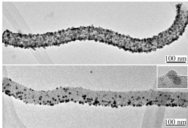
**FIGURE 15.23.** Au catalyst particles on a ceramic nanowire.
