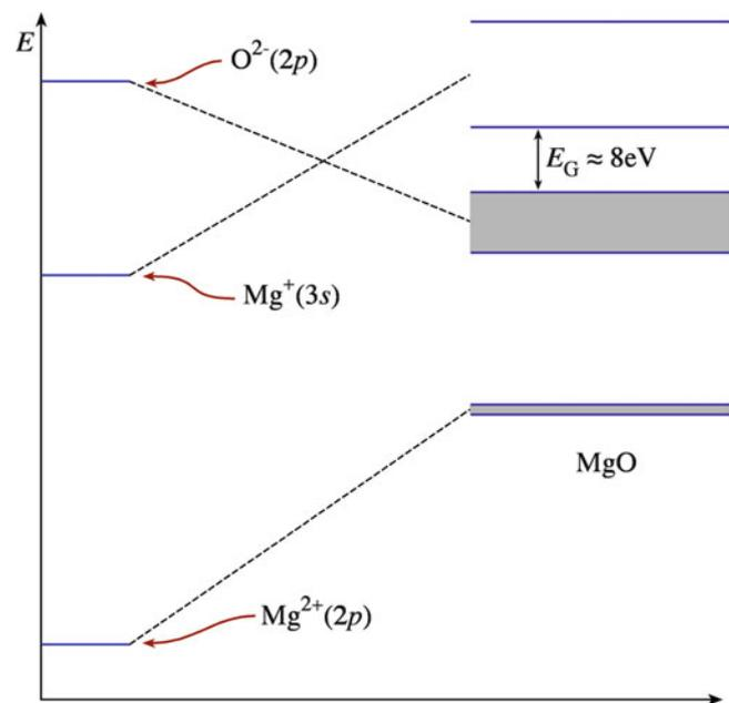
FIGURE 30.23. Energy band diagram for  $\text{MgO}$ .
