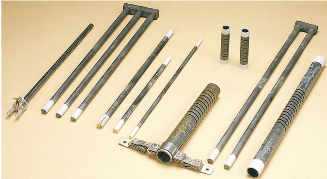
FIGURE 9.7. Examples of SiC furnace elements.
