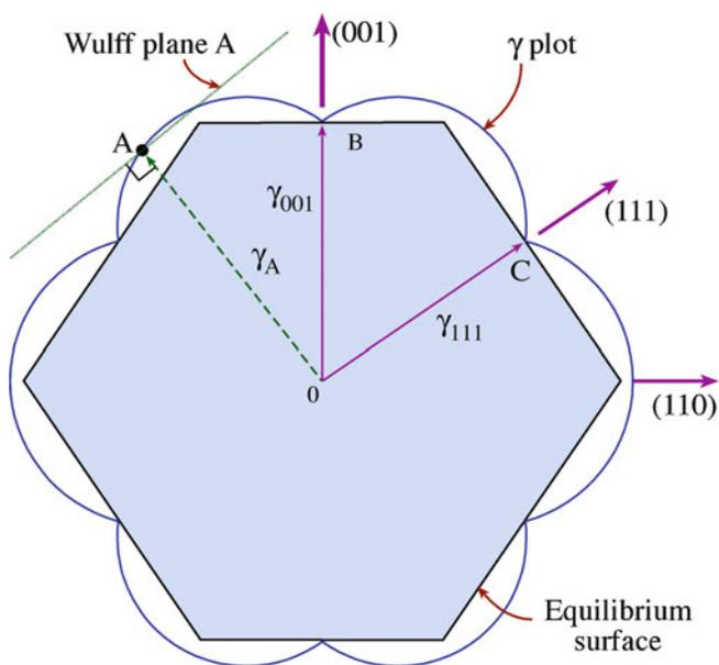
FIGURE 13.1. Wulff plot looking along the  $[1\bar{1}0]$  direction for a face-centered cubic (fcc) crystal.
