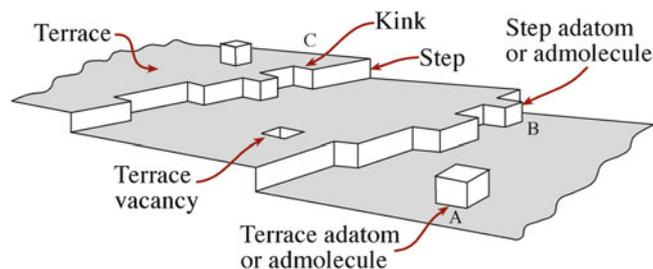
**FIGURE 13.13.** Surface attachment sites and the nucleation of thin films in 2D.
