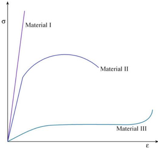
FIGURE 16.2. Idealized stress–strain curves for different materials classes.
