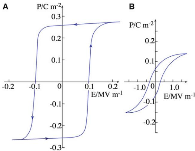
**FIGURE 31.10.** Hysteresis loops for BaTiO<sub>3</sub>. (A) Single-domain single crystal. (B) Polycrystalline ceramic.
