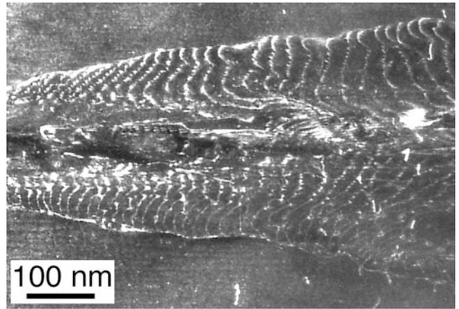
FIGURE 25.6. Movement of interfacial dislocations between hematite and NiFe<sub>2</sub>O<sub>4</sub> spinel during oxidation, leading to thickening of the precipitate.
