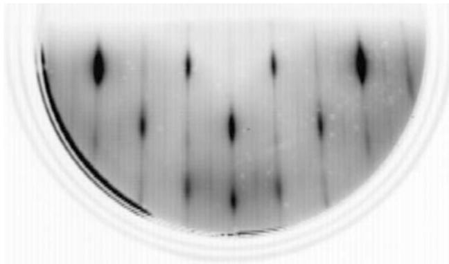
**FIGURE 13.19.** Reflection high-energy electron diffraction (RHEED) pattern from anatase film grown on  $\text{LaAlO}_3$ .
