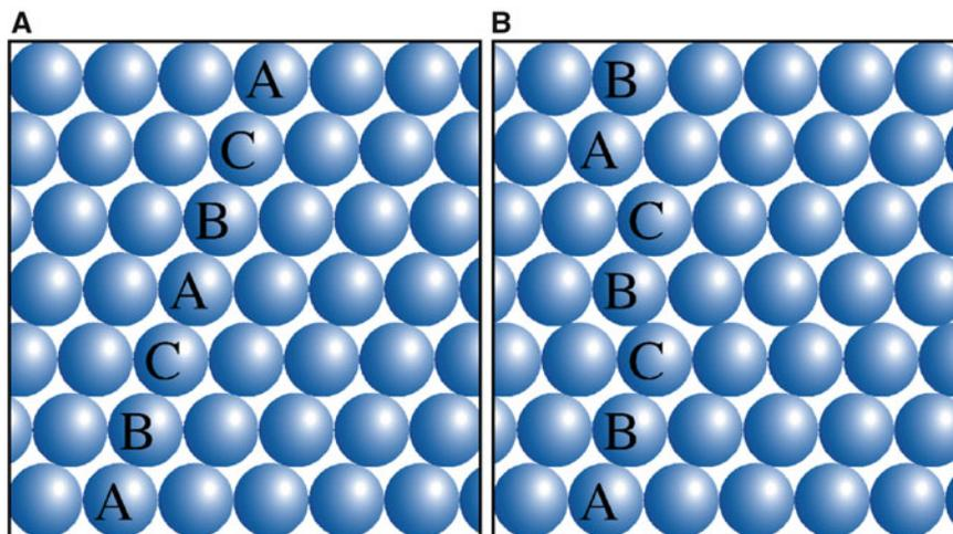
FIGURE 12.6. Intrinsic stacking fault in a face-centered cubic (fcc) crystal.
