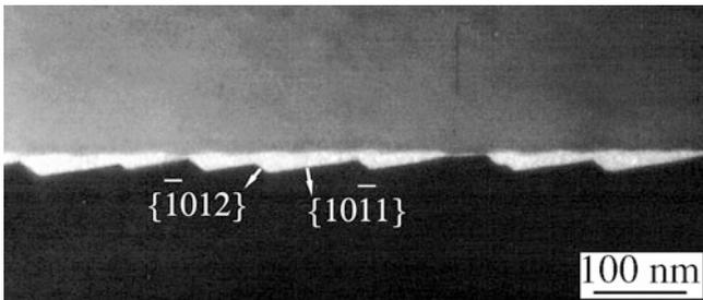
**FIGURE 14.30.** Intergranular film in Al<sub>2</sub>O<sub>3</sub> that was initially uniformly thick but varied in thickness after heat treatment.
