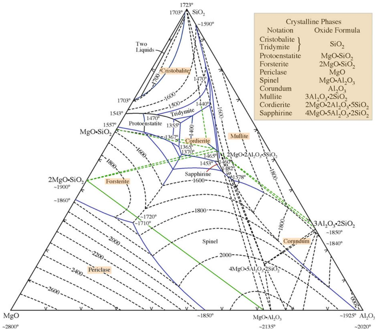
FIGURE 8.16. The MgO–Al<sub>2</sub>O<sub>3</sub>–SiO<sub>2</sub> phase diagram.
