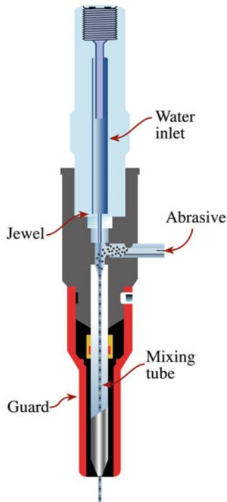
FIGURE 23.16. Abrasive waterjet cutting process.
