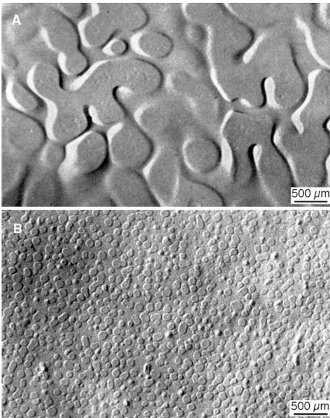
**FIGURE 21.13.** SEM images of (A) Na-Be and (B) K-Be fluoride glass 15 mol% KF (or NaF), 85 mol% BeF<sub>2</sub>. This glass is cloudy; if the droplets were smaller, the glass would be clear. Replacing K by Rb actually reduced the droplet size to 10–20 nm.
