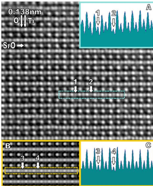
**FIGURE 10.11.** High-resolution (HR) TEM image of the structure of SrTiO<sub>3</sub>.
