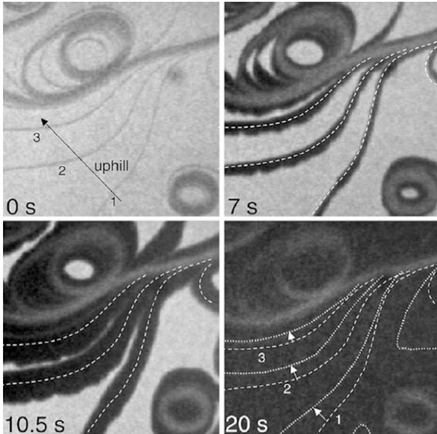
**FIGURE 13.24.** Studies of changes occurring at the surface of  $\text{TiO}_2$  using low-energy electron microscopy (LEEM). A total of 20 s separates the four images. The different contrast occurs because of the surface reconstruction.
