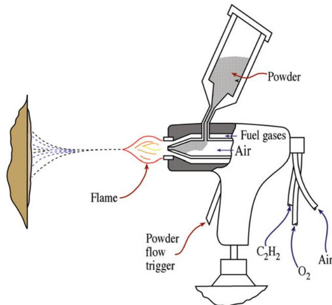
FIGURE 27.8. Thermal spraying with a gas combustion/powder gun.
