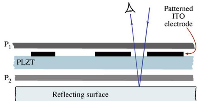
FIGURE 32.24. Basic layout of a PLZT reflective display.
