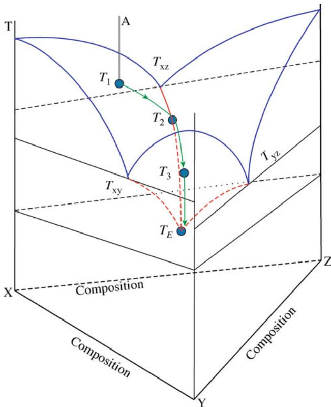
FIGURE 8.19. Cooling path in a ternary system.
