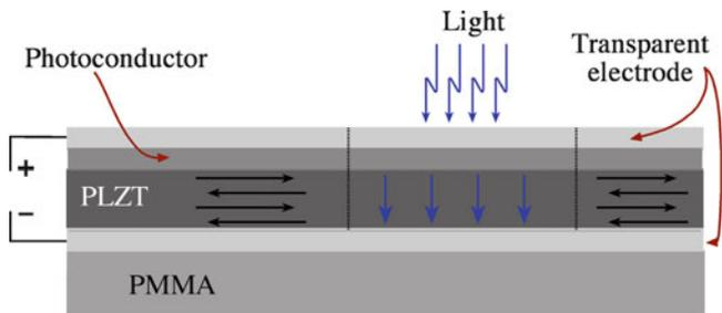
FIGURE 32.25. Image storage device using a field-induced polarized PLZT film.
