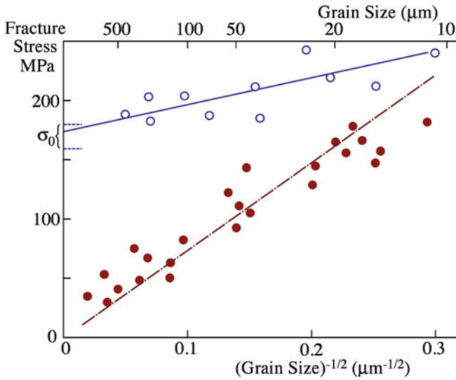
FIGURE 1.2. Dependence of fracture strength of MgO (at 20°C) on grain size.
