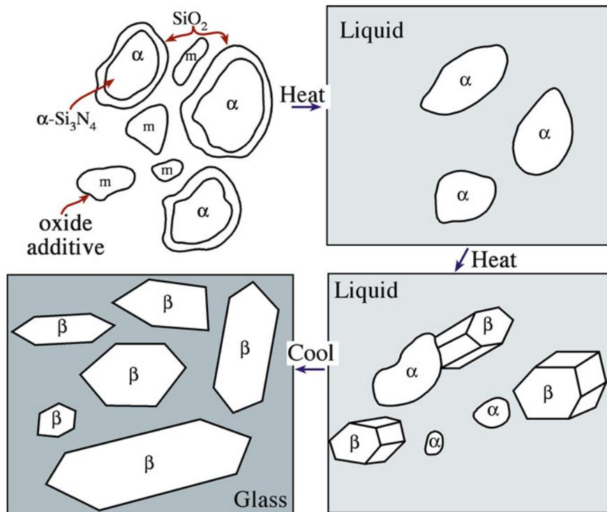
**FIGURE 38.1.** Schematic showing processing steps in forming  $\text{Si}_3\text{N}_4$  by LPS. The metal oxide additive (m) would be something like  $\text{Y}_2\text{O}_3$  and the liquid an oxynitride/silicate.
