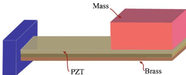
FIGURE 37.12. Cantilever piezoelectric generator.
