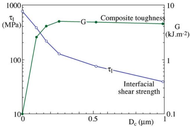
**FIGURE 20.16.** Effect of carbon coating thickness ( $D_c$ ) on the mechanical properties of Nicalon™ fibers in a SiC matrix. Interfacial shear strength was measured by push-down testing and toughness from the area under the stress–strain curve during loading along the fiber axis.
