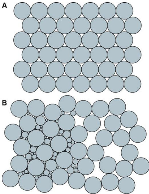
**FIGURE 24.1.** Model grain/shape distributions in two dimensions. Packing identical spheres can never achieve less than 26% porosity. (A) Ideal planar packing. (B) Less-dense packing of larger spheres, some with inserted smaller spheres giving a higher local density.
