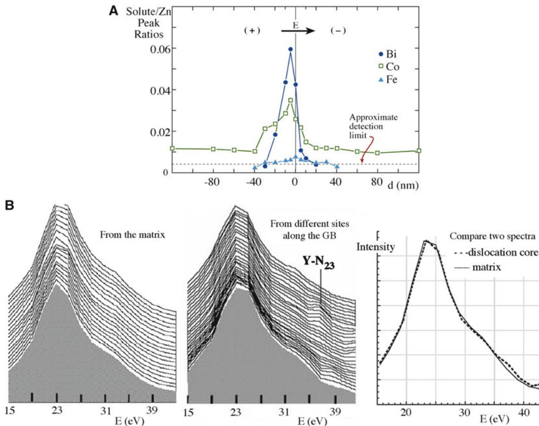
**FIGURE 14.2.** Solute distribution at GBs. (A) Profiles using X-ray energy dispersive spectroscopy (XEDS). The integrated X-ray solute/Zn peak ratios are plotted against the distance,  $d$ , from the GB. (B) Electron energy loss spectroscopy (EELS) spectra used to analyze a GB in sapphire.
