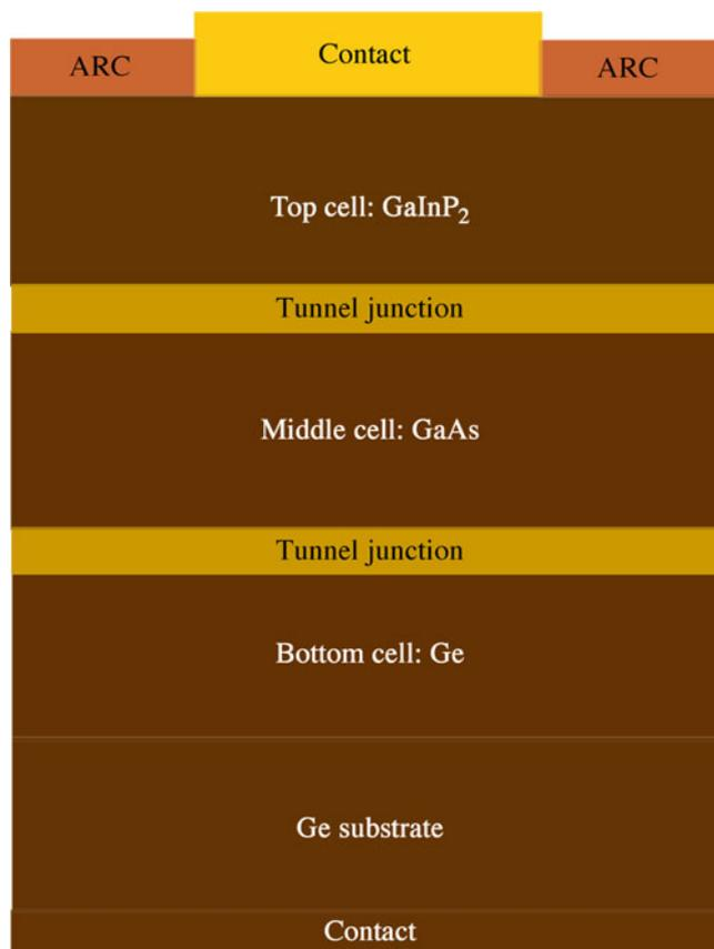
FIGURE 37.4. Spectrolab multijunction solar cell. Sizes up to 32 cm<sup>2</sup> are possible with this structure.
