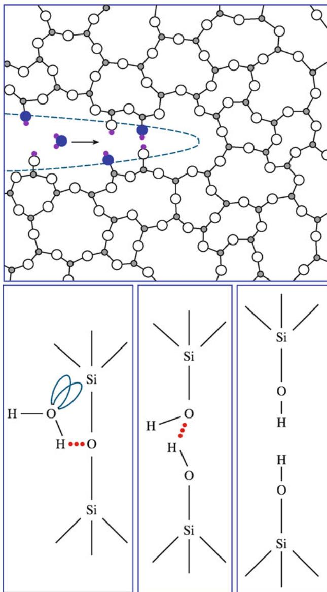
**FIGURE 18.10.** Environmental effects at the crack tip. A water molecule diffuses to the crack tip, chemisorbs, and rotates such that the lone pairs on the oxygen are aligned with the unoccupied electron orbitals of the Si atom.
