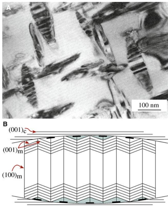
FIGURE 25.5. Twins in transformed particles. (A) Experimental observation. (B) A possible mechanism.
