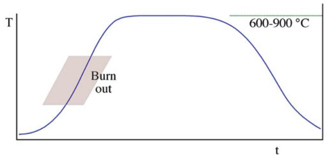
**FIGURE 27.16.** Typical thick film circuit firing profile.
