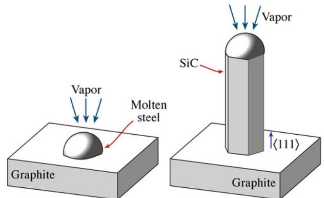
FIGURE 29.17. Vapor-liquid-solid (VLS) process for growing SiC whiskers.
