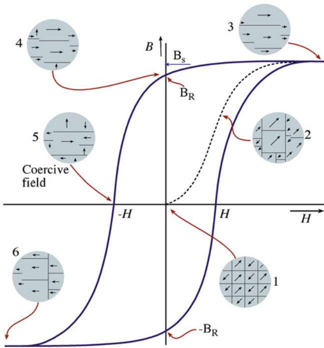
**FIGURE 33.22.** Variation of  $B$  as  $H$  alternates. Insets. Domain structure at various points along the hysteresis curve.
