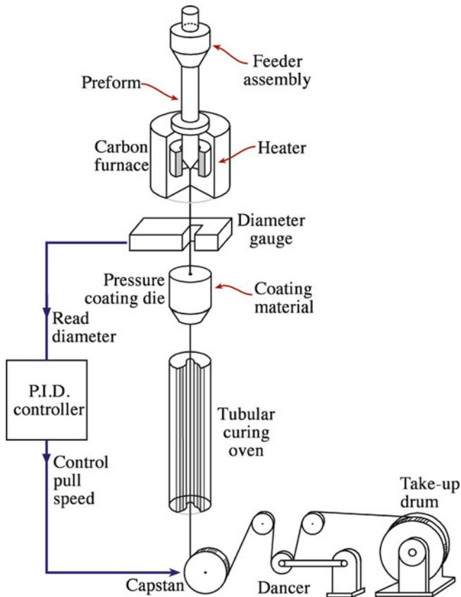
FIGURE 32.17. Fiber drawing tower.
