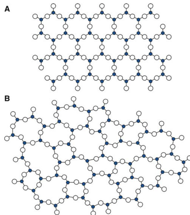
**FIGURE 7.19.** Comparing the structures of (a) crystalline silica and (b) glass.
