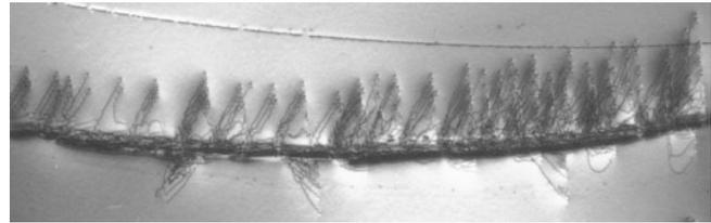
**FIGURE 12.26.** Dislocations produced by scratching  $\text{Al}_2\text{O}_3$ .
