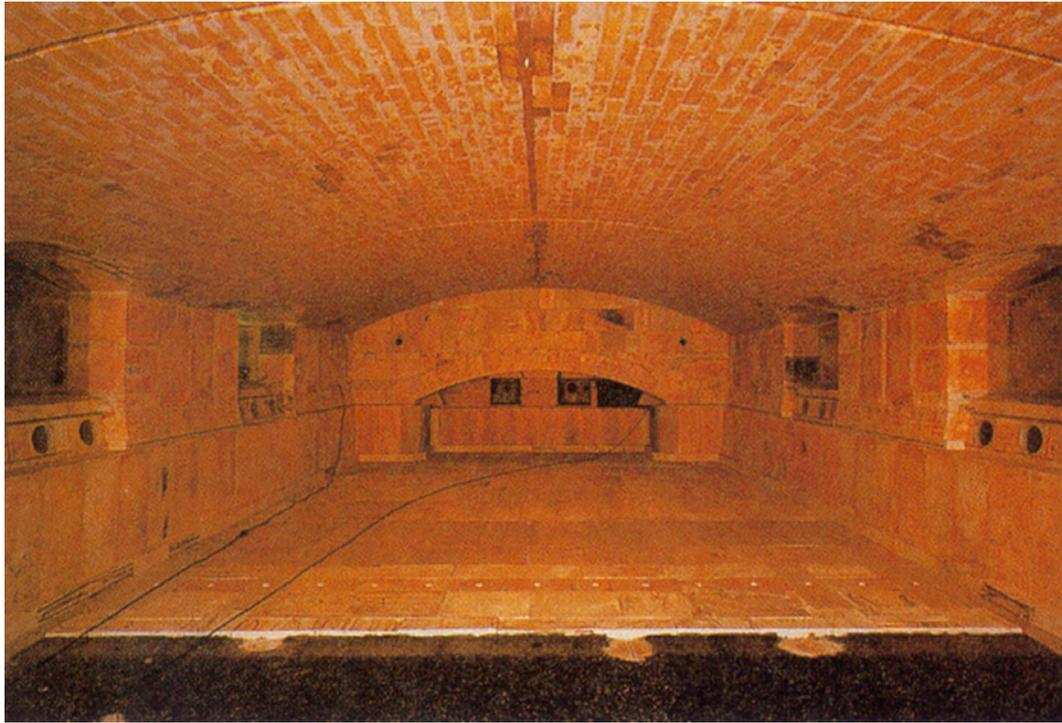
FIGURE 26.2. Inside a typical glass-melting tank.
