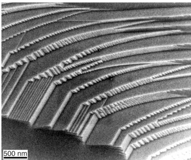
**FIGURE 10.6.** Secondary electron (SE) image shows steps on an alumina surface.
