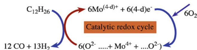
FIGURE 37.3. Mars-van Krevelen mechanism.
