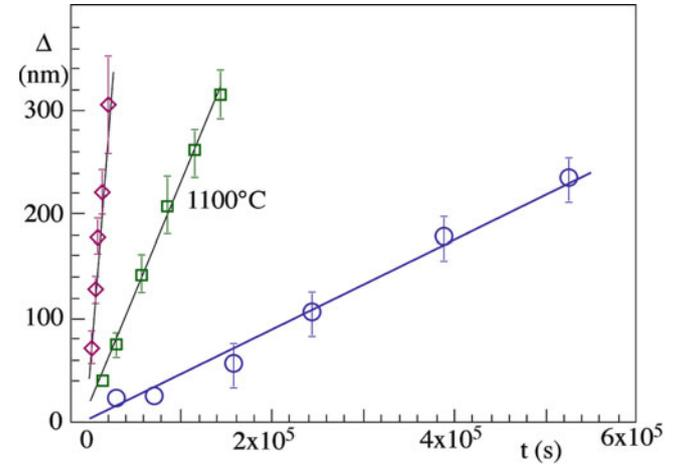
**FIGURE 25.20.** Kinetics of reactions between thin films of NiO deposited on (0001)  $\text{Al}_2\text{O}_3$  when an initial buffer layer of spinel is present.
