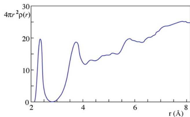
**FIGURE 7.18.** Radial distribution function of a glass showing a sharp first-neighbor peak, a broader second-neighbor peak, and then a gradual increase with increasing  $r$ .
