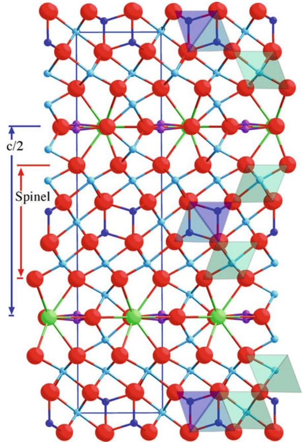
**FIGURE 7.12.** Crystal structure of  $\beta$ -alumina. The main features are the large value of  $c$ , the twinned spinel blocks, and the mirror plane containing the  $\text{Na}^+$  (or  $\text{K}^+$  or  $\text{Ca}^{2+}$ ) ion.
