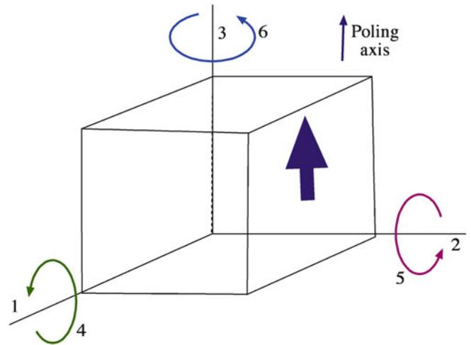
FIGURE 31.19. Notation of axes for piezoelectric ceramic.
