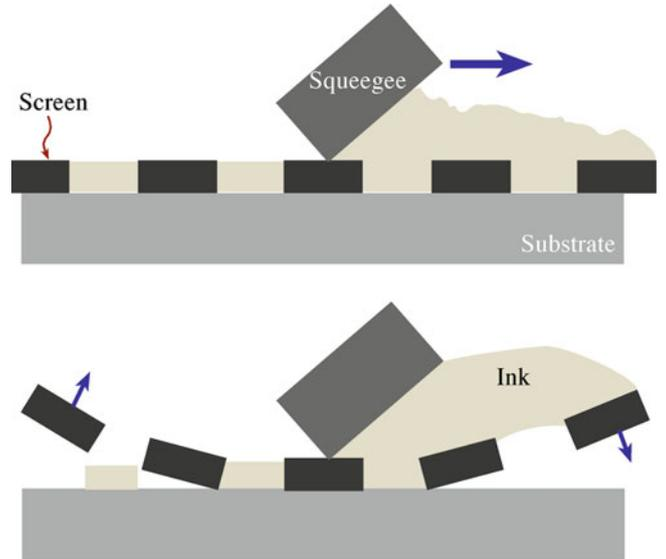
**FIGURE 27.15.** Screen-printing process for depositing thick film circuits. The ink is forced through the screen, which then snaps away, leaving a film on the substrate.
