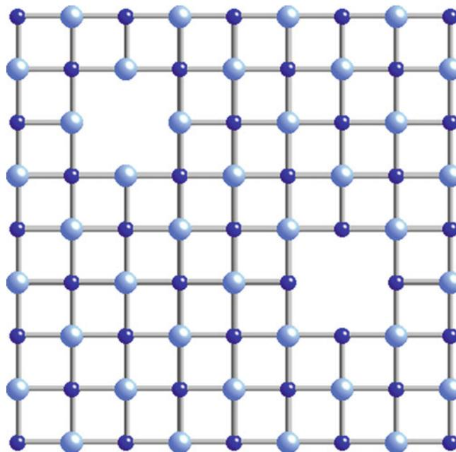
FIGURE 11.1. Schottky defect drawn in two dimensions.
