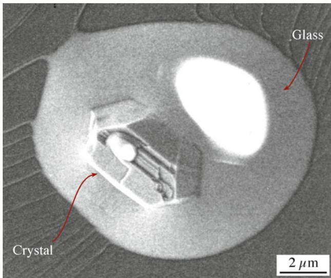
FIGURE 21.9. Example of crystallization in a glass droplet.
