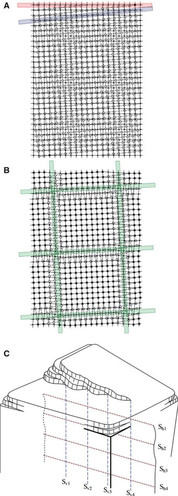
**FIGURE 14.5.** Low-angle twist GB. (A) Before and (B) after local atomic relaxations. (C) The twist when the GB emerges at the surface.
