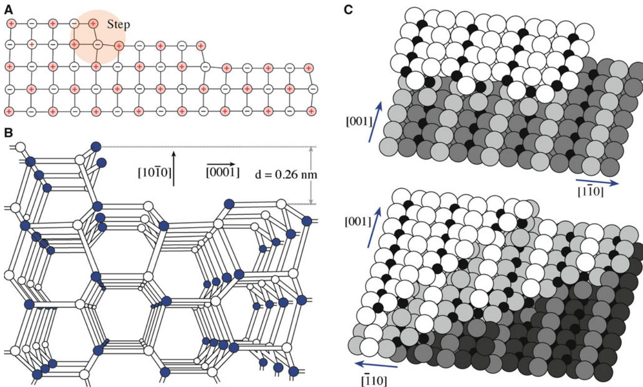
FIGURE 13.23. Representations of surface steps. (A) MgO (100) cross section. (B) Wurtzite. (C) (110) TiO<sub>2</sub>.
