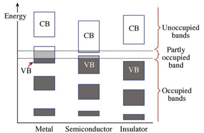
FIGURE 30.2. Electron energy bands in solids. The valence band (VB) and conduction band (CB) are indicated.
