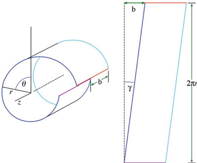
FIGURE 12.4. Deducing strain by “unwrapping” a screw dislocation.
