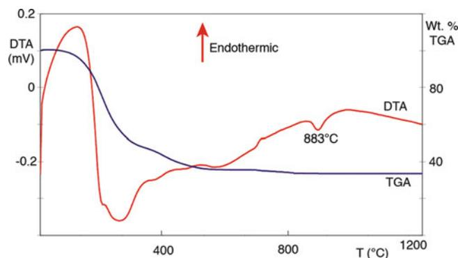
FIGURE 10.37. Differential thermal analysis (DTA) and thermogravimetric analysis (TGA) measurements show the reaction as CA $_2$  crystallizes.
