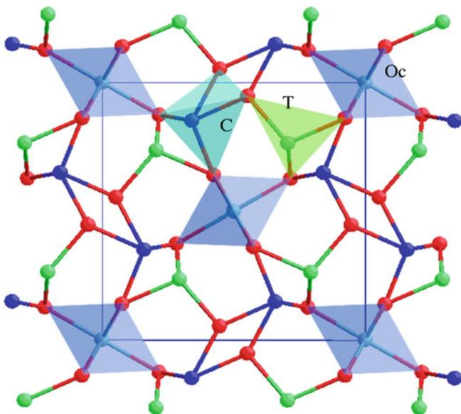
**FIGURE 7.13.** Crystal structure of mullite viewed along the short  $z$  axis ( $a = 0.76$  nm,  $b = 0.77$  nm,  $c = 0.29$  nm). The sites Oc and T are never fully occupied, so this is an idealized schematic of this orthorhombic orthosilicate. The chains of octahedra at the corners and center lie along  $z$ .
