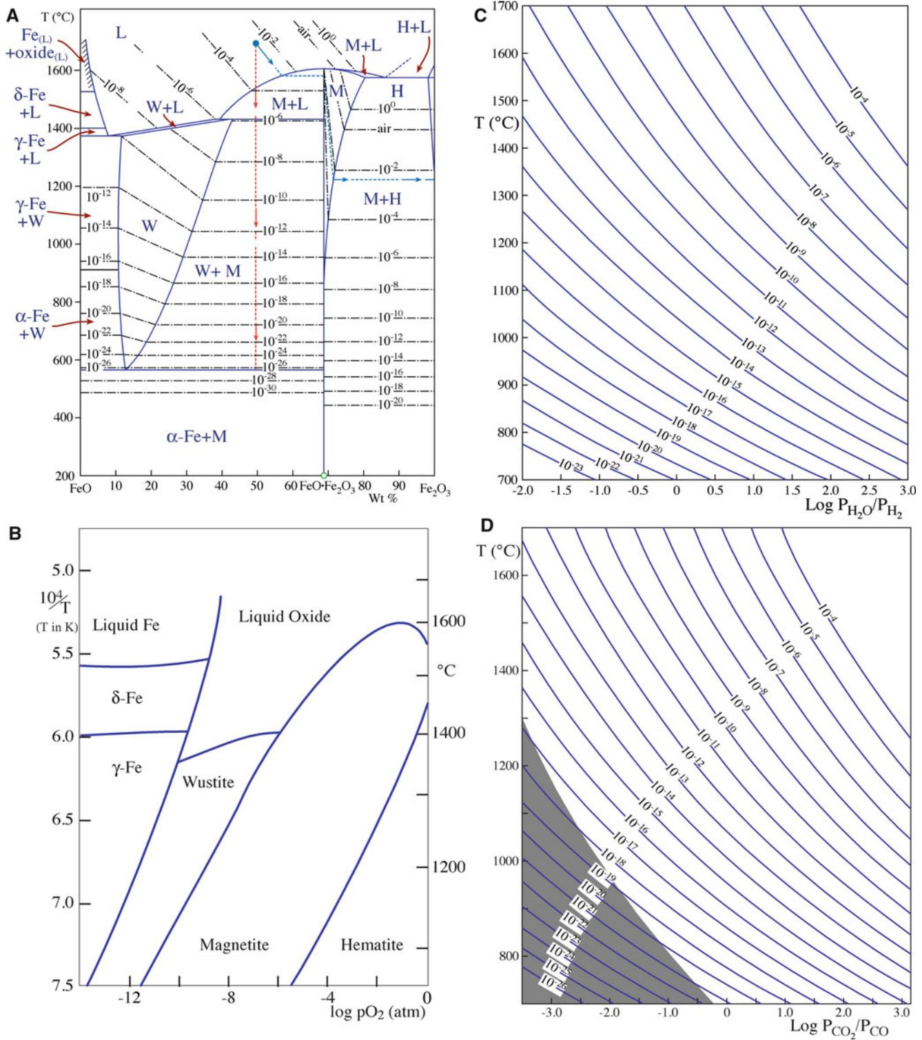
FIGURE 8.20. (a, b) The FeO–Fe<sub>2</sub>O<sub>3</sub> phase diagram; (c) the H–O system; (d) the C–O system.
