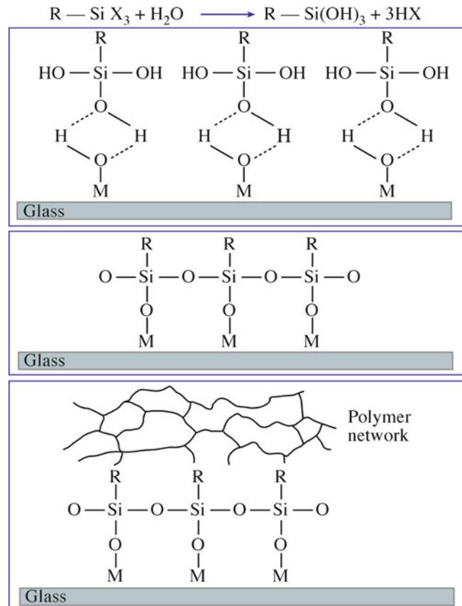
**FIGURE 20.17.** Processes involved in joining a polymer and glass using silane coupling agents. (A) Hydrolysis of the silane to the corresponding silanol. (B) Hydrogen bonding between hydroxyls on the silanol and those attached to the glass. (C) Polysiloxane bonded to the glass following condensation during drying. (D) Bonding between the functional group R and the polymer.
