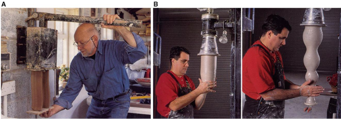
FIGURE 23.11. Extruding clay. Manual and electric extruders.
