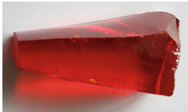
FIGURE 36.28. As grown crystal of rare-earth-doped cubic zirconia.
