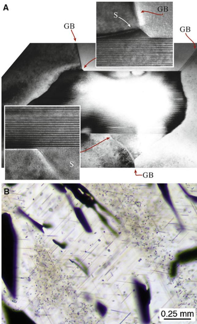
**FIGURE 15.6.** Particle in a matrix. (A) TEM image of a second-phase  $\beta\text{-Al}_2\text{O}_3$  growing along a grain boundary (GB) in  $\alpha\text{-Al}_2\text{O}_3$ . The insets show spinel (S) growing up the GBs. (B) Visible light microscopy (VLM) of rutile needles growing in a garnet grain.
