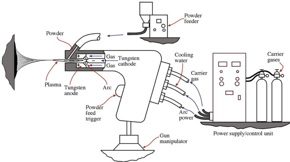
FIGURE 27.9. Thermal spraying using a plasma arc.
