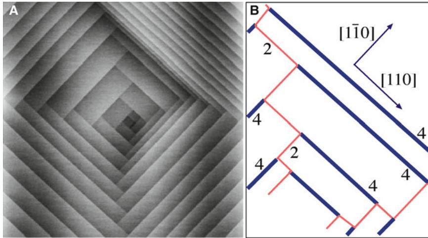
**FIGURE 13.4.** Faceted shallow thermal etch pit on the (001) surface of spinel. Numbers 2 and 4 refer to the height of the steps (0.2 and 0.4 nm, respectively).
