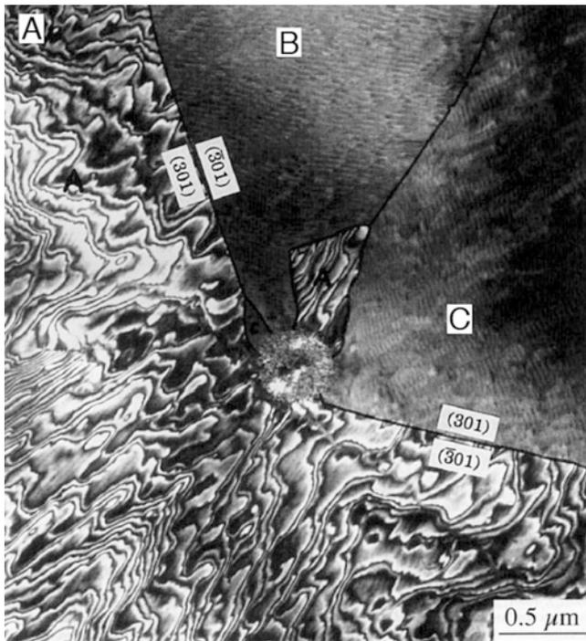
**FIGURE 14.36.** Example of GBs in thin films of anorthite on  $\text{Al}_2\text{O}_3$ . The three grains correspond to three epitaxial orientations, but only one shows the misfit dislocations in this TEM image.
