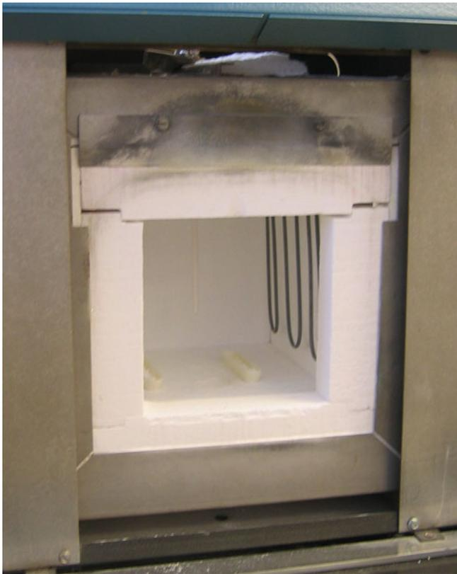
**FIGURE 9.2.** Small electrically heated box furnace.
