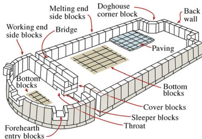
**FIGURE 9.9.** Layout of refractories in an industrial glass melting furnace.
