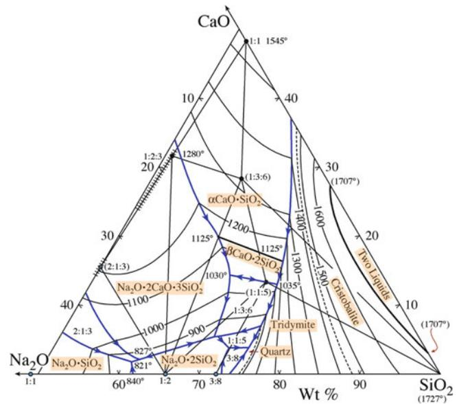
FIGURE 8.18. Na<sub>2</sub>O–CaO–SiO<sub>2</sub> phase diagram.
