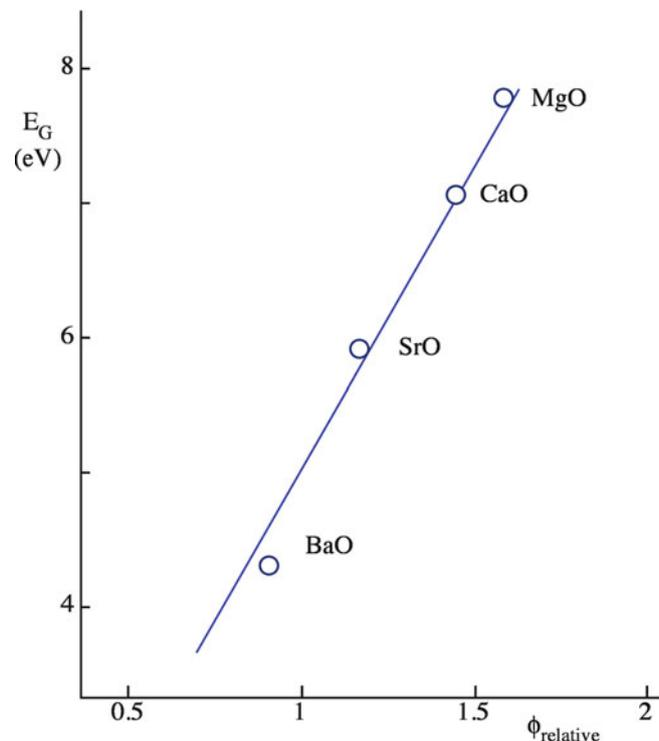
FIGURE 30.24. Effect of bond ionicity on  $E_g$  for metal oxides  $\text{MO}$  ( $\phi = Z/r$ ).
