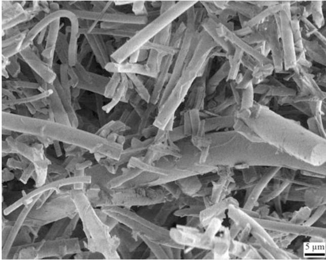
**FIGURE 15.16.** Porous material used to make insulating tiles for the space shuttle.
