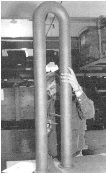
**FIGURE 24.2.** Radiant U tube produced by sintering SiC.
