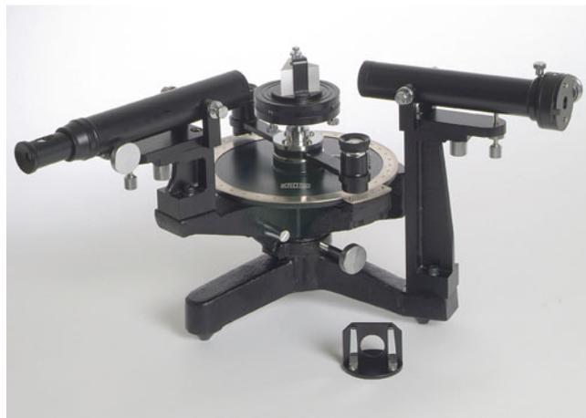
**FIGURE 36.7.** Goniometer-style refractometer.
