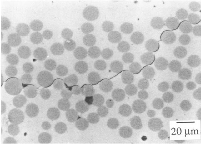
**FIGURE 38.7.** Crack propagation through a fiber-reinforced composite: SiC fiber in calcium aluminosilicate glass.
