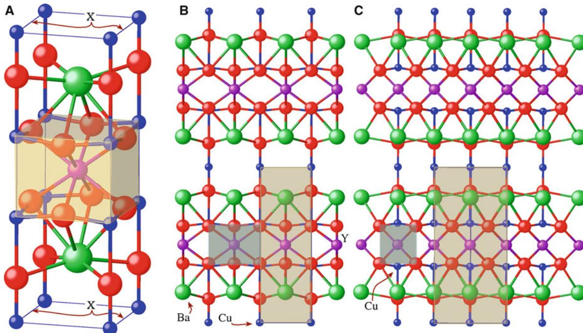
**FIGURE 7.14.** Models for YBCO. (A) Unit cell for the fully oxygenated compound (with ...O<sub>7</sub>); the shaded region shows the perovskite unit with Y in the center and Cu at the corners. (B, C) The structure is more readily appreciated from (B) [100] and (C) [110] views, each showing six unit cells. Note how the perovskite “unit cell” is rotated 45° relative to the unit cell of the YBCO.
