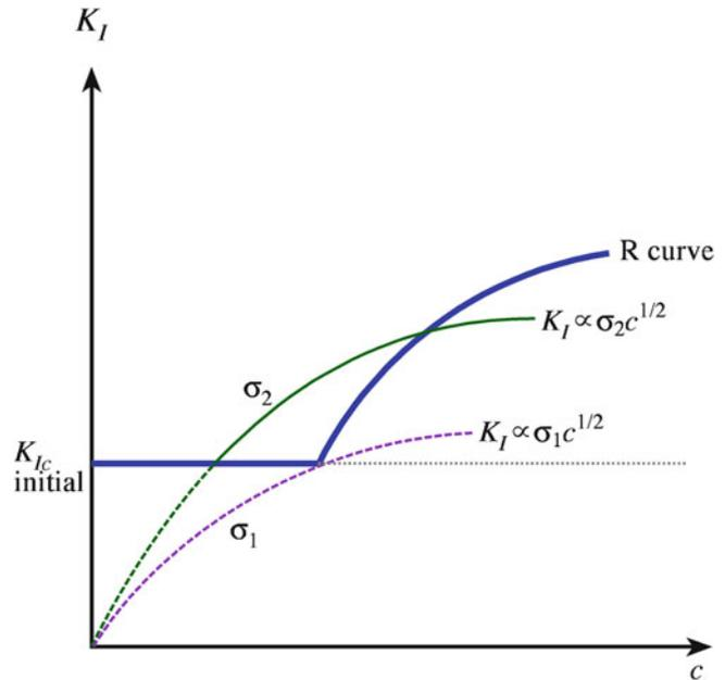
**FIGURE 18.7.** A material showing  $R$  curve behavior (bold curve) exhibits a region with stable crack growth and flaw-tolerant behavior. The lighter curves,  $\sigma_1$  and  $\sigma_2$ , represent typical Griffith behavior.
