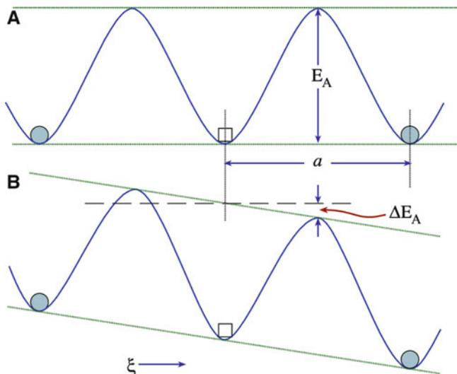
**FIGURE 30.20.** Potential energy barrier to ion movement. (A) In the absence of an applied field. (B) With an applied field.  $E_A$  is the activation energy, and  $a$  is the jump distance between ion sites.
