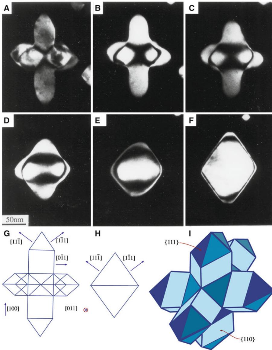
**FIGURE 15.5.** Spinel particles changing shape in NiO due to heat treatment. (Image formed as for Figure 15.4.) (A) Looking along [011]. Thirty-min heat treatment between images. (B) 800°C. (C) 825°C. (D) 850°C. (E) 875°C. (F) 900°C. The shape change is summarized in the schematics. The three-dimensional figure shows the original shape.
