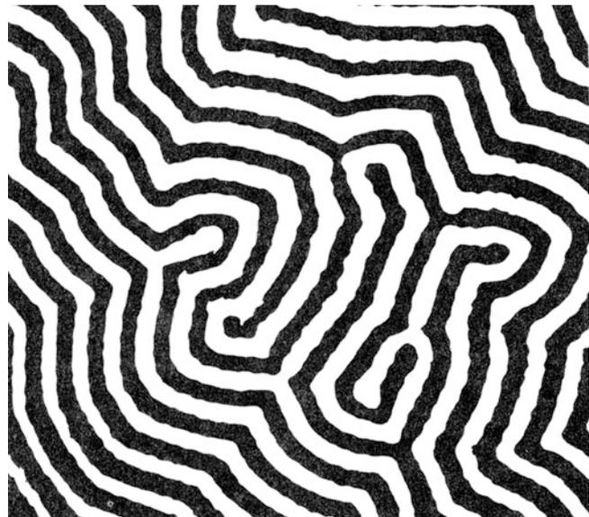
**FIGURE 33.19.** Domain pattern in a YIG thin film revealed by the Faraday effect.
