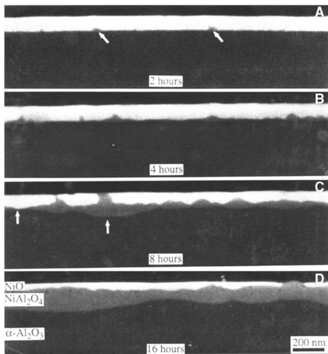
**FIGURE 25.18.** SEM images of reactions at grain boundaries (GBs) in thin films of NiO deposited on (0001)  $\text{Al}_2\text{O}_3$ .
