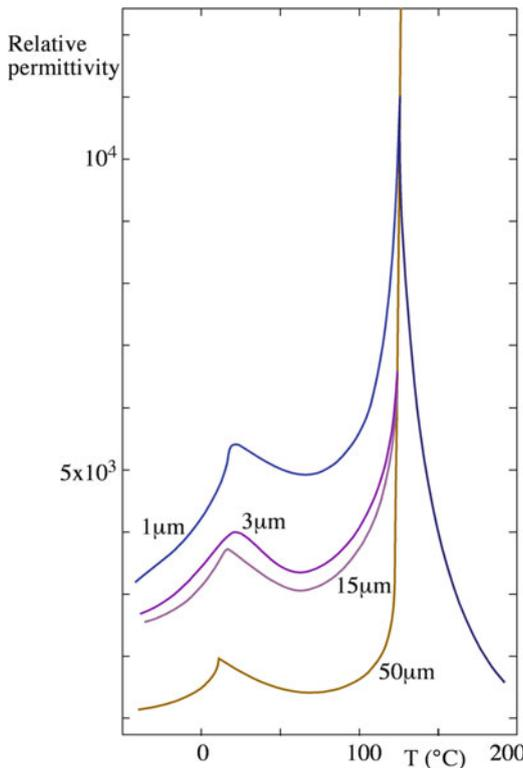
**FIGURE 31.15.** Effect of grain size on the dielectric constant of BaTiO<sub>3</sub>.
