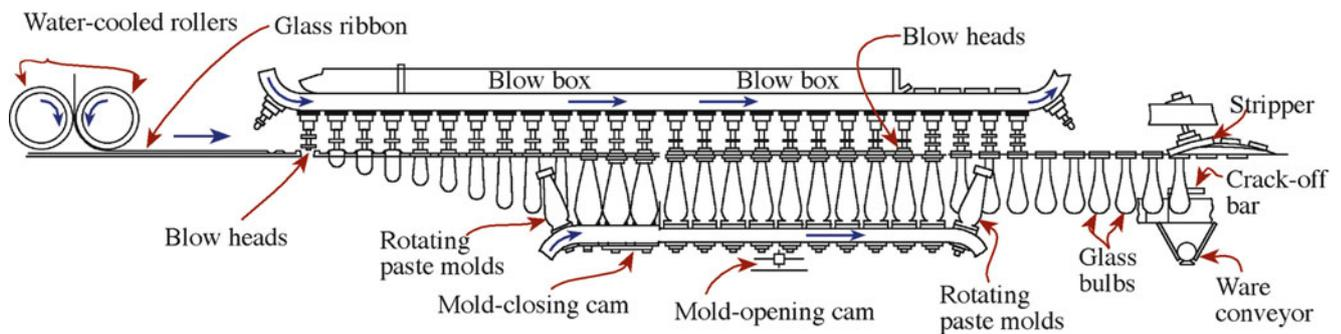
**FIGURE 26.12.** Corning ribbon machine for glass lamp bulbs.
