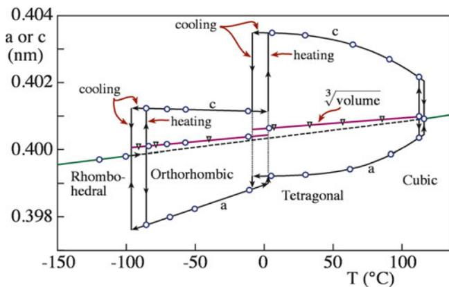
FIGURE 31.9. Experimental measurements of lattice parameters of BaTiO<sub>3</sub> as a function of temperature. (Note the change in volume at each transition and the hysteresis in the lattice parameters).
