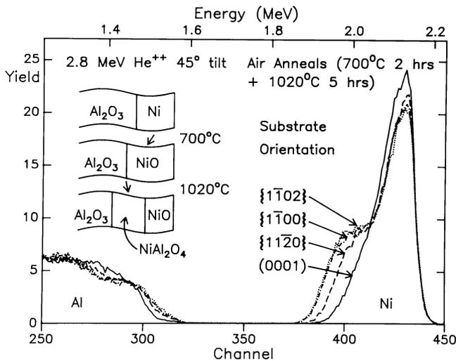
**FIGURE 25.10.** Rutherford backscattering spectrometry (RBS) of a reaction between NiO and Al<sub>2</sub>O<sub>3</sub> substrates for different surface orientations.
