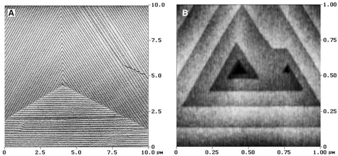
**FIGURE 10.16.** AFM image showing long (up to 10  $\mu\text{m}$ ) straight steps on the surface of an Mg–Al spinel. The steps are 0.4 nm high. The lower image shows the central region at higher magnification.
