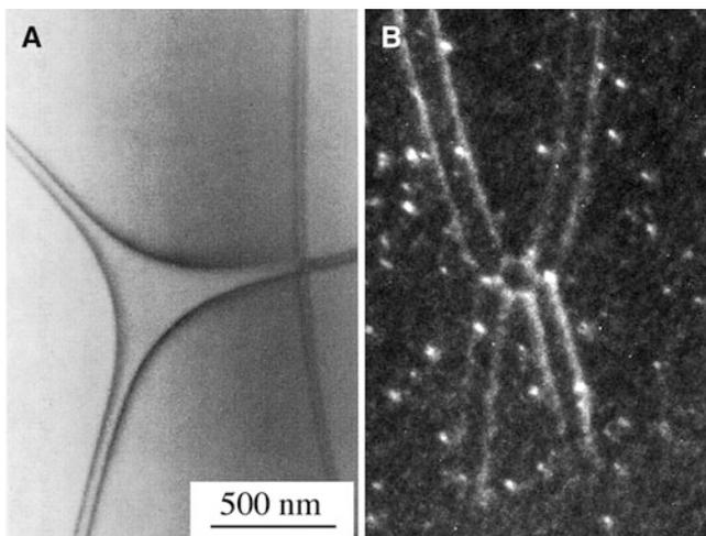
FIGURE 12.23. Dislocation nodes. (A) AlN. (B) Spinel.
