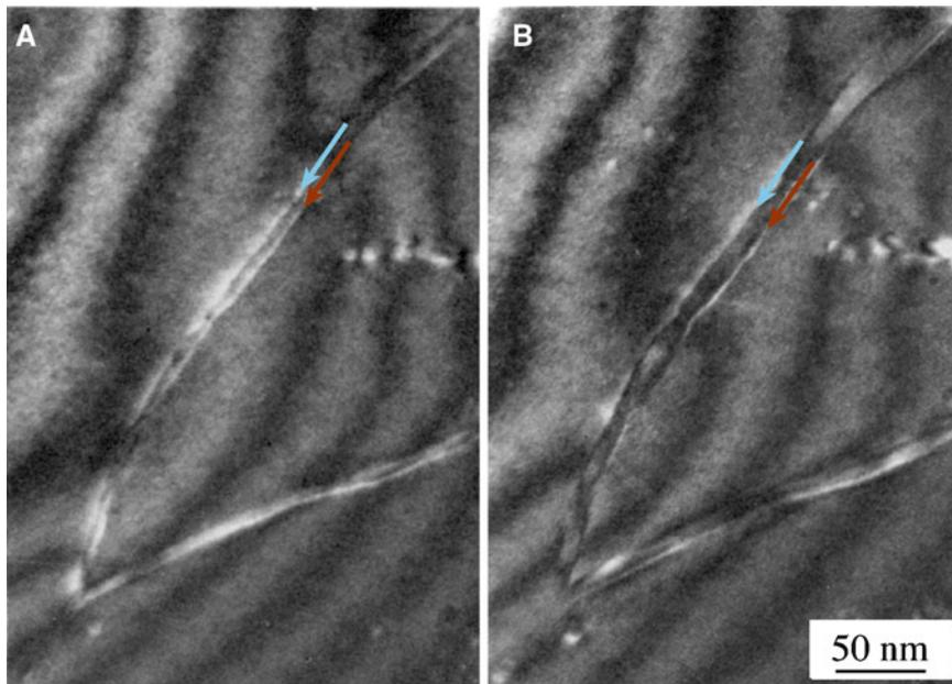
FIGURE 12.28. TEM shows amorphization of a dislocation core in quartz.
