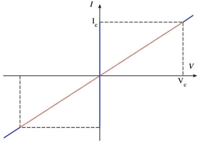
**FIGURE 30.31.**  $I$ - $V$  characteristics of a Josephson junction.
