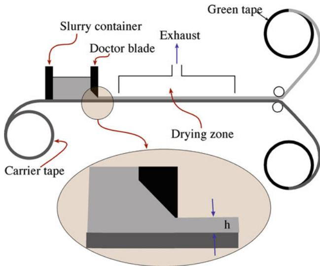
FIGURE 27.1. Tape-casting process.
