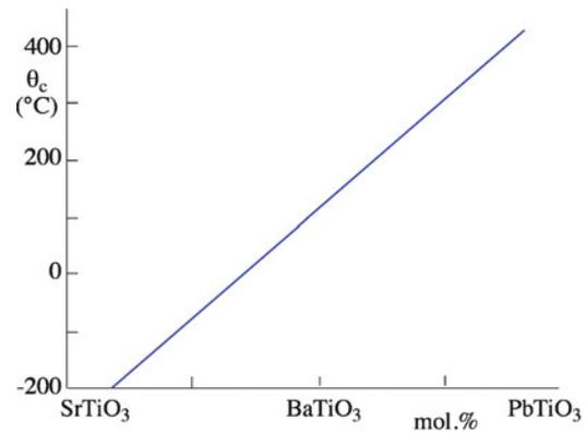
**FIGURE 31.16.** Effect of substitution on  $\theta_c$  for BaTiO<sub>3</sub> solid solutions with SrTiO<sub>3</sub> and PbTiO<sub>3</sub>.
