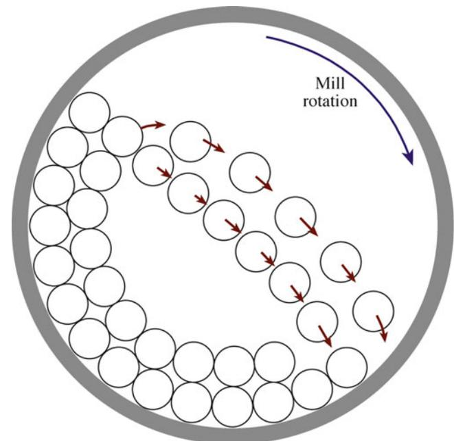
**FIGURE 20.1.** Cross section of a ball mill showing the movement of the media as the mill rotates about its axis.
