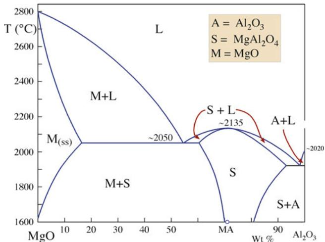
FIGURE 8.12. MgO–Al<sub>2</sub>O<sub>3</sub> phase diagram.
