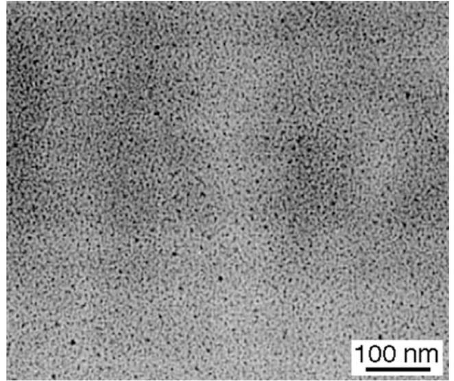
**FIGURE 21.14.** Transmission electron microscopy shows crystallization on a nanometer scale in a lithium aluminum silicate (LAS) glass-ceramic.
