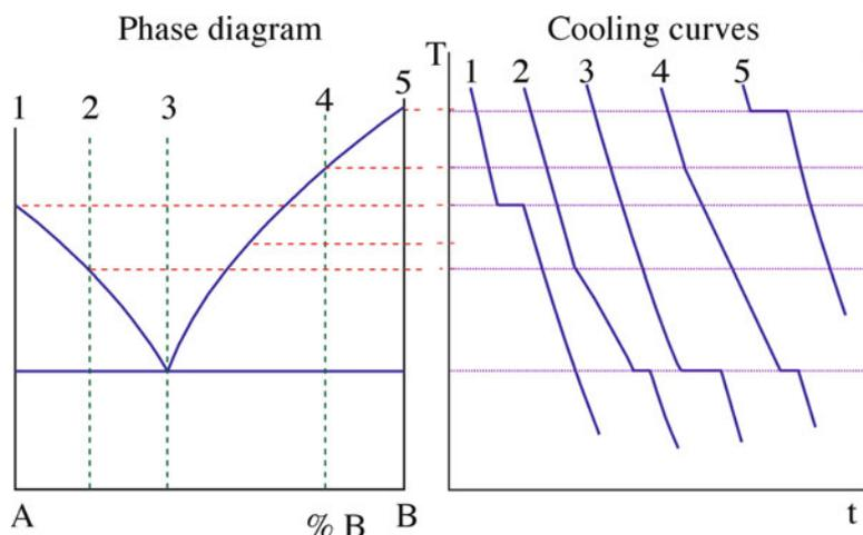
FIGURE 8.1. The use of cooling curves for determining the liquidus and eutectic in a binary phase diagram.
