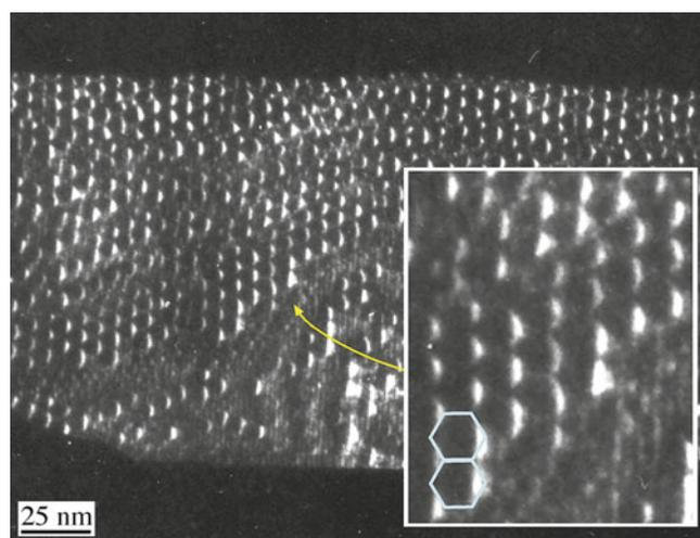
**FIGURE 15.1.** An  $\text{Fe}_2\text{O}_3$  film on an  $\text{Al}_2\text{O}_3$  substrate showing both  $\Sigma = 1$  and  $\Sigma = 3$  phase boundaries (PBs). The inset shows the hexagonal dislocation network.
