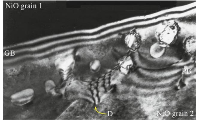
**FIGURE 15.10.** Growth of a particle along a GB. The particle is topotactically aligned with one NiO grain (along a PB at grain 2) but not the other (grain 1). D: dislocation at the coherent interface.
