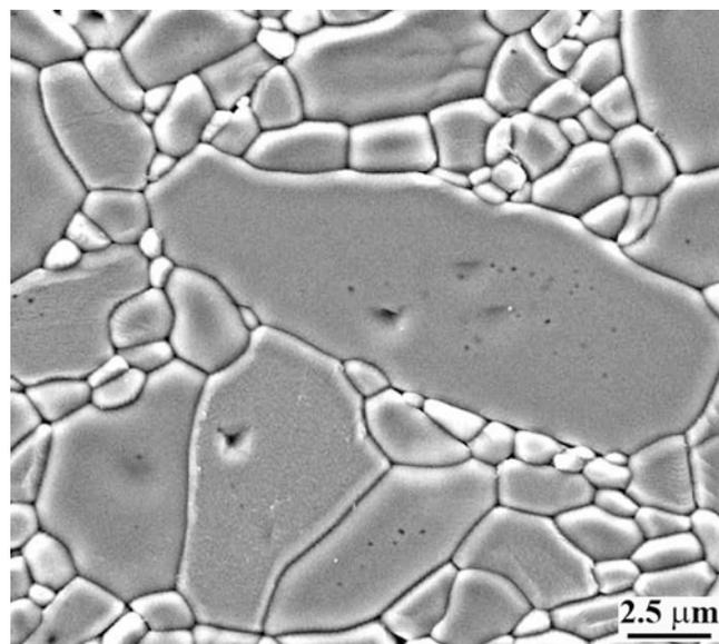
FIGURE 24.21. Elongated exaggerated grain in  $\text{Al}_2\text{O}_3$ .
