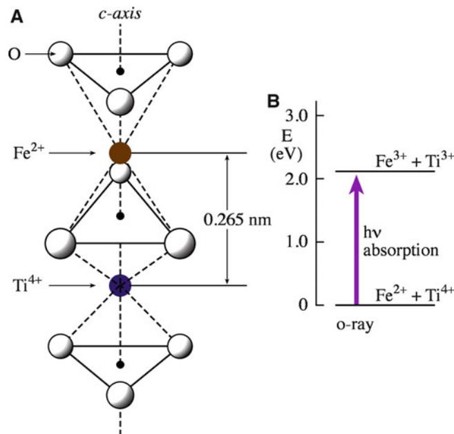
**FIGURE 36.13.** (A) Combined effect of incorporation of Ti and Fe in sapphire. The distance between the dopant cations is 0.265 nm. (B) Corresponding energy band diagram for the excitation shows how a gemstone with blue coloration is obtained by absorption.
