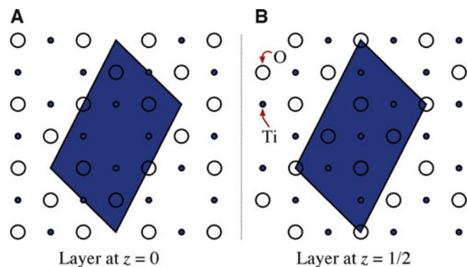
**FIGURE 30.5.** Structure of TiO (A) The (100) plane (B) The (200) plane. Both showing the absence of alternate ions along  $\langle 110 \rangle$  directions. The resultant superlattice has a monoclinic unit cell as indicated by the shaded region.
