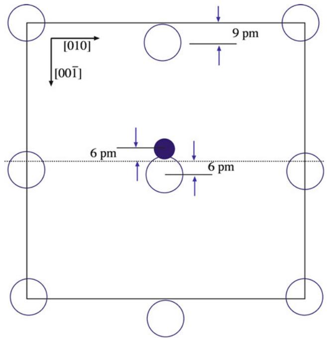
FIGURE 31.7. [100] Projection of BaTiO<sub>3</sub> shows ion displacements below  $\theta_c$  (not to scale).
