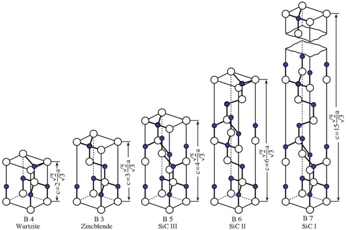
FIGURE 6.17. Stacking sequences for five SiC polytypes.
