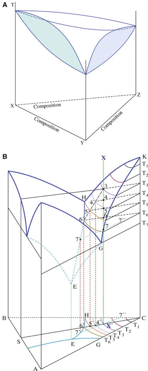
**FIGURE 8.15.** (A) A model ternary phase diagram for a system showing three solid solutions. (B) A model ternary phase diagram for a system showing three eutectics.
