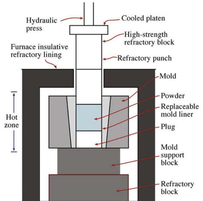
FIGURE 23.2. Essential elements of a hot press.
