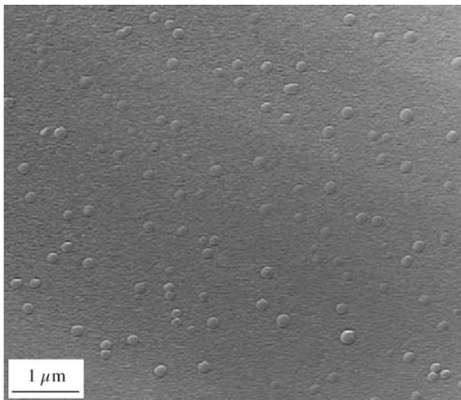
**FIGURE 8.24.** Image of small droplets of glass in a glass matrix. The composition of the glass is 16 wt.%  $\text{CaO}$ , 10 wt.%  $\text{MgO}$ , 14 wt.%  $\text{Al}_2\text{O}_3$ , 60 wt.%  $\text{SiO}_2$ .
