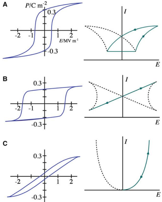
**FIGURE 32.22.** Electro-optic characteristics of PLZT. (A) Memory. (B) Linear. (C) Quadratic.  $I$  is the light output versus applied field  $E$ . (See A, B, and C in Figure 32.21).
