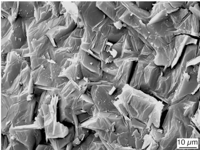
**FIGURE 18.23.** Fracture surface of Macor<sup>®</sup>.
