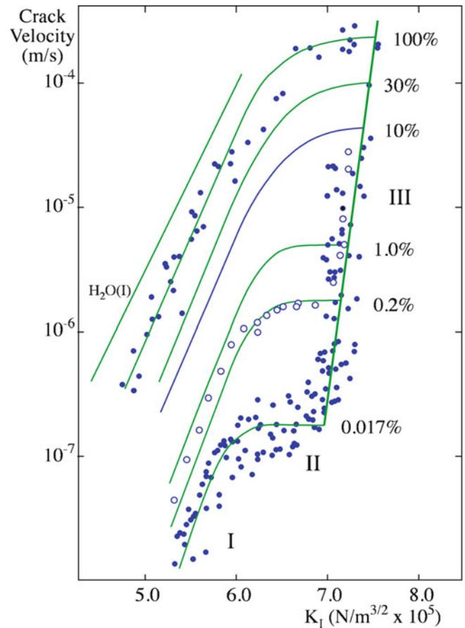
**FIGURE 18.9.** Crack velocity in soda-lime glass as a function of  $K_I$ , the stress intensity factor. The percentages indicate the relative humidity, and the Roman numerals indicate the three regions of crack propagation.
