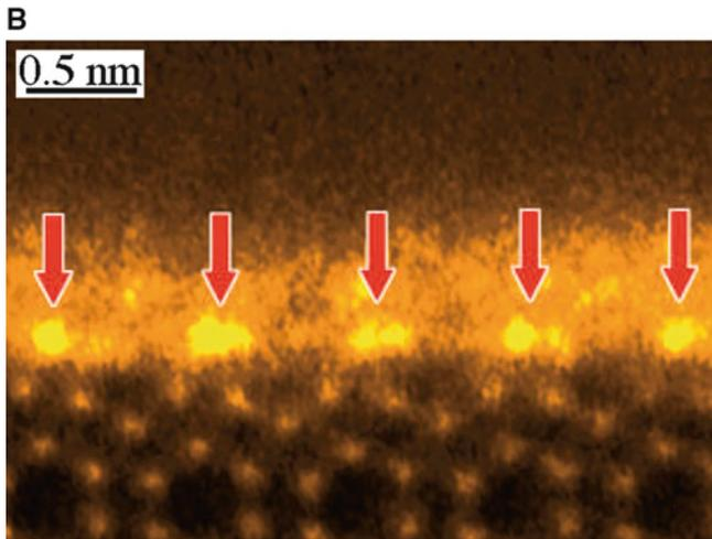
**FIGURE 14.27.** HRTEM images of intergranular films (IGFs) in  $\text{Si}_3\text{N}_4$ . (A) Phase contrast image. (B) Z-contrast image showing ordering of rare-earth dopant at the glass/crystal interface.
