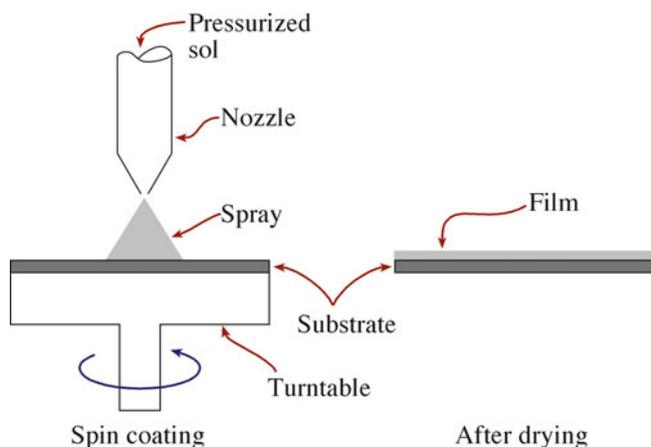
FIGURE 27.7. Spin-coating process.
