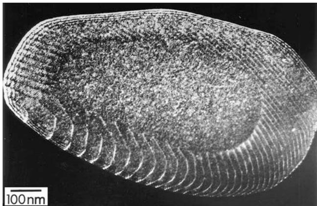
**FIGURE 25.7.** Growing particle of spinel in a matrix of Fe-doped  $\text{Al}_2\text{O}_3$  during internal reduction.
