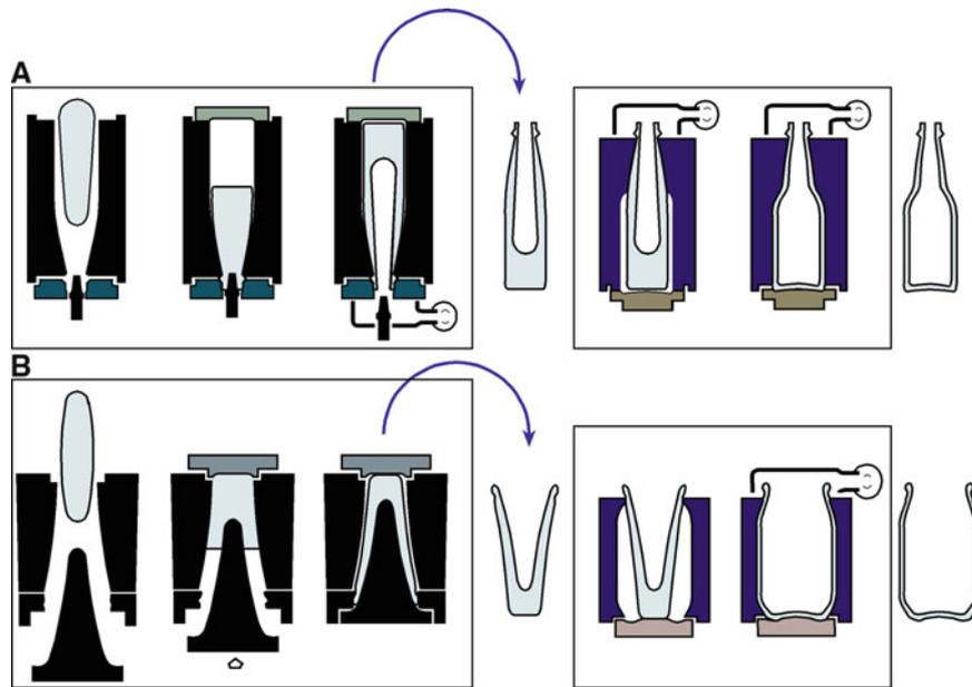
**FIGURE 26.11.** Automatic fabrication of hollow ware. (A) Formation of the blank by blowing followed by blowing in a mold (blow and blow). (B) Formation of the blank by pressing followed by blowing (press and blow).
