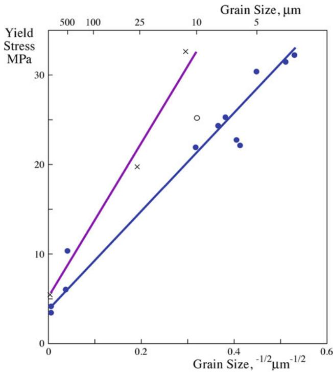
**FIGURE 17.10.** Grain size dependence of yield strength for KCl. Filled circles: pure material with a  $\langle 100 \rangle$  texture; open circles: pure material with  $\langle 111 \rangle$  texture; crosses: Sr-doped KCl.
