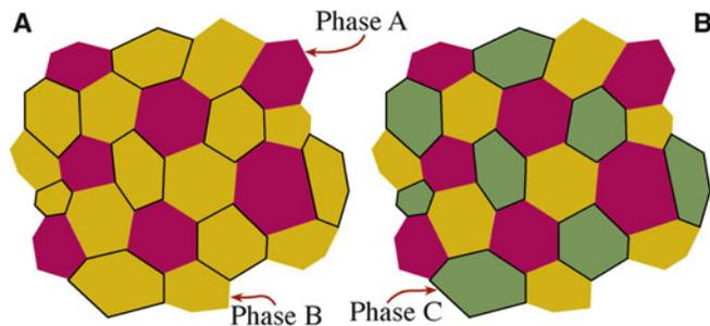
FIGURE 24.26. Multiphase ceramics. (A) Two phases. (B) Three phases.
