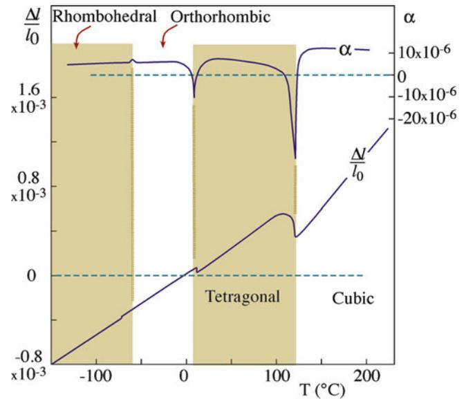
FIGURE 34.13. Coefficient of thermal expansion of BaTiO<sub>3</sub> as a function of temperature.
