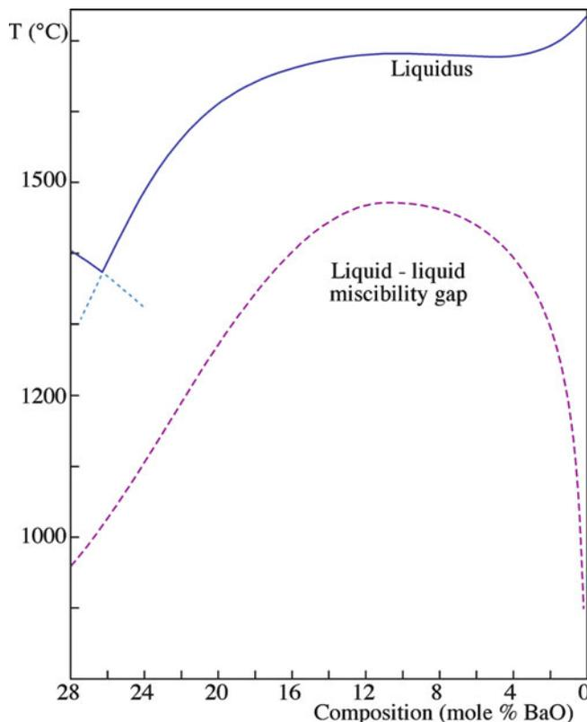
**FIGURE 8.25.** Silica-rich end of the  $\text{BaO-SiO}_2$  phase diagram.
