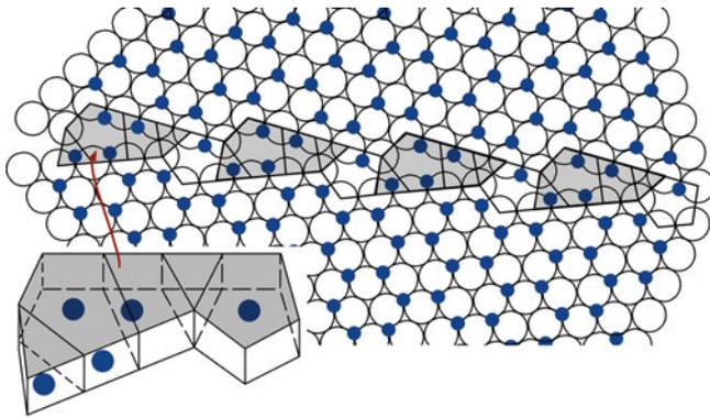
**FIGURE 14.17.** GB in  $\text{Al}_2\text{O}_3$  shows the creation of new polyhedra in the GB. Inset: tilted view of the repeating group of polyhedra.
