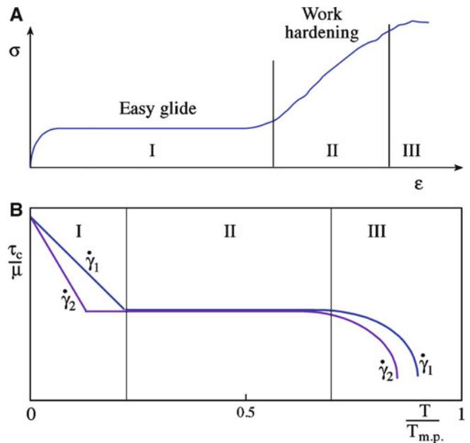
**FIGURE 17.7.** (A) Stress–strain curve for a crystal suitably oriented for plastic flow. (B) Temperature dependence of the normalized critical resolved shear stress for two strain rates, where  $\dot{\gamma}_1 > \dot{\gamma}_2$ .
