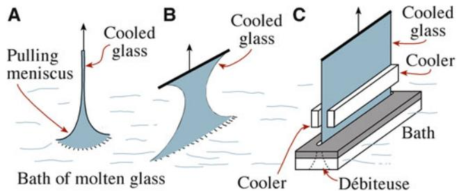
FIGURE 26.7. Principle of drawing from molten glass. (A) Circular rod. (B) Problem of pulling a planar sheet. (C) Use of a *débiteuse* and cooling to allow the formation of a sheet of constant width.
