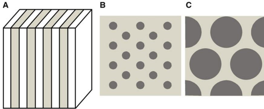
**FIGURE 34.8.** Three models for the distribution of two phases in a material. (A) Parallel slabs. (B) Continuous matrix phase, discontinuous particulate dispersion. (C) Large isolated grains separated by a continuous minor phase.
