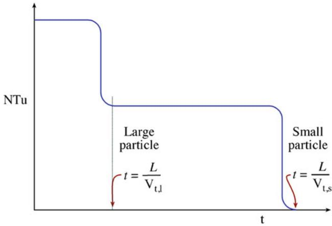
**FIGURE 20.11.** Result of sedimentation measurements using turbidity for two particle sizes in a solution;  $V_t$ : terminal velocity.
