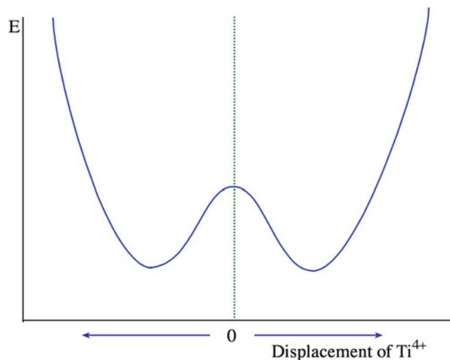
**FIGURE 31.12.** Potential energy wells for Ti<sup>4+</sup> as a function of displacement within the octahedral site.
