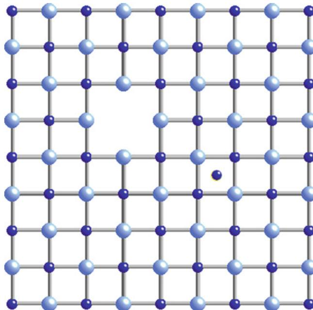
FIGURE 11.2. Frenkel defect drawn in two dimensions.
