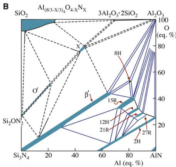
FIGURE 8.21. (a) The Si-Al-N-O phase diagram represented as a tetrahedron. (b) The Si<sub>3</sub>N<sub>4</sub>-SiO<sub>2</sub>-Al<sub>2</sub>O<sub>3</sub>-AlN phase diagram.
