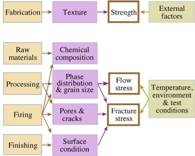
FIGURE 16.3. Factors affecting the mechanical properties of ceramics.
