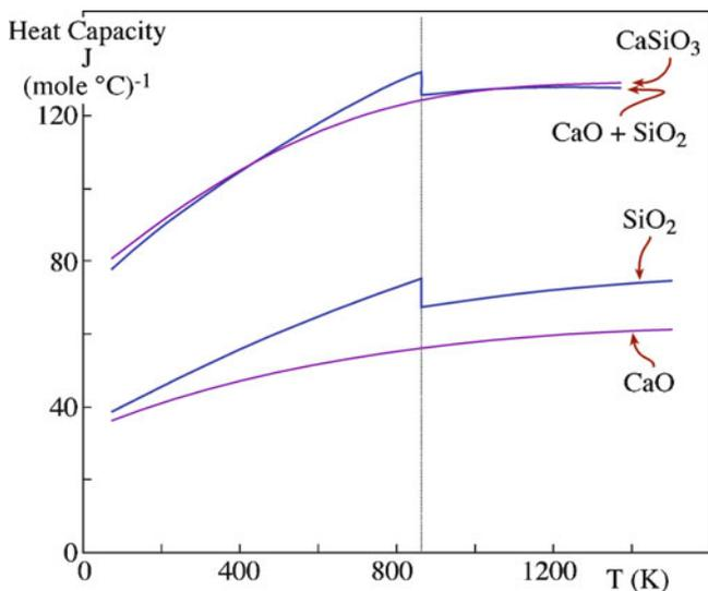
FIGURE 34.2. Heat capacity of SiO<sub>2</sub> as a function of temperature.
