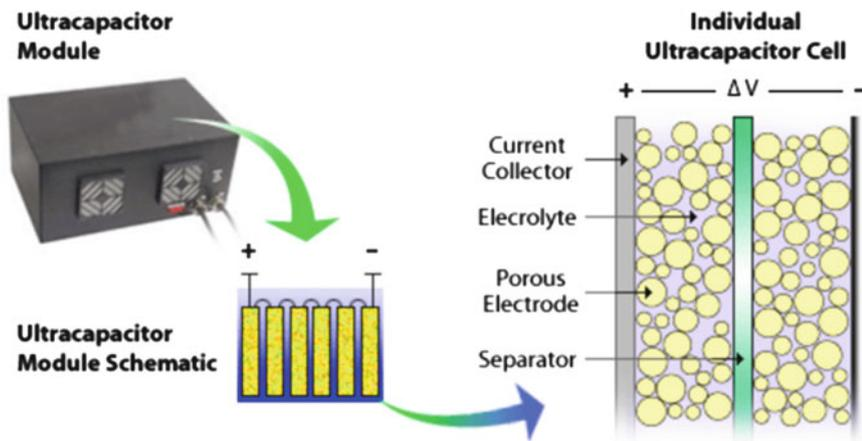
FIGURE 37.10. Basic structure of an ultracapacitor.
