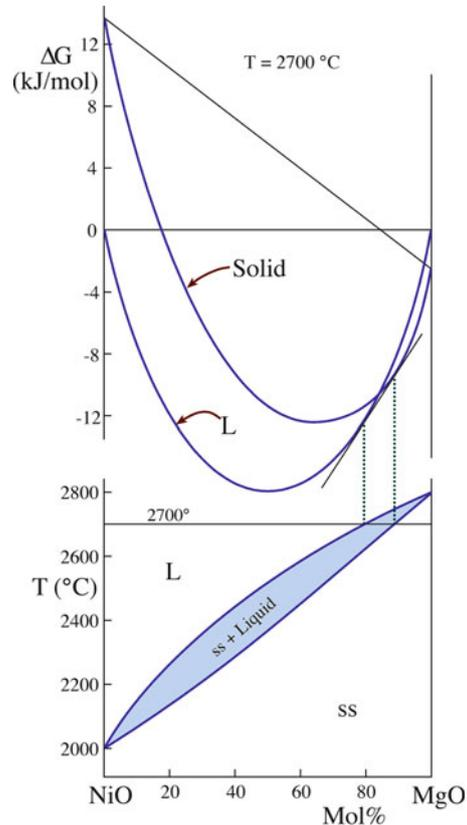
FIGURE 8.4. NiO-MgO phase diagram and free energy curves at  $T = 2,700^\circ\text{C}$ .
