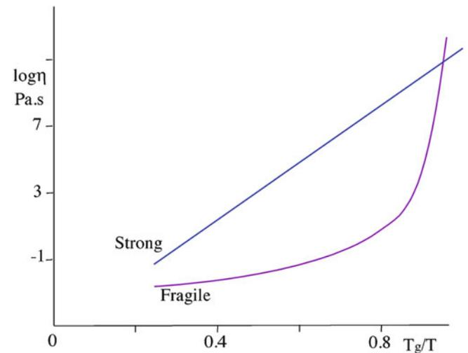
FIGURE 21.21. Viscosity versus temperature for strong and fragile liquids.
