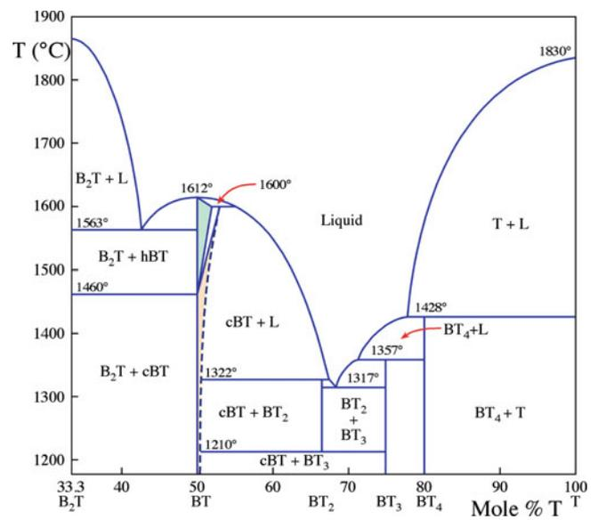
FIGURE 8.23. BaTiO<sub>3</sub> phase diagram.
