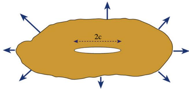
**FIGURE 18.5.** “Griffith” crack of length  $2c$ .
