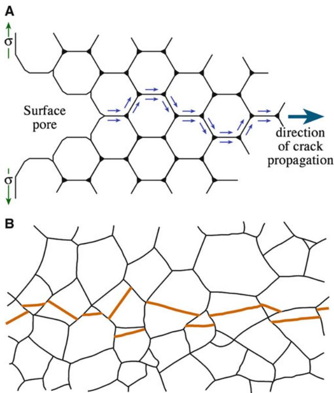
**FIGURE 18.12.** (A) Intergranular cracking. (B) Transgranular cracking.
