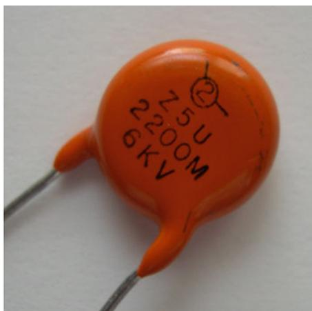
FIGURE 31.17. Ceramic disc capacitor.
