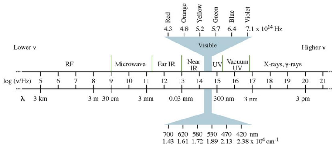
**FIGURE 32.1.** Electromagnetic spectrum. The visible region has been expanded for clarity. It is actually a very small part of the spectrum.
