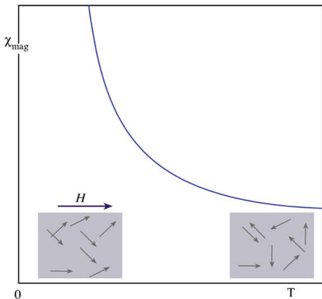
**FIGURE 33.5.** How  $\chi$  varies with temperature ( $T$ ) for a paramagnetic solid. Insets. Direction of the magnetic dipoles in the solids.
