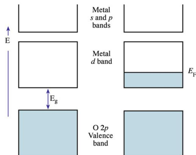
**FIGURE 30.6.** Energy bands of a transition metal oxide: (A) d band empty; (B) metallic oxide with d band partially filled.
