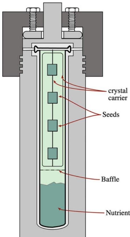
FIGURE 29.11. Silver-lined laboratory hydrothermal autoclave, about 35 cm long.
