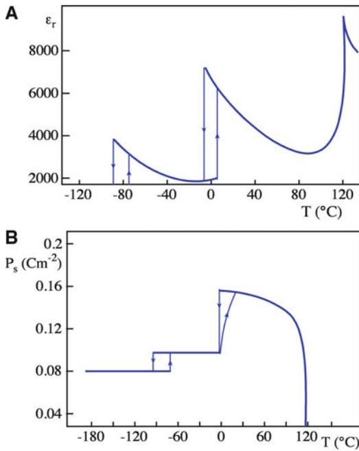
**FIGURE 31.14.** (A) Dielectric constant and (B) spontaneous polarization of single-crystal BaTiO<sub>3</sub> as a function of temperature. (Compare to Figure 31.9).
