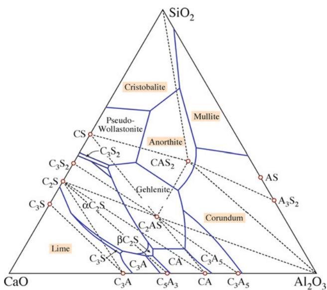
FIGURE 8.17. CaO–SiO<sub>2</sub>–Al<sub>2</sub>O<sub>3</sub> phase diagram.
