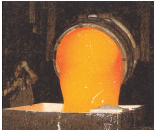
FIGURE 26.4. Pouring molten glass into a mold.
