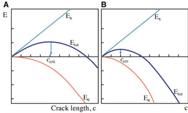
**FIGURE 18.4.** Plots of energy versus crack length.  $U_{tot}$  is the sum of  $U_s$  and  $U_e$ . The right plot corresponds to a greater applied stress (on this scale, the stress is greater by  $\sqrt{2}$ , and  $c_{crit}$  is correspondingly reduced by a factor of 2).
