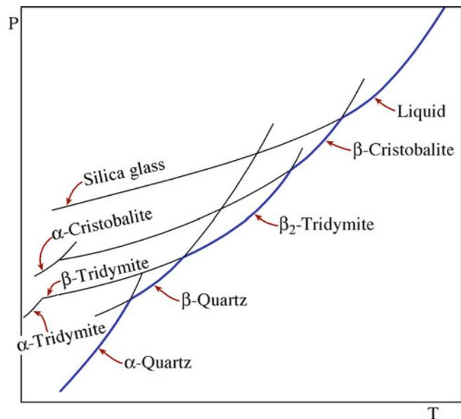
FIGURE 8.8. SiO<sub>2</sub> phase diagram.
