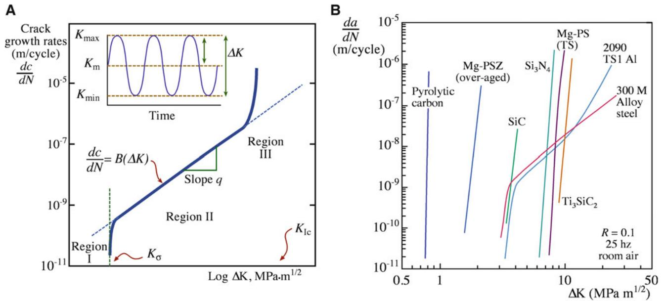
**FIGURE 18.11.** (A) Log-log plot of crack growth rate  $dc/dN$  versus  $K$  (defined in the inset). (B) Cyclic-fatigue crack growth rates for several ceramics and metal alloys as a function of applied stress intensity range,  $\Delta K$ .
