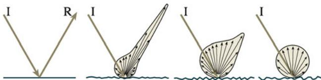
FIGURE 32.7. Effect of surface roughness on reflectivity.
