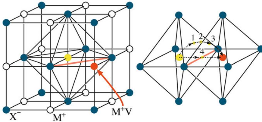
FIGURE 11.15. A probable diffusion mechanism in NaCl.
