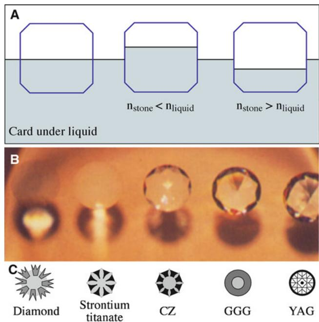
FIGURE 36.11. Determining the shadow patterns when stones are immersed in methyl iodide or liquid of another  $n$ . Different liquids are given in Table 36.4.
