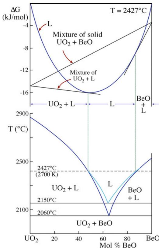
FIGURE 8.3. UO<sub>2</sub>-BeO phase diagram determined using free energy calculations.
