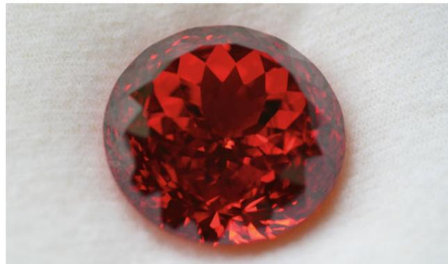
FIGURE 36.29. Single-crystal of rare earth (RE)-doped synthetic cubic zirconia that has been cut and polished.
