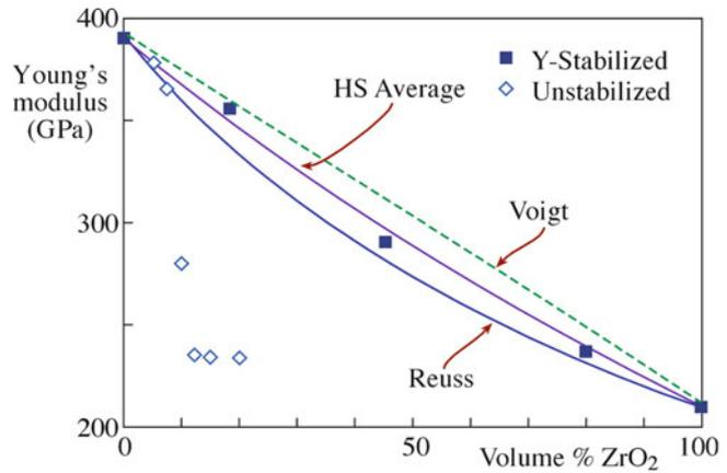
**FIGURE 16.7.** Comparison of predicted values of Young's modulus for an  $Al_2O_3$ -tetragonally stabilized  $ZrO_2$  composite with experimental data.
