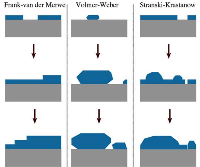
FIGURE 13.14. Three modes of thin-film growth.
