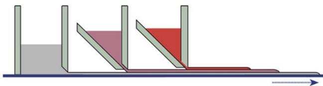
FIGURE 27.2. Triple doctor blade for producing multilayer tapes.
