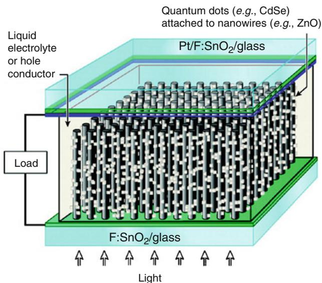
**FIGURE 37.6.** Quantum dot (QD)-sensitized solar cell. An array of ZnO nanowires—grown vertically from an F-doped SnO<sub>2</sub>/glass substrate and decorated with CdSe quantum dots—serve as the photoanode. A second F-doped SnO<sub>2</sub>/glass substrate, coated with a 10-nm layer of Pt, is the photocathode. The space between the two electrodes is filled with a liquid electrolyte, and the cell is illuminated from the bottom.
