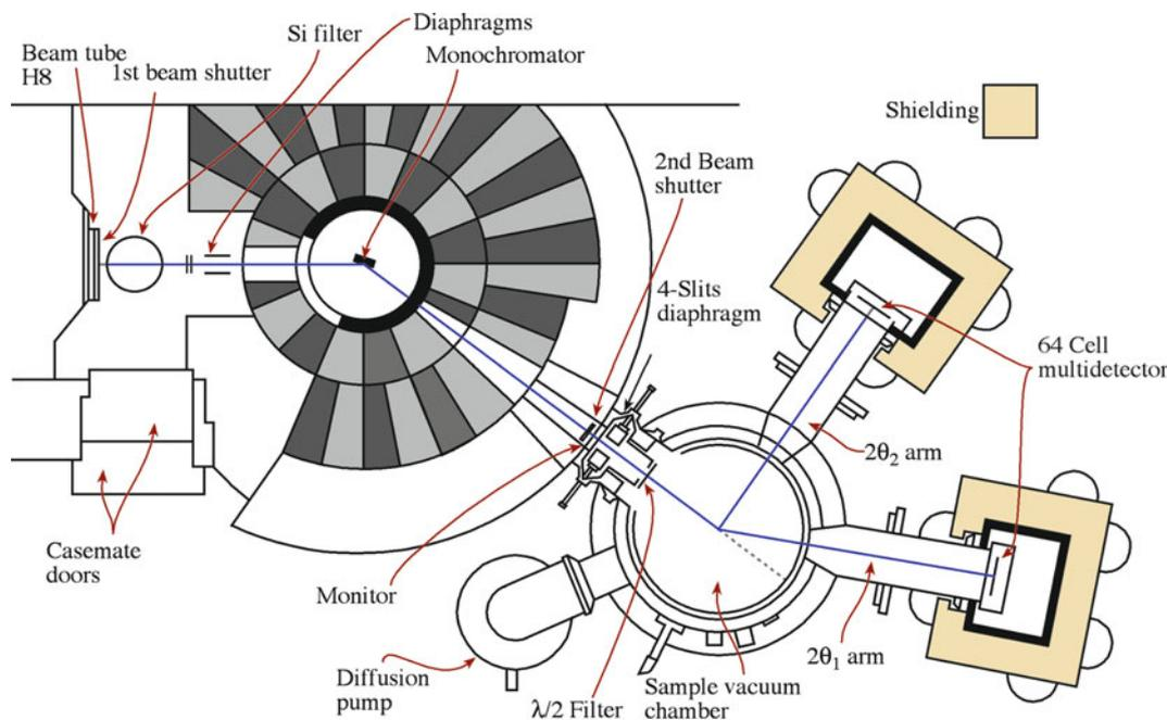
**FIGURE 10.32.** Schematic of a neutron scattering workstation. The width of the view is 10 s of meters.
