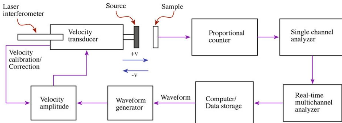
FIGURE 10.23. Setup for Mössbauer spectroscopy.
