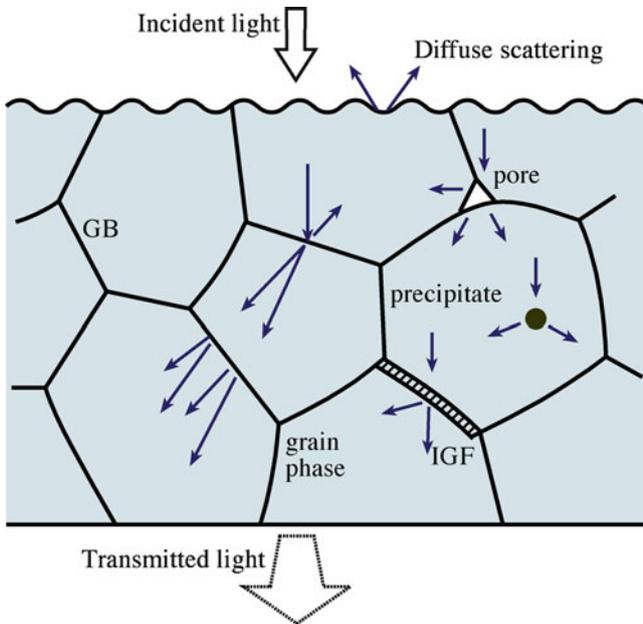
**FIGURE 32.10.** Mechanisms for loss of transparency due to scattering. Details of the individual defects are described in Chapters 12–15.
