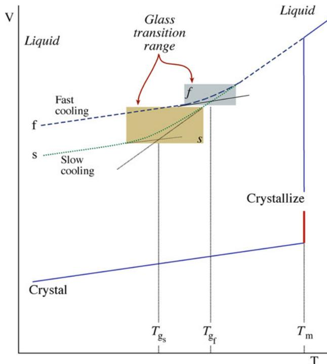
**FIGURE 21.1.** Plot of volume versus temperature for a liquid that forms a glass on cooling and one that forms a crystalline solid. The glass transition temperature,  $T_g$ , depends on the cooling rate and is not fixed like  $T_M$ .
