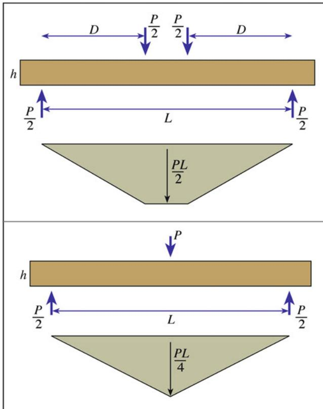
FIGURE 16.11. Geometries for three- and four-point bending.
