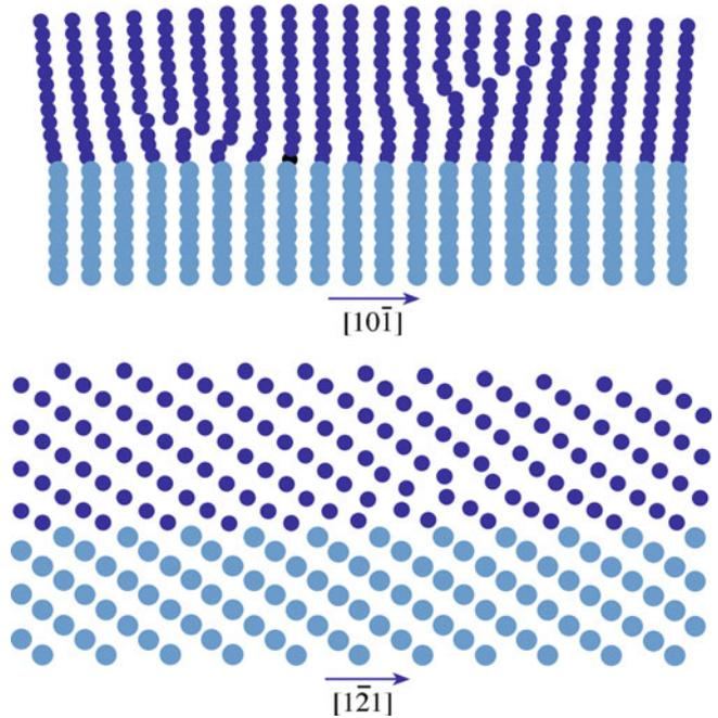
**FIGURE 15.20.** Stand-off dislocations accommodating lattice misfit between Nb and Al<sub>2</sub>O<sub>3</sub>.
