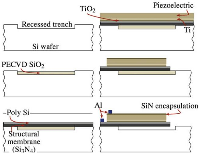
**FIGURE 31.23.** Steps in the production of a micro-electro-mechanical system cantilever. (A) Create trench by etching. (B) Deposit  $\text{SiO}_2$  layer by plasma-enhanced chemical vapor deposition. (C) Deposit  $\text{Si}_3\text{N}_4$  followed by polysilicon. (D) Deposit the piezoelectric film on an electrode/diffusion barrier system. (E) Pattern and etch. (F) Apply metal contacts and sacrificial etch.
