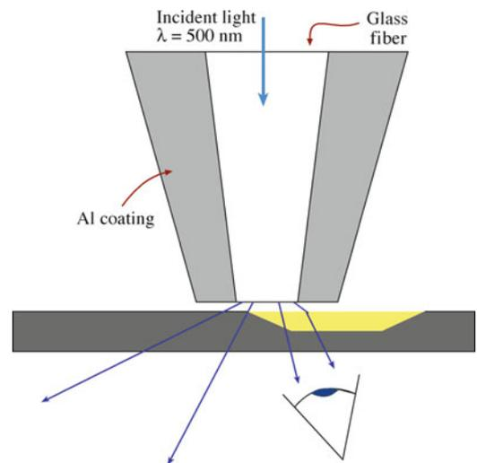
**FIGURE 10.2.** End of the fiber and the sample, seen by near-field scanning optical microscopy (NSOM).
