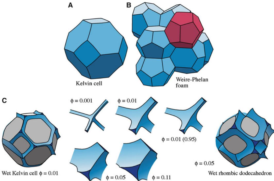
**FIGURE 15.17.** Intergranular films without grains. (A, B) Models of the Kelvin cell and a Weaire-Phelan foam used to describe soap bubbles. (C) How they relate to the structures of triple and quadruple junctions.
