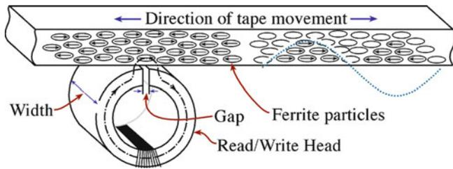
FIGURE 33.25. Principal features of longitudinal recording.
