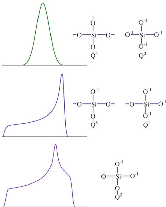
FIGURE 10.21. Nuclear magnetic resonance (NMR) signals from Si.
