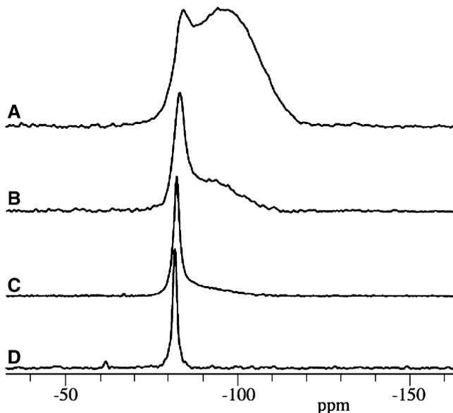
**FIGURE 37.1.** Increasing cumulative  $\alpha$ -radiation doses cause substantive changes in the local structure around silicon atoms as amorphization of the crystals progresses. (A) Undamaged zircon. (B) UG40, a zircon with  $1.2 \times 10^{18} \alpha/g$ . (C) Cam26, a zircon with  $2.9 \times 10^{18} \alpha/g$ . (D) Ni12, a zircon with  $7.1 \times 10^{18} \alpha/g$ .
