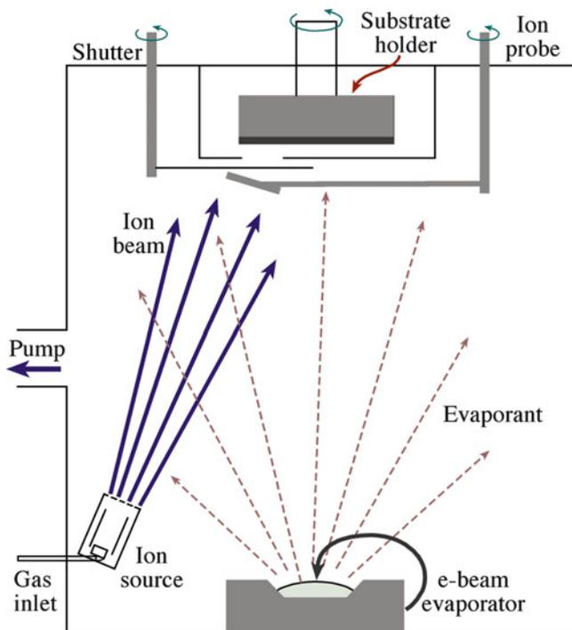
FIGURE 28.7. Ion-beam assisted deposition system.
