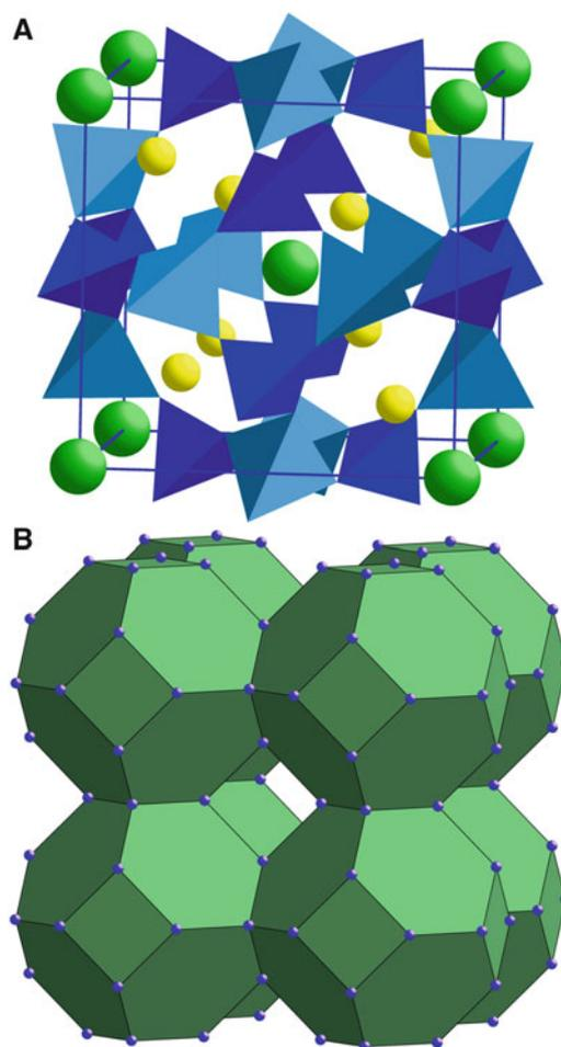
**FIGURE 7.17.** Structure of sodalite, a zeolite. The tetrahedra shown in “a” link together to form large “cages.” The most important features are the channels between the cages, which are seen in “b.” In “a” the corner and body centering ions are  $Cl^-$ ; the others are  $Na^+$  ions. The tetrahedra contain either  $Si^+$  or  $Al^+$ .
