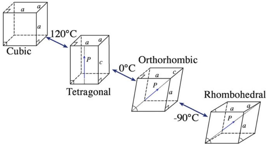
FIGURE 31.8. BaTiO<sub>3</sub> polymorphs show the direction of polarization.
