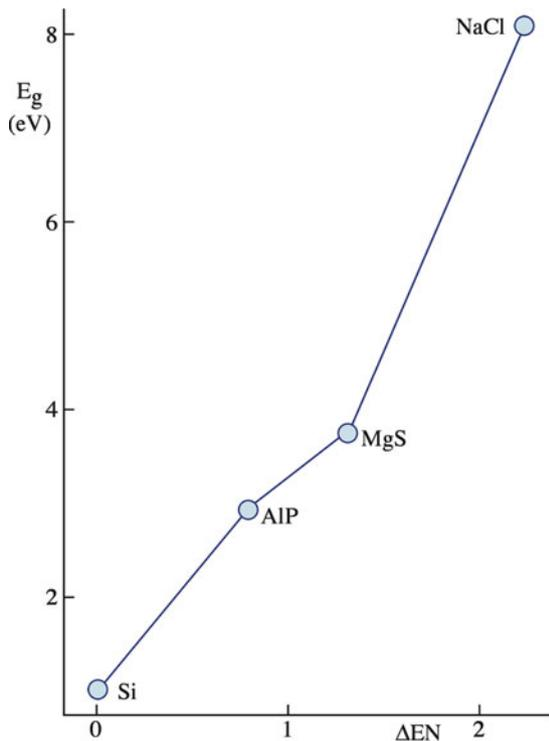
FIGURE 30.25. Correlation of  $E_g$  and the electronegativity difference.
