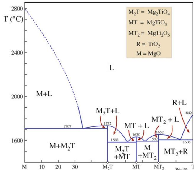
FIGURE 8.14. MgO–TiO<sub>2</sub> phase diagram.
