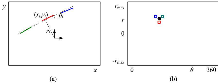
**Figure 4.42** Oriented Hough transform: (a) an edgel re-parameterized in polar  $(r, \theta)$  coordinates, with  $\hat{\mathbf{n}}_i = (\cos \theta_i, \sin \theta_i)$  and  $r_i = \hat{\mathbf{n}}_i \cdot \mathbf{x}_i$ ; (b)  $(r, \theta)$  accumulator array, showing the votes for the three edgels marked in red, green, and blue.
