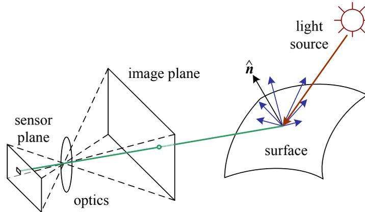
**Figure 2.14** A simplified model of photometric image formation. Light is emitted by one or more light sources and is then reflected from an object’s surface. A portion of this light is directed towards the camera. This simplified model ignores multiple reflections, which often occur in real-world scenes.
