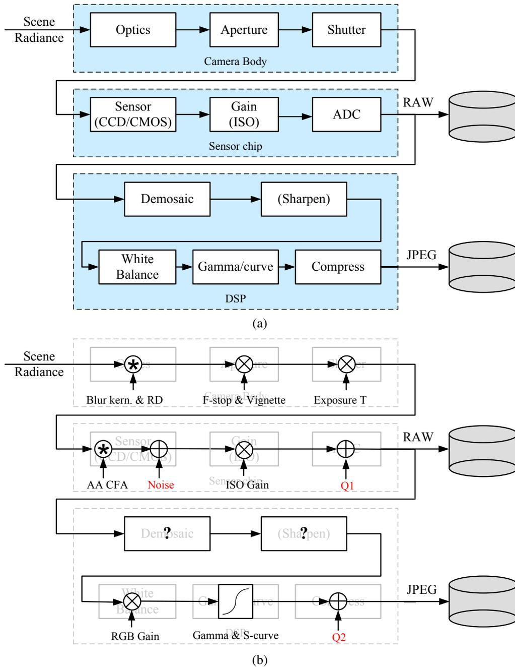
**Figure 10.2** Image sensing pipeline: (a) block diagram showing the various sources of noise as well as the typical digital post-processing steps; (b) equivalent signal transforms, including convolution, gain, and noise injection. The abbreviations are: RD = radial distortion, AA = anti-aliasing filter, CFA = color filter array, Q1 and Q2 = quantization noise.
