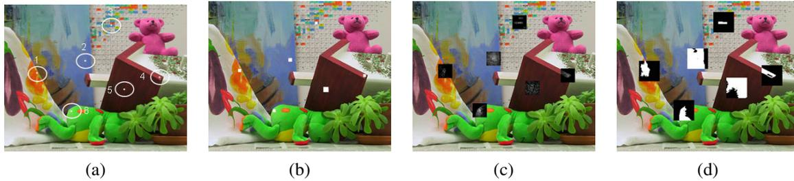
**Figure 11.9** Aggregation window sizes and weights adapted to image content (Tombari, Mattoccia, Di Stefano *et al.* 2008) © 2008 IEEE: (a) original image with selected evaluation points; (b) variable windows (Veksler 2003); (c) adaptive weights (Yoon and Kweon 2006); (d) segmentation-based (Tombari, Mattoccia, and Di Stefano 2007). Notice how the adaptive weights and segmentation-based techniques adapt their support to similarly colored pixels.
