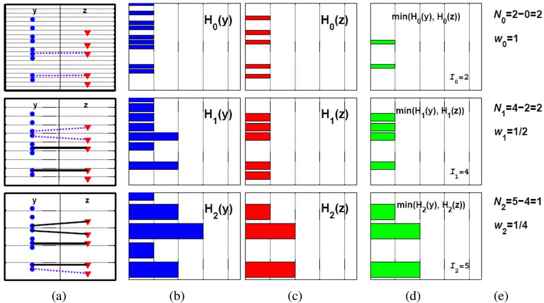
**Figure 14.38** A one-dimensional illustration of comparing collections of feature vectors using the pyramid match kernel (Grauman and Darrell 2007b): (a) distribution of feature vectors (point sets) into the pyramidal bins; (b–c) histogram of point counts in bins  $B_{il}$  and  $B'_{il}$  for the two images; (d) histogram intersections (minimum values); (e) per-level similarity scores, which are weighted and summed to form the final distance/similarity metric.
