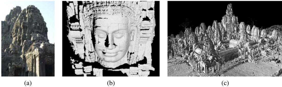
**Figure 12.10** Laser range modeling of the Bayon temple at Angkor-Thom (Banno, Masuda, Oishi *et al.* 2008) © 2008 Springer: (a) sample photograph from the site; (b) a detailed head model scanned from the ground; (c) final merged 3D model of the temple scanned using a laser range sensor mounted on a balloon.
