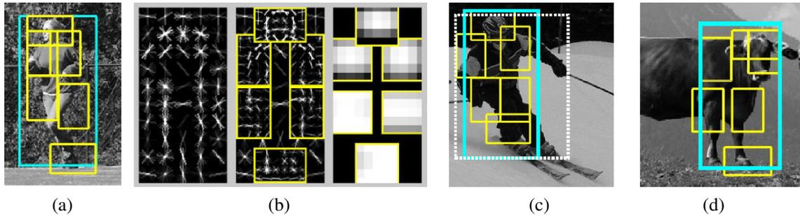
**Figure 14.9** Part-based object detection (Felzenszwalb, McAllester, and Ramanan 2008) © 2008 IEEE: (a) An input photograph and its associated person (blue) and part (yellow) detection results. (b) The detection model is defined by a coarse template, several higher resolution part templates, and a spatial model for the location of each part. (c) True positive detection of a skier and (d) false positive detection of a cow (labeled as a person).
