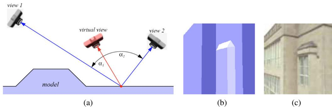
**Figure 13.3** View-dependent texture mapping (Debevec, Taylor, and Malik 1996) © 1996 ACM. (a) The weighting given to each input view depends on the relative angles between the novel (virtual) view and the original views; (b) simplified 3D model geometry; (c) with view-dependent texture mapping, the geometry appears to have more detail (recessed windows).
