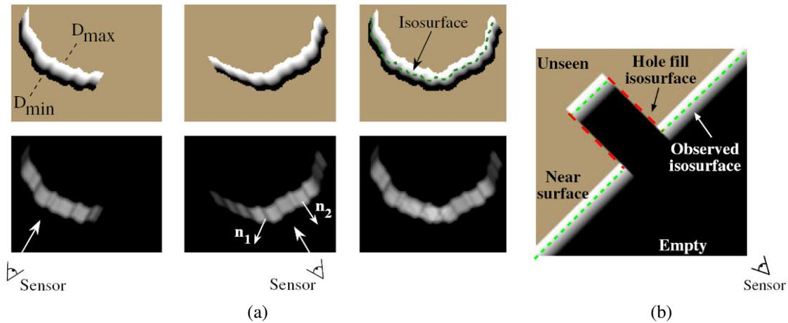
**Figure 12.8** Range data merging (Curless and Levoy 1996) © 1996 ACM: (a) two signed distance functions (top left) are merged with their (weights) bottom left to produce a combined set of functions (right column) from which an isosurface can be extracted (green dashed line); (b) the signed distance functions are combined with empty and unseen space labels to fill holes in the isosurface.
