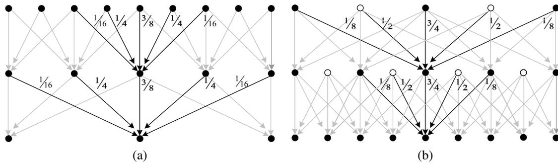
**Figure 3.33** The Gaussian pyramid shown as a signal processing diagram: The (a) analysis and (b) re-synthesis stages are shown as using similar computations. The white circles indicate zero values inserted by the  $\uparrow 2$  upsampling operation. Notice how the reconstruction filter coefficients are twice the analysis coefficients. The computation is shown as flowing down the page, regardless of whether we are going from coarse to fine or *vice versa*.
