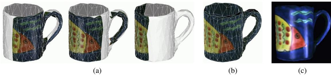
**Figure 12.22** Estimating the diffuse albedo and reflectance parameters for a scanned 3D model (Sato, Wheeler, and Ikeuchi 1997) © 1997 ACM: (a) set of input images projected onto the model; (b) the complete diffuse reflection (albedo) model; (c) rendering from the reflectance model including the specular component.
