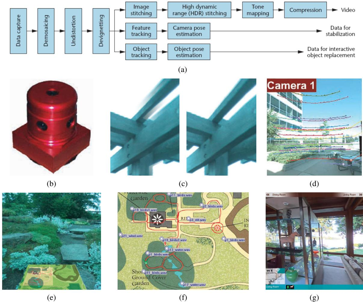
**Figure 13.16** Video-based walkthroughs (Uyttendaele, Criminisi, Kang *et al.* 2004) © 2004 IEEE: (a) system diagram of video pre-processing; (b) the Point Grey Ladybug camera; (c) ghost removal using multi-perspective plane sweep; (d) point tracking, used both for calibration and stabilization; (e) interactive garden walkthrough with map below; (f) overhead map authoring and sound placement; (g) interactive home walkthrough with navigation bar (top) and icons of interest (bottom).
