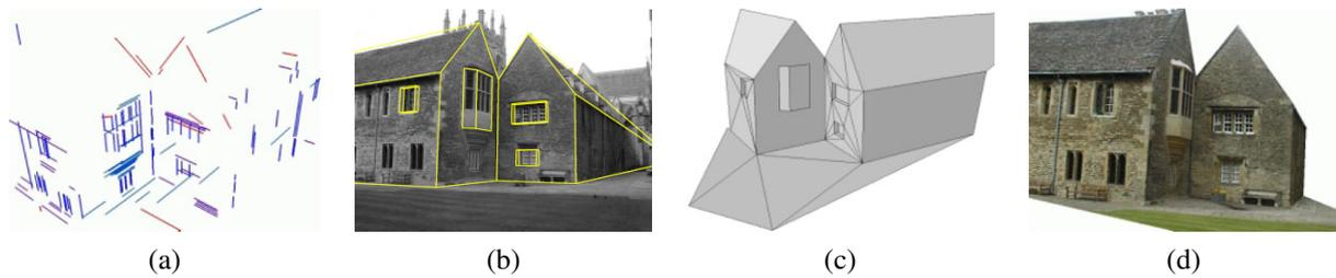
**Figure 12.16** Automated architectural reconstruction using 3D lines and planes (Werner and Zisserman 2002) © 2002 Springer: (a) reconstructed 3D lines, color coded by their vanishing directions; (b) wire-frame model superimposed onto an input image; (c) triangulated piecewise-planar model with windows; (d) final texture-mapped model.
