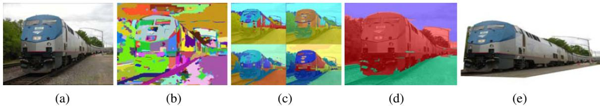
**Figure 14.47** Automatic photo pop-up (Hoiem, Efros, and Hebert 2005a) © 2005 ACM: (a) input image; (b) superpixels are grouped into (c) multiple regions; (d) labelings indicating ground (green), vertical (red), and sky (blue); (e) novel view of resulting piecewise-planar 3D model.
