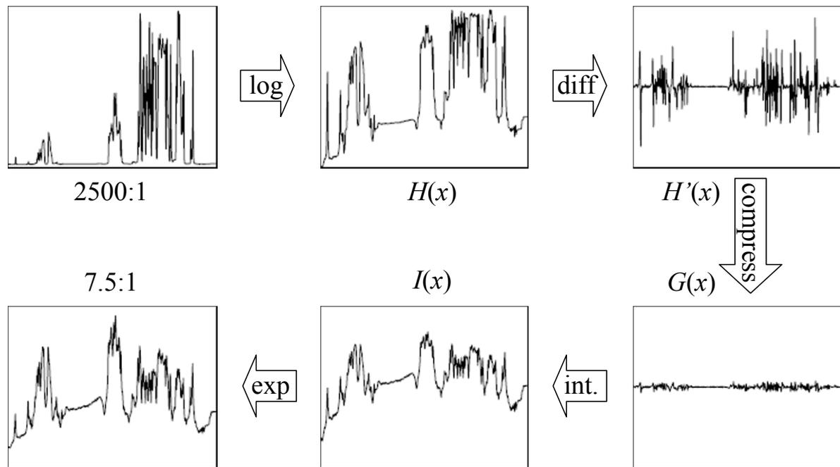
**Figure 10.25** Gradient domain tone mapping (Fattal, Lischinski, and Werman 2002) © 2002 ACM. The original image with a dynamic range of 2415:1 is first converted into the log domain,  $H(x)$ , and its gradients are computed,  $H'(x)$ . These are attenuated (compressed) based on local contrast,  $G(x)$ , and integrated to produce the new logarithmic exposure image  $I(x)$ , which is exponentiated to produce the final intensity image, whose dynamic range is 7.5:1.
