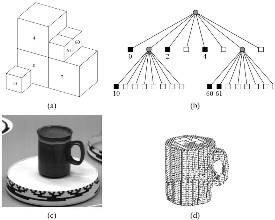
**Figure 11.22** Volumetric octree reconstruction from binary silhouettes (Szeliski 1993) © 1993 Elsevier: (a) octree representation and its corresponding (b) tree structure; (c) input image of an object on a turntable; (d) computed 3D volumetric octree model.
