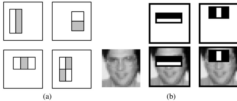
**Figure 14.6** Simple features used in boosting-based face detector (Viola and Jones 2004) © 2004 Springer: (a) difference of rectangle feature composed of 2–4 different rectangles (pixels inside the white rectangles are subtracted from the gray ones); (b) the first and second features selected by AdaBoost. The first feature measures the differences in intensity between the eyes and the cheeks, the second one between the eyes and the bridge of the nose.
