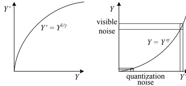
**Figure 2.31** Gamma compression: (a) The relationship between the input signal luminance  $Y$  and the transmitted signal  $Y'$  is given by  $Y' = Y^{1/\gamma}$ . (b) At the receiver, the signal  $Y'$  is exponentiated by the factor  $\gamma$ ,  $\hat{Y} = Y'^{\gamma}$ . Noise introduced during transmission is squashed in the dark regions, which corresponds to the more noise-sensitive region of the visual system.
