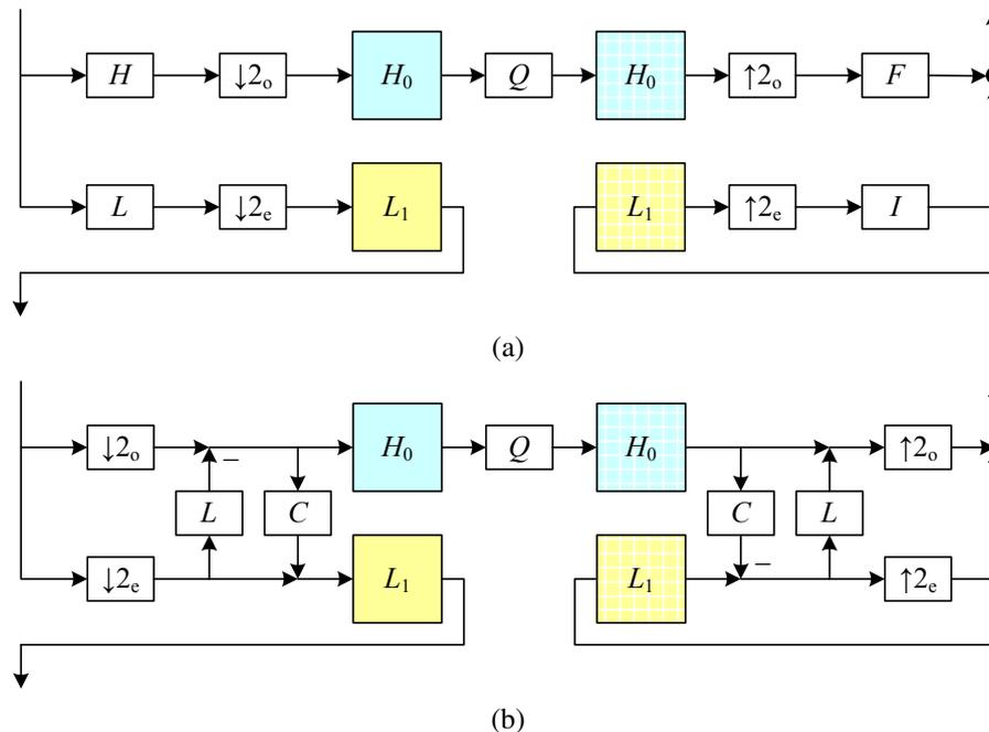
**Figure 3.38** One-dimensional wavelet transform: (a) usual high-pass + low-pass filters followed by odd ( $\downarrow 2_o$ ) and even ( $\downarrow 2_e$ ) downsampling; (b) lifted version, which first selects the odd and even subsequences and then applies a low-pass prediction stage  $L$  and a high-pass correction stage  $C$  in an easily reversible manner.
