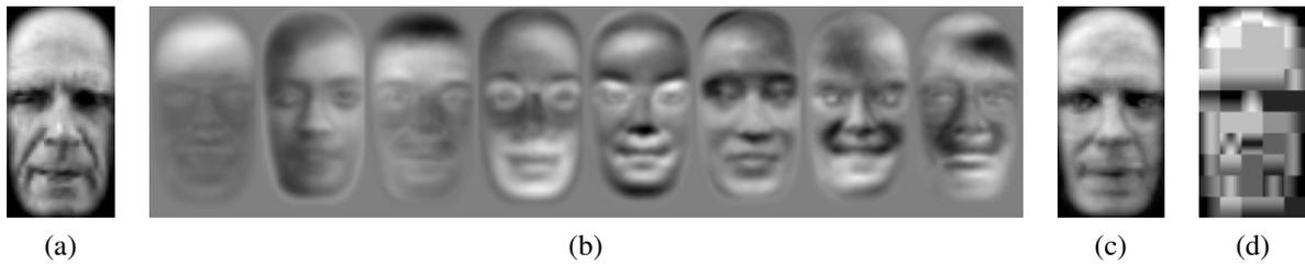
**Figure 14.13** Face modeling and compression using eigenfaces (Moghaddam and Pentland 1997) © 1997 IEEE: (a) input image; (b) the first eight eigenfaces; (c) image reconstructed by projecting onto this basis and compressing the image to 85 bytes; (d) image reconstructed using JPEG (530 bytes).
