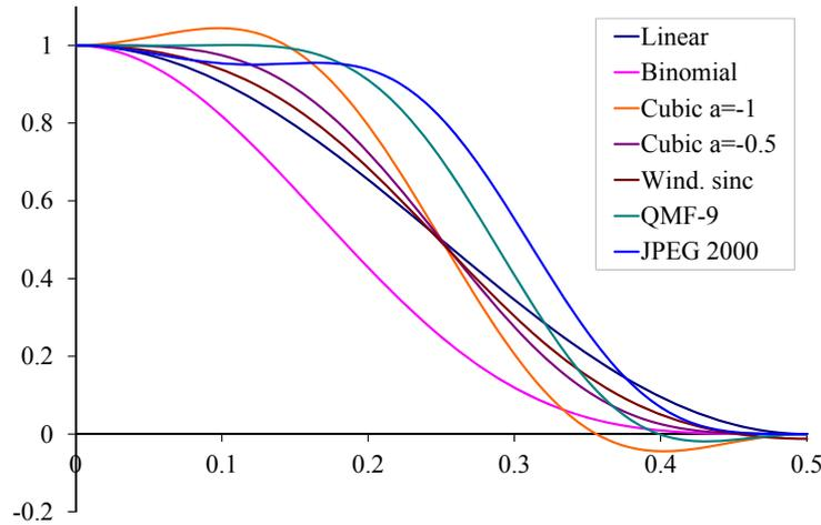
**Figure 3.31** Frequency response for some  $2\times$  decimation filters. The cubic  $a = -1$  filter has the sharpest fall-off but also a bit of ringing; the wavelet analysis filters (QMF-9 and JPEG 2000), while useful for compression, have more aliasing.
