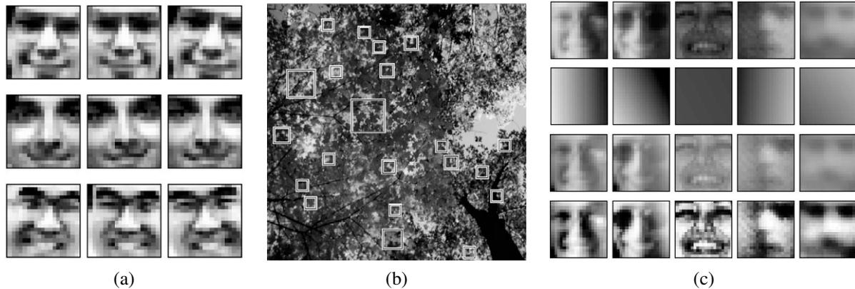
**Figure 14.3** Pre-processing stages for face detector training (Rowley, Baluja, and Kanade 1998a) © 1998 IEEE: (a) artificially mirroring, rotating, scaling, and translating training images for greater variability; (b) using images without faces (looking up at a tree) to generate non-face examples; (c) pre-processing the patches by subtracting a best fit linear function (constant gradient) and histogram equalizing.
