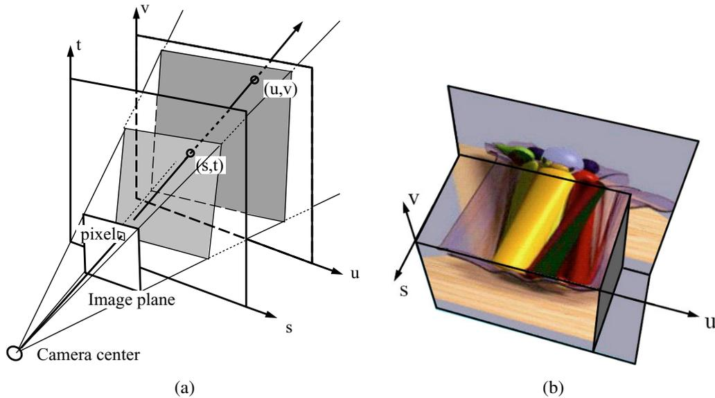
**Figure 13.7** The Lumigraph (Gortler, Grzeszczuk, Szeliski *et al.* 1996) © 1996 ACM: (a) a ray is represented by its 4D two-plane parameters  $(s, t)$  and  $(u, v)$ ; (b) a slice through the 3D light field subset  $(u, v, s)$ .
