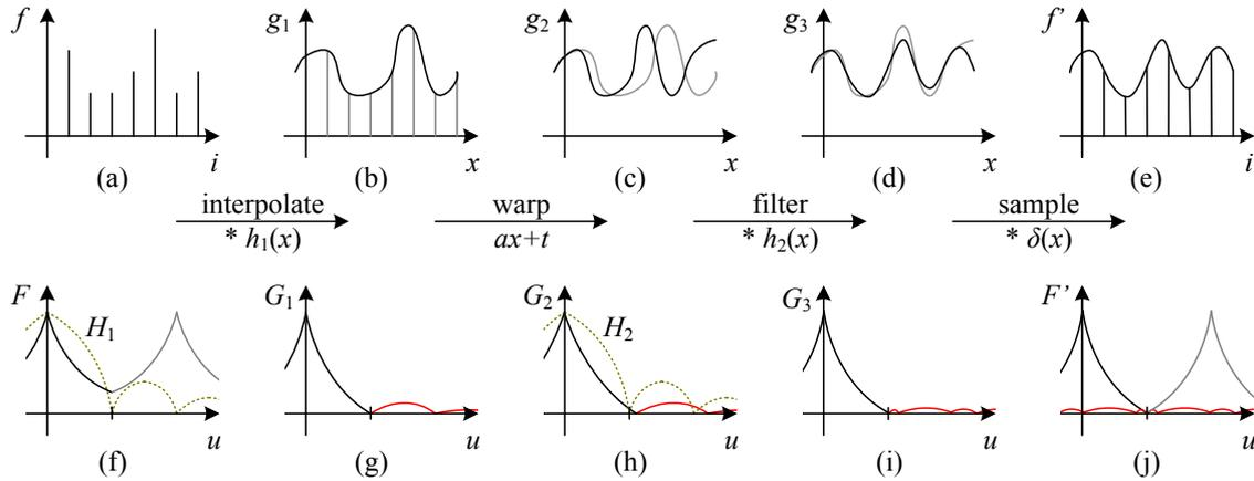
**Figure 3.49** One-dimensional signal resampling (Szeliski, Winder, and Uyttendaele 2010): (a) original sampled signal  $f(i)$ ; (b) interpolated signal  $g_1(x)$ ; (c) warped signal  $g_2(x)$ ; (d) filtered signal  $g_3(x)$ ; (e) sampled signal  $f'(i)$ . The corresponding spectra are shown below the signals, with the aliased portions shown in red.
