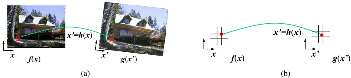
**Figure 3.46** Forward warping algorithm: (a) a pixel  $f(x)$  is copied to its corresponding location  $x' = h(x)$  in image  $g(x')$ ; (b) detail of the source and destination pixel locations.
