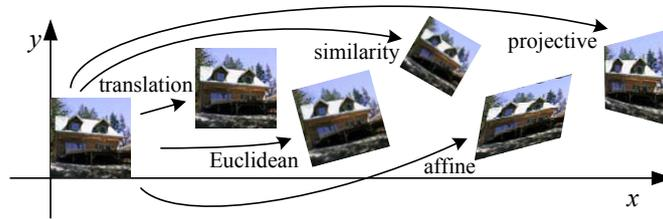
**Figure 3.45** Basic set of 2D geometric image transformations.
