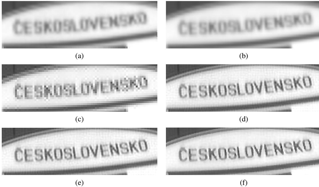
**Figure 10.31** Super-resolution results using a variety of image priors (Capel 2001): (a) Low-res ROI (bicubic  $3\times$  zoom); (b) average image; (c) MLE @  $1.25\times$  pixel-zoom; (d) simple  $\|x\|^2$  prior ( $\lambda = 0.004$ ); (e) GMRF ( $\lambda = 0.003$ ); (f) HMRF ( $\lambda = 0.01$ ,  $\alpha = 0.04$ ). 10 images are used as input and a  $3\times$  super-resolved image is produced in each case, except for the MLE result in (c).
