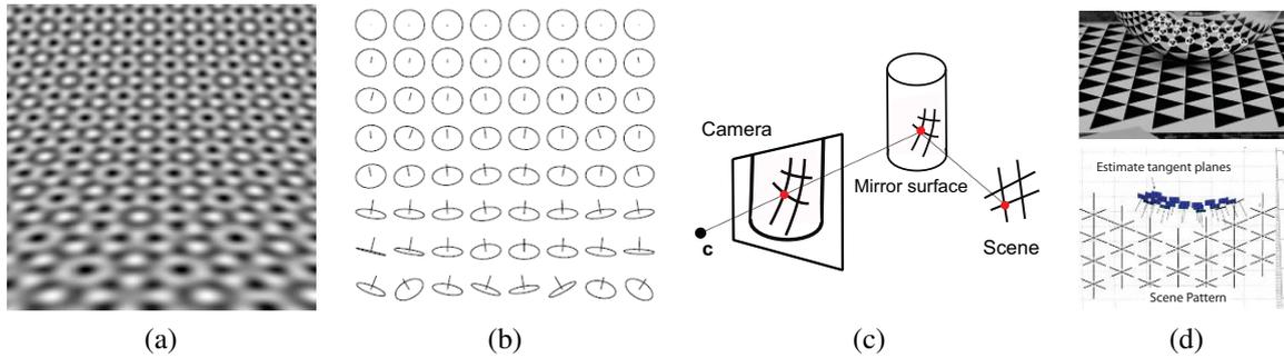
**Figure 12.3** Synthetic shape from texture (Garding 1992) © 1992 Springer: (a) regular texture wrapped onto a curved surface and (b) the corresponding surface normal estimates. Shape from mirror reflections (Savarese, Chen, and Perona 2005) © 2005 Springer: (c) a regular pattern reflecting off a curved mirror gives rise to (d) curved lines, from which 3D point locations and normals can be inferred.
