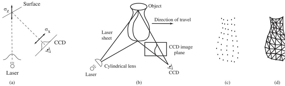
**Figure 12.5** Range data scanning (Curless and Levoy 1996) © 1996 ACM: (a) a laser dot on a surface is imaged by a CCD sensor; (b) a laser stripe (sheet) is imaged by the sensor (the deformation of the stripe encodes the distance to the object); (c) the resulting set of 3D points are turned into (d) a triangulated mesh.
