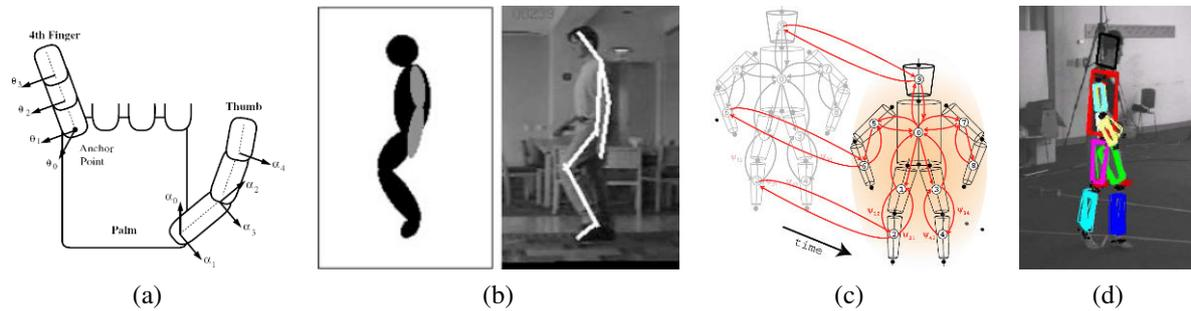
**Figure 12.20** Tracking 3D human motion: (a) kinematic chain model for a human hand (Rehg, Morris, and Kanade 2003) © 2003, reprinted by permission of SAGE; (b) tracking a kinematic chain blob model in a video sequence (Bregler, Malik, and Pullen 2004) © 2004 Springer; (c–d) probabilistic loose-limbed collection of body parts (Sigal, Bhatia, Roth *et al.* 2004)
