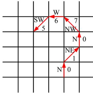
**Figure 4.34** Chain code representation of a grid-aligned linked edge chain. The code is represented as a series of direction codes, e.g., 0 1 0 7 6 5, which can further be compressed using predictive and run-length coding.
