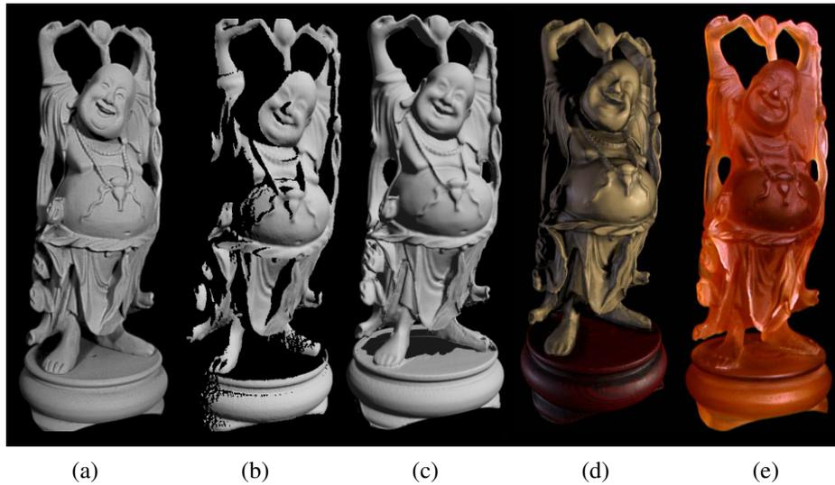
**Figure 12.9** Reconstruction and hardcopy of the “Happy Buddha” statuette (Curless and Levoy 1996) © 1996 ACM: (a) photograph of the original statue after spray painting with matte gray; (b) partial range scan; (c) merged range scans; (d) colored rendering of the reconstructed model; (e) hardcopy of the model constructed using stereolithography.
