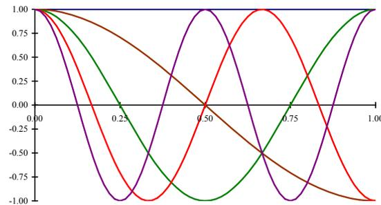
**Figure 3.26** Discrete cosine transform (DCT) basis functions: The first DC (i.e., constant) basis is the horizontal blue line, the second is the brown half-cycle waveform, etc. These bases are widely used in image and video compression standards such as JPEG.
