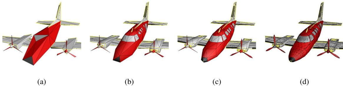
**Figure 12.11** Progressive mesh representation of an airplane model (Hoppe 1996) © 1996 ACM: (a) base mesh  $M^0$  (150 faces); (b) mesh  $M^{175}$  (500 faces); (c) mesh  $M^{425}$  (1000 faces); (d) original mesh  $M = M^n$  (13,546 faces).
