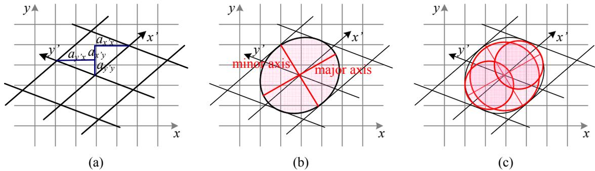
**Figure 3.48** Anisotropic texture filtering: (a) Jacobian of transform  $A$  and the induced horizontal and vertical resampling rates  $\{a_{x'x}, a_{x'y}, a_{y'x}, a_{y'y}\}$ ; (b) elliptical footprint of an EWA smoothing kernel; (c) anisotropic filtering using multiple samples along the major axis. Image pixels lie at line intersections.
