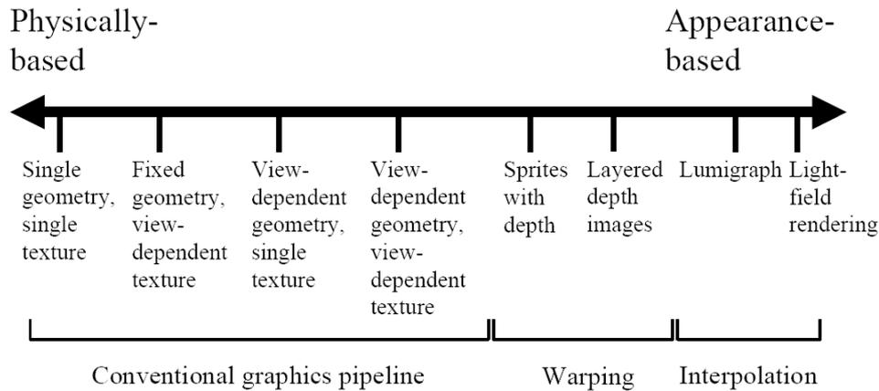
**Figure 13.11** The geometry-image continuum in image-based rendering (Kang, Szeliski, and Anandan 2000) © 2000 IEEE. Representations at the left of the spectrum use more detailed geometry and simpler image representations, while representations and algorithms on the right use more images and less geometry.
