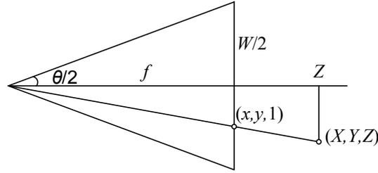
**Figure 2.10** Central projection, showing the relationship between the 3D and 2D coordinates,  $\mathbf{p}$  and  $\mathbf{x}$ , as well as the relationship between the focal length  $f$ , image width  $W$ , and the field of view  $\theta$ .
