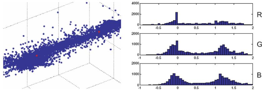
**Figure 10.36** Two-color model computed from a collection of local  $5 \times 5$  neighborhoods (Bennett, Uyttendaele, Zitnick *et al.* 2006) © 2006 Springer. After two-means clustering and reprojecting along the line joining the two dominant colors (red dots), the majority of the pixels fall near the fitted line. The distribution along the line, projected along the RGB axes, is peaked at 0 and 1, the two dominant colors.
