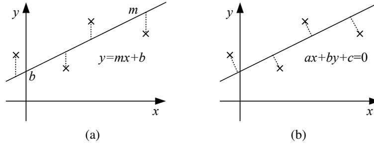
**Figure A.2** Least squares regression. (a) The line  $y = mx + b$  is fit to the four noisy data points,  $\{(x_i, y_i)\}$ , denoted by  $\times$  by minimizing the squared vertical residuals between the data points and the line,  $\sum_i \|y_i - (mx_i + b)\|^2$ . (b) When the measurements  $\{(x_i, y_i)\}$  are assumed to have noise in all directions, the sum of orthogonal squared distances to the line  $\sum_i \|ax_i + by_i + c\|^2$  is minimized using total least squares.
