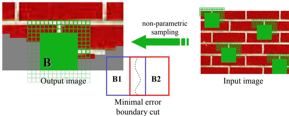
**Figure 10.51** Texture synthesis by image quilting (Efros and Freeman 2001). Instead of generating a single pixel at a time, larger blocks are copied from the source texture. The transitions in the overlap regions between the selected blocks are then optimized using dynamic programming. (Figure courtesy of Alyosha Efros.)
