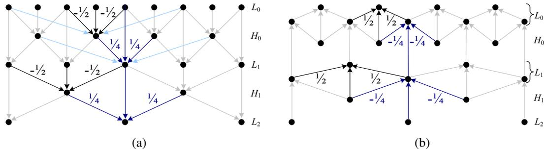
**Figure 3.39** Lifted transform shown as a signal processing diagram: (a) The analysis stage first predicts the odd value from its even neighbors, stores the difference wavelet, and then compensates the coarser even value by adding in a fraction of the wavelet. (b) The synthesis stage simply reverses the flow of computation and the signs of some of the filters and operations. The light blue lines show what happens if we use four taps for the prediction and correction instead of just two.
