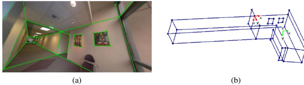
**Figure 12.15** Interactive 3D modeling from panoramas (Shum, Han, and Szeliski 1998) © 1998 IEEE: (a) wide-angle view of a panorama with user-drawn vertical and horizontal (axis-aligned) lines; (b) single-view reconstruction of the corridors.
