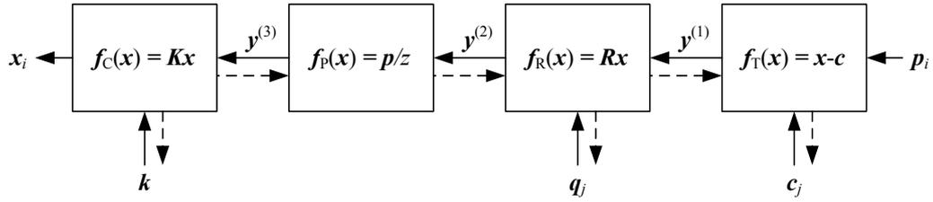
**Figure 6.5** A set of chained transforms for projecting a 3D point  $p_i$  to a 2D measurement  $x_i$  through a series of transformations  $f^{(k)}$ , each of which is controlled by its own set of parameters. The dashed lines indicate the flow of information as partial derivatives are computed during a backward pass.
