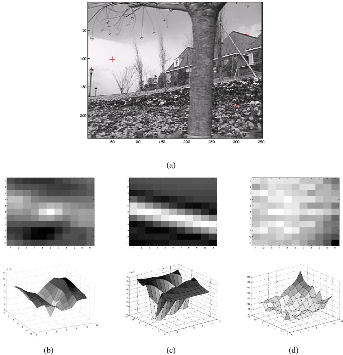
**Figure 4.5** Three auto-correlation surfaces  $E_{AC}(\Delta \mathbf{u})$  shown as both grayscale images and surface plots: (a) The original image is marked with three red crosses to denote where the auto-correlation surfaces were computed; (b) this patch is from the flower bed (good unique minimum); (c) this patch is from the roof edge (one-dimensional aperture problem); and (d) this patch is from the cloud (no good peak). Each grid point in figures b–d is one value of  $\Delta \mathbf{u}$ .
