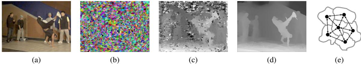
**Figure 11.12** Segmentation-based stereo matching (Zitnick, Kang, Uyttendaele *et al.* 2004) © 2004 ACM: (a) input color image; (b) color-based segmentation; (c) initial disparity estimates; (d) final piecewise-smoothed disparities; (e) MRF neighborhood defined over the segments in the disparity space distribution (Zitnick and Kang 2007) © 2007 Springer.
