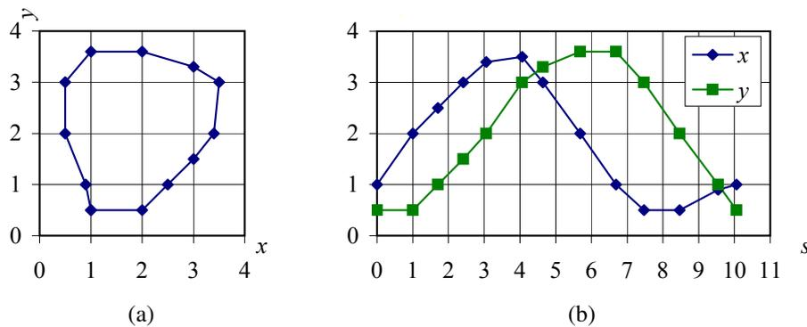
**Figure 4.35** Arc-length parameterization of a contour: (a) discrete points along the contour are first transcribed as (b)  $(x, y)$  pairs along the arc length  $s$ . This curve can then be regularly re-sampled or converted into alternative (e.g., Fourier) representations.
