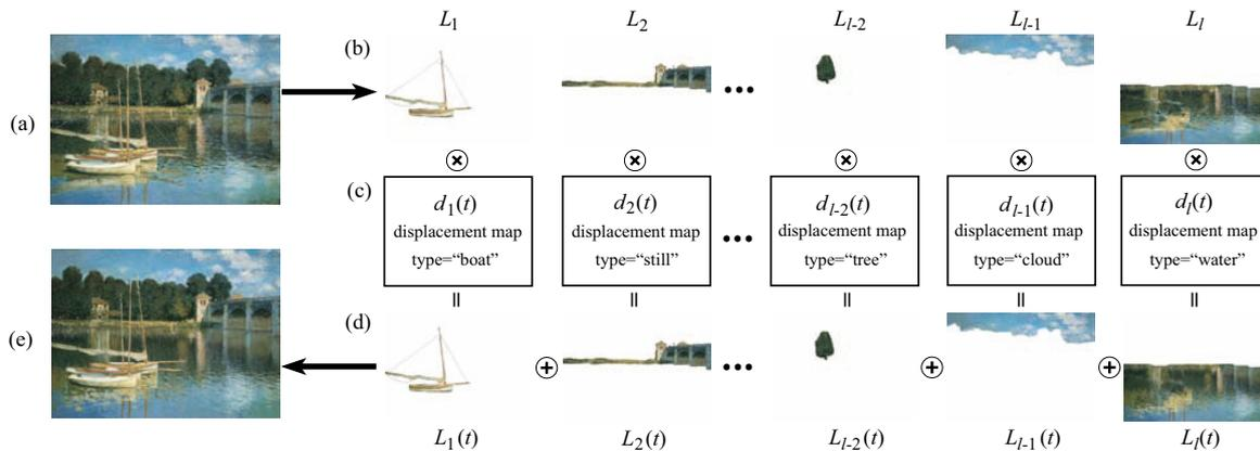
**Figure 13.14** Animating still pictures (Chuang, Goldman, Zheng *et al.* 2005) © 2005 ACM. (a) The input still image is manually segmented into (b) several layers. (c) Each layer is then animated with a different stochastic motion texture (d) The animated layers are then composited to produce (e) the final animation
