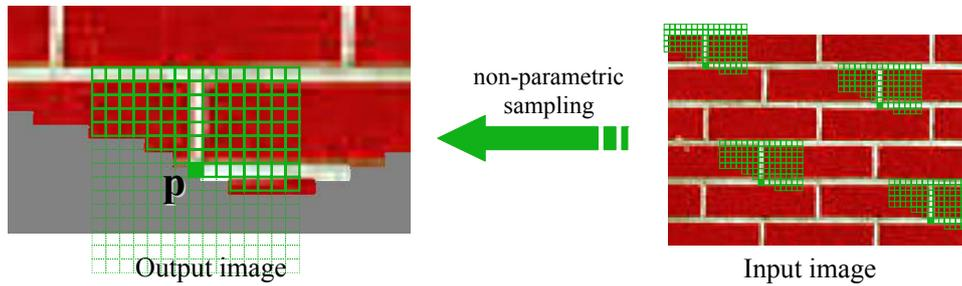
**Figure 10.50** Texture synthesis using non-parametric sampling (Efros and Leung 1999). The value of the newest pixel  $p$  is randomly chosen from similar local (partial) patches in the source texture (input image). (Figure courtesy of Alyosha Efros.)
