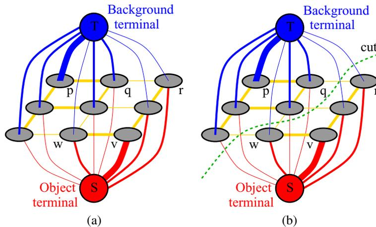
**Figure B.3** Graph cuts for minimizing binary sub-modular MRF energies (Boykov and Jolly 2001) © 2001 IEEE: (a) energy function encoded as a max flow problem; (b) the minimum cut determines the region boundary.
