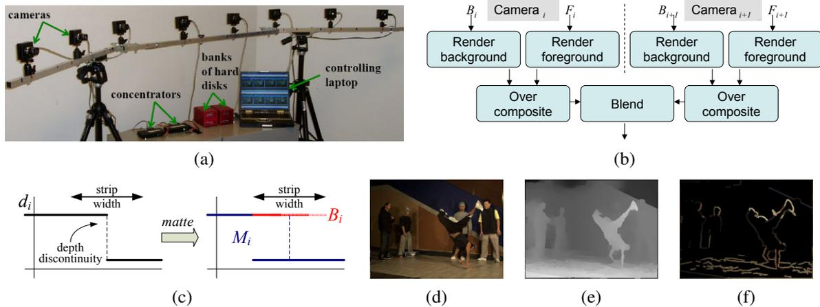
**Figure 13.15** Video view interpolation (Zitnick, Kang, Uyttendaele *et al.* 2004) © 2004 ACM: (a) the capture hardware consists of eight synchronized cameras; (b) the background and foreground images from each camera are rendered and composited before blending; (c) the two-layer representation, before and after boundary matting; (d) background color estimates; (e) background depth estimates; (f) foreground color estimates.
