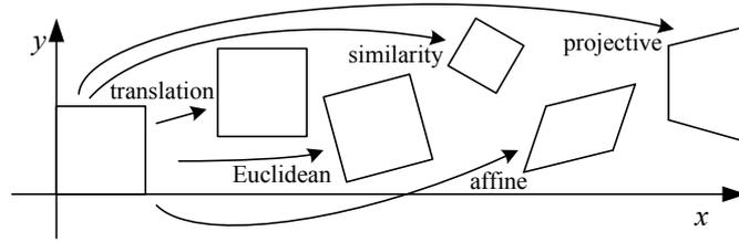
**Figure 2.4** Basic set of 2D planar transformations.
