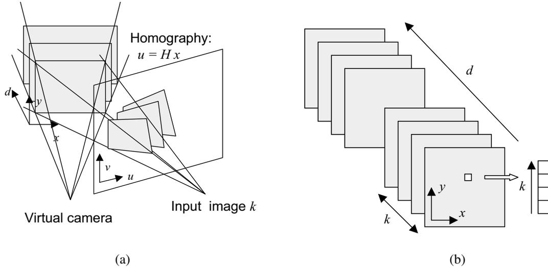
**Figure 11.6** Sweeping a set of planes through a scene (Szeliski and Golland 1999) © 1999 Springer: (a) The set of planes seen from a virtual camera induces a set of homographies in any other source (input) camera image. (b) The warped images from all the other cameras can be stacked into a generalized disparity space volume  $\tilde{I}(x, y, d, k)$  indexed by pixel location  $(x, y)$ , disparity  $d$ , and camera  $k$ .
