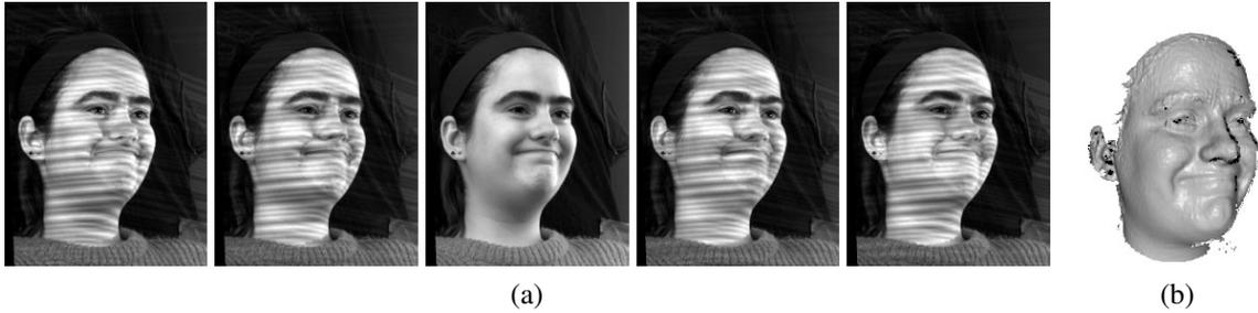
**Figure 12.7** Real-time dense 3D face capture using spacetime stereo (Zhang, Snavely, Curless *et al.* 2004) © 2004 ACM: (a) set of five consecutive video frames from one of two stereo cameras (every fifth frame is free of stripe patterns, in order to extract texture); (b) resulting high-quality 3D surface model (depth map visualized as a shaded rendering).
