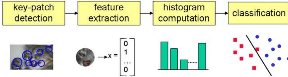
**Figure 14.36** A typical processing pipeline for a bag-of-words category recognition system (Csurka, Dance, Perronnin *et al.* 2006) © 2007 Springer. Features are first extracted at keypoints and then quantized to get a distribution (histogram) over the learned *visual words* (feature cluster centers). The feature distribution histogram is used to learn a decision surface using a classification algorithm, such as a support vector machine.
