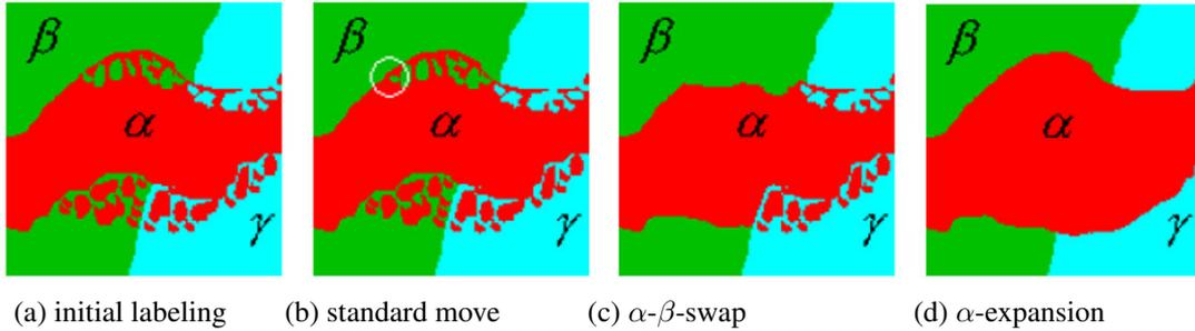
**Figure B.4** Multi-level graph optimization from (Boykov, Veksler, and Zabih 2001) © 2001 IEEE: (a) initial problem configuration; (b) the standard move changes only one pixel; (c) the  $\alpha$ - $\beta$ -swap optimally exchanges all  $\alpha$ - and  $\beta$ -labeled pixels; (d) the  $\alpha$ -expansion move optimally selects among current pixel values and the  $\alpha$  label.
