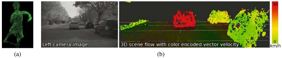
**Figure 11.18** Three-dimensional scene flow: (a) computed from a multi-camera dome surrounding the dancer shown in Figure 11.2h–j (Vedula, Baker, Rander *et al.* 2005) © 2005 IEEE; (b) computed from stereo cameras mounted on a moving vehicle (Wedel, Rabe, Vaudrey *et al.* 2008) © 2008 Springer.
