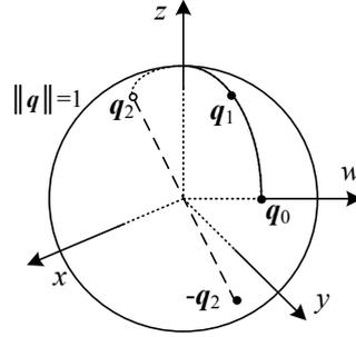
**Figure 2.6** Unit quaternions live on the unit sphere  $\|q\| = 1$ . This figure shows a smooth trajectory through the three quaternions  $q_0$ ,  $q_1$ , and  $q_2$ . The *antipodal* point to  $q_2$ , namely  $-q_2$ , represents the same rotation as  $q_2$ .
