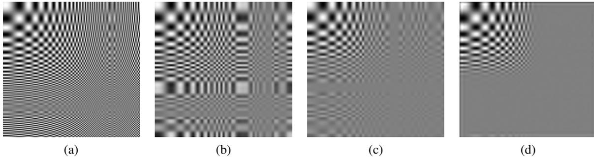
**Figure 2.25** Aliasing of a two-dimensional signal: (a) original full-resolution image; (b) downsampled  $4\times$  with a 25% fill factor box filter; (c) downsampled  $4\times$  with a 100% fill factor box filter; (d) downsampled  $4\times$  with a high-quality 9-tap filter. Notice how the higher frequencies are aliased into visible frequencies with the lower quality filters, while the 9-tap filter completely removes these higher frequencies.
