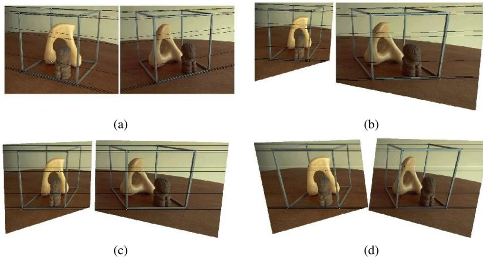
**Figure 11.4** The multi-stage stereo rectification algorithm of Loop and Zhang (1999) © 1999 IEEE. (a) Original image pair overlaid with several epipolar lines; (b) images transformed so that epipolar lines are parallel; (c) images rectified so that epipolar lines are horizontal and in vertical correspondence; (d) final rectification that minimizes horizontal distortions.
