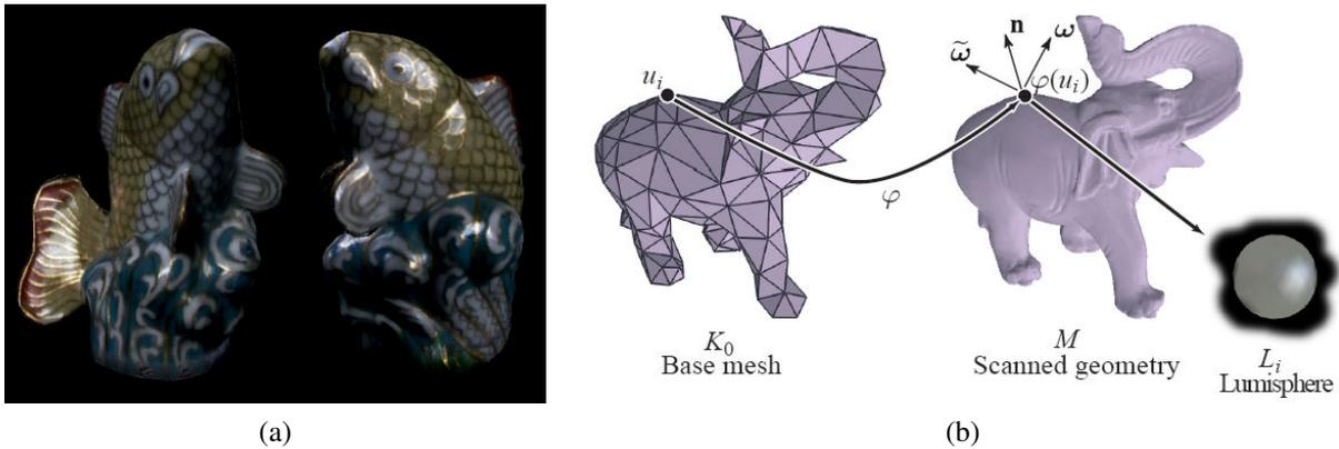
**Figure 13.9** Surface light fields (Wood, Azuma, Aldinger *et al.* 2000) © 2000 ACM: (a) example of a highly specular object with strong inter-reflections; (b) the surface light field stores the light emanating from each surface point in all visible directions as a “Lumisphere”.
