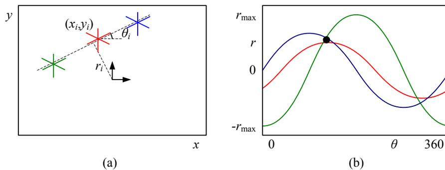
**Figure 4.41** Original Hough transform: (a) each point votes for a complete family of potential lines  $r_i(\theta) = x_i \cos \theta + y_i \sin \theta$ ; (b) each pencil of lines sweeps out a sinusoid in  $(r, \theta)$ ; their intersection provides the desired line equation.
