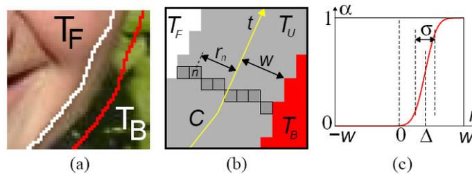
**Figure 10.38** Softening a hard segmentation boundary (border matting) (Rother, Kolmogorov, and Blake 2004) © 2004 ACM: (a) the region surrounding a segmentation boundary where pixels of mixed foreground and background colors are visible; (b) pixel values along the boundary are used to compute a soft alpha matte; (c) at each point along the curve  $t$ , a displacement  $\Delta$  and a width  $\sigma$  are estimated.
