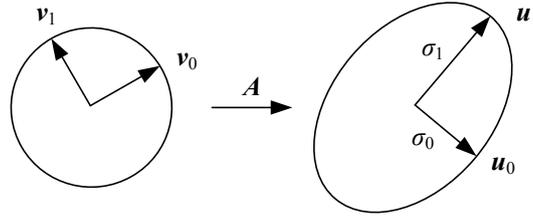
**Figure A.1** The action of a matrix  $A$  can be visualized by thinking of the domain as being spanned by a set of orthonormal vectors  $v_j$ , each of which is transformed to a new orthogonal vector  $u_j$  with a length  $\sigma_j$ . When  $A$  is interpreted as a covariance matrix and its eigenvalue decomposition is performed, each of the  $u_j$  axes denote a principal direction (component) and each  $\sigma_j$  denotes one standard deviation along that direction.
