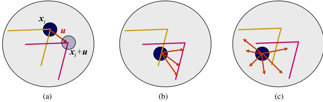
**Figure 4.4** Aperture problems for different image patches: (a) stable (“corner-like”) flow; (b) classic aperture problem (barber-pole illusion); (c) textureless region. The two images  $I_0$  (yellow) and  $I_1$  (red) are overlaid. The red vector  $\mathbf{u}$  indicates the displacement between the patch centers and the  $w(\mathbf{x}_i)$  weighting function (patch window) is shown as a dark circle.
