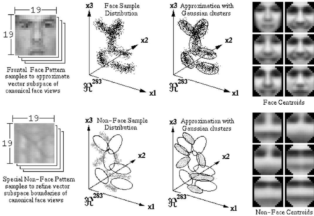
**Figure 14.4** Learning a mixture of Gaussians model for face detection (Sung and Poggio 1998) © 1998 IEEE. The face and non-face images ( $19^2$ -long vectors) are first clustered into six separate clusters (each) using k-means and then analyzed using PCA. The cluster centers are shown in the right-hand columns.
