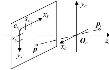
**Figure 2.8** Projection of a 3D camera-centered point  $p_c$  onto the sensor planes at location  $p$ .  $O_c$  is the camera center (nodal point),  $c_s$  is the 3D origin of the sensor plane coordinate system, and  $s_x$  and  $s_y$  are the pixel spacings.
