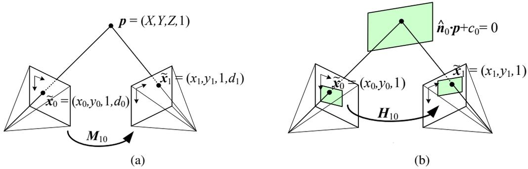
**Figure 2.12** A point is projected into two images: (a) relationship between the 3D point coordinate  $(X, Y, Z, 1)$  and the 2D projected point  $(x, y, 1, d)$ ; (b) planar homography induced by points all lying on a common plane  $\hat{\mathbf{n}}_0 \cdot \mathbf{p} + c_0 = 0$ .
