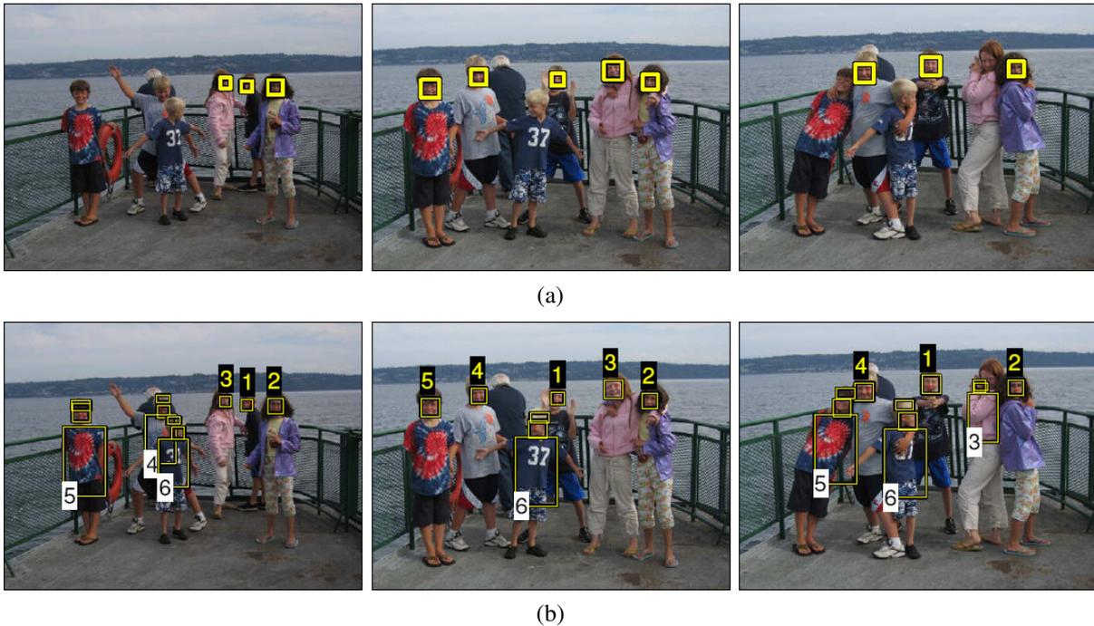
**Figure 14.25** Person detection and re-recognition using a combined face, hair, and torso model (Sivic, Zitnick, and Szeliski 2006) © 2006 Springer. (a) Using face detection alone, several of the heads are missed. (b) The combined face and clothing model successfully re-finds all the people.
