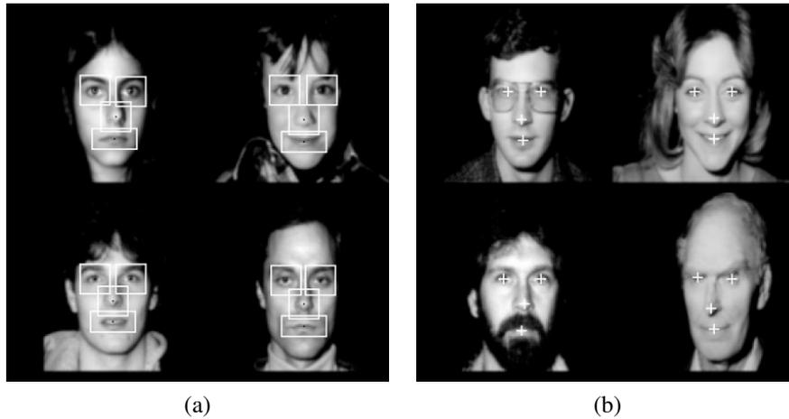
**Figure 14.18** Modular eigenspace for face recognition (Moghaddam and Pentland 1997) © 1997 IEEE. (a) By detecting separate features in the faces (eyes, nose, mouth), separate eigenspaces can be estimated for each one. (b) The relative positions of each feature can be detected at recognition time, thus allowing for more flexibility in viewpoint and expression.
