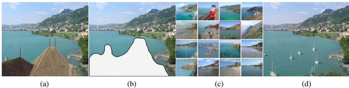
**Figure 14.46** Scene completion using millions of photographs (Hays and Efros 2007) © 2007 ACM: (a) original image; (b) after unwanted foreground removal; (c) plausible scene matches, with the one the user selected highlighted in red; (d) output image after replacement and blending.
