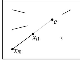
**Figure 7.4** Pure translational camera motion results in visual motion where all the points move towards (or away from) a common *focus of expansion* (FOE)  $e$ . They therefore satisfy the triple product condition  $(\mathbf{x}_0, \mathbf{x}_1, \mathbf{e}) = \mathbf{e} \cdot (\mathbf{x}_0 \times \mathbf{x}_1) = 0$ .
