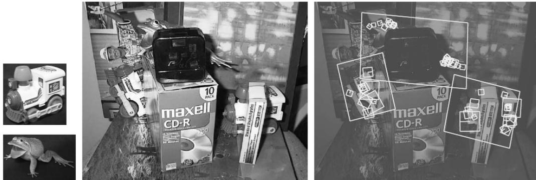
**Figure 14.26** Recognizing objects in a cluttered scene (Lowe 2004) © 2004 Springer. Two of the training images in the database are shown on the left. They are matched to the cluttered scene in the middle using SIFT features, shown as small squares in the right image. The affine warp of each recognized database image onto the scene is shown as a larger parallelogram in the right image.
