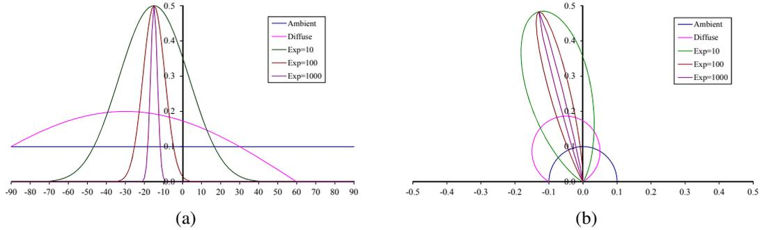
**Figure 2.18** Cross-section through a Phong shading model BRDF for a fixed incident illumination direction: (a) component values as a function of angle away from surface normal; (b) polar plot. The value of the Phong exponent  $k_e$  is indicated by the “Exp” labels and the light source is at an angle of  $30^\circ$  away from the normal.
