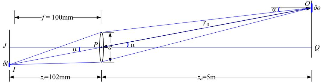
**Figure 2.22** The amount of light hitting a pixel of surface area  $\delta i$  depends on the square of the ratio of the aperture diameter  $d$  to the focal length  $f$ , as well as the fourth power of the off-axis angle  $\alpha$  cosine,  $\cos^4 \alpha$ .
