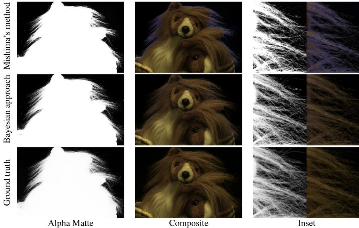
**Figure 10.40** Blue-screen matting results (Chuang, Curless, Salesin *et al.* 2001) © 2001 IEEE. Mishima’s method produces visible blue spill (color fringing in the hair), while Chuang’s Bayesian matting approach produces accurate results.
