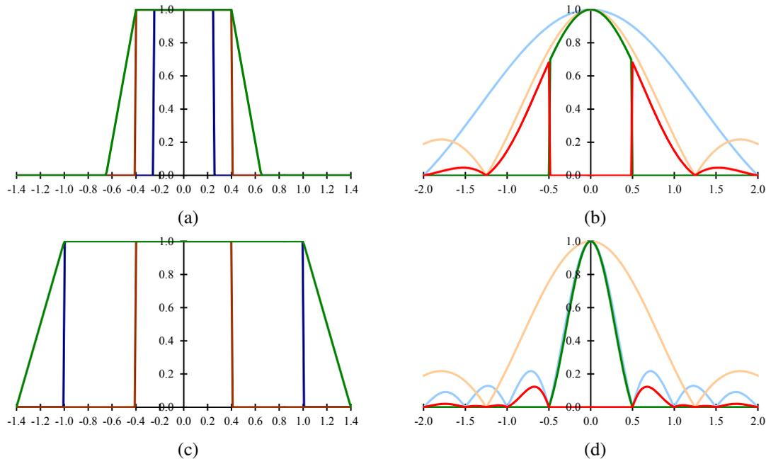
**Figure 2.26** Sample point spread functions (PSF): The diameter of the blur disc (blue) in (a) is equal to half the pixel spacing, while the diameter in (c) is twice the pixel spacing. The horizontal fill factor of the sensing chip is 80% and is shown in brown. The convolution of these two kernels gives the point spread function, shown in green. The Fourier response of the PSF (the MTF) is plotted in (b) and (d). The area above the Nyquist frequency where aliasing occurs is shown in red.
