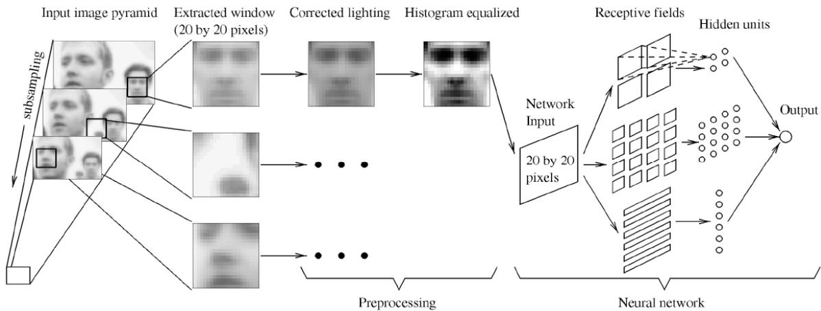
**Figure 14.5** A neural network for face detection (Rowley, Baluja, and Kanade 1998a) © 1998 IEEE. Overlapping patches are extracted from different levels of a pyramid and then pre-processed as shown in Figure 14.3b. A three-layer neural network is then used to detect likely face locations.
