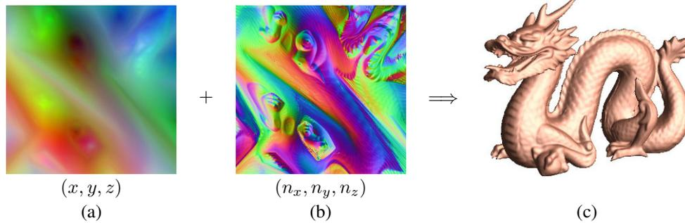
**Figure 12.12** Geometry images (Gu, Gortler, and Hoppe 2002) © 2002 ACM: (a) the  $257 \times 257$  geometry image defines a mesh over the surface; (b) the  $512 \times 512$  normal map defines vertex normals; (c) final lit 3D model.
