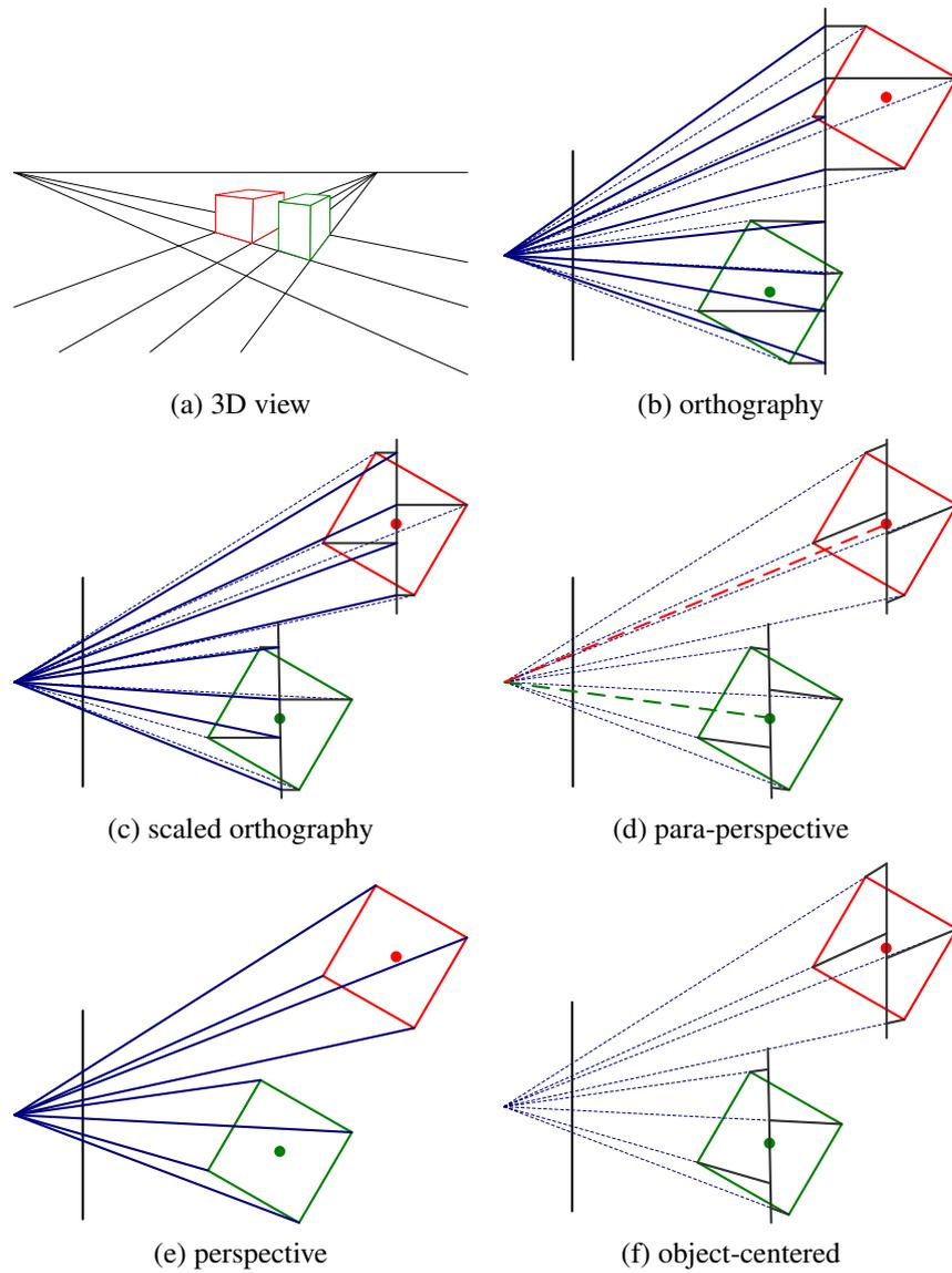
**Figure 2.7** Commonly used projection models: (a) 3D view of world, (b) orthography, (c) scaled orthography, (d) para-perspective, (e) perspective, (f) object-centered. Each diagram shows a top-down view of the projection. Note how parallel lines on the ground plane and box sides remain parallel in the non-perspective projections.
