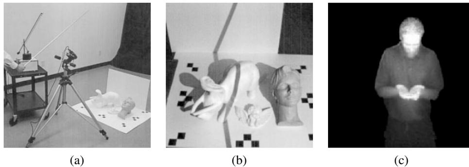
**Figure 12.6** Shape scanning using cast shadows (Bouguet and Perona 1999) © 1999 Springer: (a) camera setup with a point light source (a desk lamp without its reflector), a hand-held stick casting a shadow, and (b) the objects being scanned in front of two planar backgrounds. (c) Real-time depth map using a pulsed illumination system (Iddan and Yahav 2001) © 2001 SPIE.
