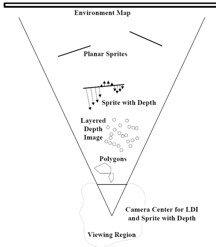
**Figure 13.5** A variety of image-based rendering primitives, which can be used depending on the distance between the camera and the object of interest (Shade, Gortler, He *et al.* 1998) © 1998 ACM. Closer objects may require more detailed polygonal representations, while mid-level objects can use a layered depth image (LDI), and far-away objects can use sprites (potentially with depth) and environment maps.
