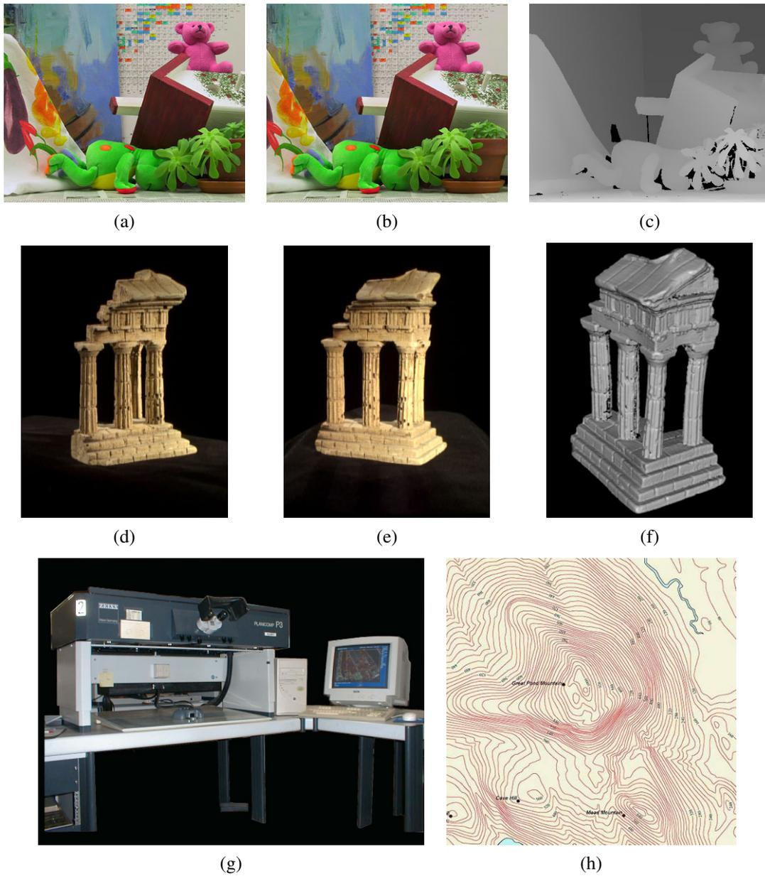
**Figure 11.1** Stereo reconstruction techniques can convert (a–b) a pair of images into (c) a depth map (<http://vision.middlebury.edu/stereo/data/scenes2003/>) or (d–e) a sequence of images into (f) a 3D model (<http://vision.middlebury.edu/mview/data/>). (g) An analytical stereo plotter, courtesy of Kenney Aerial Mapping, Inc., can generate (h) contour plots.
