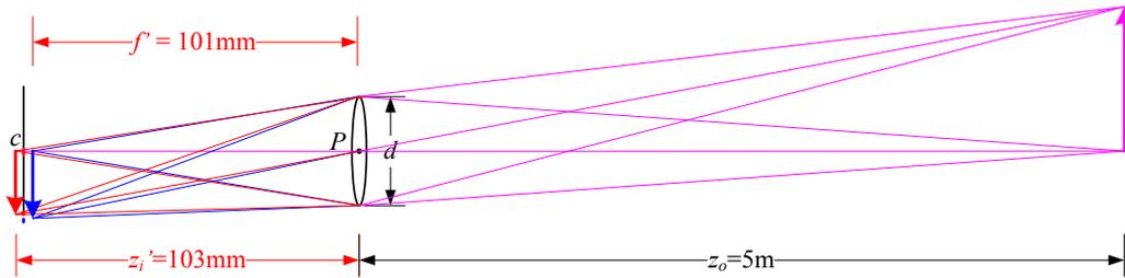
**Figure 2.21** In a lens subject to *chromatic aberration*, light at different wavelengths (e.g., the red and blue arrows) is focused with a different focal length  $f'$  and hence a different depth  $z_i'$ , resulting in both a geometric (in-plane) displacement and a loss of focus.
