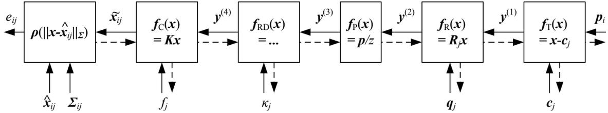
**Figure 7.7** A set of chained transforms for projecting a 3D point  $p_i$  into a 2D measurement  $x_{ij}$  through a series of transformations  $f^{(k)}$ , each of which is controlled by its own set of parameters. The dashed lines indicate the flow of information as partial derivatives are computed during a backward pass. The formula for the radial distortion function is  $f_{RD}(\mathbf{x}) = (1 + \kappa_1 r^2 + \kappa_2 r^4)\mathbf{x}$ .
