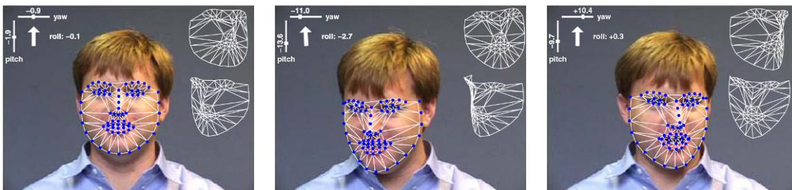
**Figure 14.24** Head tracking with 3D AAMs (Matthews, Xiao, and Baker 2007) © 2007 Springer. Each image shows a video frame along with the estimate yaw, pitch, and roll parameters and the fitted 3D deformable mesh.
