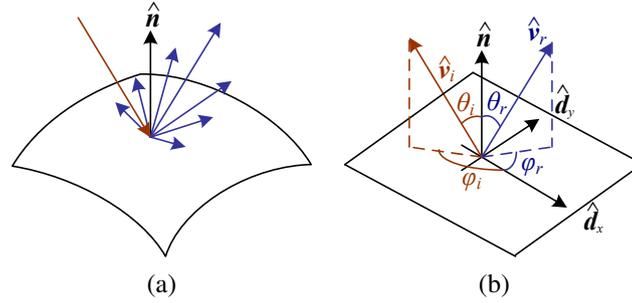
**Figure 2.15** (a) Light scatters when it hits a surface. (b) The bidirectional reflectance distribution function (BRDF)  $f(\theta_i, \phi_i, \theta_r, \phi_r)$  is parameterized by the angles that the incident,  $\hat{v}_i$ , and reflected,  $\hat{v}_r$ , light ray directions make with the local surface coordinate frame  $(\hat{d}_x, \hat{d}_y, \hat{n})$ .
