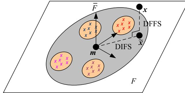
**Figure 14.14** Projection onto the linear subspace spanned by the eigenface images (Moghaddam and Pentland 1997) © 1997 IEEE. The distance from face space (DFFS) is the orthogonal distance to the plane, while the distance in face space (DIFS) is the distance along the plane from the mean image. Both distances can be turned into Mahalanobis distances and given probabilistic interpretations.
