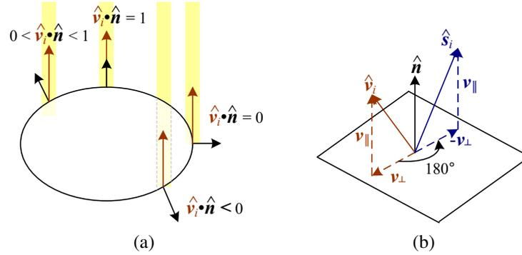
**Figure 2.17** (a) The diminution of returned light caused by *foreshortening* depends on  $\hat{v}_i \cdot \hat{n}$ , the cosine of the angle between the incident light direction  $\hat{v}_i$  and the surface normal  $\hat{n}$ . (b) Mirror (specular) reflection: The incident light ray direction  $\hat{v}_i$  is reflected onto the specular direction  $\hat{s}_i$  around the surface normal  $\hat{n}$ .
