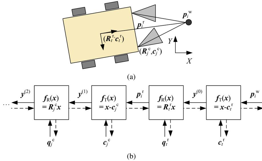
**Figure 7.8** A camera rig and its associated transform chain. (a) As the mobile rig (robot) moves around in the world, its pose with respect to the world at time  $t$  is captured by  $(R_t^r, c_t^r)$ . Each camera's pose with respect to the rig is captured by  $(R_j^c, c_j^c)$ . (b) A 3D point with world coordinates  $p_i^w$  is first transformed into rig coordinates  $p_i^r$ , and then through the rest of the camera-specific chain, as shown in Figure 7.7.
