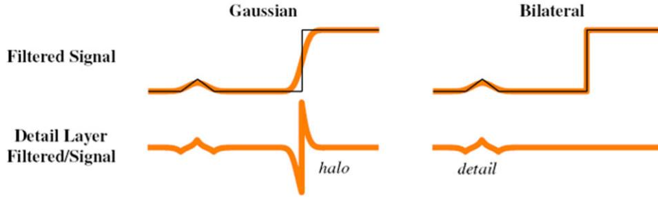
**Figure 10.23** Gaussian vs. bilateral filtering (Petschnigg, Agrawala, Hoppe *et al.* 2004) © 2004 ACM: A Gaussian low-pass filter blurs across all edges and therefore creates strong peaks and valleys in the detail image that cause halos. The bilateral filter does not smooth across strong edges and thereby reduces halos while still capturing detail.
