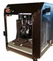
integrated scanning, dispensing and motion control systems for DW. Both companies have a wide range of nozzle designs, and have feedback systems in place to make sure that the stand-off distance between the nozzle and the substrate remains substantially constant; to enable repeatable and accurate deposition of traces across conformal surfaces.
