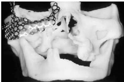
**Fig. 15.3** Titanium mesh formed around a maxillofacial model
