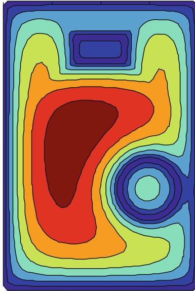
**Fig. 11.17** Material distribution, light indicates hard material
