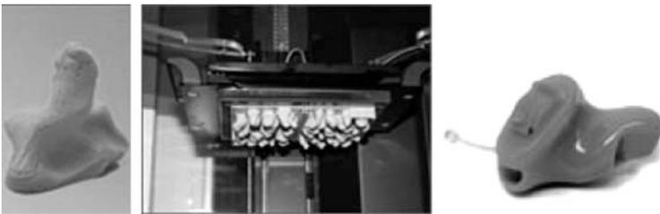
**Fig. 2.9** RM of custom hearing aids, from a wax ear impression, on to the machine to the final product (photo courtesy of Phonak)
