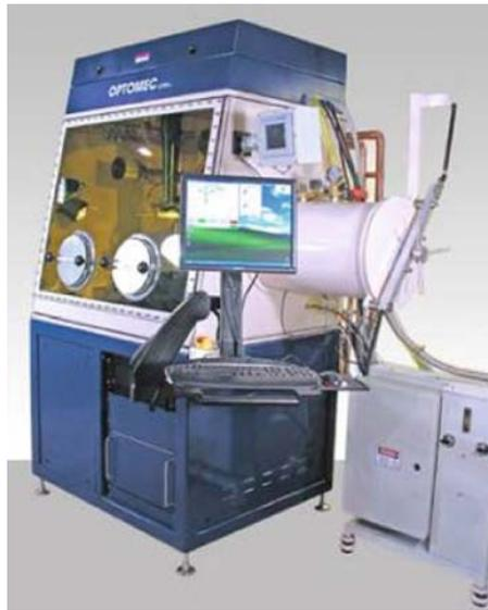
**Fig. 9.6** Optomec LENS 750 system (courtesy Optomec)
