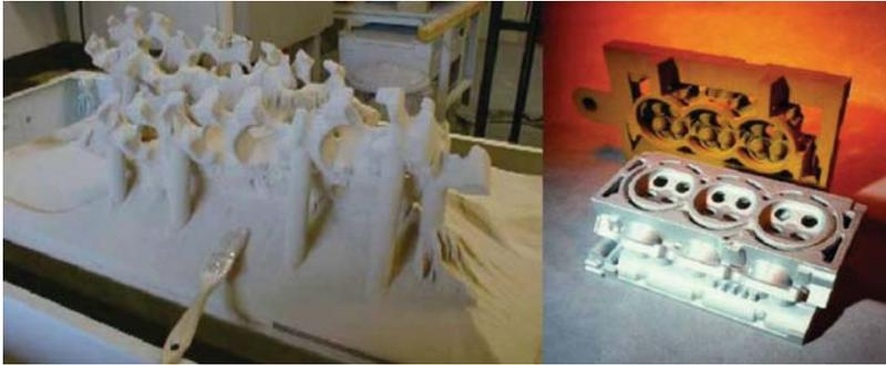
**Fig. 16.12** Sand casting pattern for a cylinder head of a V6, 24-valve car engine (*left*) during loose powder removal and (*right*) pattern prepared for casting alongside a finished casting. (Joint project between CAD/CAM Becker GmbH and VAW Südalumin GmbH, made on an EOSINT S laser-sintering machine, courtesy EOS)
