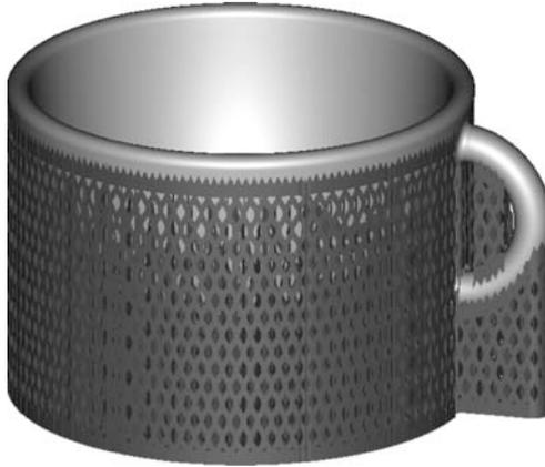
square pattern or something more complex like a hexagonal or even a fractal mesh. Furthermore, the lattice could be connected to the part with a tapered region that may be more convenient to remove when compared with thicker connecting edges.
