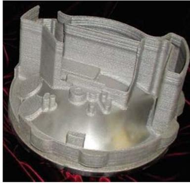
Council's Integrated Manufacturing Technologies Institute. The key features of this process are the small spot-size laser, accurate motion control, and single-nozzle powder feeding. This enables the creation of small parts with much better accuracy and surface finish than other BD processes, but with the drawback of a significantly lower deposition rate.
