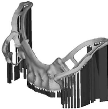
processes the metal supports are often too strong to be removed by hand; and thus the use of milling, band-saws, cut-off blades, wire-EDM and other metal cutting techniques are widely employed.
