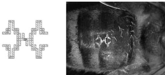
**Fig. 10.11** 35-GHz fractal antenna design (*left*) and MAPLE-DW printed antenna on the abdomen of a dead drone honeybee (*right*). (Courtesy Douglas B. Chrisey)
