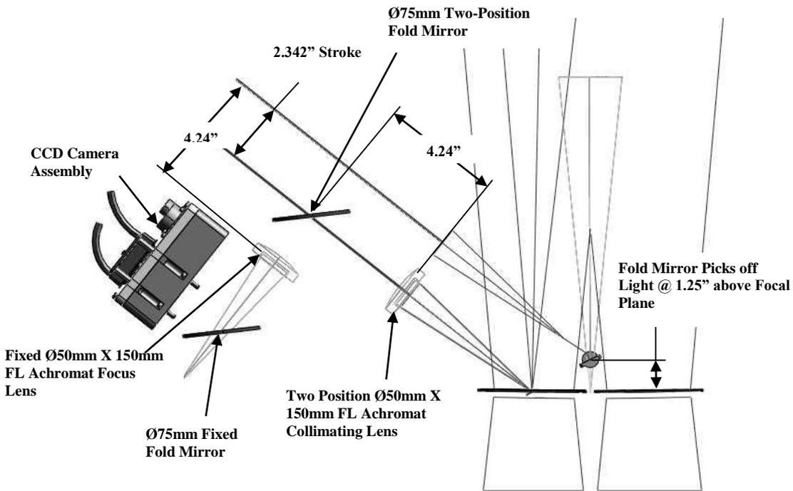
Figure 5. Single Object Guider (SOG). The SOG can be used to locate a star at the center of the field of view or to look a spilled light long slit on a special slit mask frame. The fold mirror at the center of the field of view is 20 mm in diameter and is placed at an angle of  $27.5^\circ$  to bend the light path by  $55^\circ$ . The mirror has a projected width of 17.7 mm. The 13.3 mm field of the CCD would require a 19.3 mm diameter mirror, so the edges of the image will be vignetted.
