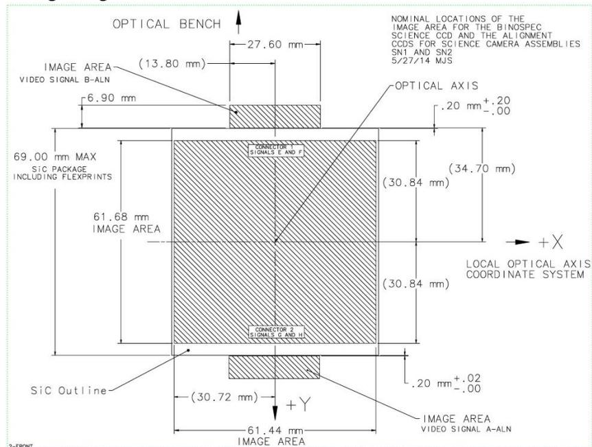
**Figure 2. Binospec detector focal plane layout. A pair of fiber images will appear in each flexure control CCD.**
