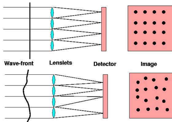
Figure 4. Principle of a Shack Hartmann wave front sensor
